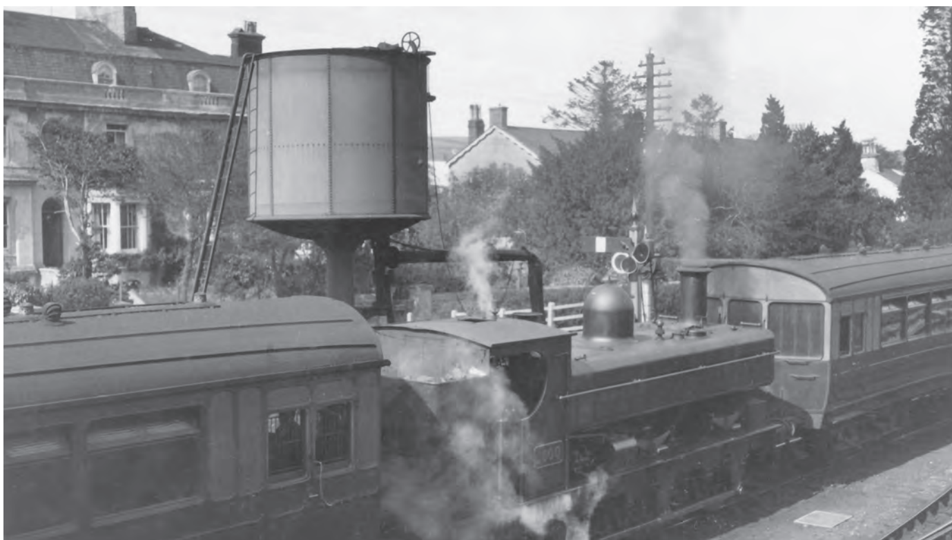
1600 , built in November 1879 and rebuilt as a pannier tank in 1924, in an auto train 'sandwich' at an unknown location, c1930. It was withdrawn from Pontypool Road shed in 1937. (GW Trust/P.J. Reed Collection)
