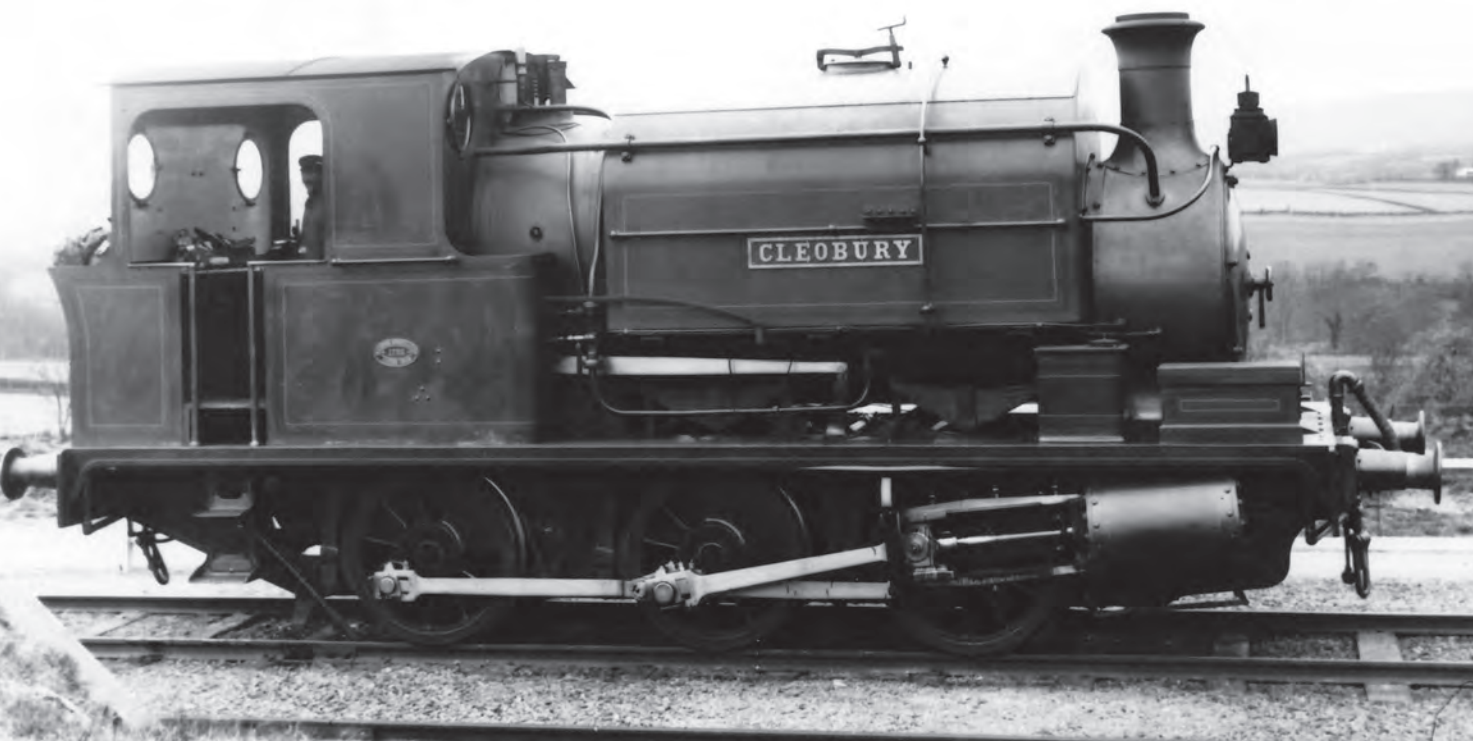
Cleobury , a Manning Wardle 0-6-0 saddle tank of 1908, rebuilt later as a pannier tank in 1931, here c1912. (MLS)
