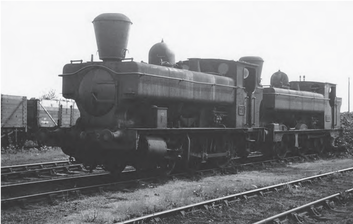
GW 29 with '2021' class 2051, both equipped with spark arrester chimneys, at Kidderminster, 3 June 1951. (MLS/N.H. Spilsbury)
