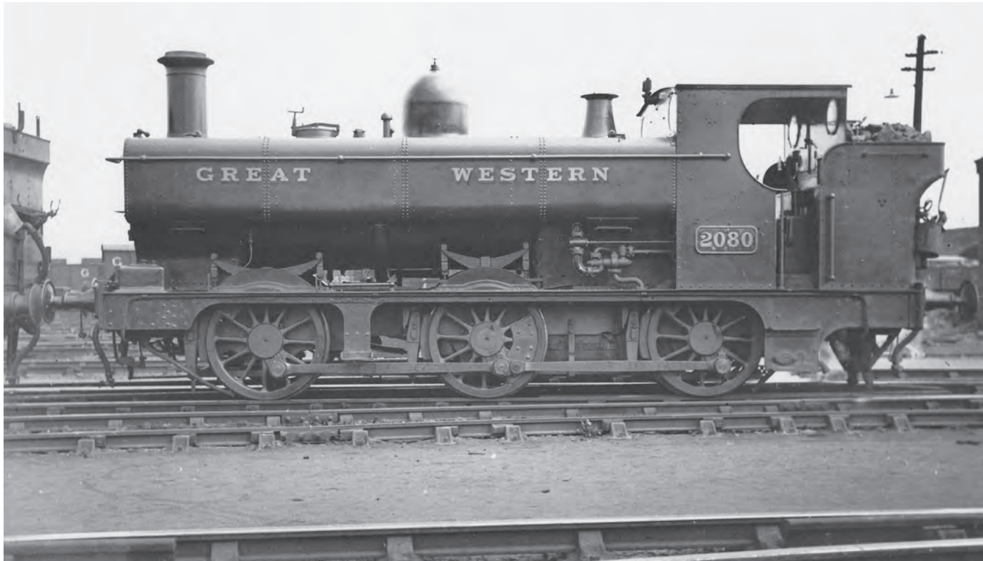
2080 restored to conventional '2021' design with 4ft 1½in diameter wheels, at Pontypool Road, 10 May 1936. (F.K. Davies/John Hodge Collection)
