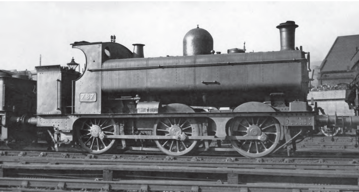
'655' class No.767, built in February 1892, and converted as a pannier tank in March 1921, took the number of an earlier '645' class engine sold to the South Wales Mineral Railway in 1875. It is shown here shortly before withdrawal in October 1934. (MLS)
