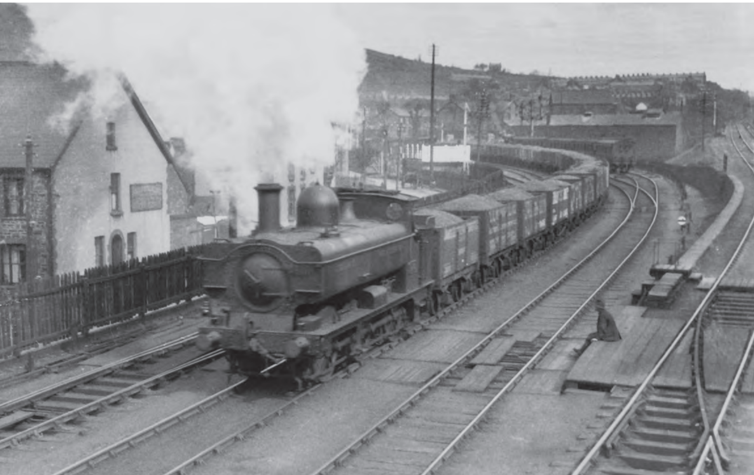
1826 , built in 1882 as a 0-6-0 side tank, rebuilt in 1897 as a saddle tank and as a pannier tank in 1911, on a coal train at Abercynon off the Aberdare line, c1922. (John Hodge Collection)
