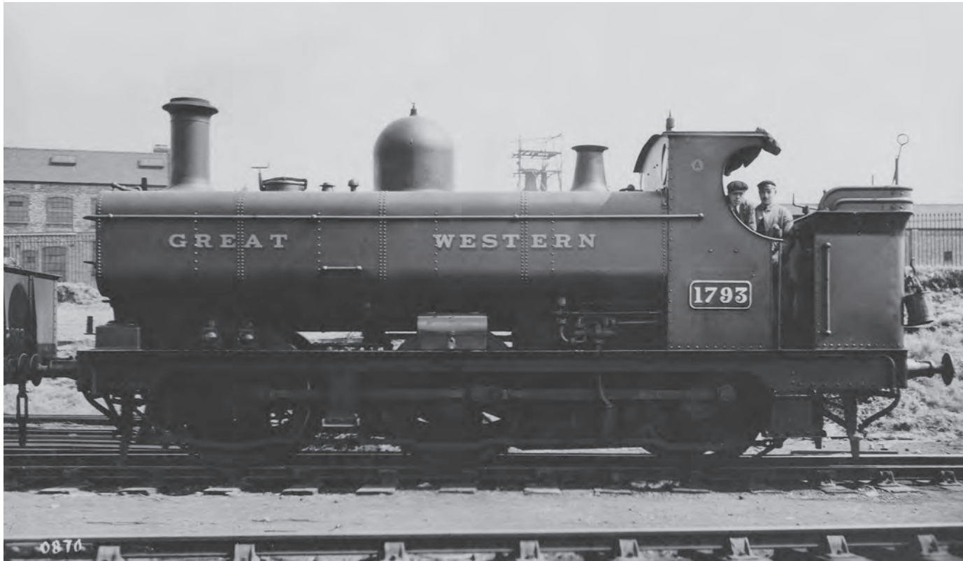
1793 , built in May 1895, rebuilt with pannier tanks in February 1921, seen here c1923 before receiving an enclosed cab and enlarged bunker. (MLS)
