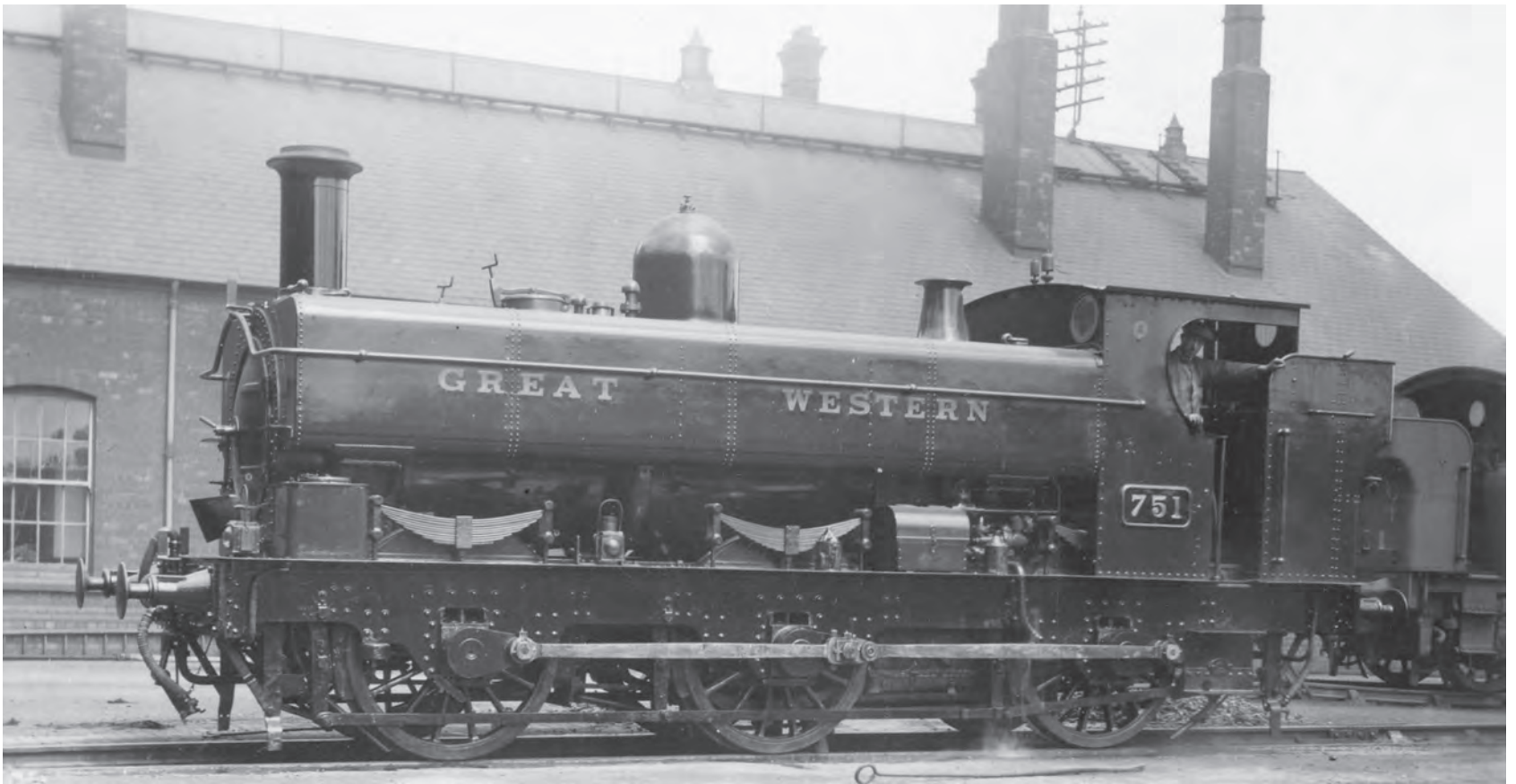
751 , built in March 1873 and rebuilt with pannier tanks in April 1915, at Swindon after equipping with enlarged bunker and enclosed cab, c1924. (GW Trust/P.J. Reed Collection)
