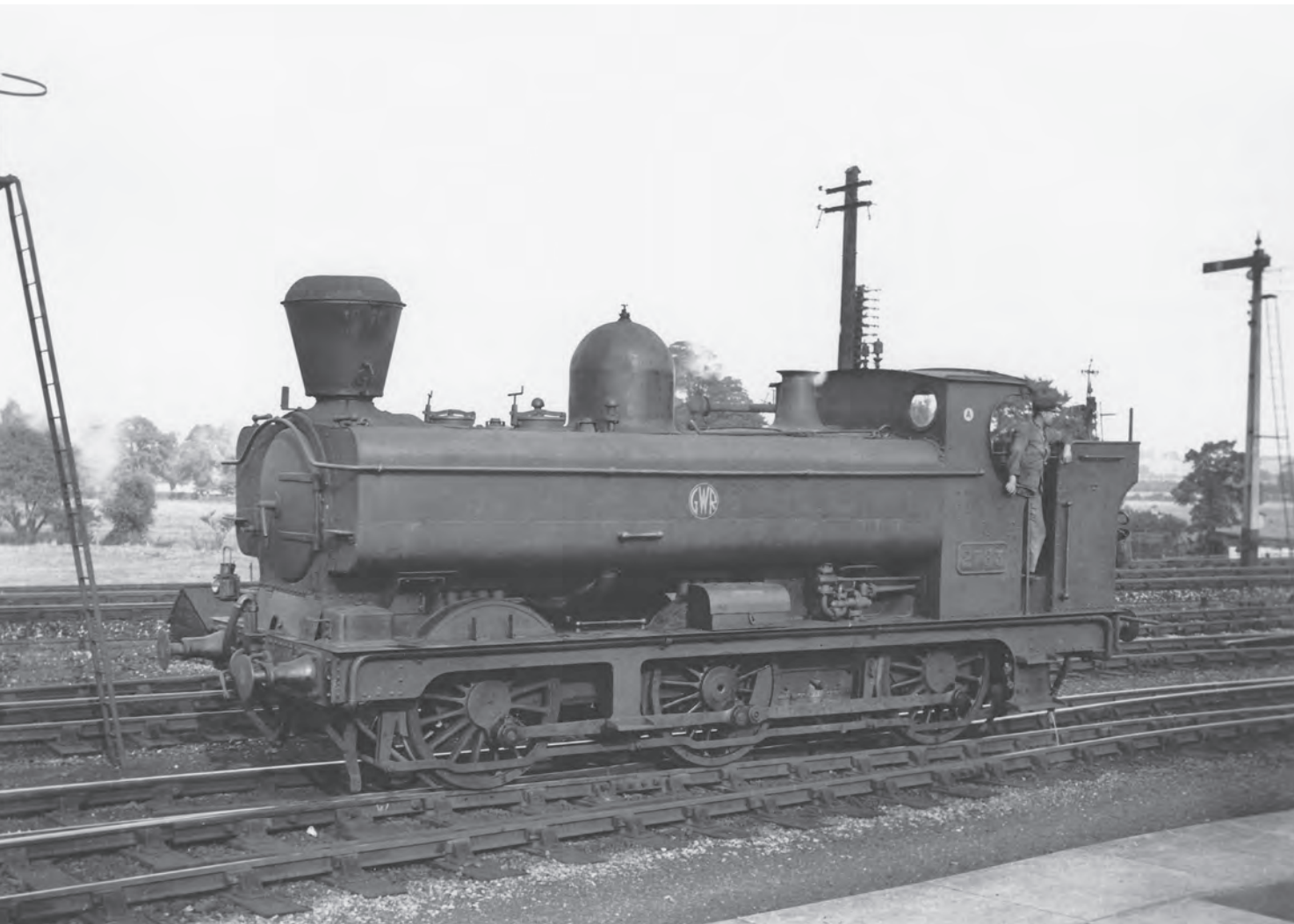
2783 , built in January 1901 and rebuilt with pannier tanks in October 1913, at Didcot, fitted with spark arrester chimney for shunting in the Ordnance depot at Milton, 26 September 1937. (F.K. Davies/John Hodge Collection)
