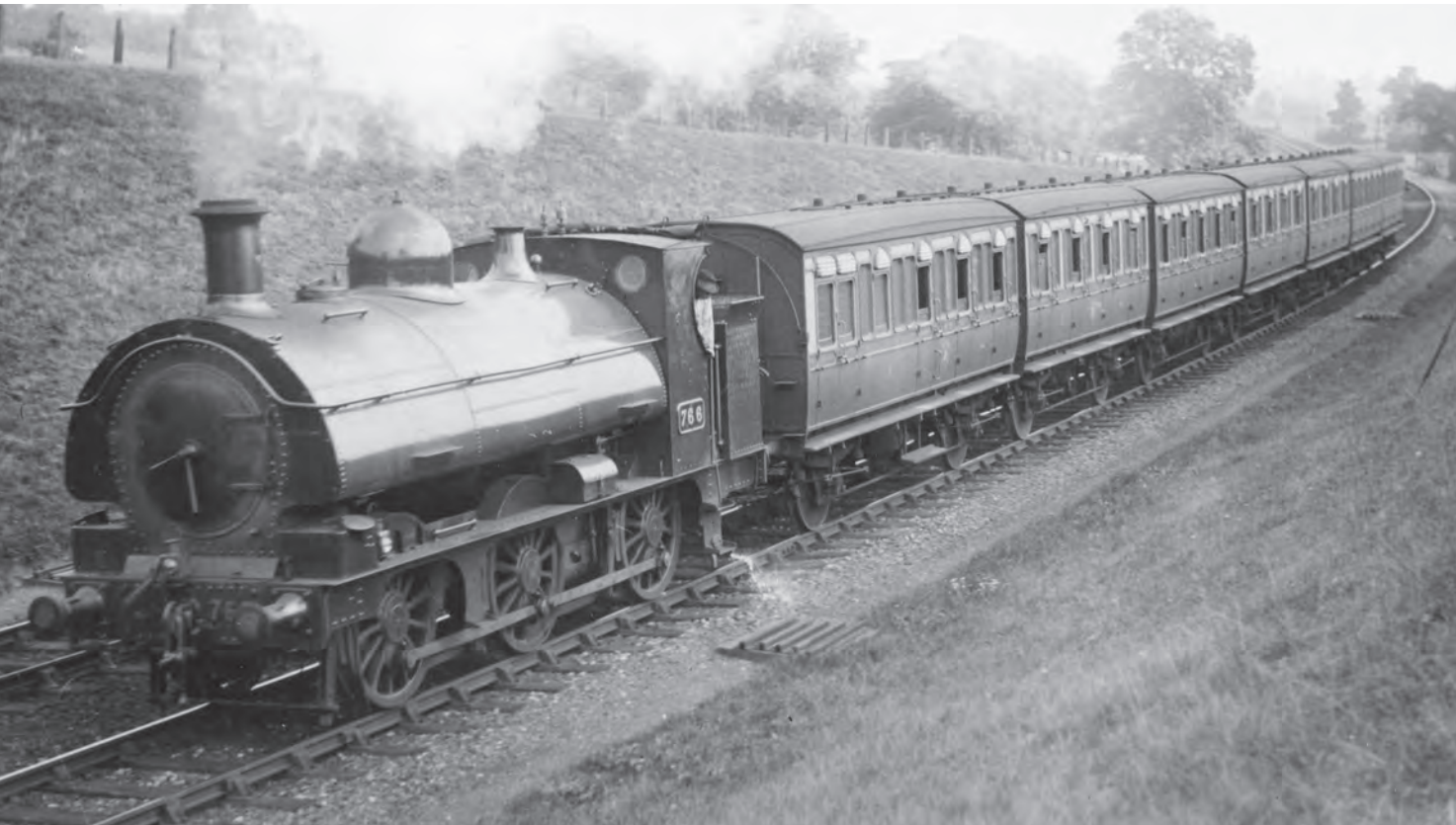
Saddle tank 766 built in 1873, with a string of Dean 4-wheel coaches at an unidentified location, c1910. It was rebuilt as a pannier tank in 1929 and withdrawn at Chester in 1935. (GW Trust/P.J. Reed Collection)
