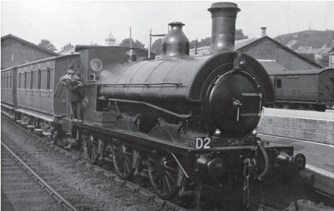
Brecon & Merthyr Railway saddle tank No.17 as built in 1881 at Merthyr before rebuilding as a pannier tank and renumbered 2190 by the GWR, c1905. (MLS)
