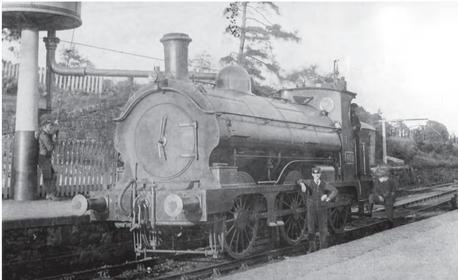
651 as built as a saddle tank in July 1872, at Dolgelley, c1900. It was rebuilt as a pannier tank in 1921 and withdrawn from Neath shed in 1932. (GW Trust/P.J. Reed Collection)
