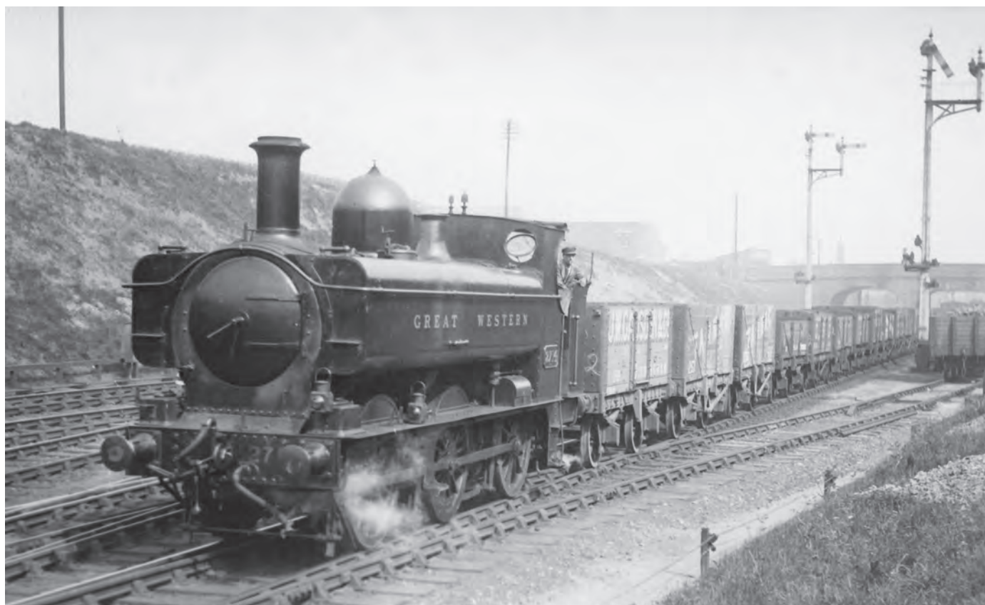
2704 , built in March 1896 and rebuilt as a pannier tank in March 1930 on a freight at Oxley, 14 September 1936. (GW Trust/F.K. Davies)
