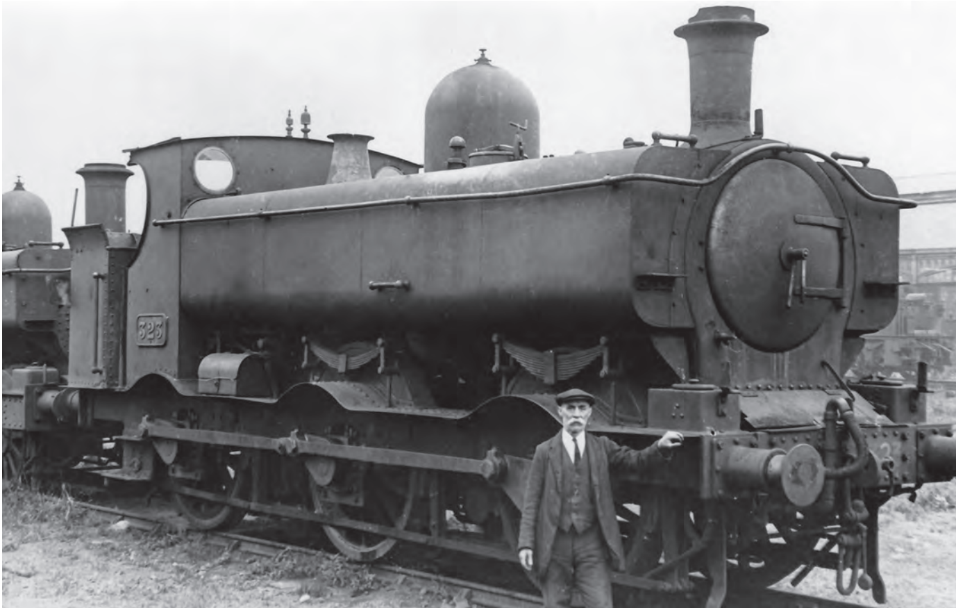
No.323 rebuilt from 0-6-0 tender engine in December 1879, with open cab and original small bunker, but well-worn and nearing withdrawal in July 1932 as the last survivor of the small class. (MLS/Bob Miller Collection)
