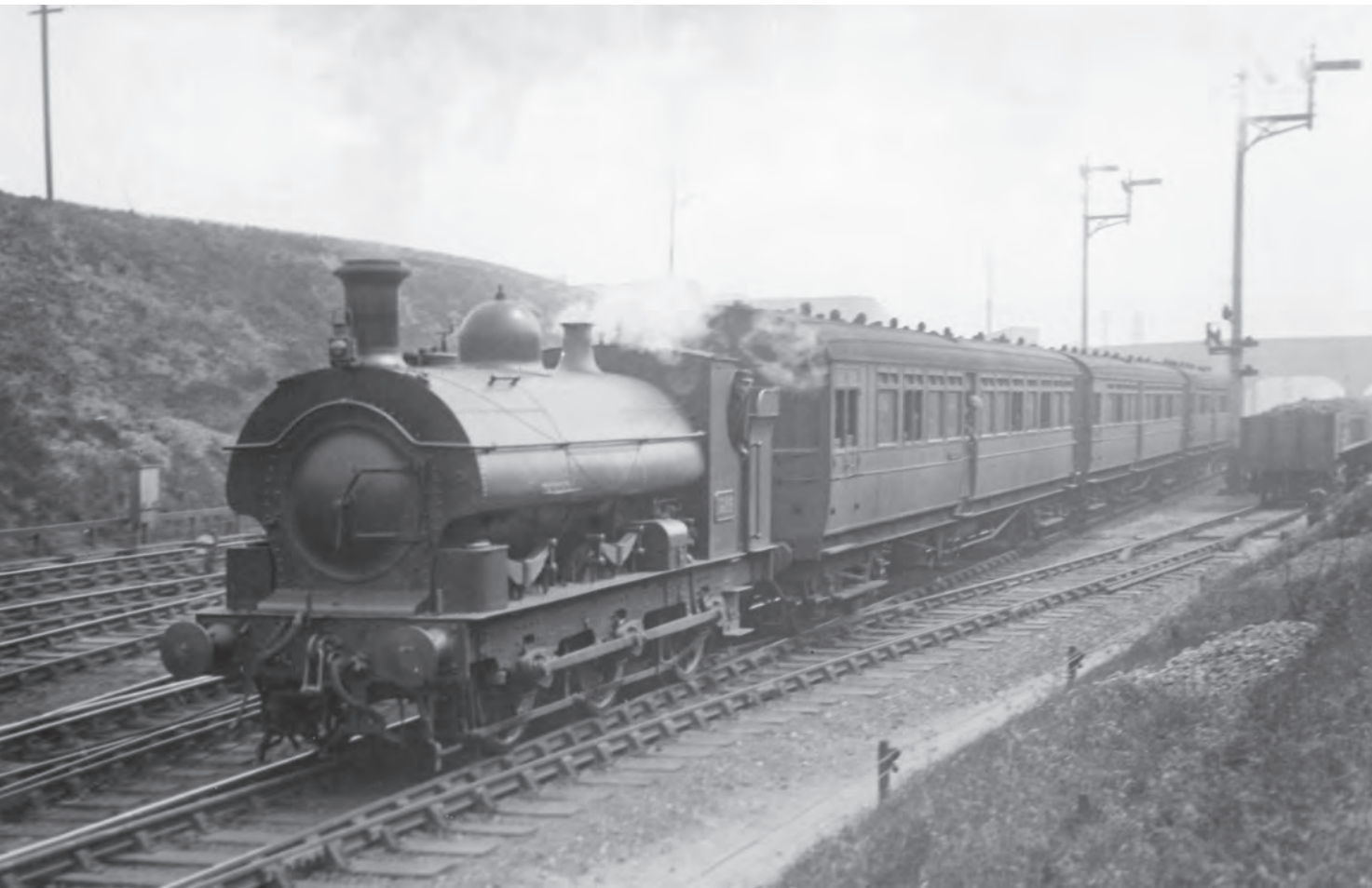
Saddle tank 1234 hauling three auto trailers, thought to be in the West Midlands, c1920. 1234 was rebuilt as a pannier tank in 1928. (GW Trust/P.J. Reed Collection)
