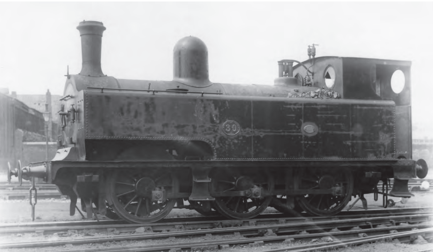
Cardiff Railways No.30 (GW number 691), built in March 1889, with hybrid pannier/side tanks, at Cardiff Docks, c1920. Note the absence of bunker and the coal stacked on the tank top in front of the cab. It was withdrawn in 1929. (MLS/Bob Miller Collection)
