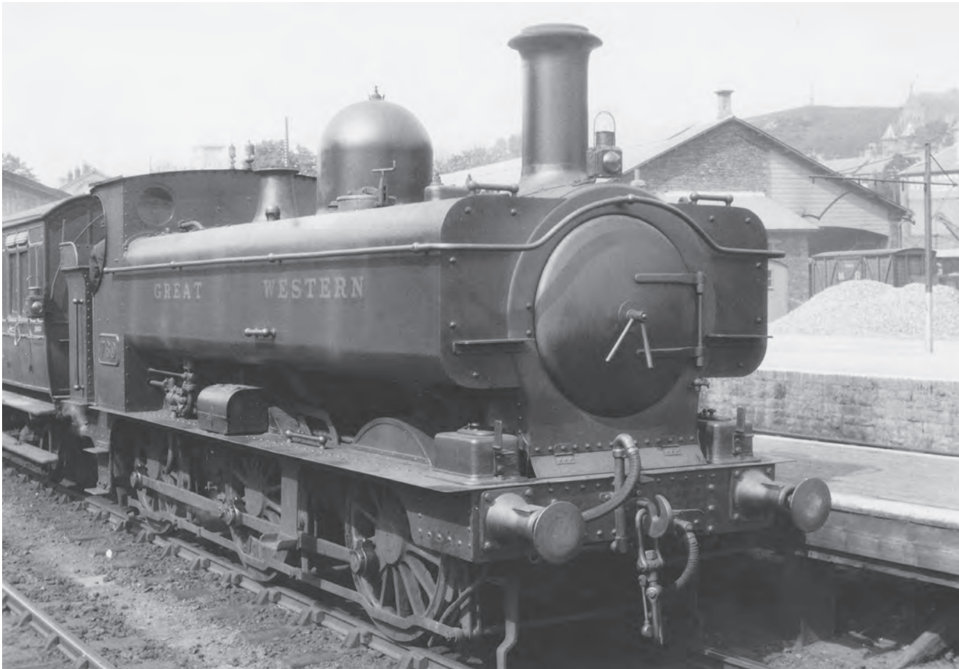
769 , built in April 1873 and rebuilt with pannier tanks in November 1922, at Merthyr on a passenger train, c1925. It was withdrawn in April 1930. (John Hodge Collection)
