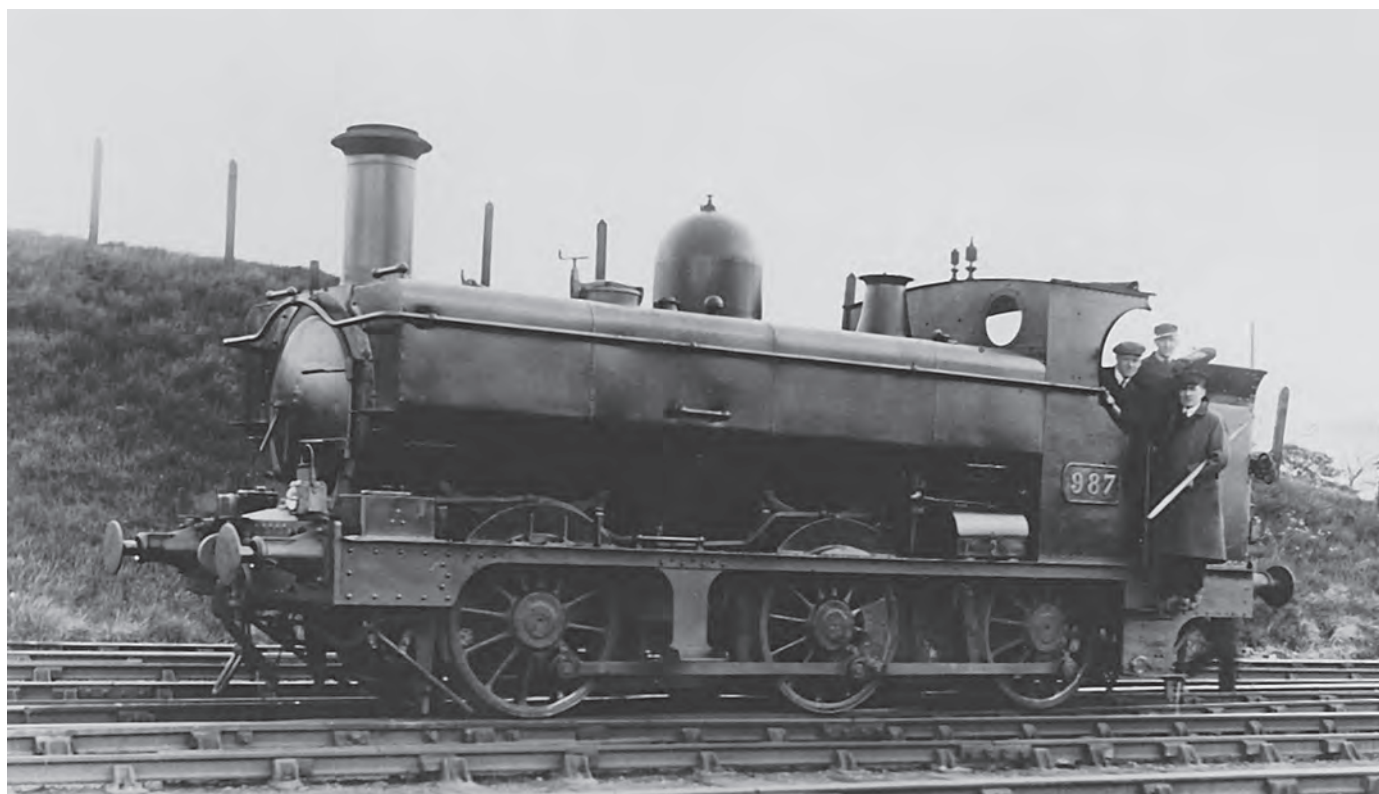
No.987 , built in June 1875, and rebuilt with pannier tanks in March 1924, c1925. It was withdrawn in April 1925. (MLS)
