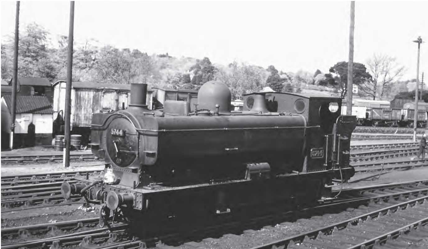
5744 shorn of its spark arrester chimney and left with the stovepipe rather than GW Collett chimney, transferred from Didcot to Truro, 29 April 1961. (R.C. Riley)
