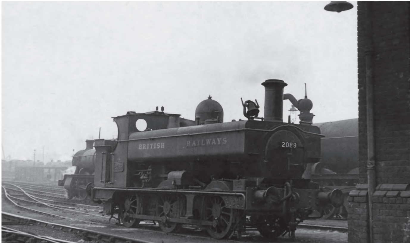
2089 was one of the Birkenhead based engines fitted with a warning bell for working in the dock area. It was built in March 1901, rebuilt with pannier tanks in July 1924, but retained its original small bunker and open cab. It survived until nationalisation and received BR lettering on the tank side before the 'lion and wheel' totem was introduced. However, it was withdrawn in September 1951 and replaced by others of the class for the dock shunting. It is seen on the LMR Birkenhead shed (6C) with a 63XX mogul and LMR engines in the background, c1950. (MLS/Bob Miller Collection)
