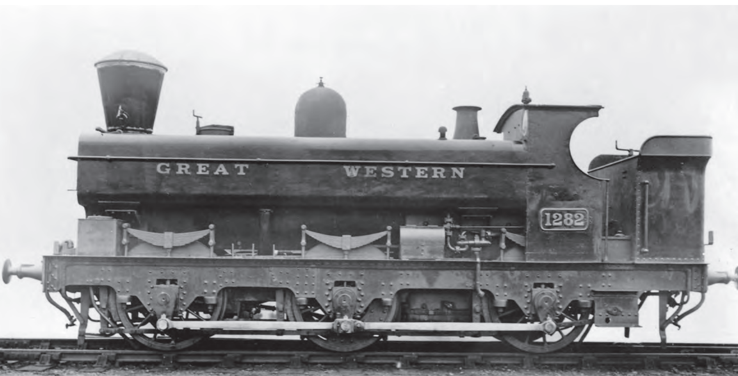
1282 built in 1877, rebuilt with pannier tanks in April 1916, and equipped with a spark-arresting chimney. It still has an open cab, so the photo was taken before 1924 when it received an enclosed cab and enlarged bunker. (MLS/F. Moore)
