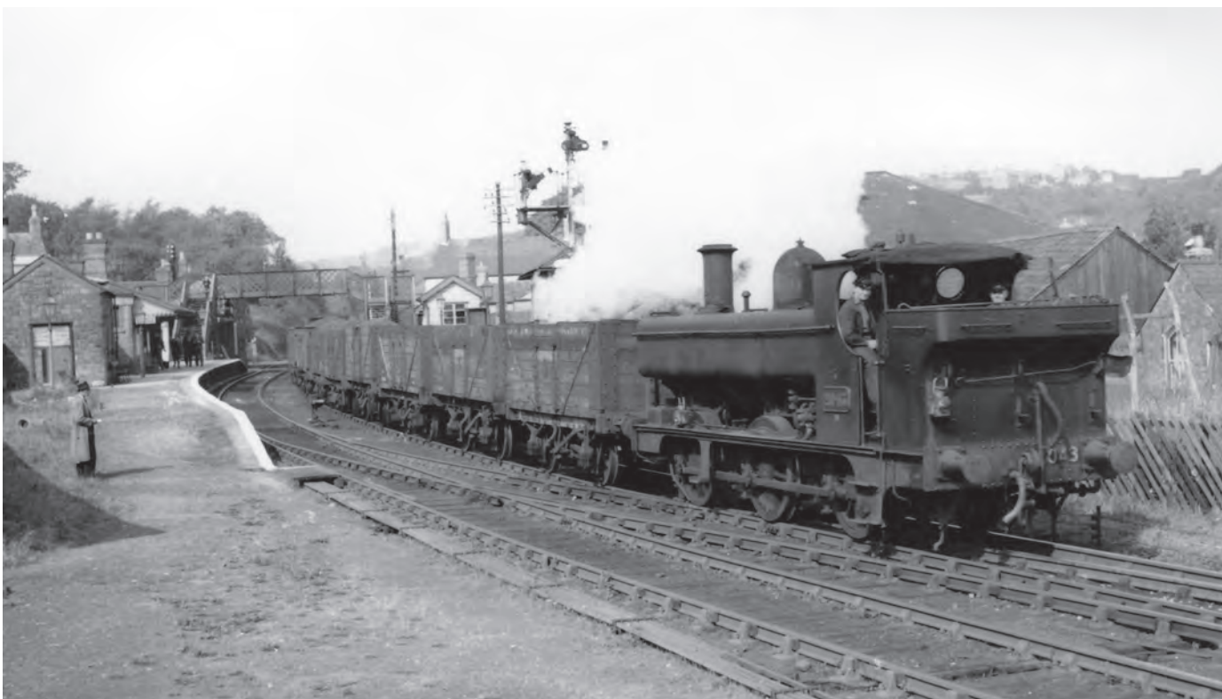
2043 , built in May 1898 and rebuilt with pannier tanks and enlarged bunker in December 1917, but retaining its open cab, running bunker first with a coal train from the Forest of Dean at Lydney Town, signalled into the yard, c1930s. (SLS/John Hodge Collection)
