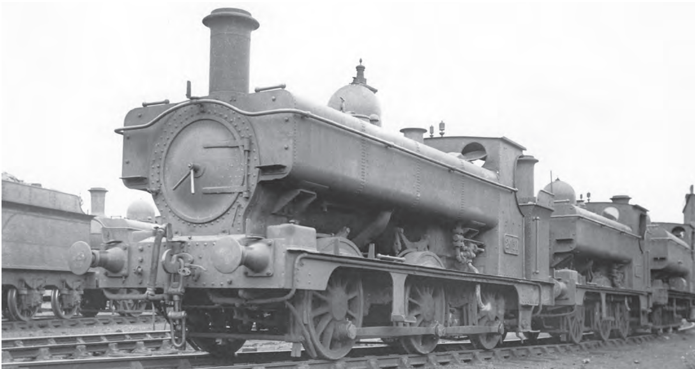
2031 , built in 1897 and rebuilt with pannier tanks in 1923 with '655' tank 2013 at Bristol St Philip's Marsh, 16 August 1936. (F.K. Davies/John Hodge Collection)
