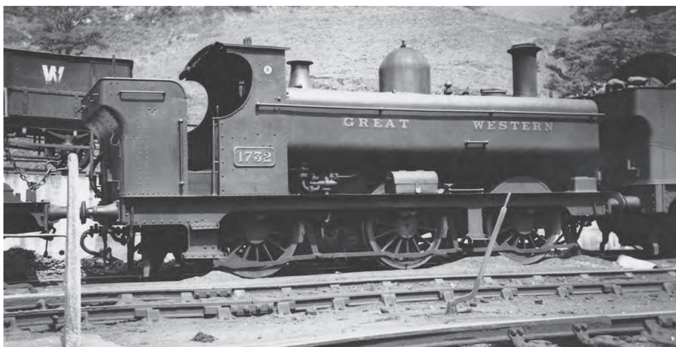
1732 , built in July 1892 and fitted with pannier tanks in August 1914, at Port Talbot, 26 May 1935. It received an enlarged bunker but retained its open cab, before withdrawal in July 1946. (F.K. Davies/John Hodge Collection)
