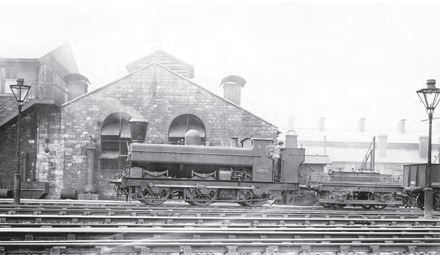
Didcot's 1263 , built in 1877, rebuilt as a pannier tank in March 1920, with spark arrester chimney. It was condemned in January 1934. (CW Trust)
