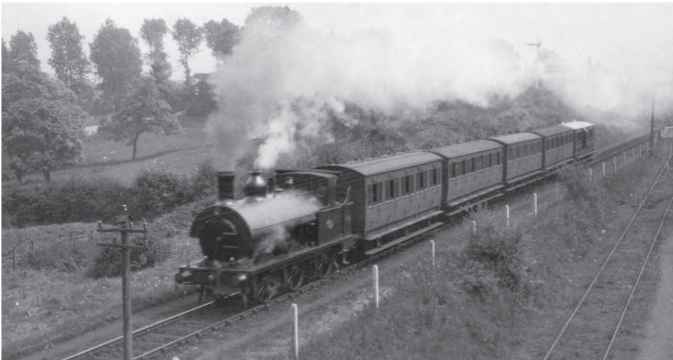
No.17 (later GWR 2190) in saddle tank form on a Merthyr-Brecon train, c1905. It was rebuilt as a pannier tank in 1922. (MLS)
