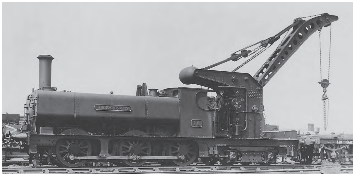
GW crane tank No.16 Hercules built in 1921 but to similar design and allocated to Swindon Works where it is seen with jib raised, c1925. (MLS/Bob Miller Collection)
