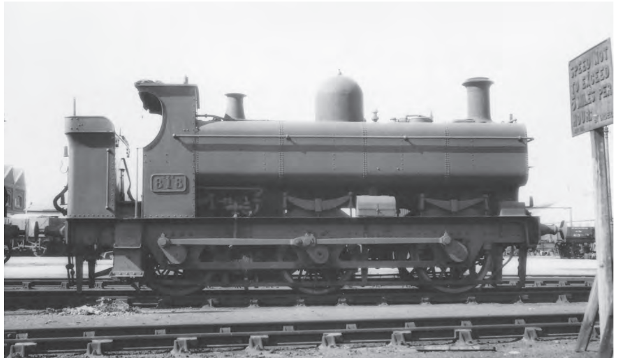
GW 818 , South Wales Mineral Railway No.7, ex South Devon Railway 0-6-0ST built in 1873, rebuilt as a pannier tank in 1924. (MLS)
