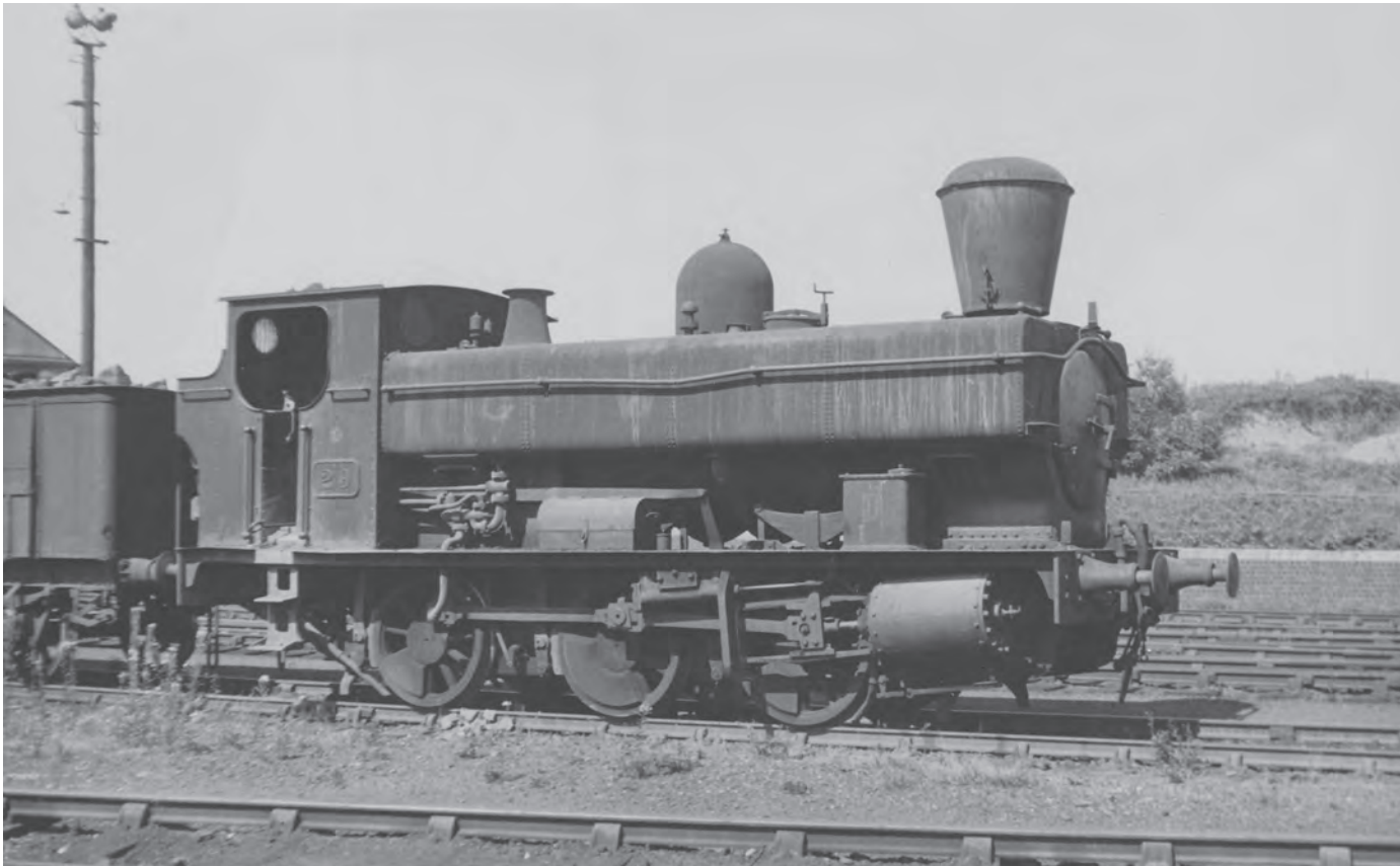
GW 29 , rebuilt as a pannier tank in 1924, at Kidderminster with spark arrester chimney in August and November 1948. (MLS/W. Potter)
