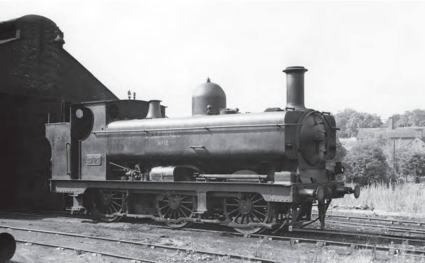
2794 , built in February 1901, rebuilt with pannier tanks in February 1916, and sold to the Lilleshall Company in October 1950 after withdrawal from BR service in November 1948, here stripped of its BR identity apart from GW numberplate, c1952. (MLS)
