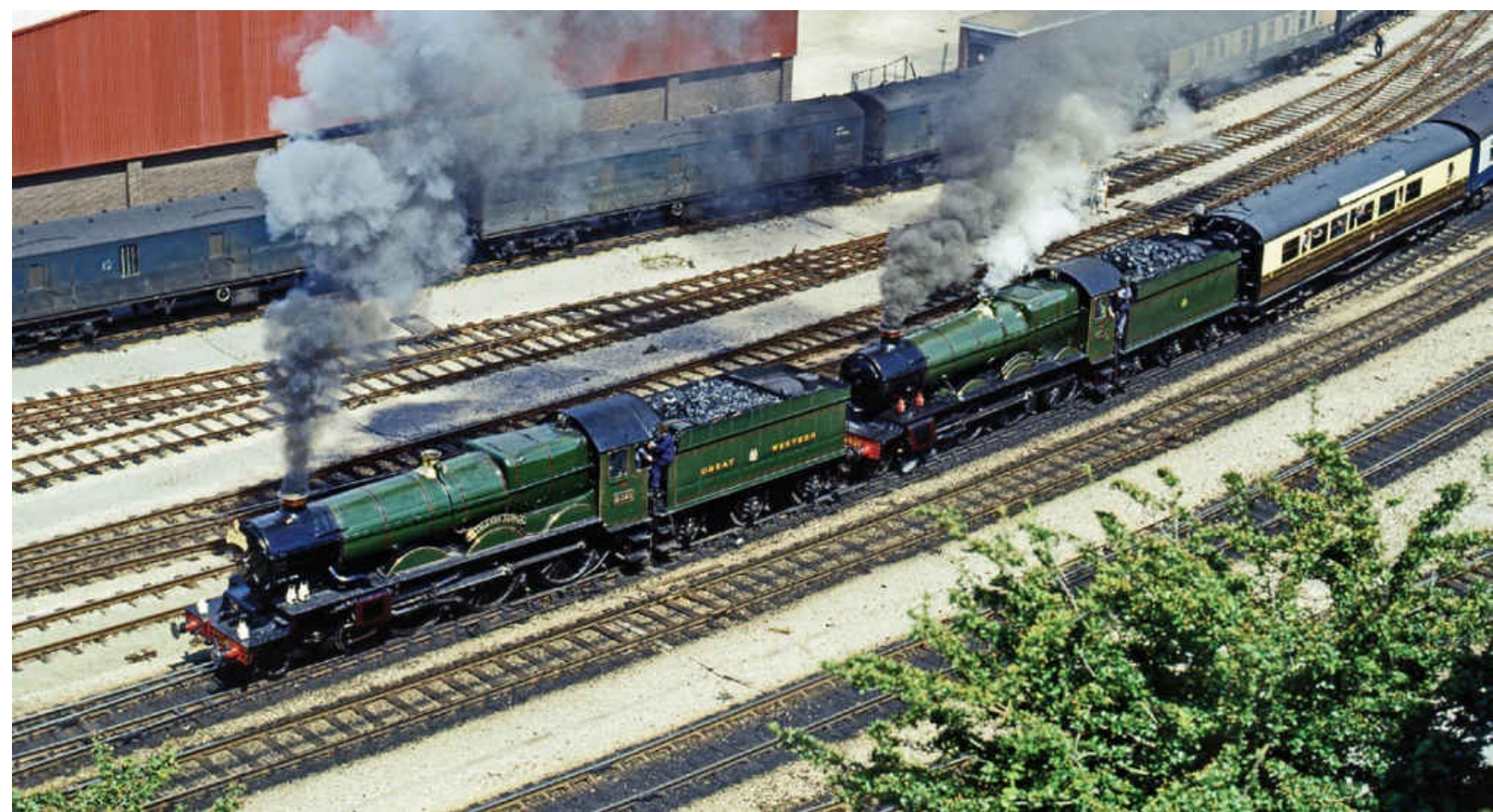
GWR 'Castle' class 4-6-0 No 5051 DRYSLLOWYN CASTLE and GWR 'Hall' class 4-6-0 No 4930 KINLET HALL are seen leaving Bristol Temple Meads with the 'Great Western Limited'. Steam traction operated unaided from Bristol to 'Milepost 217' on Dainton Bank where the pair stalled, 'Class 50' diesel No 50045 ACHILLES then assisted the train up the bank, after which the 2 steam locomotives worked as far as Totnes where the tour was terminated, on the 7th July 1985. John Chalcraft/Rail Photoprints
