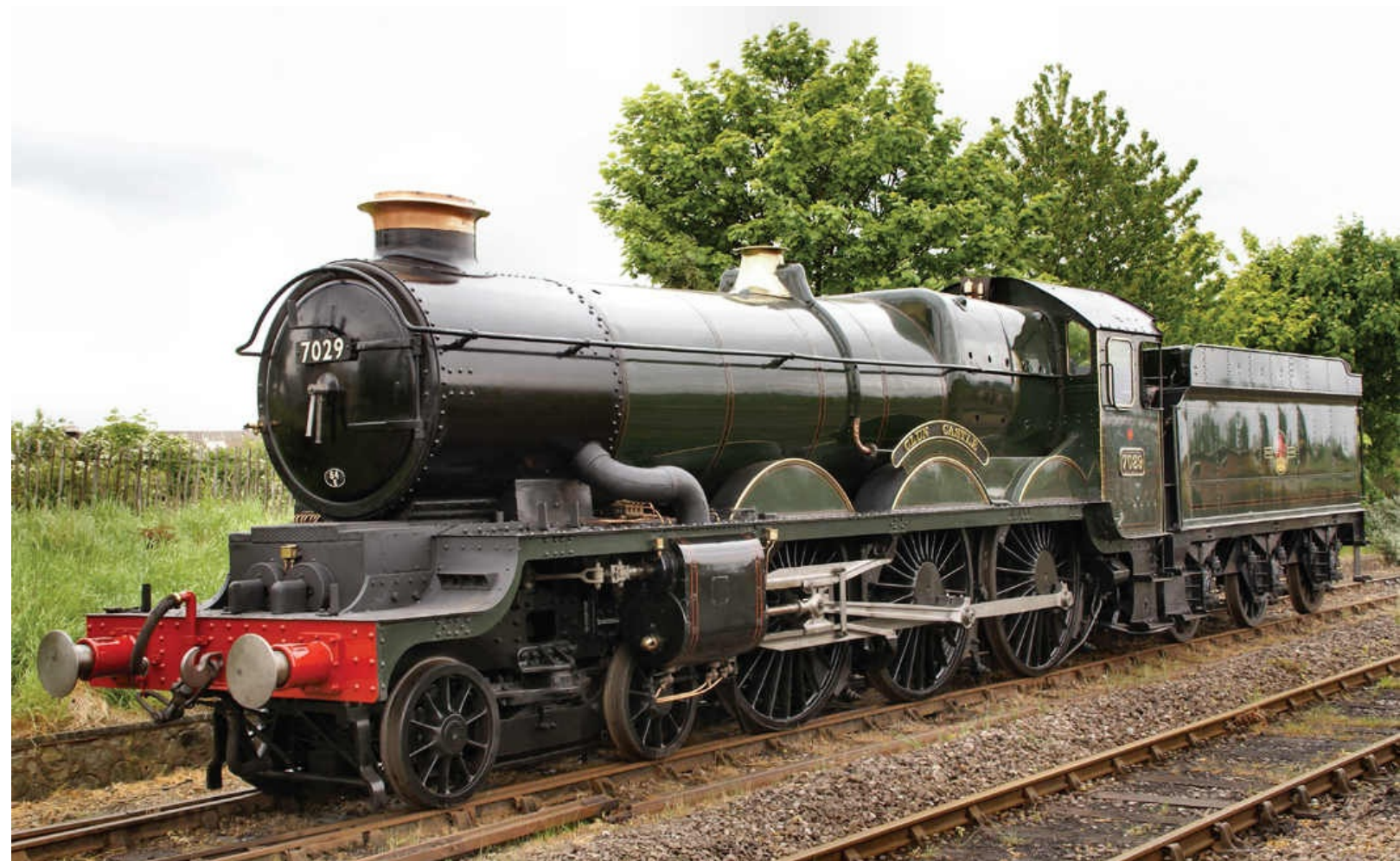
This superb 2008 image of the preserved BR/WR 'Castle' class 4-6-0 No 7029 CLUN CASTLE shows the pleasing lines of the Collett design to great effect, (Collett 4000g tender). The locomotive has the benefit of British Railways final modifications which included a Diagram HD boiler with a 4-row superheater, double chimney and mechanical
