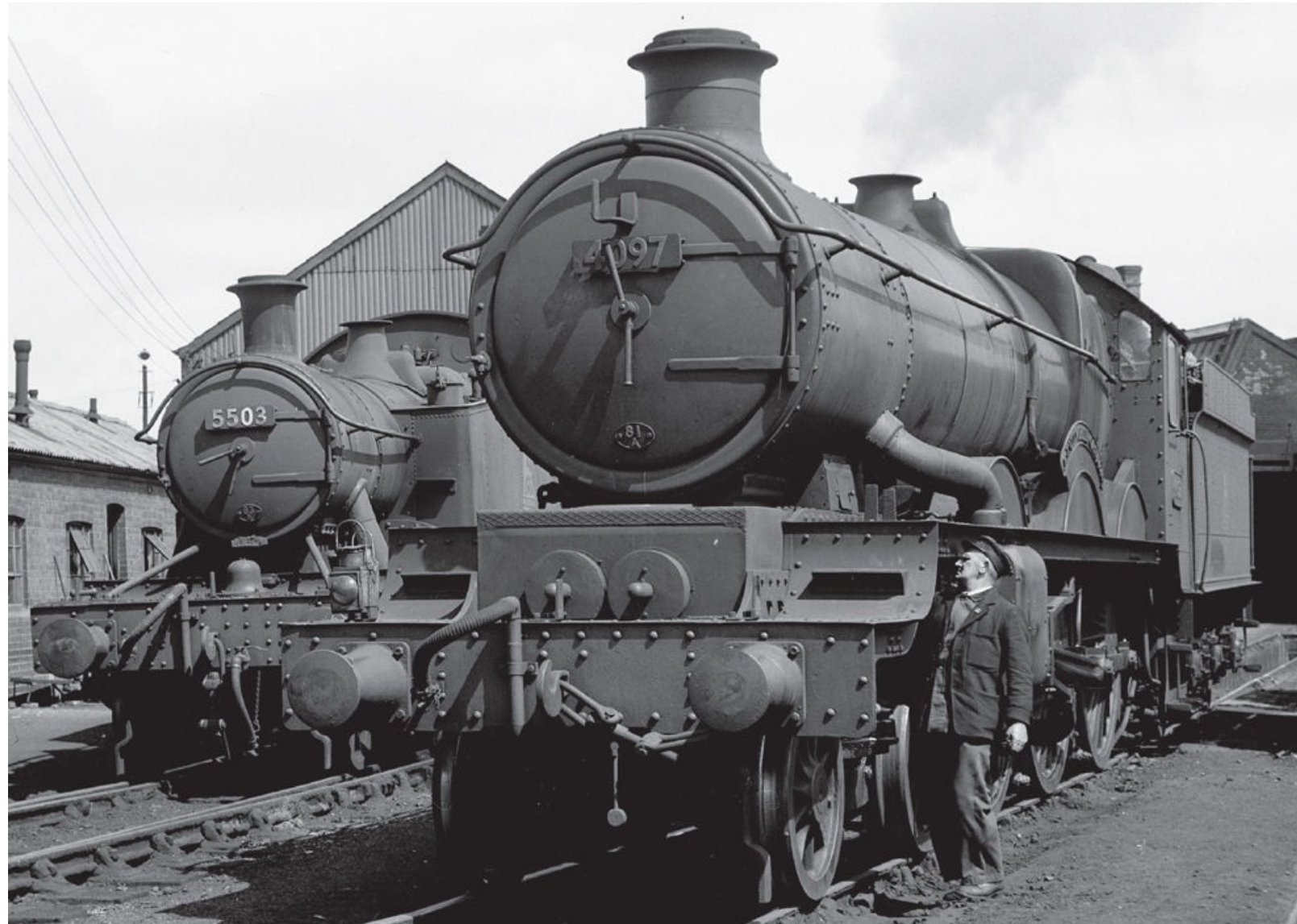
GWR 'Castle' class 4-6-0 No 4097 KENILWORTH CASTLE is examined by the rostered driver before moving off shed at Taunton on 8th June 1955. Note the shorter single chimney which contrasts well with the taller chimney on the tank locomotive to the left, BR re-build style un-stepped inside cylinder cover and (81A) Old Oak Common shed plate. The 'Castle' is in the company of GWR Modified '4500' class 2-6-2T No 5503 which was at that time a Taunton (83B) engine. David Anderson
