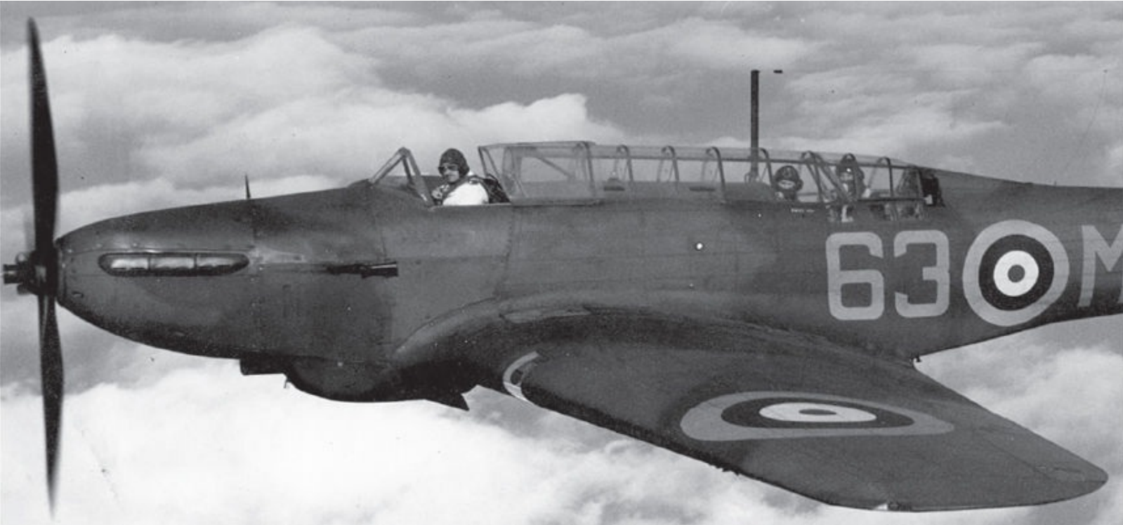
RAF Fairey Battle light bomber K7650/63M of No 63 Squadron RAF Benson is pictured in flight, November 1939, the three crew members can be seen. The original order called for the building of 2,419 aircraft but that was cut short as production ceased in September 1940 when only 2,185 of the aircraft had been built. Royal Air Force
