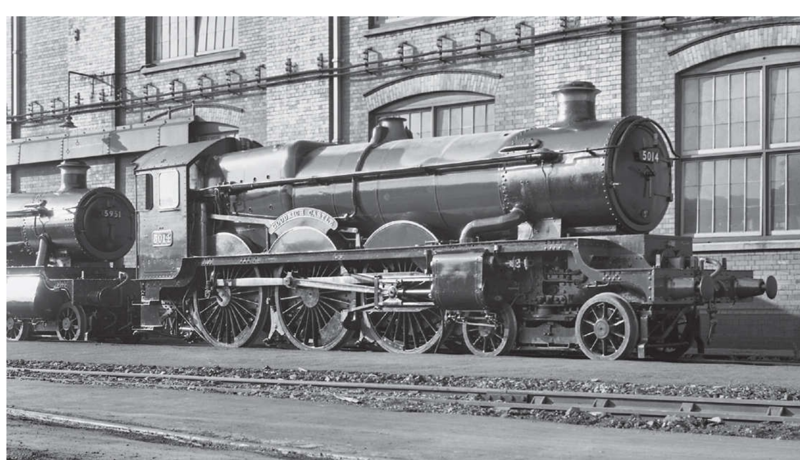
No 5014 GOODRICH CASTLE at Swindon following a 'Heavy Intermediate' overhaul in 1957. Note tapered barrel buffers and box pattern inside cylinder casing, sandboxes under cab floor. The 'Castle' is in the company 'Hall' class No 5951 CLYFFE HALL. Mike Morant Collection
