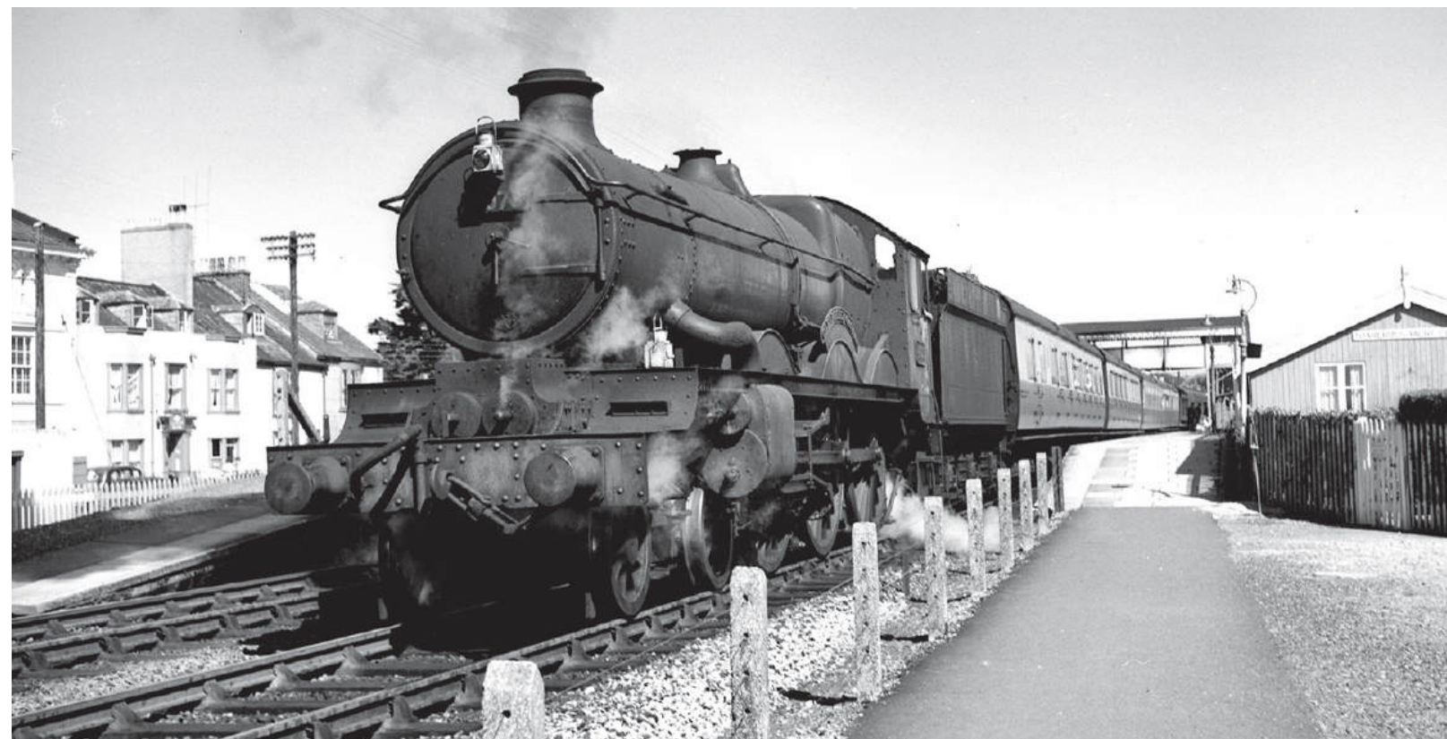
GWR 'Castle' Class No 4073 CAERPHILLY CASTLE is seen at Starcross station with a down local train, on 25 July 1956. This image clearly shows the original style GWR curved sided inside cylinder casing. The steam leak indicates that the engine was only one month away from a heavy overhaul. David Anderson
