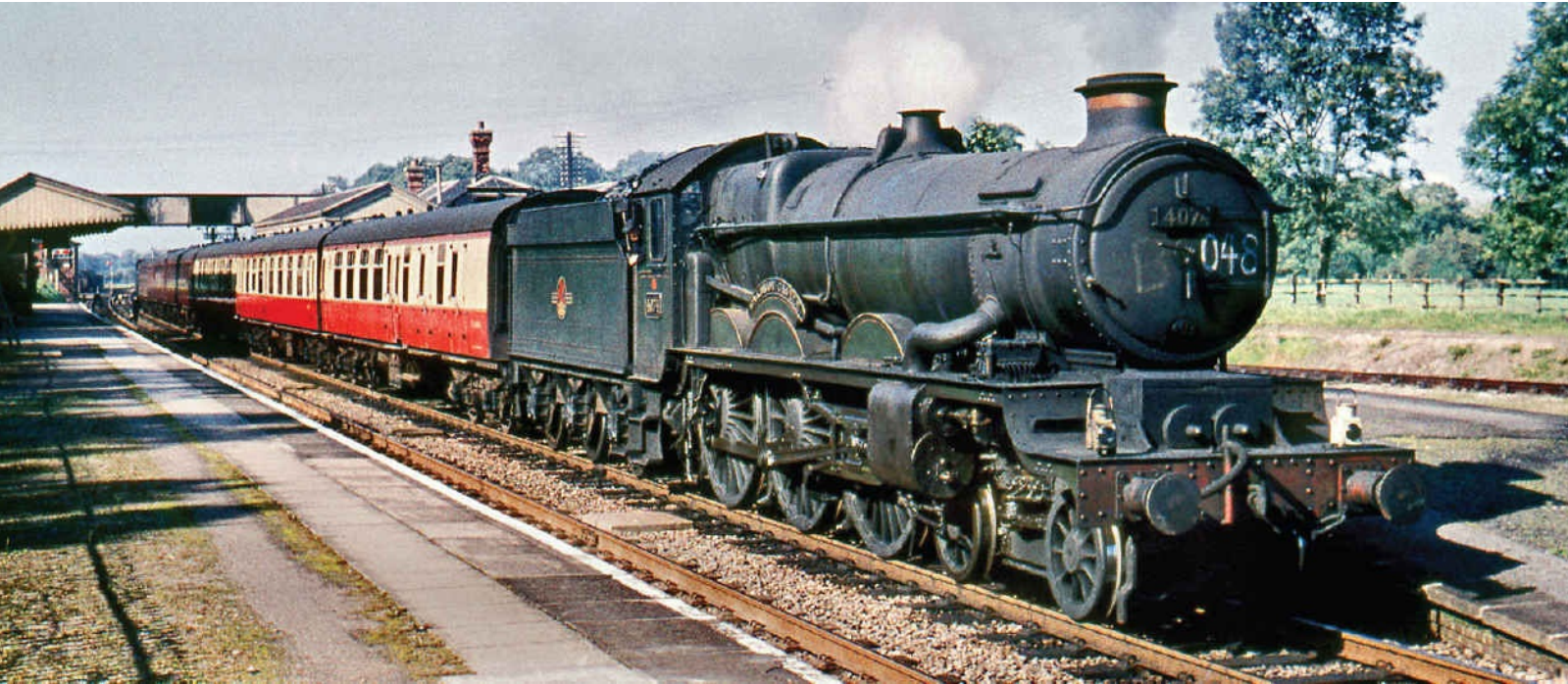
GWR ‘Castle’ class 4-6-0 No 4074 CALDICOT CASTLE (BR ‘Box’ style un-stepped inside cylinder cover) is seen at Patney & Chirton station on the Berks and Hants line with a local service in July 1958. It appears that 3 maroon coaches are being removed from the rear of the train. Alan Sainty Collection
