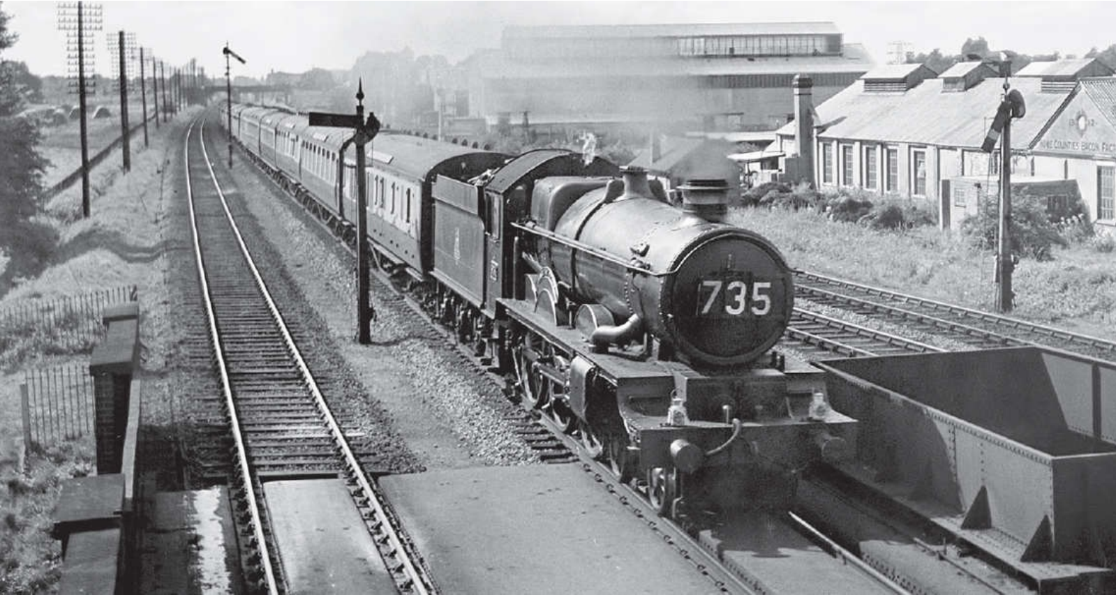
GWR ‘Castle’ class 4-6-0 No 5054 EARL OF DUCIE is seen passing Langley with an up South Wales-Paddington express, on 14th August 1954. Note the profile of the modified pattern steam pipe and the shorter style chimney. C. R. L. Coles (Dave Cobbe Collection)/Rail Photoprints
