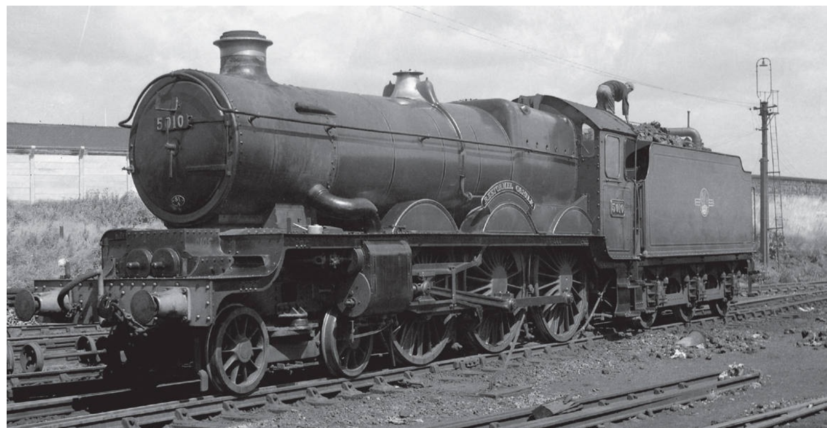
GWR 'Castle' class 4-6-0 No 5010 RESTORMEL CASTLE is seen being serviced at Old Oak Common (81A) on 20th July 1958. Note the Hawksworth tender, also the oil can at the front end of the running plate, brass embellishments and original GWR inside cylinder casing. A.E Bennett/Transport Treasury
