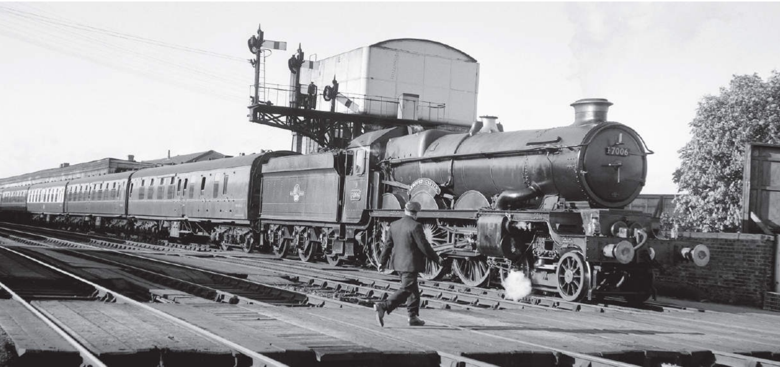
GWR ‘Castle’ class 4-6-0 No 7006 LYDFORD CASTLE is seen at Oxford station with an up Paddington service on 8th May 1961. This image shows the engine’s (some may say incongruous) double chimney to good effect. Note also the mechanical lubricator located behind the offside steam pipe. David Anderson
