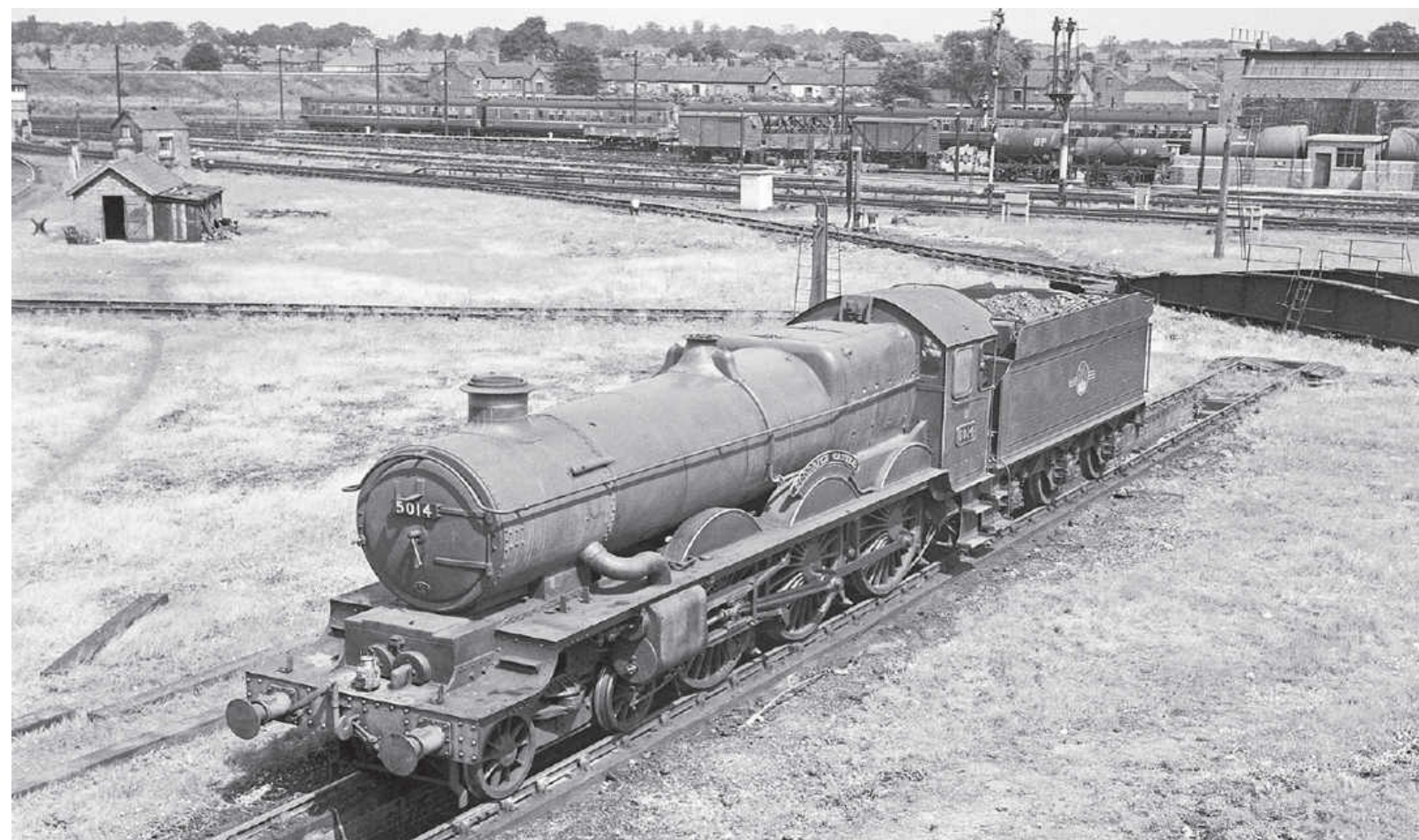
Changing times, GWR 'Castle' class 4-6-0 No 5014 GOODRICH CASTLE is seen being serviced at Chester in the summer of 1962. The brass beading on the cab front edges and centre cylinder cover step can be seen, as can the short fire iron compartment. Note the BP oil tankers and the Diesel Multiple Units outside the new depot buildings. The embankment in the background carried the Cheshire Lines route, Manchester Central via Northwich to Chester Northgate Station. Jim Carter/Rail Photoprints
