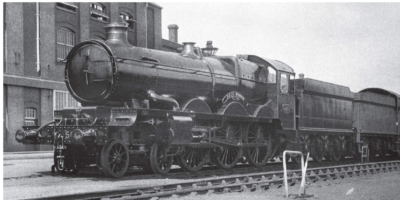
GWR 'Castle' class 4-6-0 No 5083 BATH ABBEY is seen when newly rebuilt at Swindon Works in June 1937. Rail Photoprints Collection
