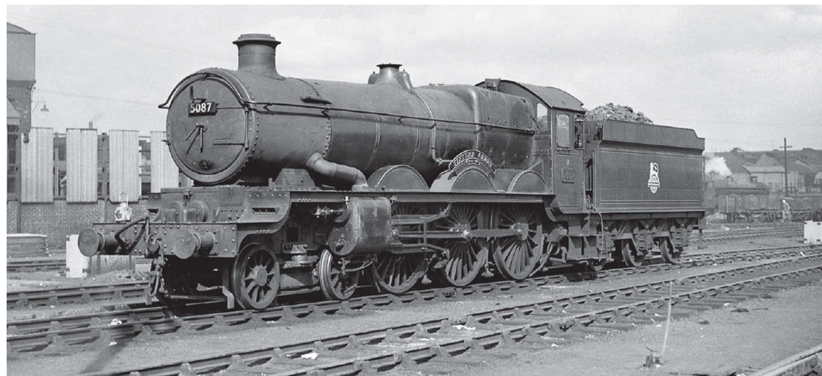
GWR 'Castle' class 4-6-0 No 5087 TINTERN ABBEY is seen at Old Oak Common in May 1954, note Collett 4000g tender. Rail Photoprints Collection
