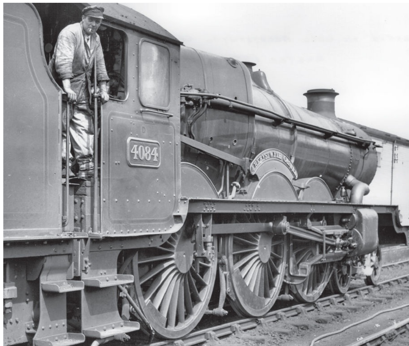
Two distinctly different types of rear sandboxes were fitted, on locomotives numbers 4073–5059 and 'Star' class rebuilds. It was located below the cab floor with only the delivery pipes being visible (see No 4084 ABERYSTWYTH CASTLE). David Anderson
