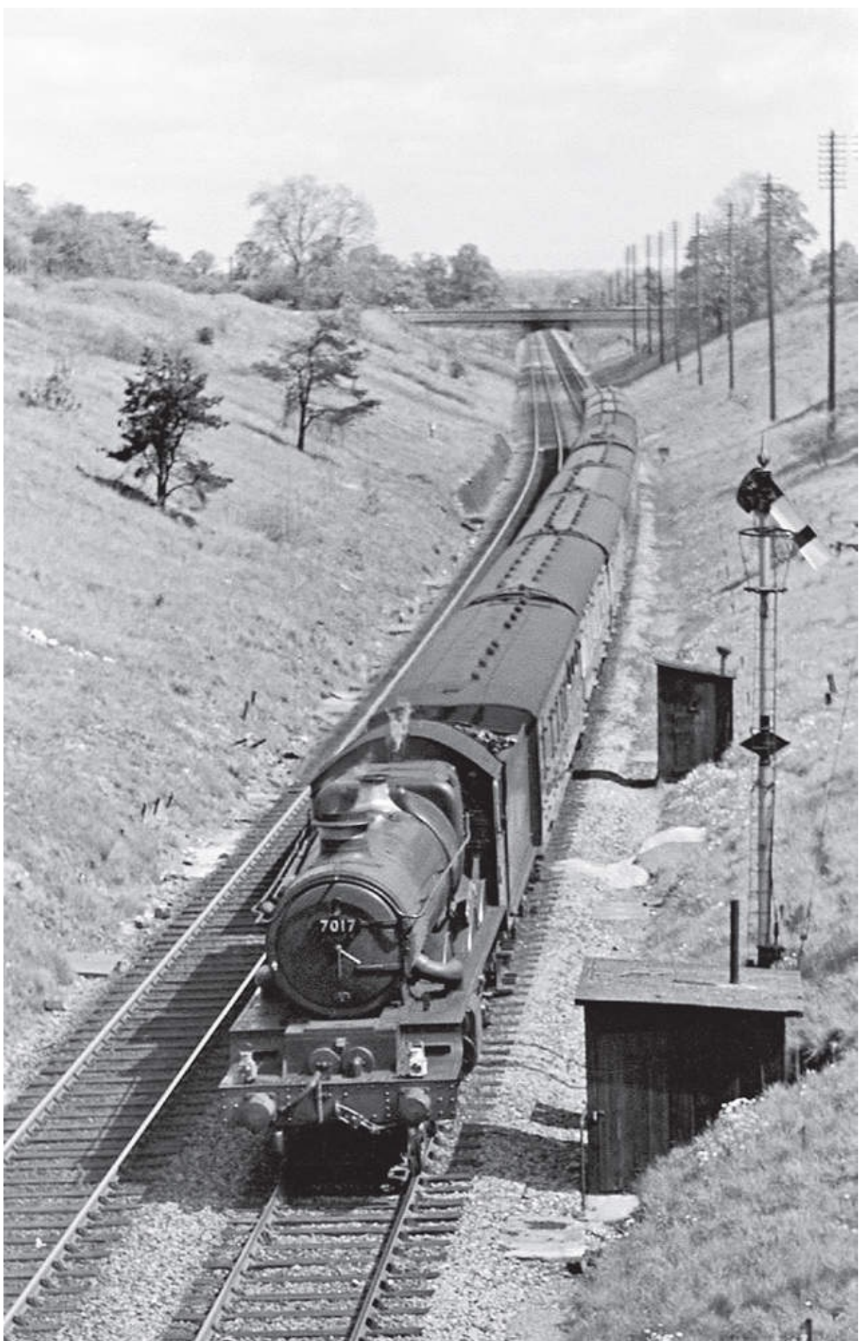
BR/WR 'Castle' class 4-6-0 No 7017 G. J. CHURCHWARD approaches Corsham and Box Tunnel with a down Paddington-Bristol service, in 1960. Note the diamond shaped plate on the signal post informing footplate crews that track circuiting is in use. Rail Photoprints Collection
