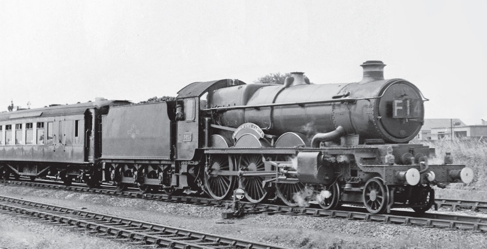
GWR ‘Castle’ class No 5013 ABERGAVENNY CASTLE (stepped inside cylinder cover) passes Patchway with the ‘South Wales Pullman’ during November 1960, no headboard carried. Locomotive No 5013 was the first of the class to be built with a compartment for housing short fire irons which was accessible from the cab, the housing was situated between the left hand (nearside) centre and trailing driving splasher. Rail Photoprints Collection
