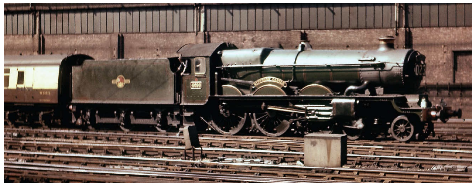
GWR 'Castle' class 4-6-0 No 4098 KIDWELLY CASTLE is seen arriving at Paddington Station. Note the Hawksworth straight sided tender with which the engine was paired between 15/03/1957 and 28/11/1959. Mike Morant Collection
