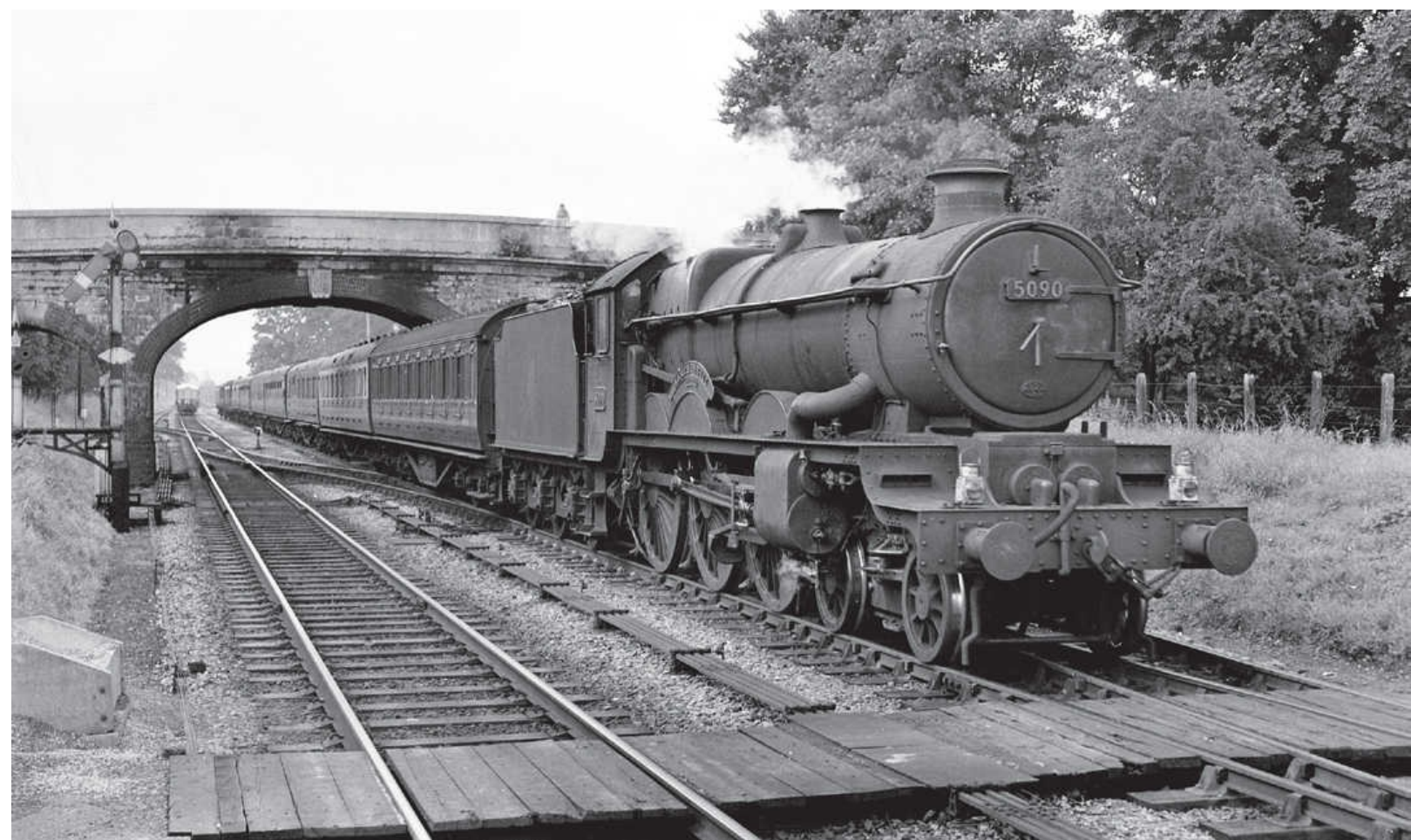
GWR 'Castle' class 4-6-0 No 5090 NEATH ABBEY, built from 'Star' class No 4070, is seen approaching Bathampton with the 10.30am Cardiff-Portsmouth service, on 19th August 1958. Note this engine was one of the 31 examples which retained 'Joggled Frames'. Hugh Ballantyne/Rail Photoprints
