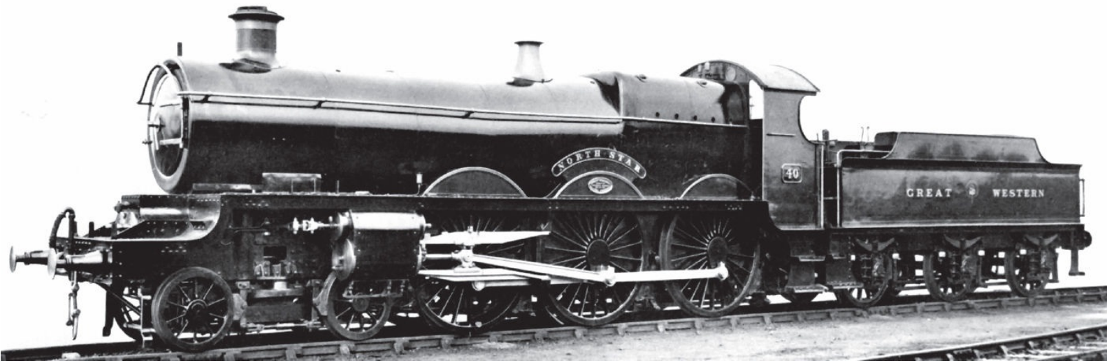
GWR No 40 NORTH STAR seen as outshopped from Swindon Works as a 'Star' class 4-6-0 in September 1909, re-built as a 'Castle' in November 1929. Authors Collection
