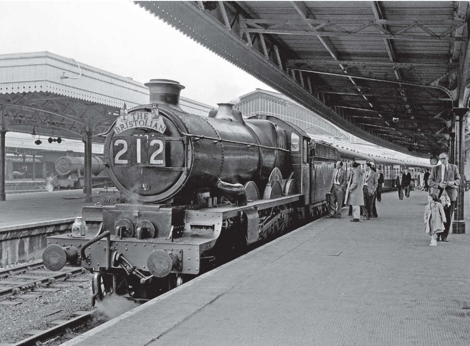
BR/WR 'Castle' class 4-6-0 No 7024 POWIS CASTLE stands at Bristol Temple Meads after arrival with the last booked steam hauled down 'Bristolian' (08.45 Paddington-Bristol) 12/6/59. Note the mechanical lubricator in the final forward position. Hugh Ballantyne/Rail Photoprints
