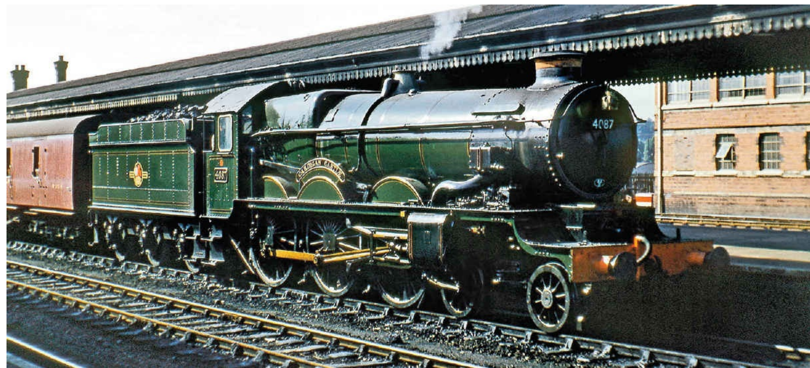
Laira based 'Castle' class 4-6-0 No 4087 CARDIGAN CASTLE freshly out of Swindon Works (General overhaul outshopped 13th August) and coupled to a Collett 4000 gallon tender is seen with a 'running in turn' at Reading General in August 1959. Note the double chimney, Davies & Metcalf valveless lubricator with additional oil reservoir attached to the smokebox, BR pattern parallel barrel buffers and stepped inside cylinder cover. Alan Sainty Collection
