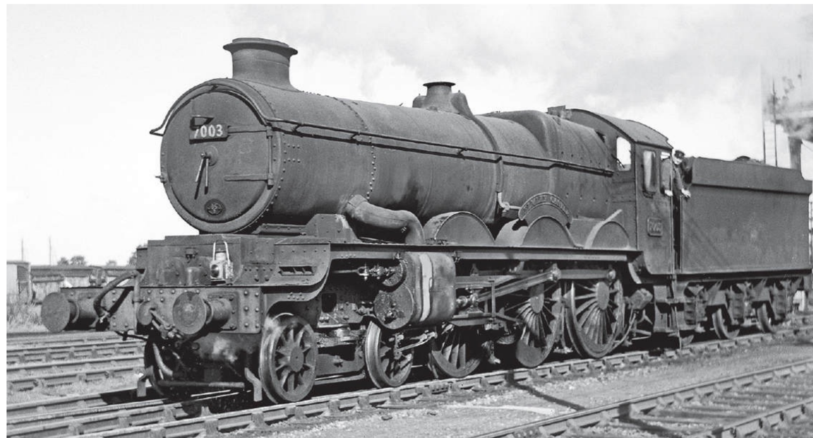
GWR 'Castle' class 4-6-0 No 7003 ELMLEY CASTLE, now with double chimney is seen at Westbury depot in June 1963. Rail Photoprints Collection
