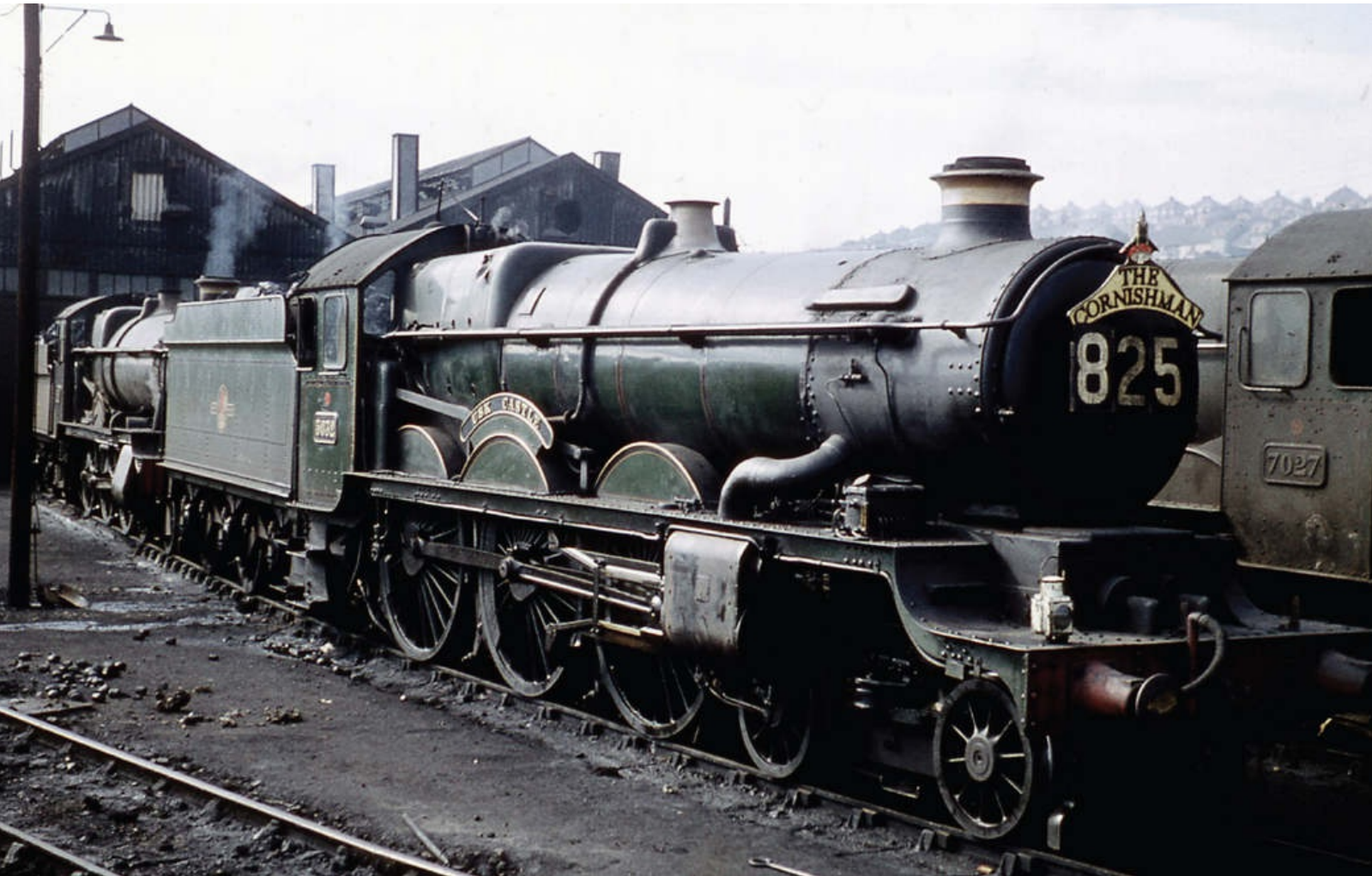
GWR 'Castle' class 4-6-0 No 5032 USK CASTLE is seen in the company of sister engine No 7027 THORNBURY CASTLE at Laira shed (83D) in July 1958. Note the cab window handrail on 7027 which is not simply under the window but instead carries on upwards forward of the window frame, a feature of 'Castle' class engines from No 5098 onwards. R.E.Vincent/Transport Treasury
