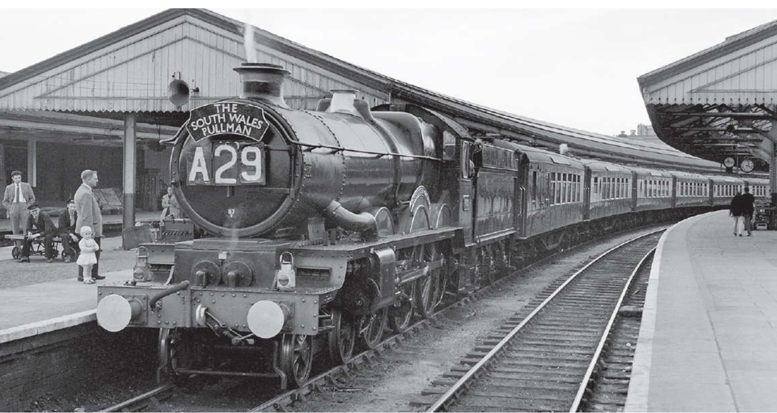
The last up steam hauled ‘South Wales Pullman’ prepares to leave Swansea High Street for London Paddington behind GWR ‘Castle’ class 4-6-0 No 4090 DORCHESTER CASTLE. The mechanical lubricator can clearly be seen on the platform side running board. ‘South Wales Pullman’ from Paddington-Swansea High Street introduced 27th June
