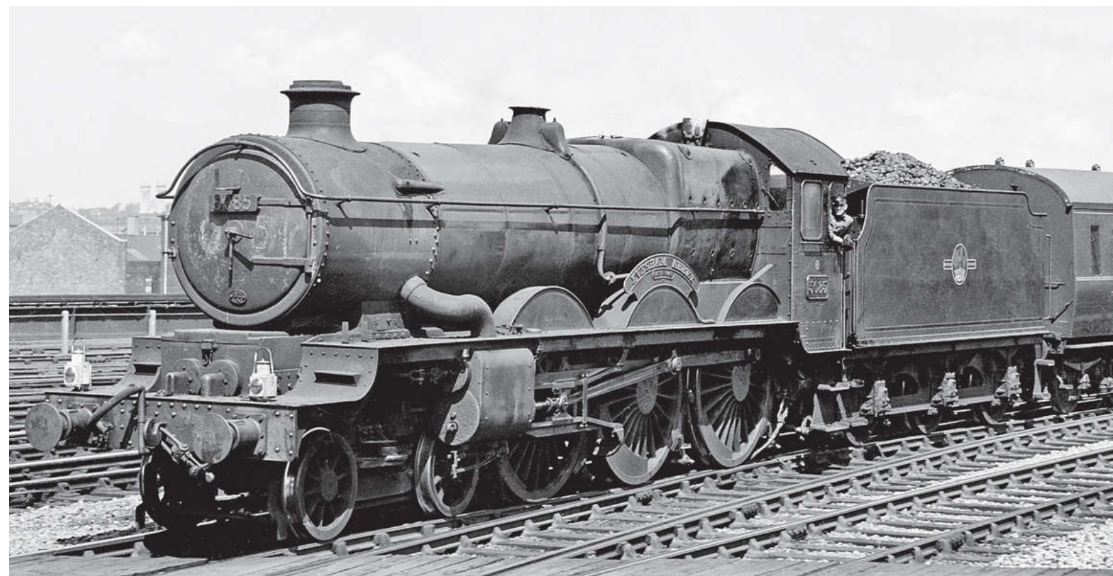
GWR 'Castle' class 4-6-0 No 5085 EVESHAM ABBEY is seen arriving Bristol Temple Meads, note the window wiper fitted to the front cab window(s). Rail Photoprints Collection
