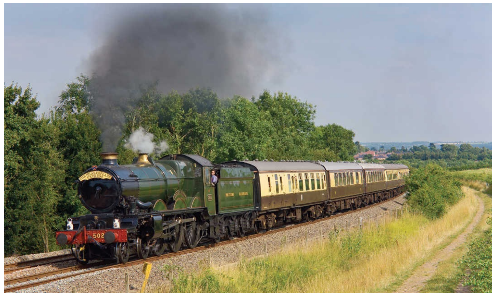
Preserved GWR 'Castle' class 4-6-0 No 5029 NUNNEY CASTLE is seen heading a 'Shakespeare Express' charter past Churchill Cottage on the climb out of Stratford on Avon towards Wilmcote on 27th July 2008. The locomotive is coupled to Collett tender No 2690 which was originally a 4000 gallon capacity unit but in preservation that capacity has been increased to 4610 gallons. In GWR/BR service No 5029 was coupled to several different Collett and Hawksworth 4000g tenders, but never to the one now in use. Mathew Wilson
