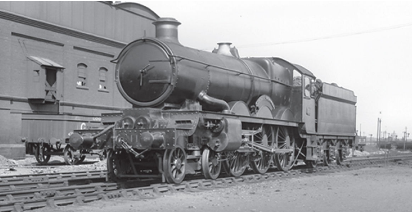
GWR ‘Castle’ class 4-6-0 No 111 VISCOUNT CHURCHILL, seen at Old Oak Common depot (PDN) in 1934. The locomotive has a tall single chimney of a style which was gradually replaced from 1936 onwards. The engine is coupled with a Collett 4000 gallon/6 ton capacity tender. Note the tapered barrel buffers, original style inside valve spindle covers and curved side inside cylinder casing, plus the stencilled front buffer beam number. The original style brass beading embellishments to the cab front edge, number and nameplates and wheel splashers can also be seen. Mike Morant Collection
