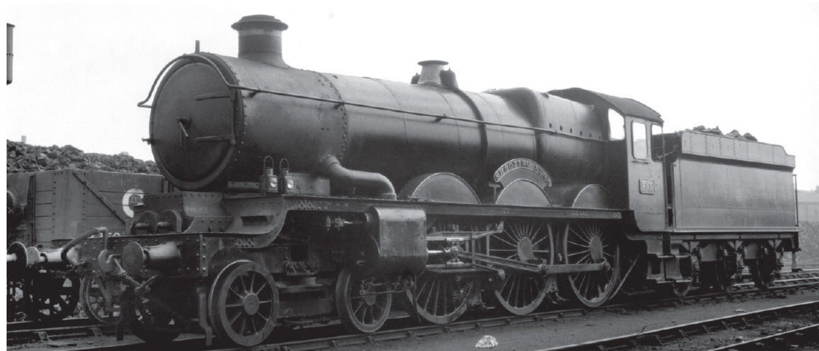
GWR 'Castle' class 4-6-0 No 4009 SHOOTING STAR was rebuilt from a 'Star' class engine of the same name and number. No 4009 is thought to be on shed at Laira in this 1930s study. J. J. Cunningham/Transport Treasury
