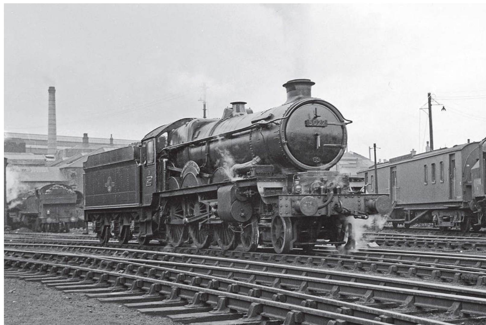
GWR 'Castle' class 4-6-0 No 5022 WIGMORE CASTLE is seen at Stafford Road (84A) in 1959. Note the stepped inside cylinder cover and the mechanical lubricator located in front of the outside steam pipe. Keith Langston Collection
