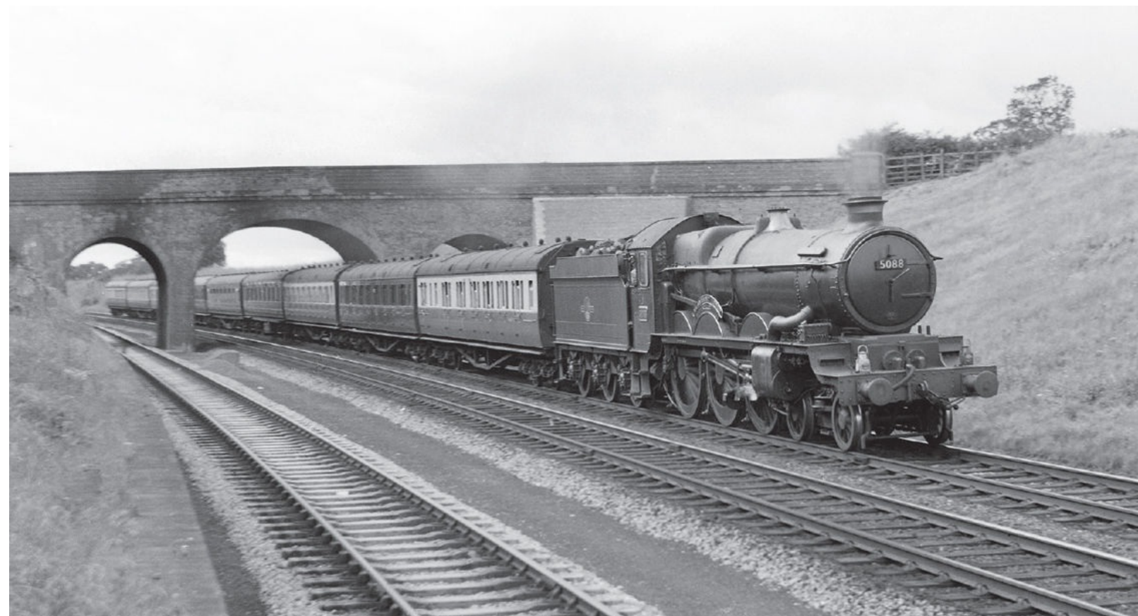
GWR 'Castle' class 4-6-0 No 5088 LLANTHONY ABBEY is seen coupled with a Collett 4000g tender displaying the 'Ferret and Dartboard' motif, near Hatton with an up express, circa 1959. Rail Photoprints Collection
