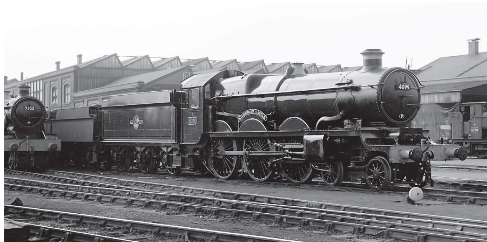
GWR 'Castle' 4-6-0 No 4099 KILGERRAN CASTLE is seen ex works at Swindon, in October 1957 after a 'Heavy Intermediate' overhaul. Note also No 7923 SPEKE HALL and Collett 'Pannier' tank No 6730. Rail Photoprints Collection
