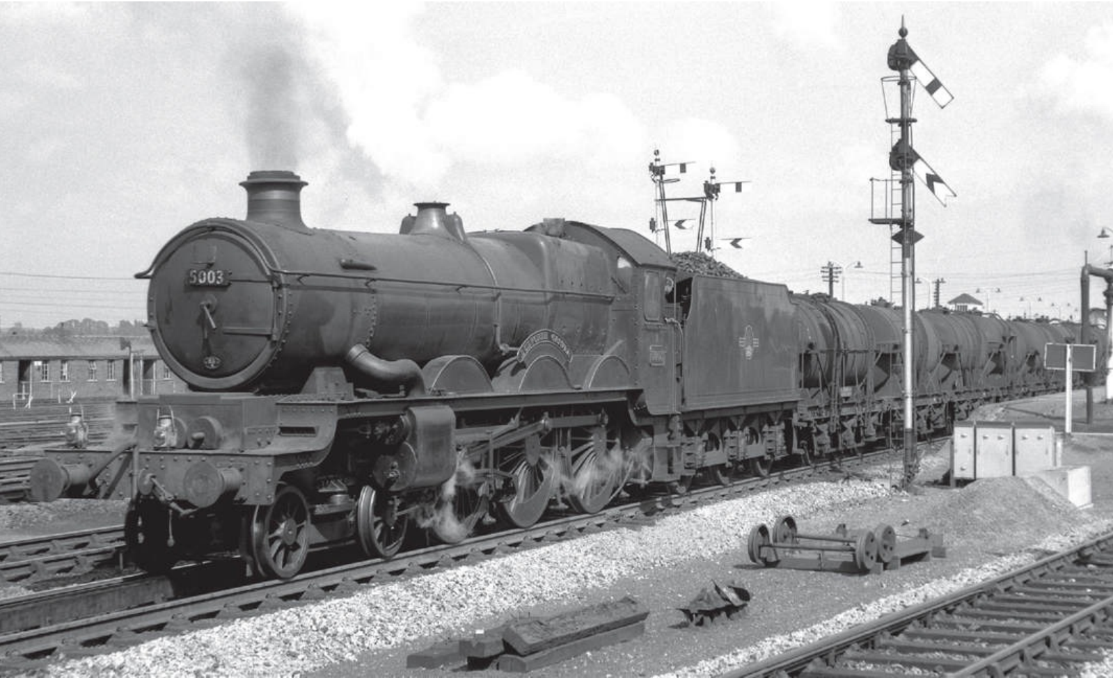
GWR 'Castle' class 4-6-0 No 5003 LULWORTH CASTLE is seen passing Didcot in the summer of 1961 with a train of milk tank empties bound for the West Country. Note that the locomotive's Hawksworth tender is filled with Ovoids*,
