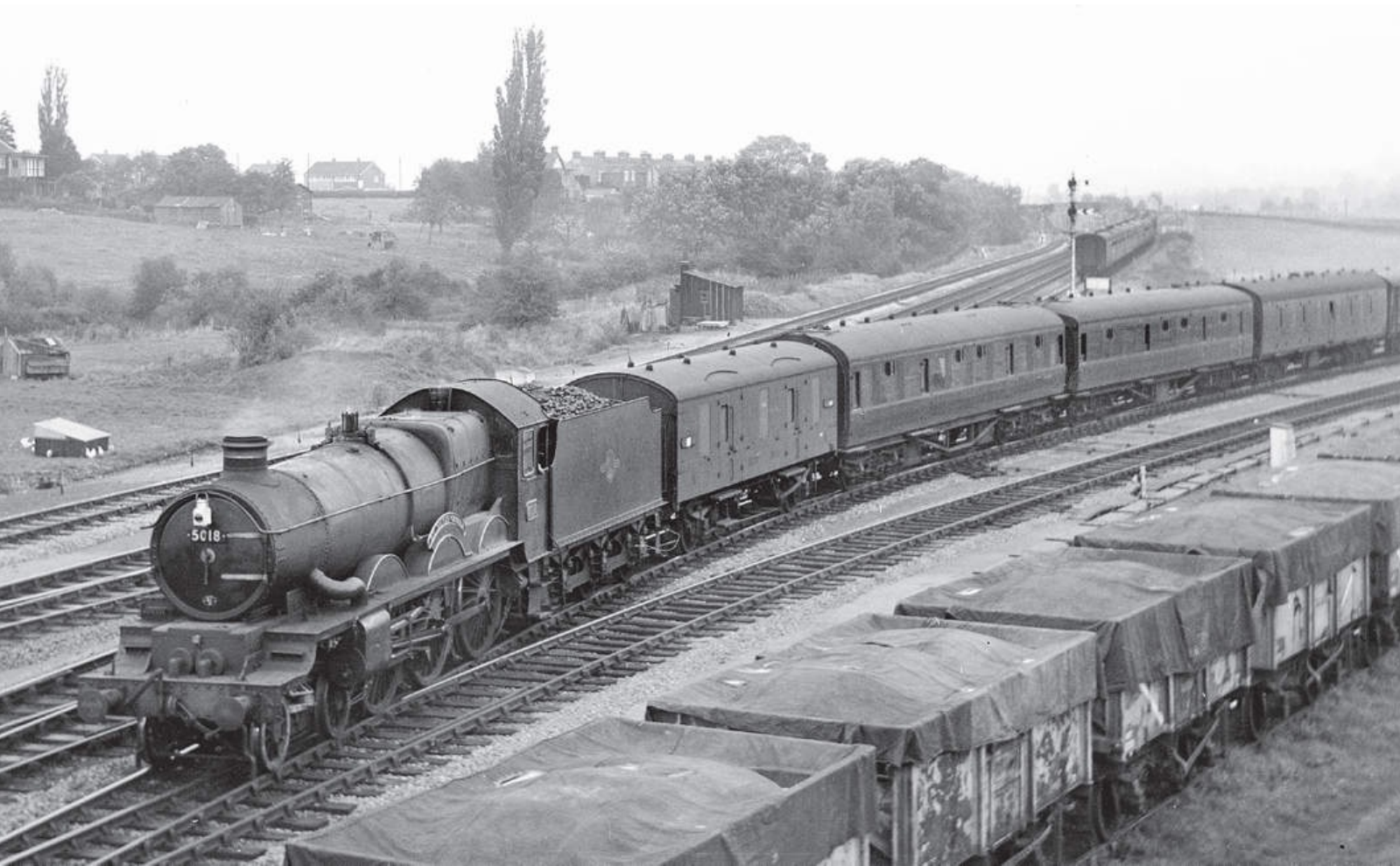
GWR ‘Castle’ class 4-6-0 No 5018 ST.MAWES CASTLE is seen without a safety valve cover. Note also the higher central step section of the inside cylinder cover. No 5018 approaches Westbury with a service from Reading, during May 1963. The Hawksworth tender looks to be filled with anthracite ovoids. Rail Photoprints Collection
