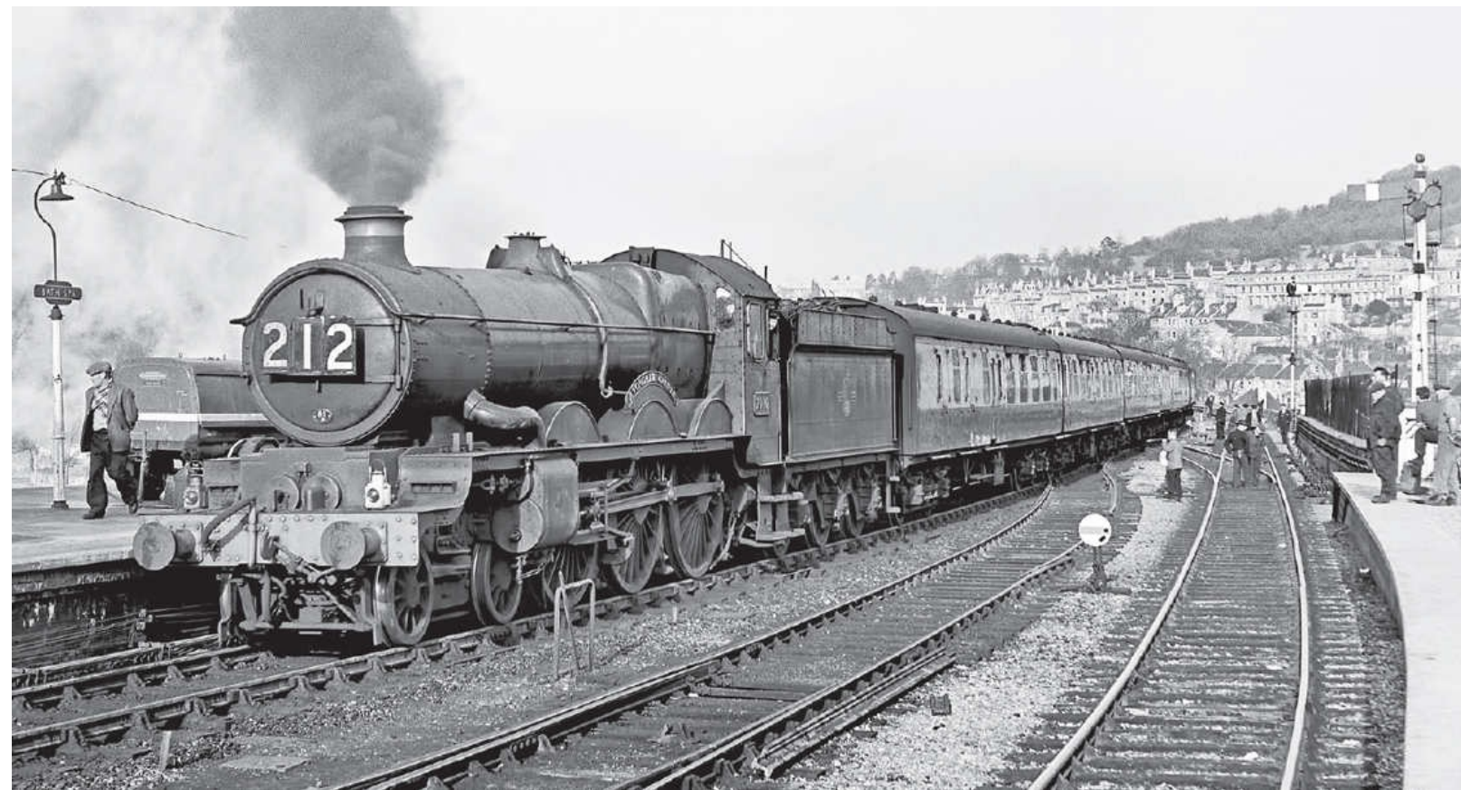
Running wrong line BR/WR 'Castle' class 4-6-0 No 7010 AVONDALE CASTLE (in single chimney form) arrives at Bath Spa with the 12.30 (Sun) Paddington-Bristol service, on 28th February 1960. The reason for the wrong line running was ongoing permanent way repairs and the 'gang' can be seen to the right of the train. Hugh Ballantyne/Rail Photoprints
