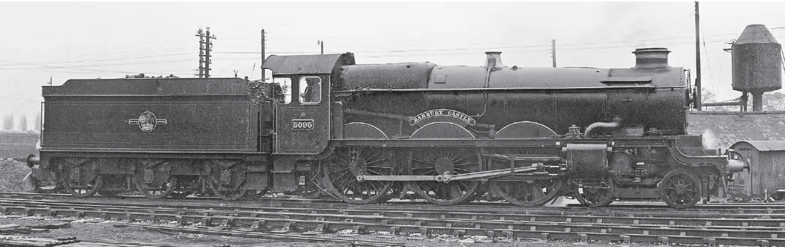
GWR ‘Castle’ class 4-6-0 No 5095 BARBURY CASTLE, with double chimney, is seen at Shrewsbury in June 1960. Rail Photoprints Collection
