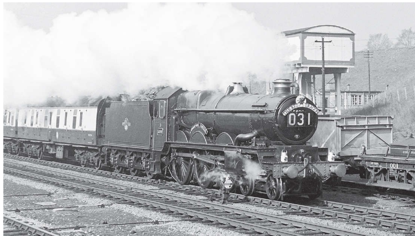
GWR 'Castle' class 4-6-0 No 5099 COMPTON CASTLE, with Hawksworth 4000g tender, is seen passing Stoke Gifford with the up 'The Red Dragon', in 1960. The engine is carrying the 3rd style of 'The Red Dragon' headboard (introduced in 1956) which was surmounted by a disc containing a dragon emblem. Rail Photoprints Collection
