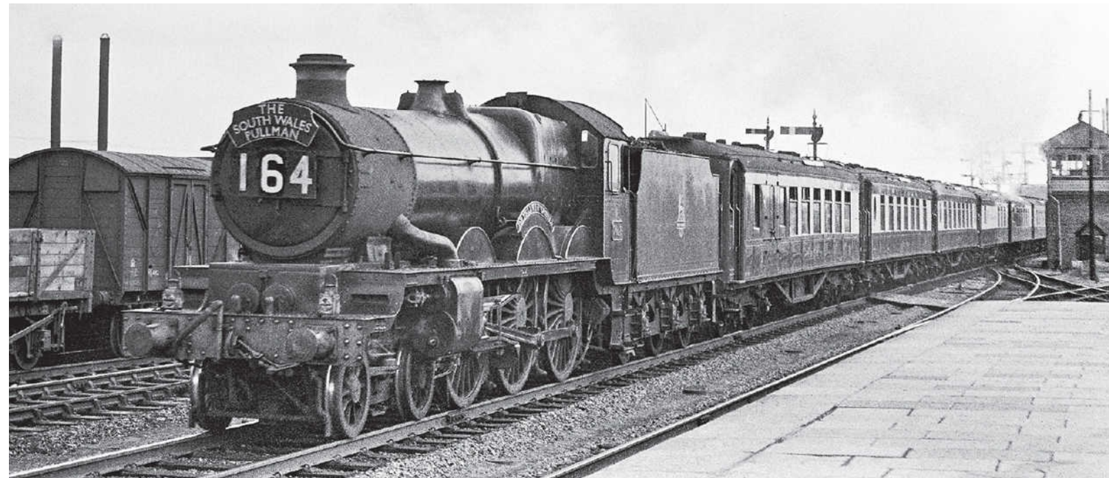
BR/WR 'Castle' class 4-6-0 No 7018 DRYSLLOWYN CASTLE is seen as a single chimney engine running through Swindon station with the up 'South Wales Pullman' on 10th August 1955. Rail Photoprints Collection
