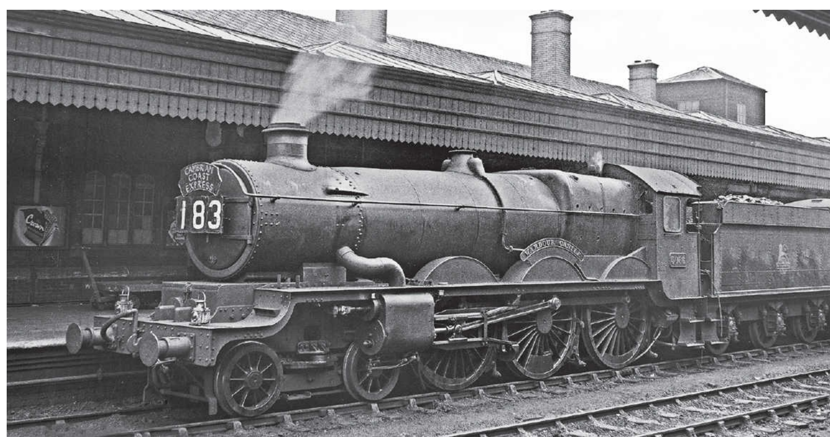
GWR 'Castle' class 4-6-0 No 5066 seen as WARDOUR CASTLE after arriving at Shrewsbury with the down 'Cambrian Coast Express', 1954. Note the non-stepped inside cylinder cover, two brackets for out of use lamps forward of the steam pipe and also the short fire iron compartment between the cab and trailing wheel splasher. Cresselly Photos Collection
