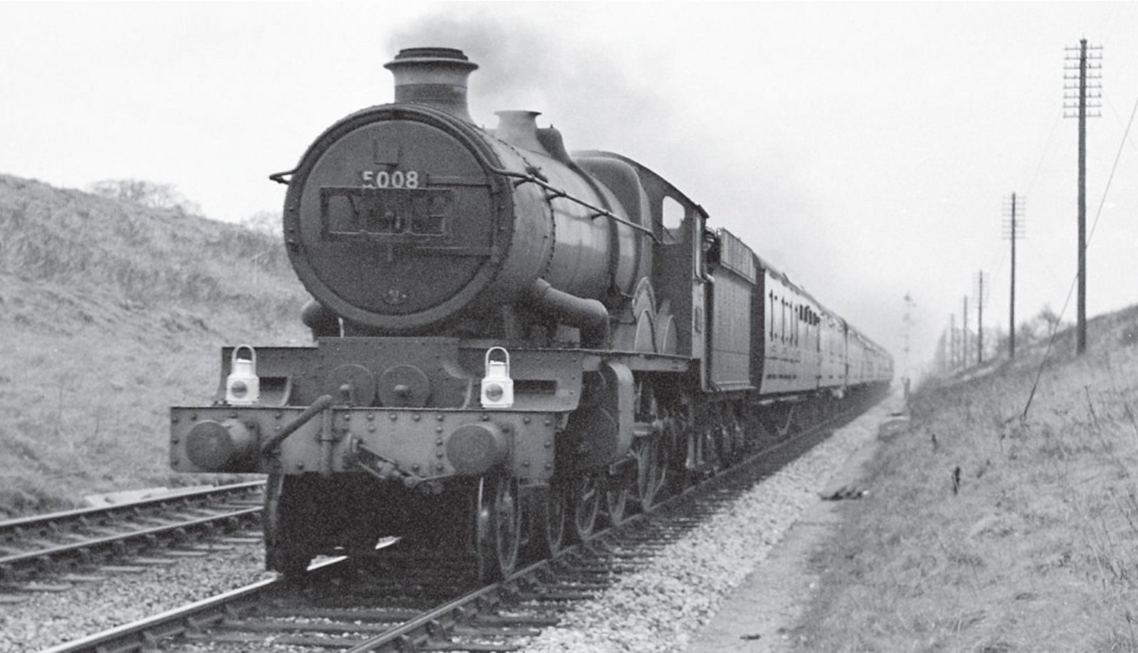
GWR 'Castle' class 4-6-0 No 5008 RAGLAN CASTLE (original GWR inside cylinder casing) is seen approaching Chippenham with a Paddington-Bristol service, circa 1955. Rail Photoprints Collection
