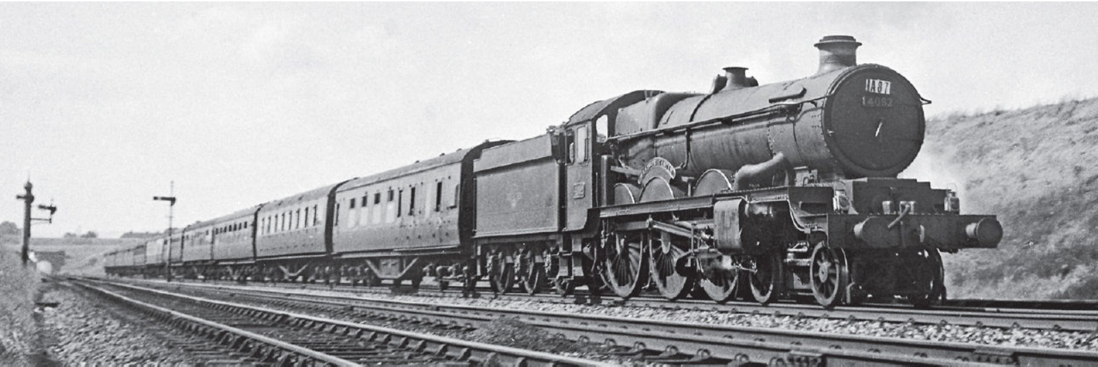
GWR ‘Castle’ class 4-6-0 No 4082 WINDSOR CASTLE (BR style stepped inside cylinder cover) climbs away from the Severn Tunnel towards Pilning with a South Wales-Paddington service, in August 1961. This engine was originally No 7013 BRISTOL CASTLE. A.E.Durrant/Rail Photoprints
