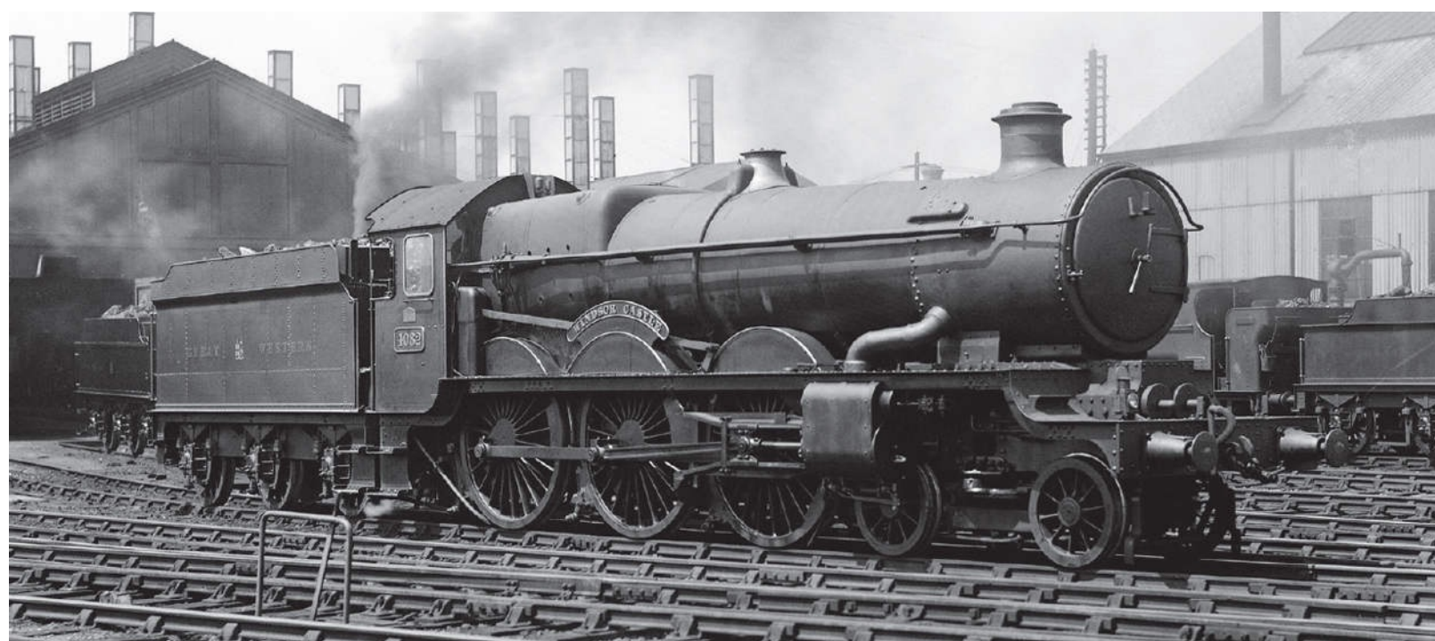
The first GWR ‘Castle’ class No 4082 WINDSOR CASTLE, seen at Reading in 1934. Note the extra plate above the cabside numberplate, commemorating the occasion of the engine being driven from Swindon Works to Swindon Station by King George VI on April 28th 1924. Note GWR original style curved sided inside cylinder casing. Rail Photoprints Collection
