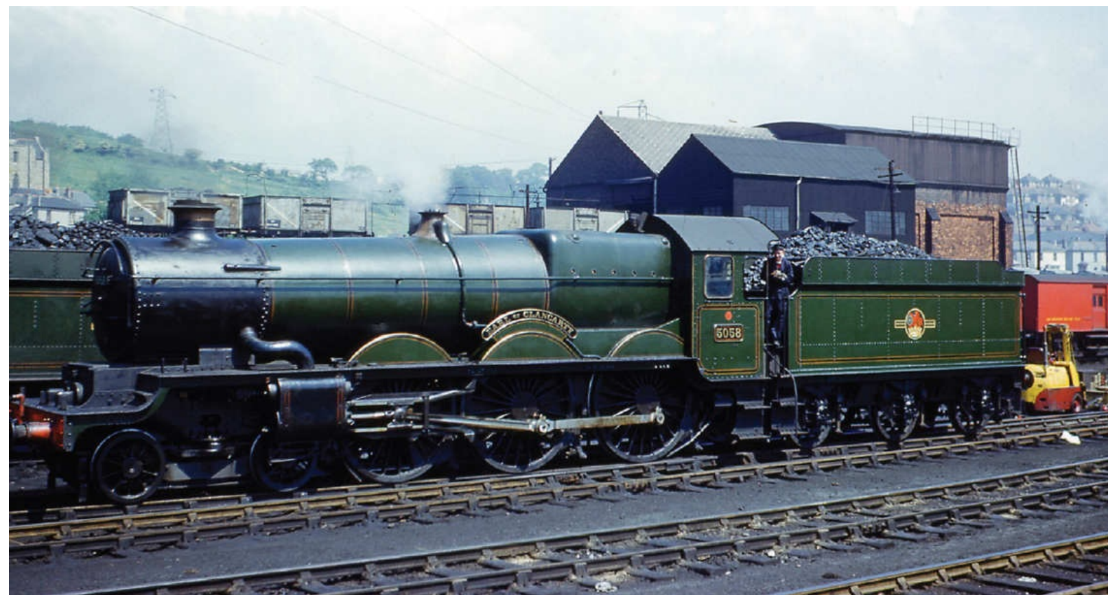
GWR 'Castle' class 4-6-0 No 5058 EARL OF CLANCARTY is seen at Plymouth Laira on 17th May 1960. Note the 'Ferret and Dartboard' BR emblem on the Collett 4000g tender. This locomotive was only ever coupled to Collett tenders during its service life (17 tender swops, the last on 21st July 1962). R.E. Vincent/Transport Treasury
