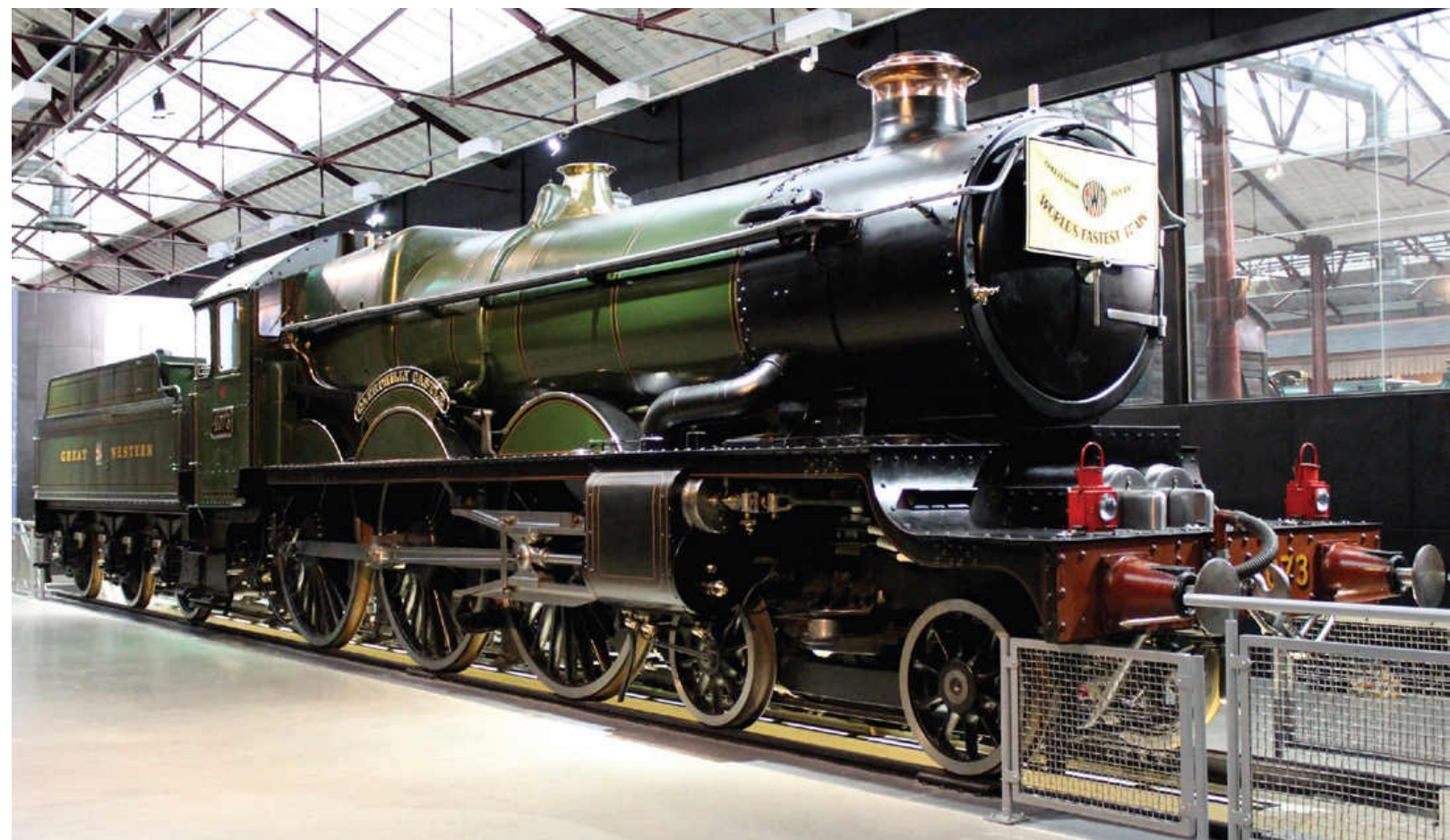
Preserved GWR built 'Castle' class locomotive No 4073 CAERPHILLY CASTLE has an example of the original small (low sided) 3,500 gallon/7 ton coal capacity tender to which the early 'Castles' were coupled until the Collett 4,000 gallon/6ton coal capacity type was put into service from 1927 onwards. The locomotive is seen at STEAM, Museum of
