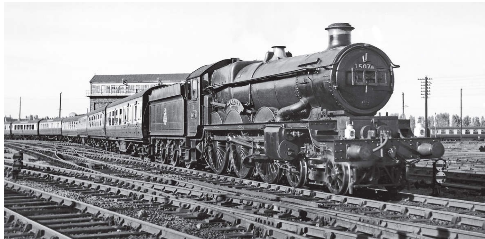
GWR 'Castle' class 4-6-0 No 5074 HAMPDEN (originally DENBIGH CASTLE) is seen leaving Shrewsbury with a long southbound train on the North and West route in 1956. Note the mechanical lubricator in the first position behind the modified outside steampipe. Rail Photoprints Collection
