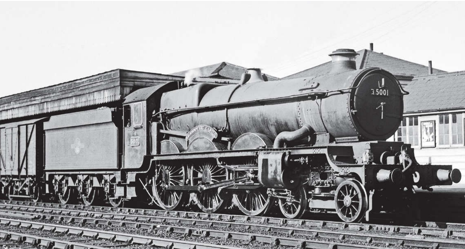
GWR 'Castle' class 4-6-0 No 5001 LLANDOVERY CASTLE is seen at Oxford station with a train of fitted vans on 18th July 1959. Note the brass beading embellishments and stepped inside cylinder cover (BR rebuild). Norman Preedy
