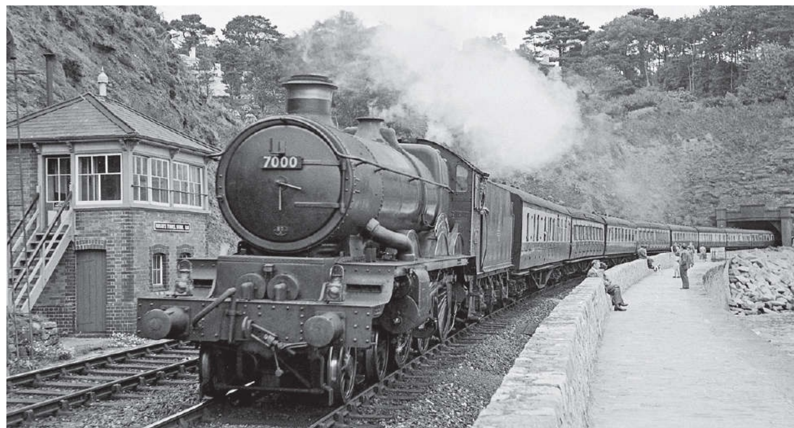
GWR 'Castle' class 4-6-0 No 7000 VISCOUNT PORTAL with Hawksworth 4000g tender is seen passing Parsons Tunnel signalbox and running along the sea wall near Teignmouth, 1957. Note the un-stepped inside cylinder cover. John Day Collection/Rail Photoprints
