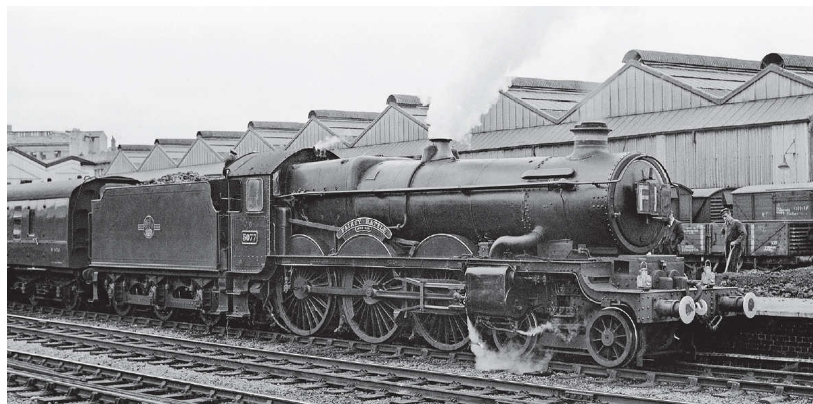
GWR 'Castle' class 4-6-0 No 5077 FAIREY BATTLE is seen in its final BR form, at Newport in April 1959. Note the rectangular hole cut into the side panel of the inside cylinder cover, presumably as an aid to inspection. Norman Preedy Collection/Rail Photoprints
