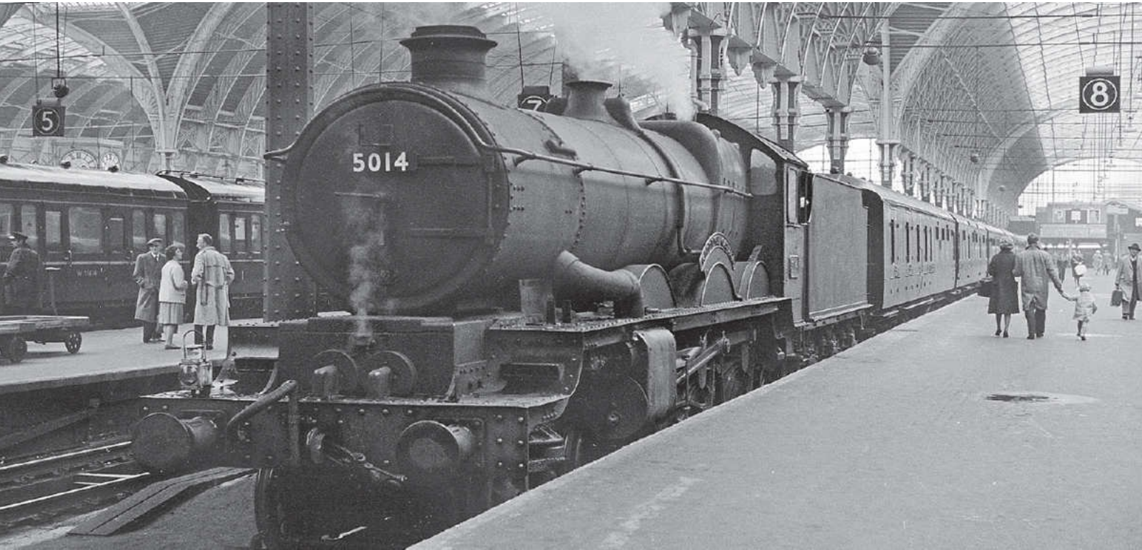
GWR ‘Castle’ class 4-6-0 No 5014 GOODRICH CASTLE is seen at Platform 8 Paddington station on 6th July 1963. Note the new BR/WR units standing at an adjacent platform. The larger stepped inside cylinder cover with associated valve cylinder lubricator is clearly visible. Rail Photoprints Collection
