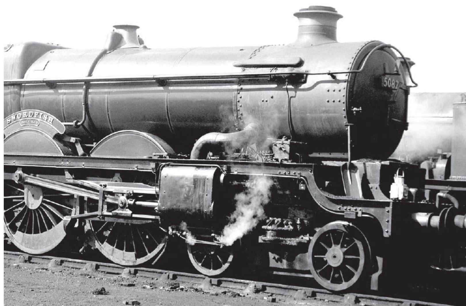
No 5082 SWORDFISH seen with 'modified' outside steampipe, shorter chimney (introduced 1936) straight frames, box pattern inside cylinder casing (Nos 5013 onwards and BR straight frame rebuilds) BR pattern parallel barrel buffers and mechanical lubricator in the final forward position, circa 1961. David Anderson
