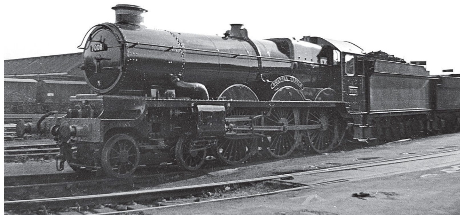
BR/WR 'Castle' class 4-6-0 No 7008 SWANSEA CASTLE is seen ex works after receiving a double chimney in June 1959. Rail Photoprints Collection
