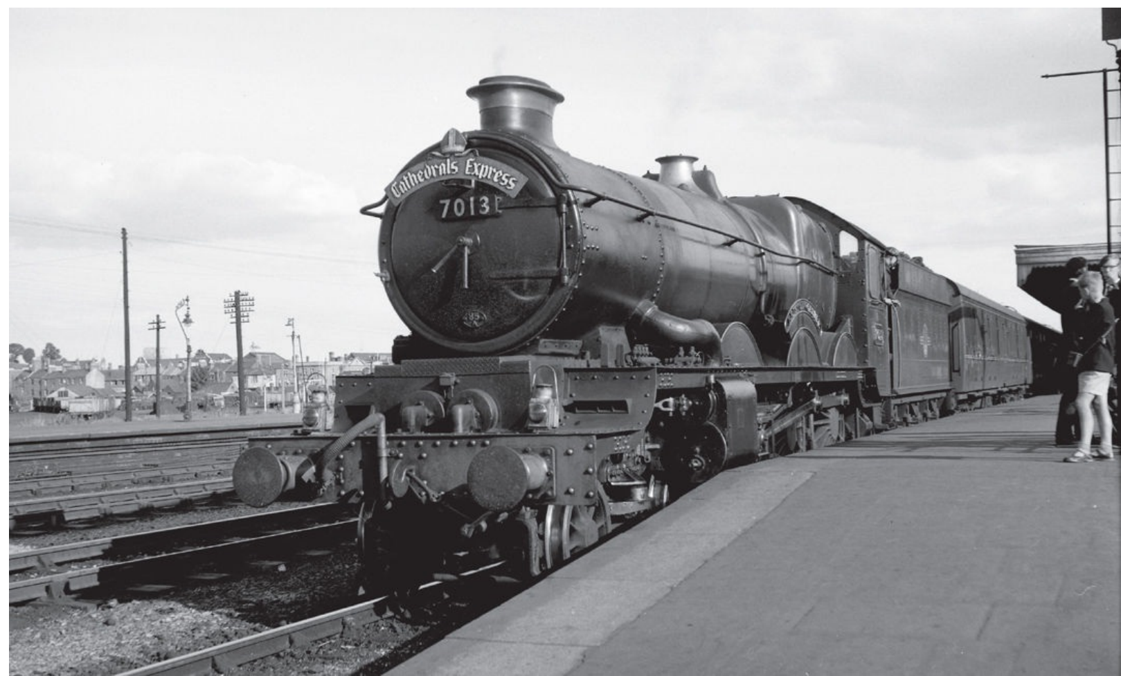
GWR 'Castle' class 4-6-0 No 7013 BRISTOL CASTLE (formerly locomotive 4082) is seen with a down 'Cathedrals Express' working at Oxford in 1962. Note the double chimney, pipe smoking driver and young admirers. David Anderson
