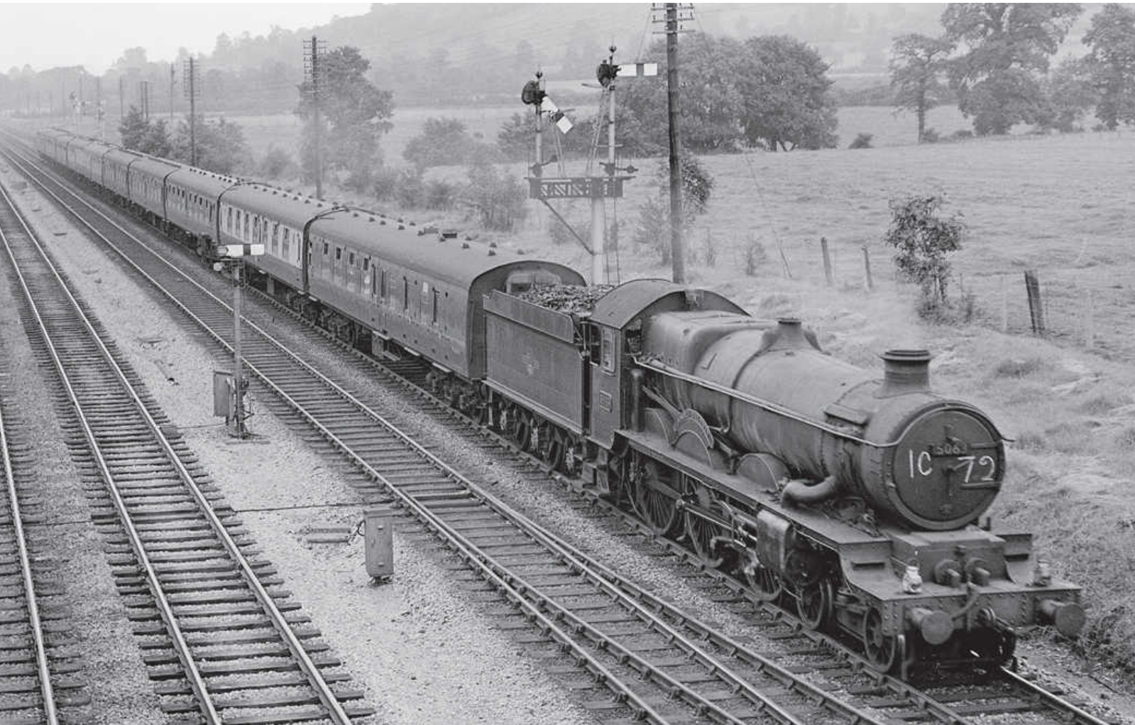
GWR 'Castle' class 4-6-0 No 5063 EARL BALDWIN approaches Standish Junction and is signalled to cross from BR/WR to BR/MR metals, as it heads the 08.00 Wolverhampton-Minehead service, on 20th July 1963. Hugh Ballantyne/Rail Photoprints
