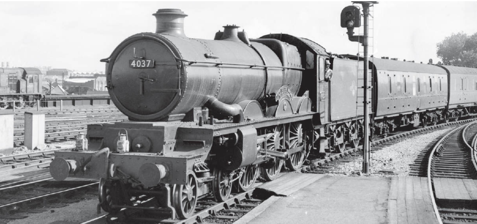
GWR Castle Class 4-6-0 No 4037 THE SOUTH WALES BORDERERS approaches Bristol Temple Meads in August 1960. Note the newer BR style 'Box' pattern inside cylinder cover with central step, Hawksworth 4000 gallon/6 ton tender, BR style parallel buffers and the regimental crest on the centre wheel splasher. Circa 1947 the brass beading was removed from the front end of the cabs on all engines up to and including No 5012. Rail Photoprints Collection
