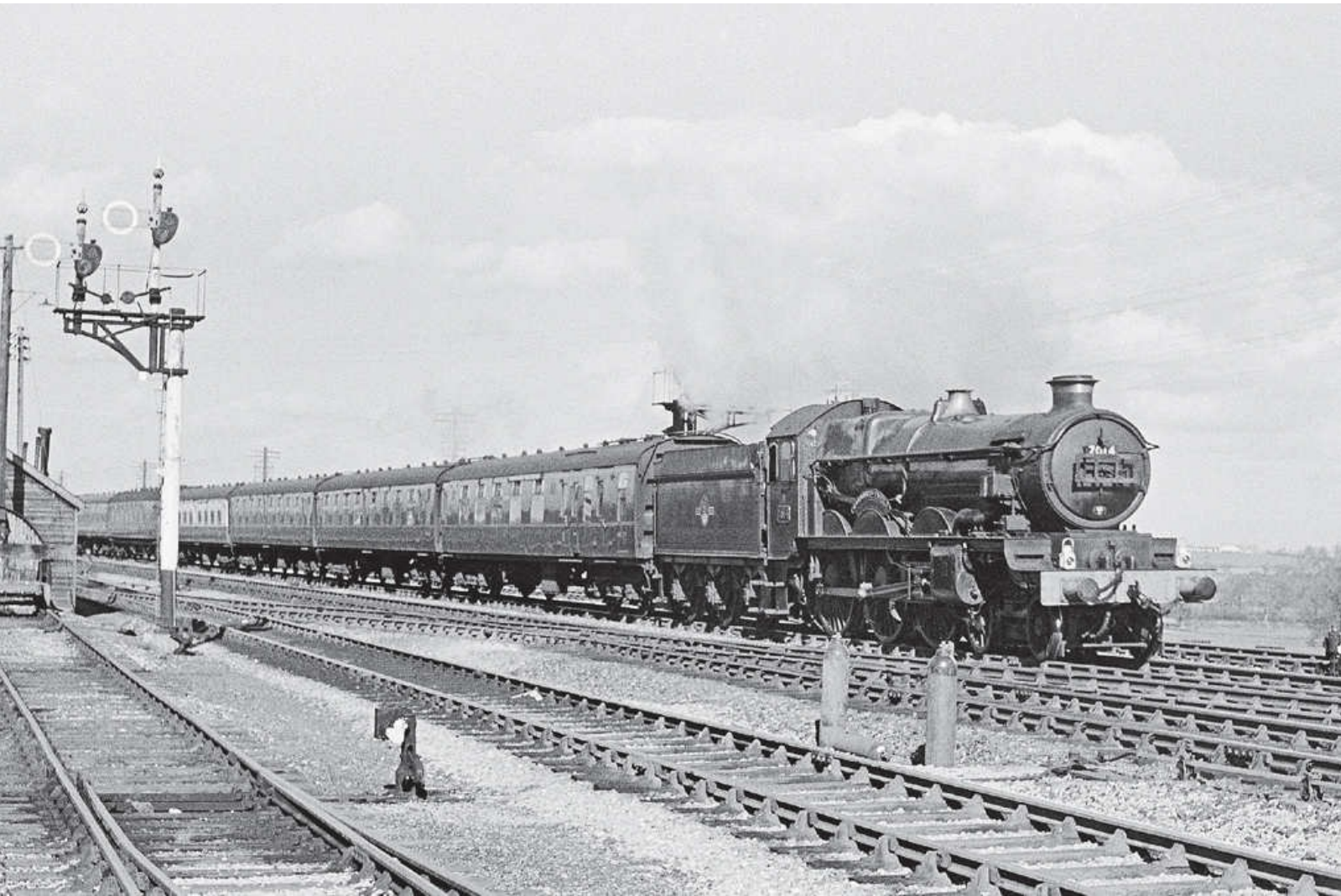
BR/WR ‘Castle’ class 4-6-0 No 7014 CAERHAYS CASTLE is seen passing Thingley Sidings, near Chippenham with a down Bristol service, in 1959. Note the smokebox mounted reservoir associated with the Davies & Metcalf lubricator. Norman Preedy Collection/Rail Photoprints
