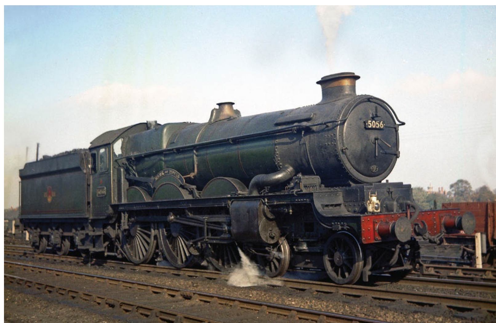
GWR 'Castle' class 4-6-0 No 5056 EARL OF POWIS is seen at Shrewsbury in October 1962. Note the mechanical lubricator mounted in front of the 'steam' pipe, also the box cover housing the lubricator pipes to valves, pistons and the regulator valve as they leave the 4 row superheater boiler and enter the smokebox (seen above the handrail and below the double chimney). Rail Photoprints Collection
