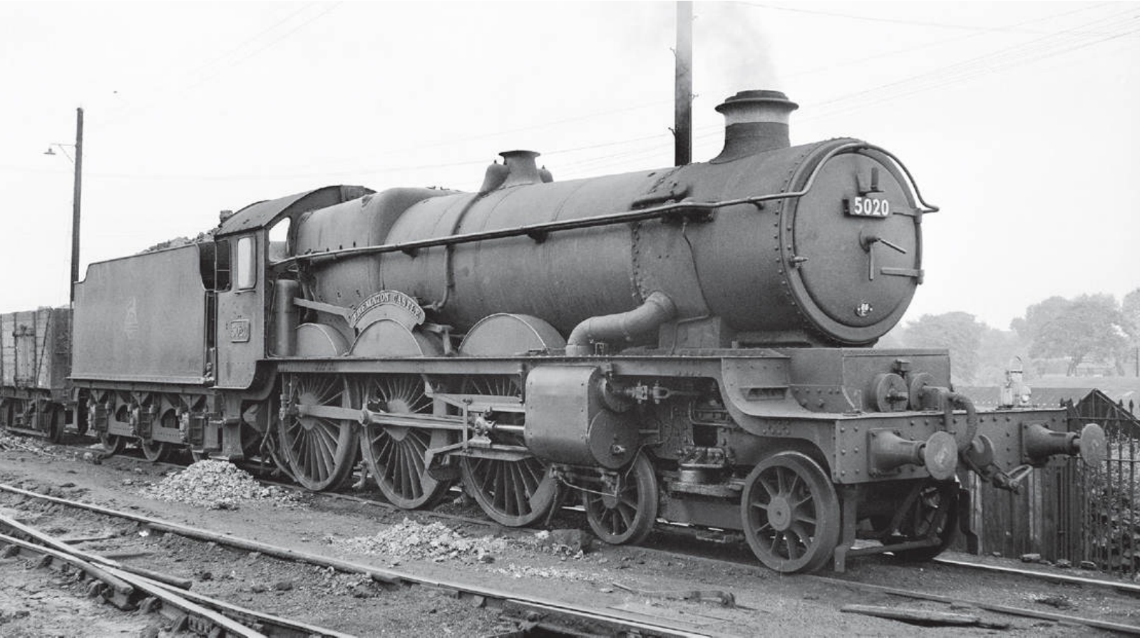
GWR ‘Castle’ class 4-6-0 No 5020 TREMATON CASTLE (un-stepped inside cylinder cover) is seen at Shrewsbury, circa 1957. Rail Photoprints Collection
