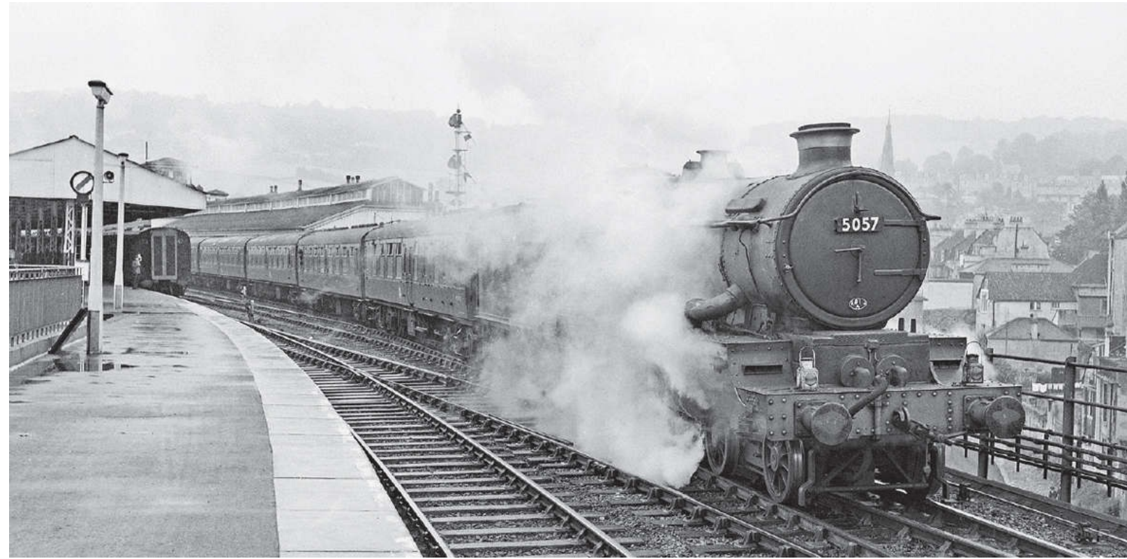
GWR 'Castle' class 4-6-0 No 5057 EARL WALDEGRAVE draws forward to make a second stop with the 09.45 Paddington-Weston-super-Mare service, on 29th June 1963. Note the banner repeater signal on the up platform is 'off' as that train leaves the station. Hugh Ballantyne/Rail Photoprints
