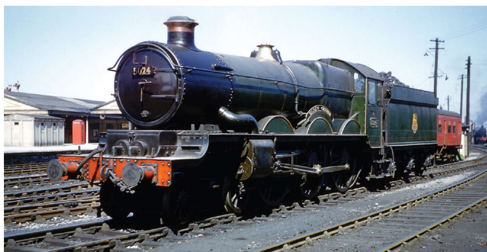
GWR 'Castle' class 4-6-0 No 5024 CAREW CASTLE is seen at Newton Abbot (83A) in April 1956. Note the rounded front edge of the centre cylinder cover. Roy Vincent Collection/Transport Treasury
