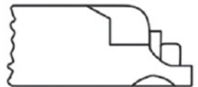
Fig 2. Straight frame with dished area, giving bogie wheel clearance. Locomotive No 4093 and all later GWR/BR 'Castles' (and rebuilds).
