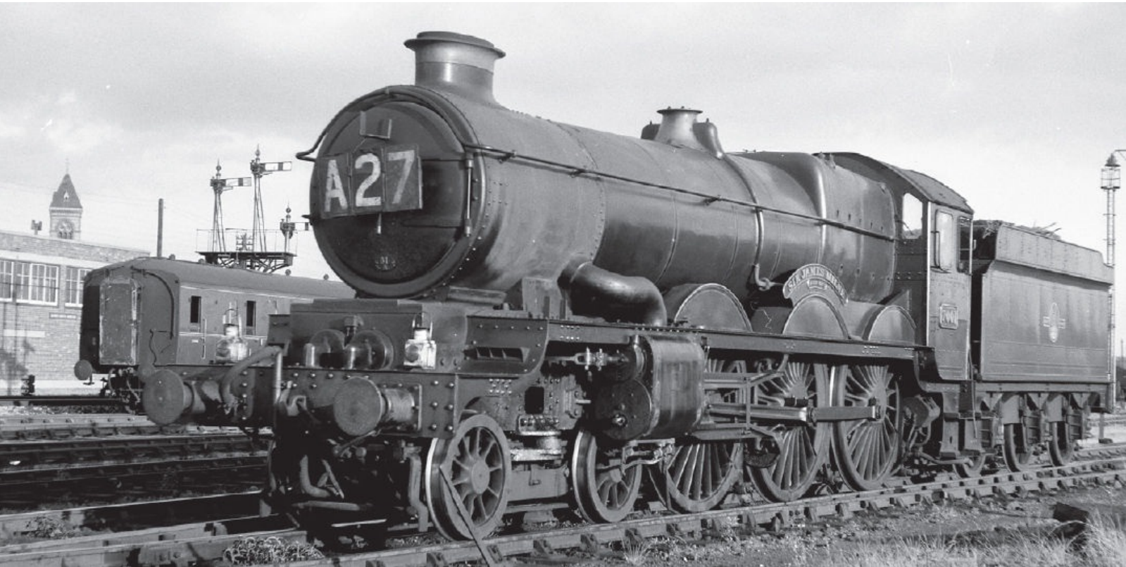
GWR 'Castle' class 4-6-0 No 7001 SIR JAMES MILNE is seen at Oxford. The locomotive's double chimney is seen to good effect in this 1961 image. Note the Hawksworth coach beyond the locomotive. David Anderson
