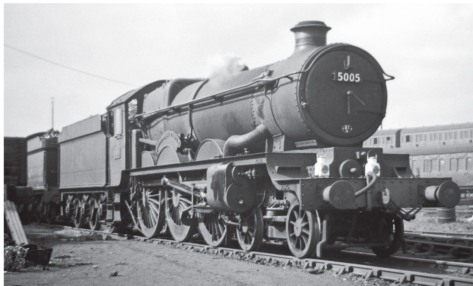
GWR 'Castle' class 4-6-0 No 5005 MANORBIER CASTLE without streamlining and with original GWR style inside cylinder casing is seen at Old Oak Common depot (81A) in May 1958. The modified design of curved steam pipe which over time replaced the original straight pattern in order to eliminate occasional incidences of fractures can clearly be seen. Note also the special type of snifting valve on the centre cylinder cover which is a survivor from the locomotives streamlined days. Keith Langston Collection
