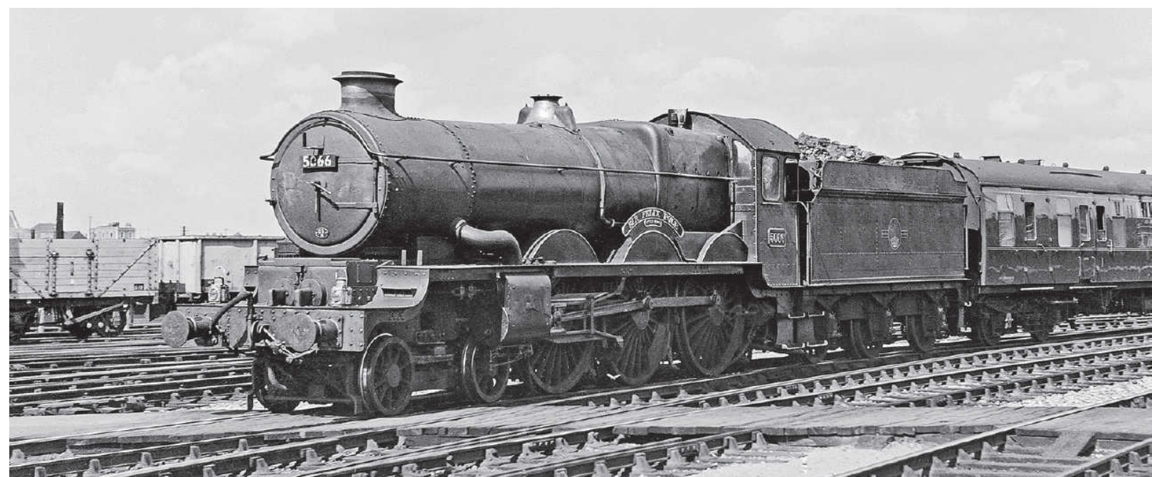
GWR 'Castle' class 4-6-0 No 5066 seen with double chimney as SIR FELIX POLE whilst approaching Bristol Temple Meads with a southbound North and West route service, in August 1960. Note the stepped inside cylinder cover. Rail Photoprints Collection
