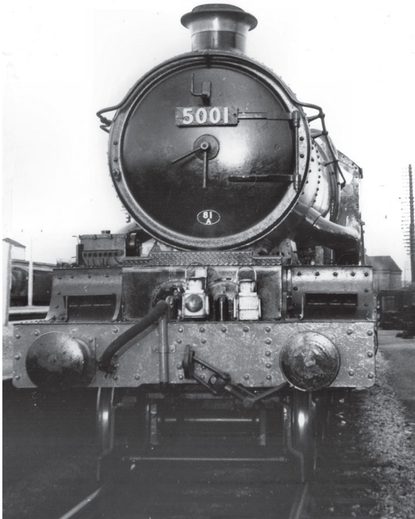
GWR 'Castle' class 4-6-0 No 5001 LLANDOVERY CASTLE is seen in ex works condition at Didcot in August 1961. Note the BR style higher central step section of the 'Box' style inside cylinder cover, and also the mechanical lubricator located in front of the offside outside steam pipe. David Anderson
