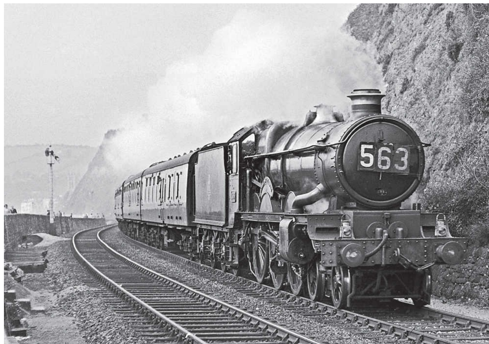
GWR 'Castle' class 4-6-0 No 5059 EARL ST ALDWYN runs along the sea wall at Teignmouth with an up express, on 1st August 1951. The then Exeter allocated Hawksworth tendered engine looked to be in fine fettle. Norman Preedy Collection/Rail Photoprints
