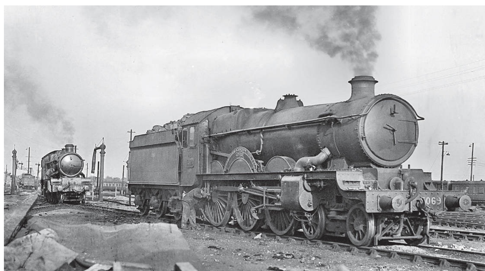
GWR 'Castle' class 4-6-0 No 5069 ISAMBARD KINGDOM BRUNEL is seen in 1947 at Old Oak Common depot in the company of sister engine No 5013 ABERGAVENNY CASTLE, circa 1947. Note the locomotive numbers on the buffer beam and the qualifying wording 'Castle Class' which is clearly seen beneath the main nameplate. Mike Morant Collection
