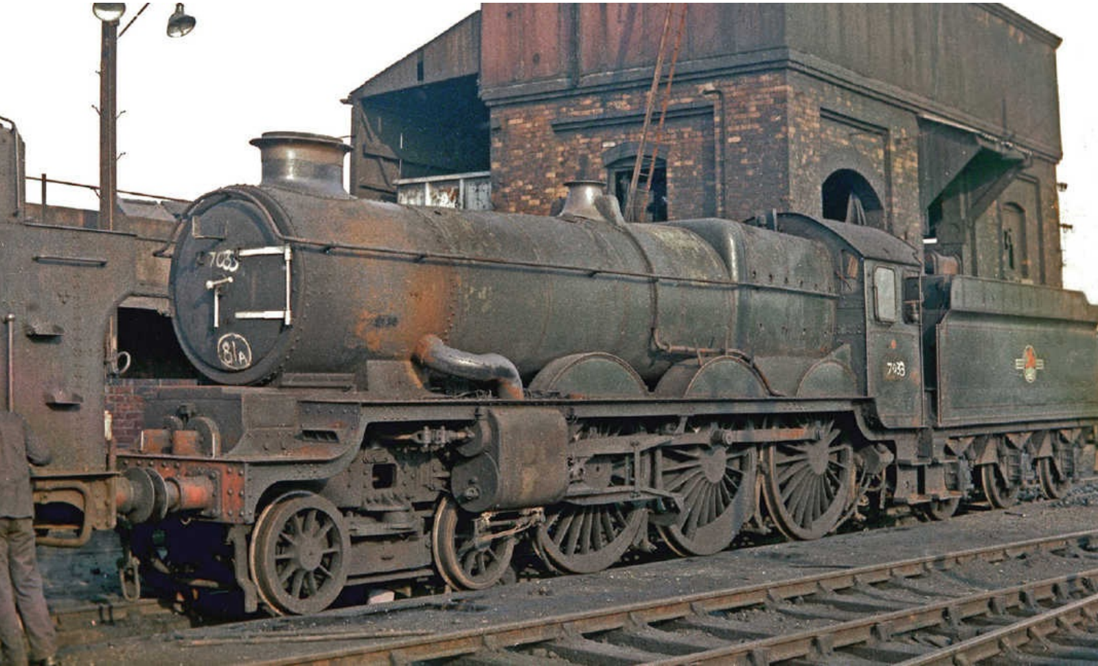
'The end is nigh!' Shorn of name and number plates BR/WR 'Castle' class 4-6-0 No 7033 HARTLEBURY CASTLE is seen in rundown condition at Shrewsbury depot pending the locomotive's last trip to Cashmores Great Bridge, Tipton. Rail Photoprints Collection
