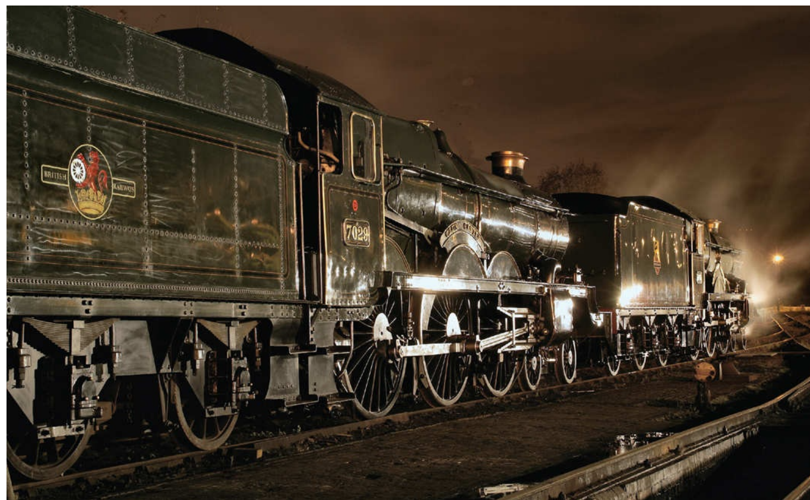
‘Castles in the Night’. An evocative study of two Tyseley based preserved ‘Castle’ class engines seen on shed. No 7029 CLUN CASTLE (BR/WR) with a Collett 4000g tender and No 5043 EARL OF MOUNT EDGCUMBE (GWR) with a Hawksworth 4000g tender. Phil Neale
