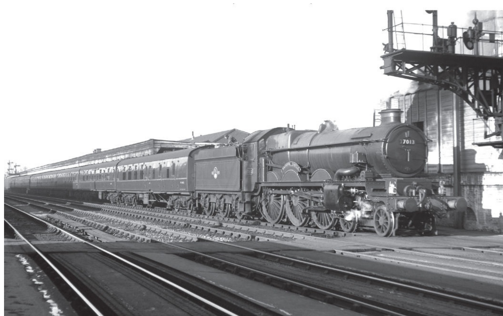
GWR 'Castle' class 4-6-0 No 7013 BRISTOL CASTLE is again seen at Oxford station on this occasion with a Worcester-Paddington service on 18th March 1961. Note that the smokebox reservoir associated with the Davies & Metcalf patent lubricator can be clearly identified. David Anderson
