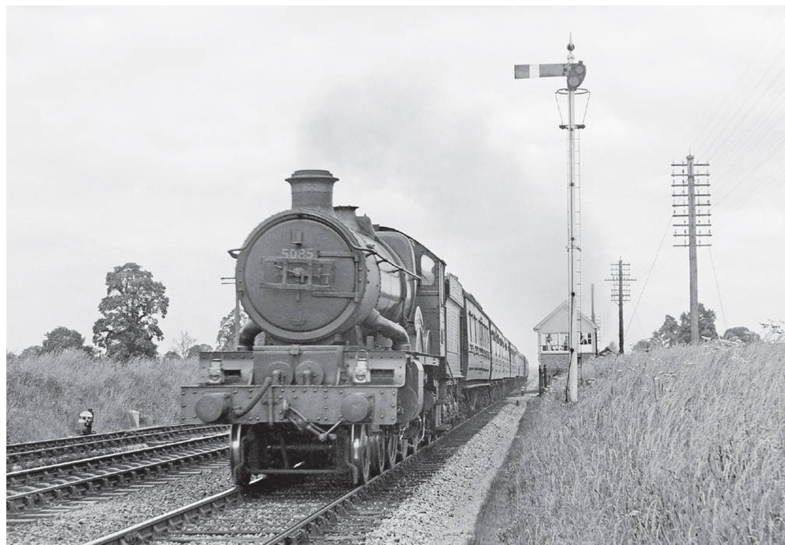
'Castle' class No 5085 EVESHAM ABBEY, built from 'Star' class No 4065, is seen passing Langley Crossing (east of Chippenham) in 1957. Note this engine was one of the 11 given new front section frames. Rail Photoprints Collection
