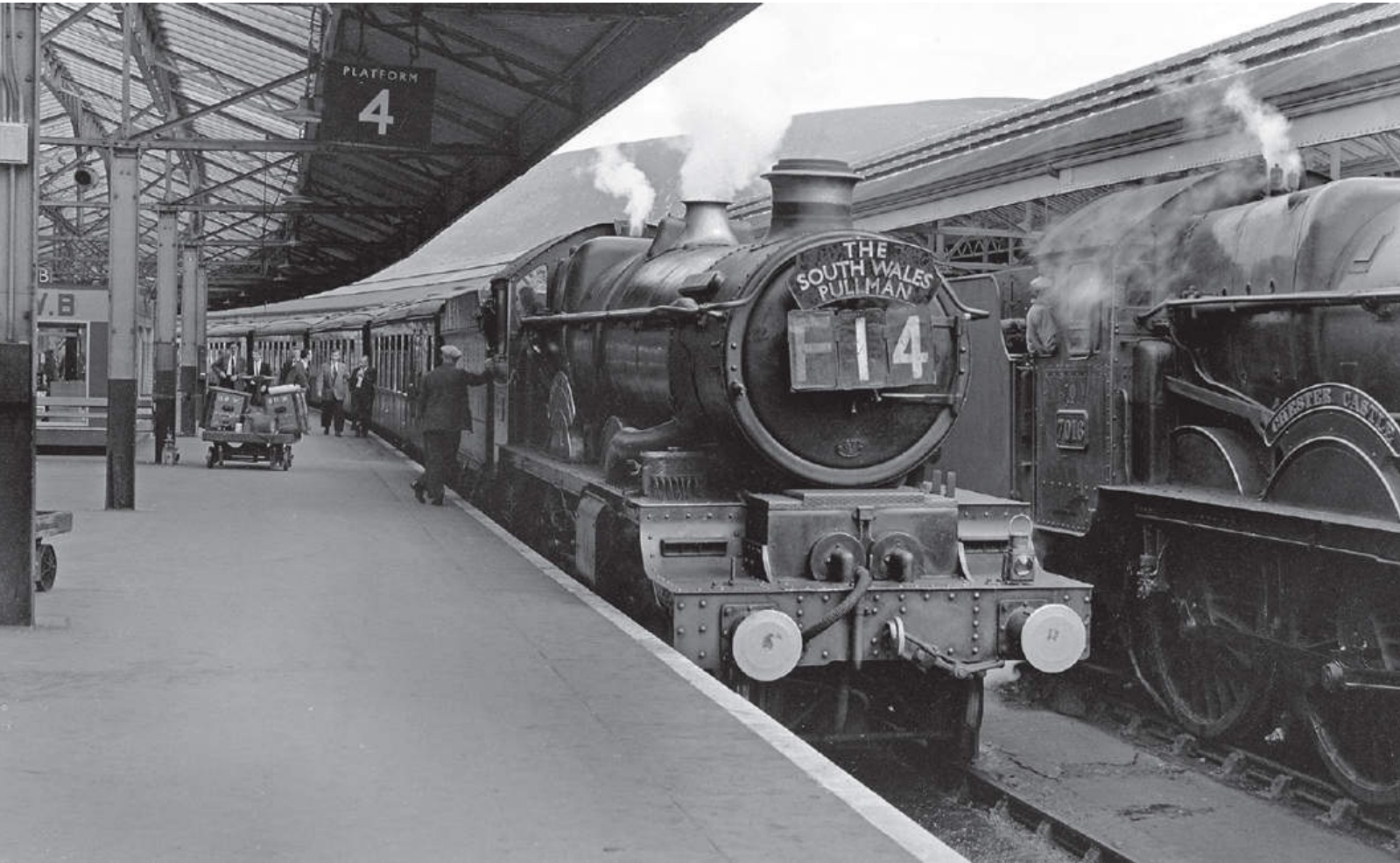
One of the last steam operated ‘South Wales Pullman’ services stands at Swansea High Street after arrival behind Castle 4-6-0 5048 EARL OF DEVON, September 1961. Part of ‘Castle’ class No 7016 CHESTER CASTLE can be also be seen. Note the Mechanical lubricator forward of the steam pipe and the stepped inside cylinder cover. Hugh Ballantyne/Rail Photoprints
