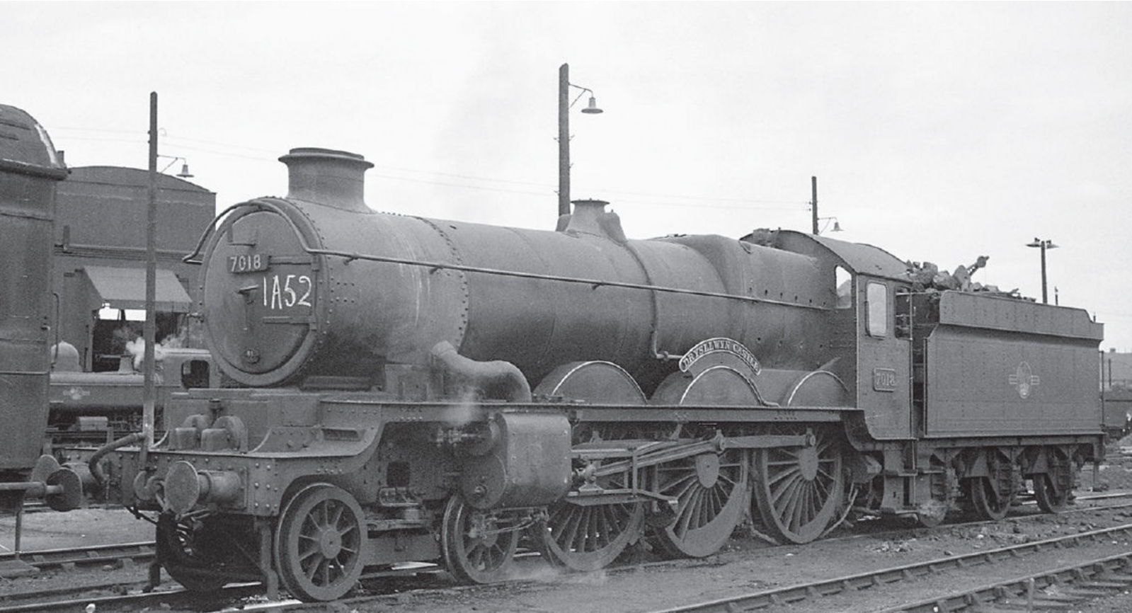
BR/WR ‘Castle’ class 4-6-0 No 7018 DRYSLWYN CASTLE is seen as a double chimney engine in the shed yard at Old Oak Common (81A) in August 1962. On 28th April 1958 this engine whilst working the up ‘Bristolian’ had reportedly passed Little Somerford at 100mph, arriving at London Paddington in 94 minutes. Rail Photoprints Collection
