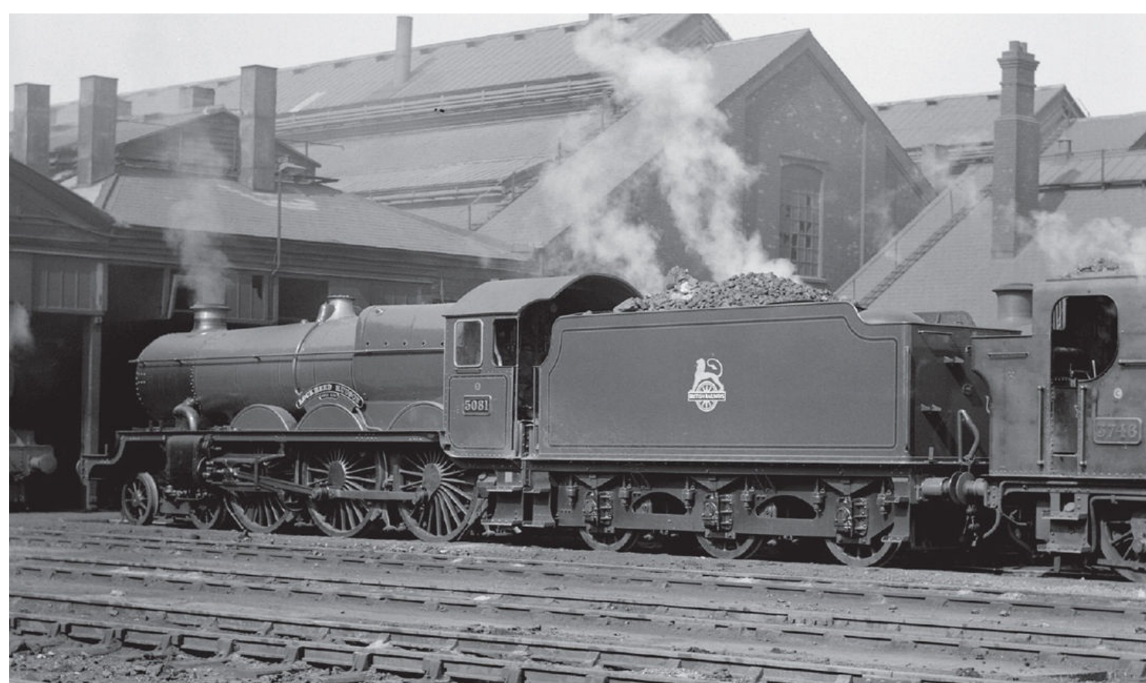
GWR 'Castle' class 4-6-0 No 5081 LOCKHEED HUDSON is seen on shed at Swindon (82C) on 24th April 1956. Note Hawksworth tender No 4105 which was coupled with this engine 5 days before this picture was taken. Transport Treasury
