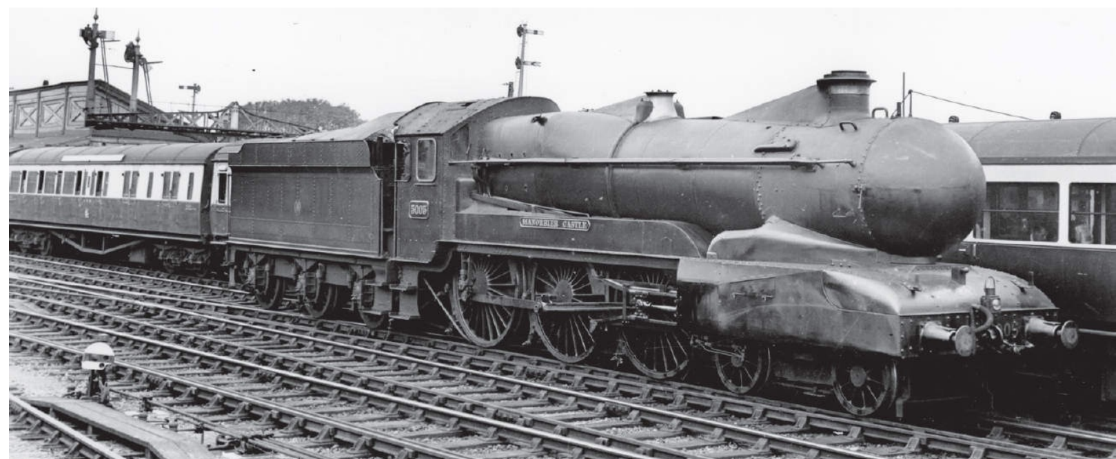
Streamlined GWR 'Castle' class 4-6-0 No 5005 MANORBIER CASTLE seen at Leamington Spa with the full casing and cab roof extension in May 1935. Note the straight nameplate on the splasher. Mike Bentley Collection
