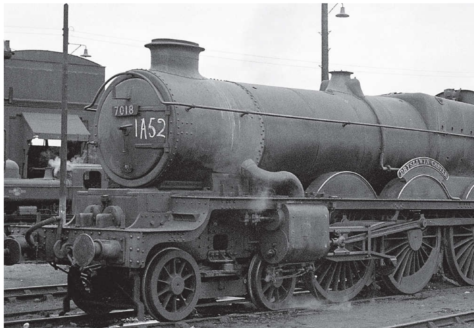
'Castle' class 4-6-0 No 7018 DRYSLLYN CASTLE was fitted with an experimental double chimney in May 1956, the engine is seen with a GWR 'Standard' double chimney which was fitted in April 1958. The ultimate 'Castle' class development was achieved when No 4090 DORCHESTER CASTLE became the first to be fitted with a double chimney and 4-row superheated boiler (HD 7671) in March 1957. Following that successful development a total of 65 'Castles' were eventually rebuilt with 4-row superheaters and double chimneys. Image circa 1962. Keith Langston Collection
