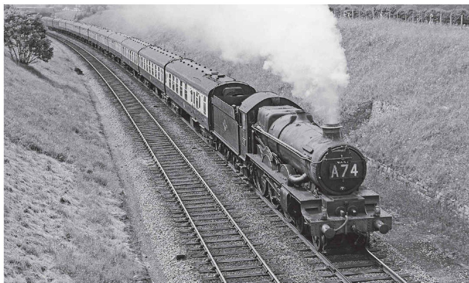
BR/WR 'Castle' class 4-6-0 No 7026 TENBY CASTLE, with Collett 4000g tender and stepped inside cylinder cover, is seen approaching Twerton Tunnel with the 10.35 (So) Weston-super-Mare to Paddington service, on 30th June 1962.
