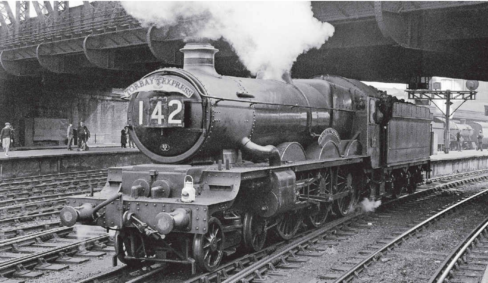
GWR ‘Castle, Class 4-6-0 No 5024 CAREW CASTLE is seen preparing to back onto the down ‘Torbay Express’ at Paddington circa 1959. Note the stepped inside cylinder cover and the storage compartment for short fire irons between the nearside centre and trailing wheel splashers. The Swindon BR/WR cast headboard carried in this instance is the third and final design incorporating the Devon county crest. Rail Photoprints Collection
