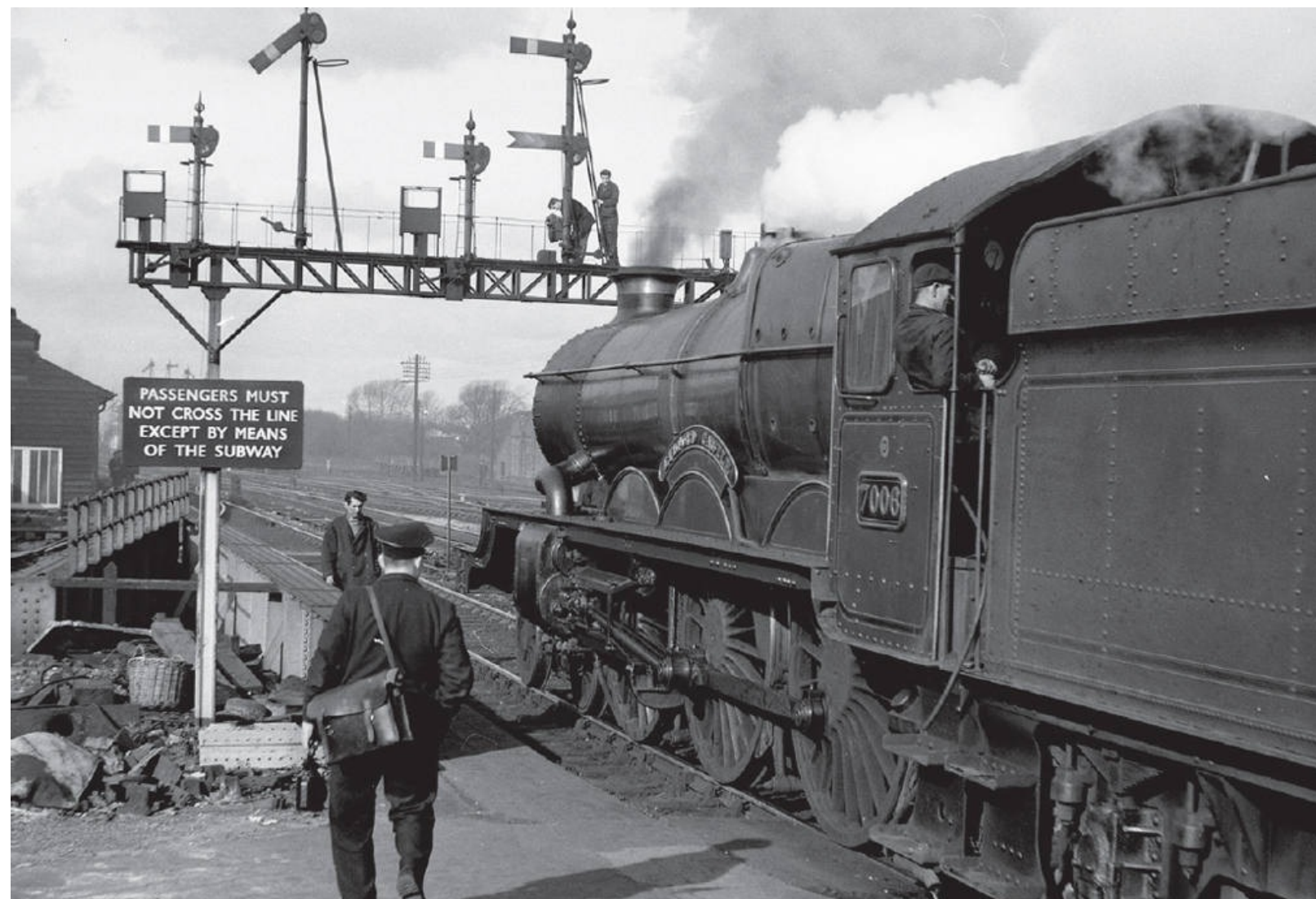
Plenty of activity to be seen in this study, as GWR 'Castle' class 4-6-0 No 7006 LYDFORD CASTLE waits to depart from Oxford station with a down Paddington-Worcester service on 2nd March 1961. Note that the rear nearside sandbox can be clearly seen located between the cab steps and trailing driving wheel. David Anderson
