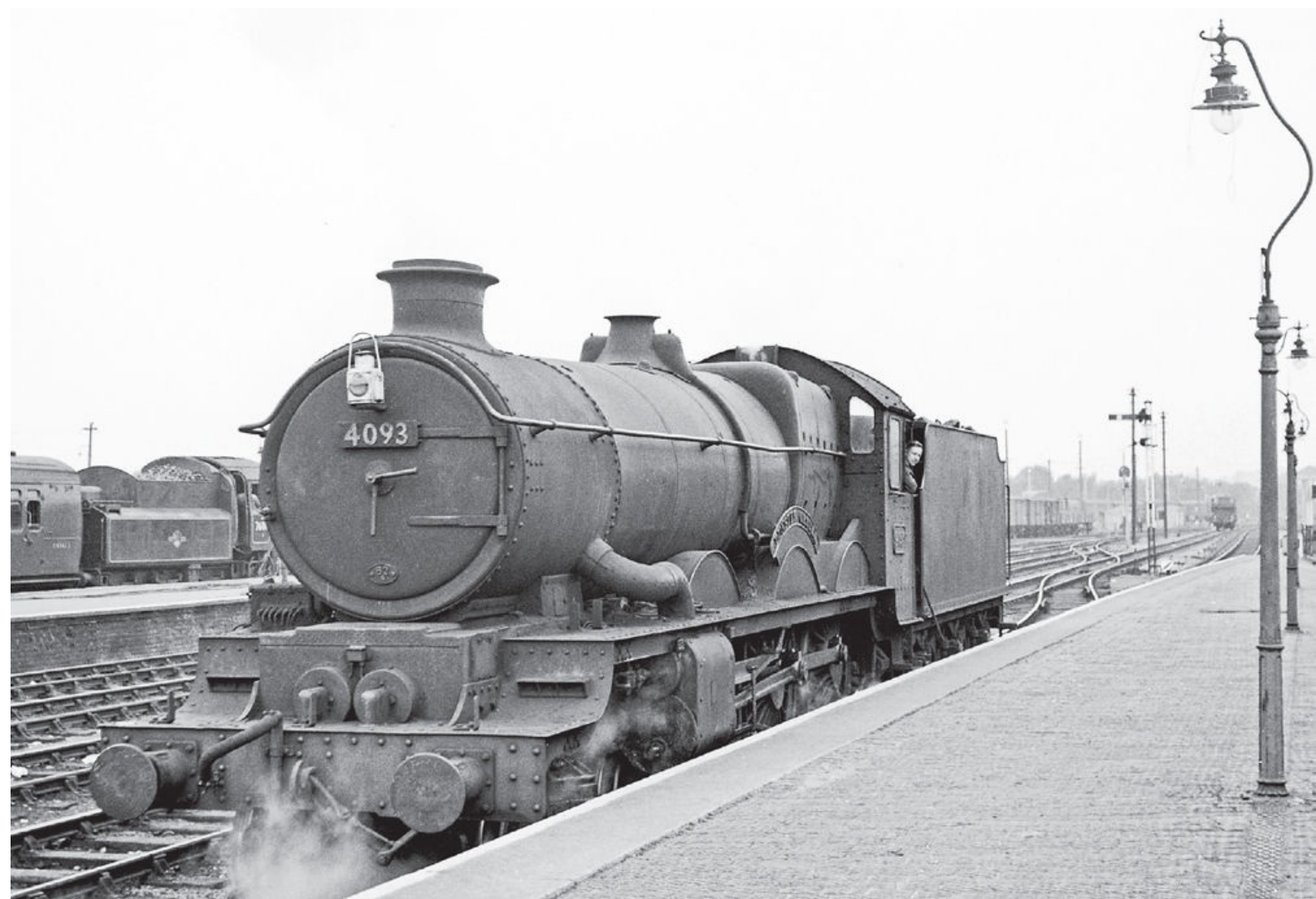
GWR 'Castle' class 4-6-0 No 4093 DUNSTER CASTLE backs out of Weymouth having arrived with a service from Bristol, 22nd July 1963. Note the Hawksworth 4000 gallon, 6 ton tender attached 28/03/60 and the stepped inside cylinder cover. Rail Photoprints Collection
