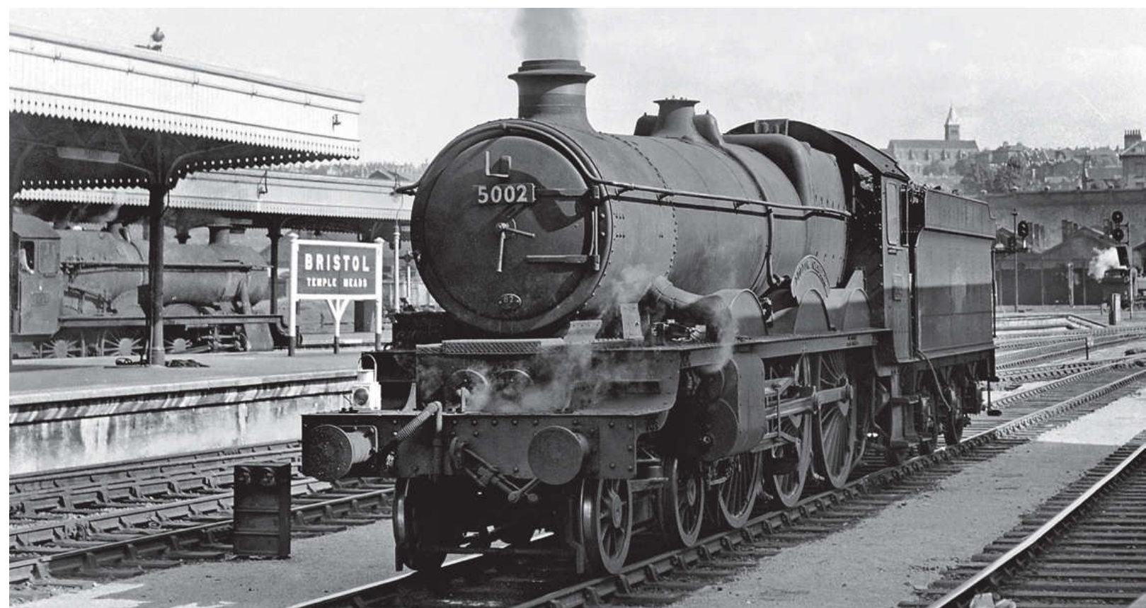
GWR 'Castle' class 4-6-0 No 5002 LUDLOW CASTLE, is seen on a through road at Bristol Temple Meads station, circa 1959. The higher central step on the inside cylinder casing is clearly visible (BR rebuild). Rail Photoprints Collection
