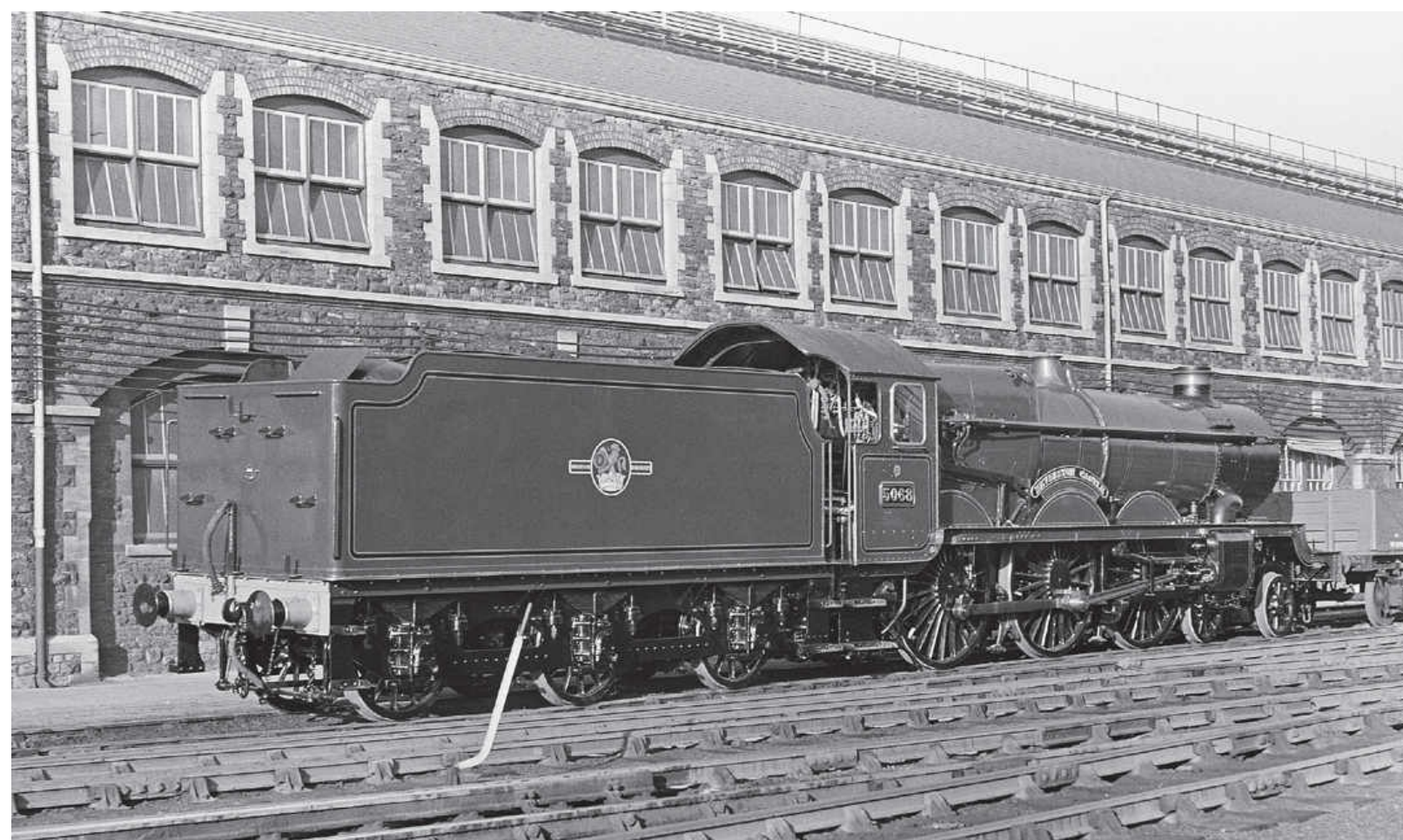
GWR 'Castle' class 4-6-0 No 5068 BEVERSTON CASTLE is seen outside the works at Swindon in February 1959 following a 'Heavy Intermediate' overhaul. Rail Photoprints Collection
