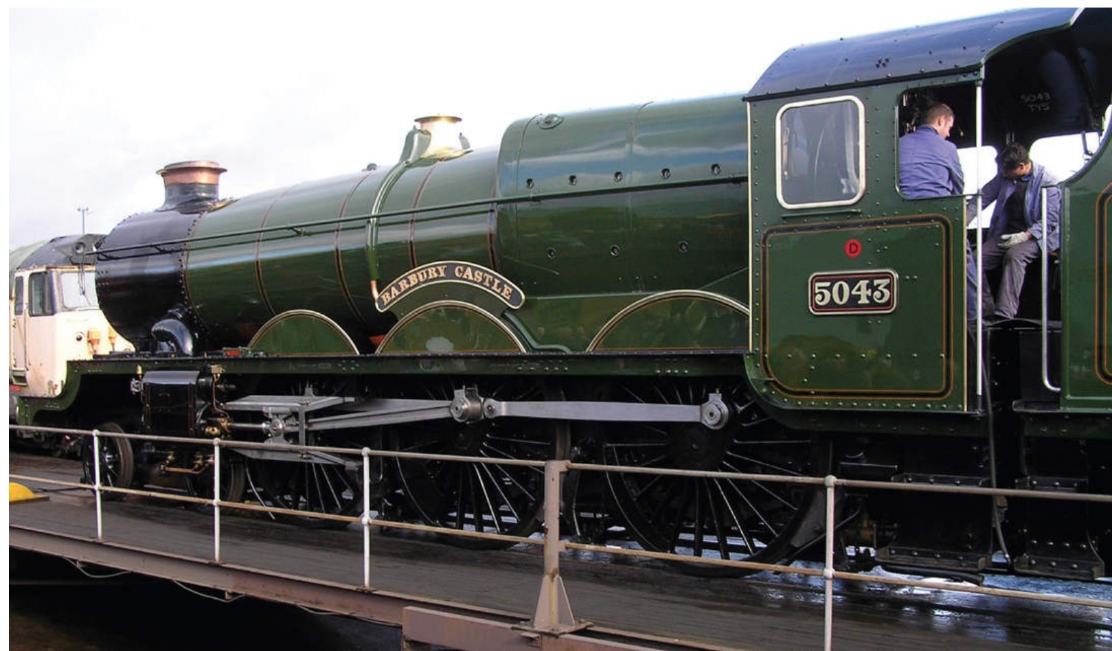
GWR 'Castle' class 4-6-0 No 5043 seen as BARBURY CASTLE the name it carried from March 1936 until renamed EARL OF MOUNT EDGCUMBE in September 1937. The engine is located on the turntable at Tyseley Locomotive Works, October 2008. Brian Wilson
