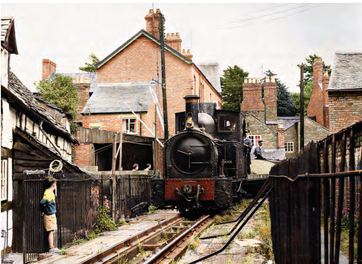
Welshpool & Llanfair narrow gauge engine 822 The Earl sneaks through the back streets of Welshpool en route to Llanfair Caereinion with an engineer's train. The 2ft 6in line was authorised after the passing of the Light Railways Act in 1896 and opened in 1903. The Earl was one of the original two 0-6-0T locomotives built by Beyer, Peacock. (Andrew Dyke collection)
