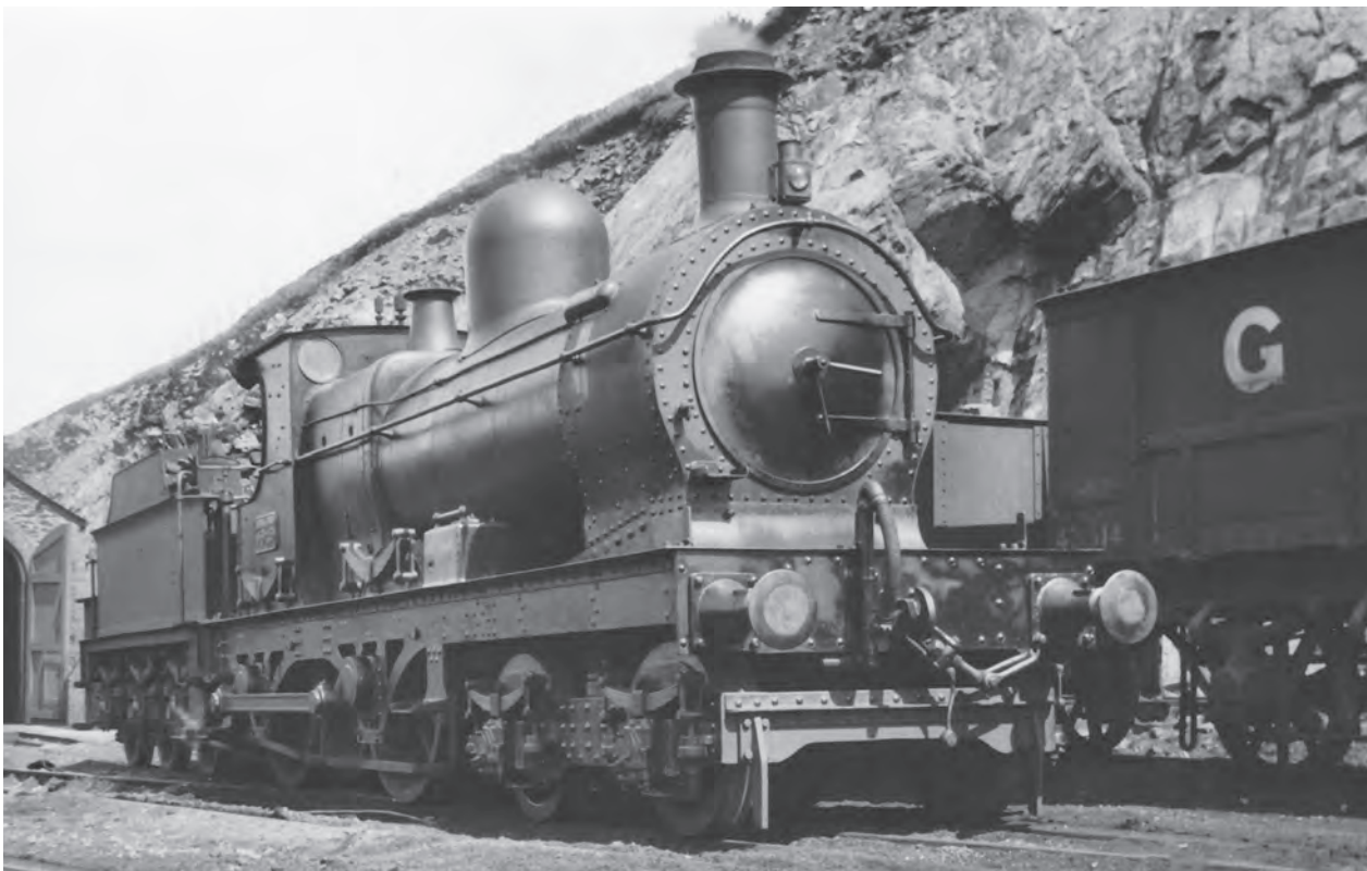
One of the class '3521' 4-4-0s rebuilt by Churchward in 1900 from Dean 0-4-4Ts built in 1888, No.3545, that was transferred to the Cambrian in 1921 as a replacement for the two Cambrian 4-4-0s destroyed in the Abermule accident. 3545 is seen here at Machynlleth, c1930. It was withdrawn in 1931 having run just under a million miles. (MLS)
