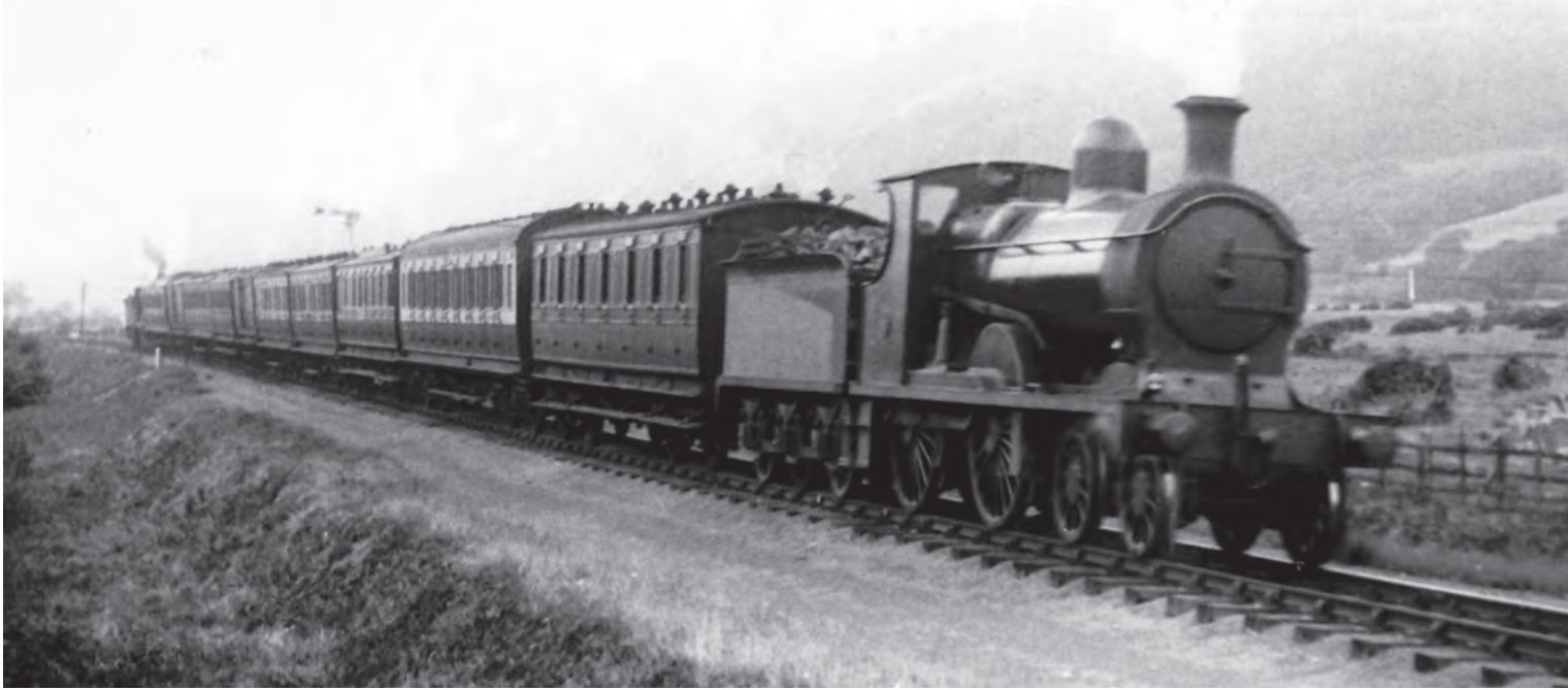
'Large Belpaire' 4-4-0 No.95 with the 9.5am express from Aberystwyth to Whitchurch on Talerddig bank, assisted in the rear to the summit by '61' class 4-4-0 'Large Bogie' No.72, 15 August 1913. The train engine (No.95) was involved in the head-on collision with '61' class No.82 in the Abermule disaster in January 1921 and both were cut up at the accident site. (MLS/R.W. Miller collection)
