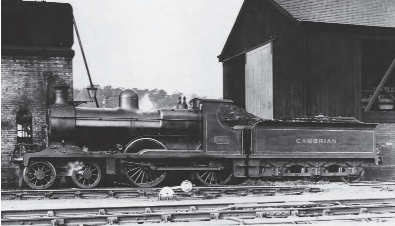
'Large Belpaire' 4-4-0 GW No.1029, formerly Cambrian Railways No.96, built in November 1904, shortly after the Cambrian's absorption by the GWR, c1923. The engine has received the new number but is still in Cambrian Railways livery. The engine, with 1014, was based at Oswestry.
