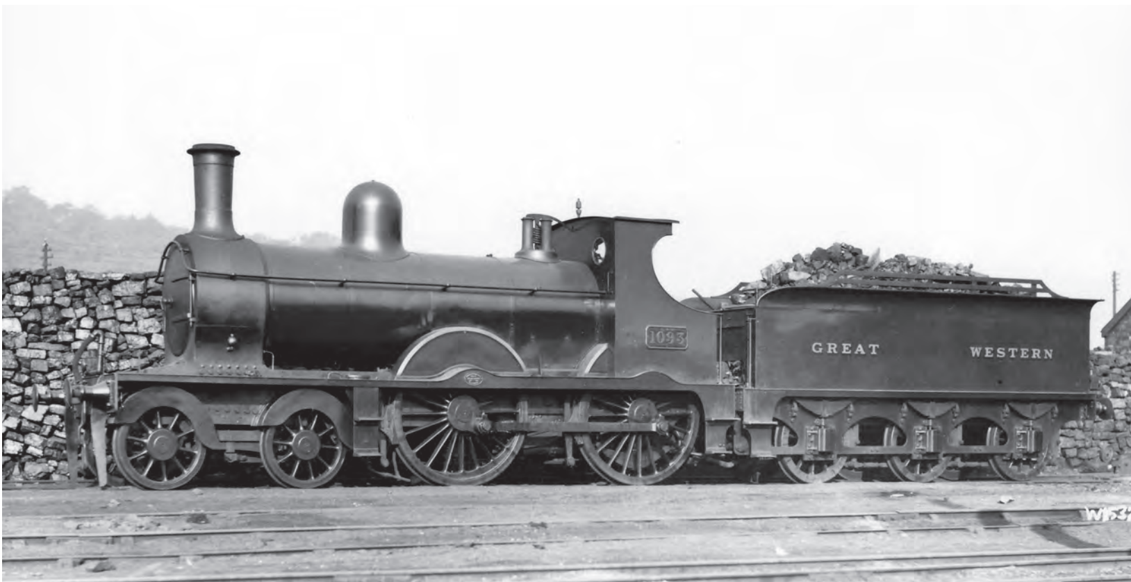
'61' class large bogie 1093 (Cambrian Railways No.64), built in 1893, just repainted after absorption by the GWR, withdrawn in April 1926, c1923.
