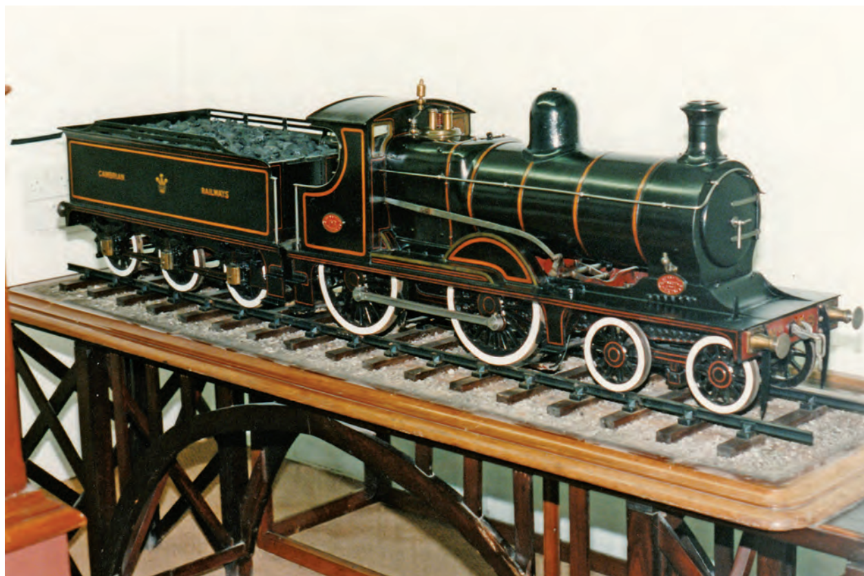
A superb model of 'Large Belpaire Passenger' No.98 in Cambrian livery, constructed at Oswestry Works in 1907 to 11½in to 1ft scale, 7¼in gauge.
