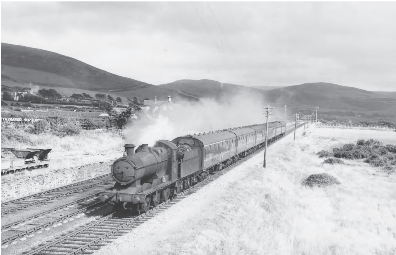
Collett 0-6-0 2236 approaching Towyn with the Pwllheli portion of the Cambrian Coast Express , 30 June 1964. By this time the train was formed of BR maroon Mark 1 rather than chocolate & cream carriages and the loco north of Machynlleth bore no headboard. The Collett 0-6-0 has been painted BR passenger lined green, but the locomotive shows signs of neglect and has lost its front numberplate. The train has even lost its express passenger headcode and is now indicated as a stopping service. (MLS)
