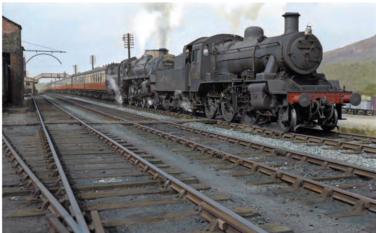
A difficult photo to date, as the BR Standard pair, 75006 4MT 4-6-0 and 78002 2MT 2-6-0, are from a later era whilst the 'plum & spilt milk' ex-GW coaches are from an earlier period. Some 'Standards' came to the Cambrian in the mid-1950s, so this photo, taken of the up Cambrian Coast Express at Machynlleth, must have been taken around 1956, before the train was earmarked for chocolate and cream rolling stock and Brunswick Green 'Manor' haulage in the late 1950s and early 1960s. (Andrew Dyke colourisation/Rail on Line)
