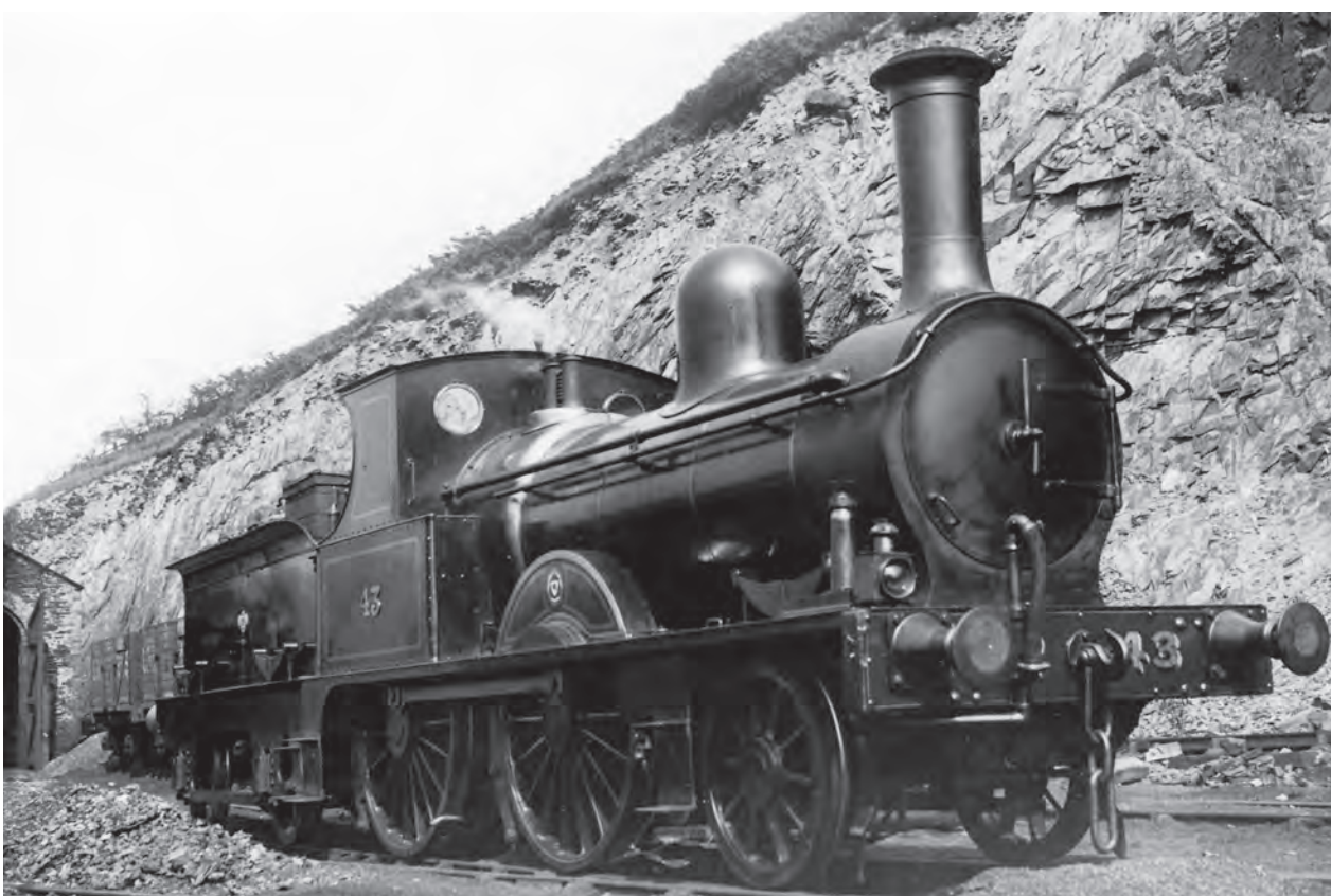
Sharp, Stewart 2-4-0 No.43, originally named Plynlimon , rebuilt by Aston in 1892, at Machynlleth shed, 2 July 1909, allocated GW No. 1331 but the number was never carried, and the engine was withdrawn in July 1922. (MLS/R.W. Miller collection)
