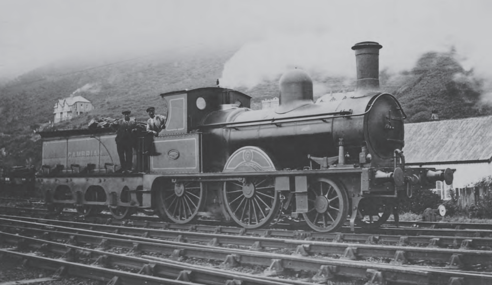
Sharp, Stewart 2-4-0, No.41, built in March 1864 for the Oswestry & Newtown Joint Committee, initially named Cader Idris but renamed Countess Vane after the Chairman's wife (name transferred from an 0-6-0 goods engine, thought inappropriate for the Chairman's wife!) seen here at Aberdovey, c1903. No.41 was reboilered in 1893 and name removed, allocated to 'surplus stock' in 1906, but then survived to be taken over by the GWR though never receiving its allocated new number, 1330, being condemned in July 1922.
