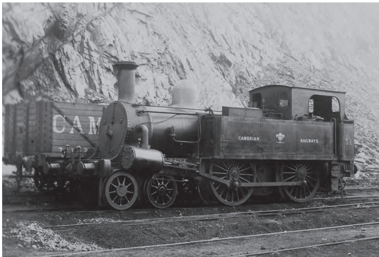
Cambrian Railways No.34, formerly Metropolitan Railway No.13, at Machynlleth where it was based until rebuilding in 1915, when it was one of two former Met tanks rebuilt as a 4-4-0. It was one of five former Beyer, Peacock 4-4-0Ts, built in 1864, and purchased by the Cambrian in November 1905 at the bargain price of £500 after they were made redundant on the Metropolitan Railway by electrification. Their condensing gear was removed, and this locomotive was based at Machynlleth performing local passenger work to Aberystwyth and Barmouth.
