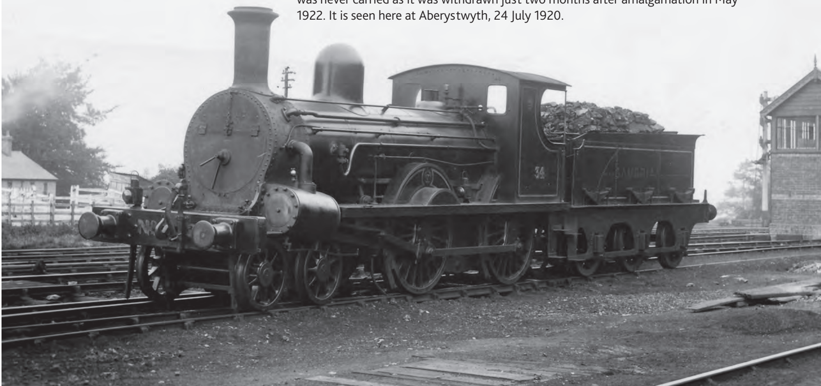
'Small Bogie' No.21 built in July 1886 to the Sharp, Stewart 1878 design (see photo of the prototype No.16 Beaconsfield earlier, page 25), poses after reboiling at Oswestry in October 1910.
