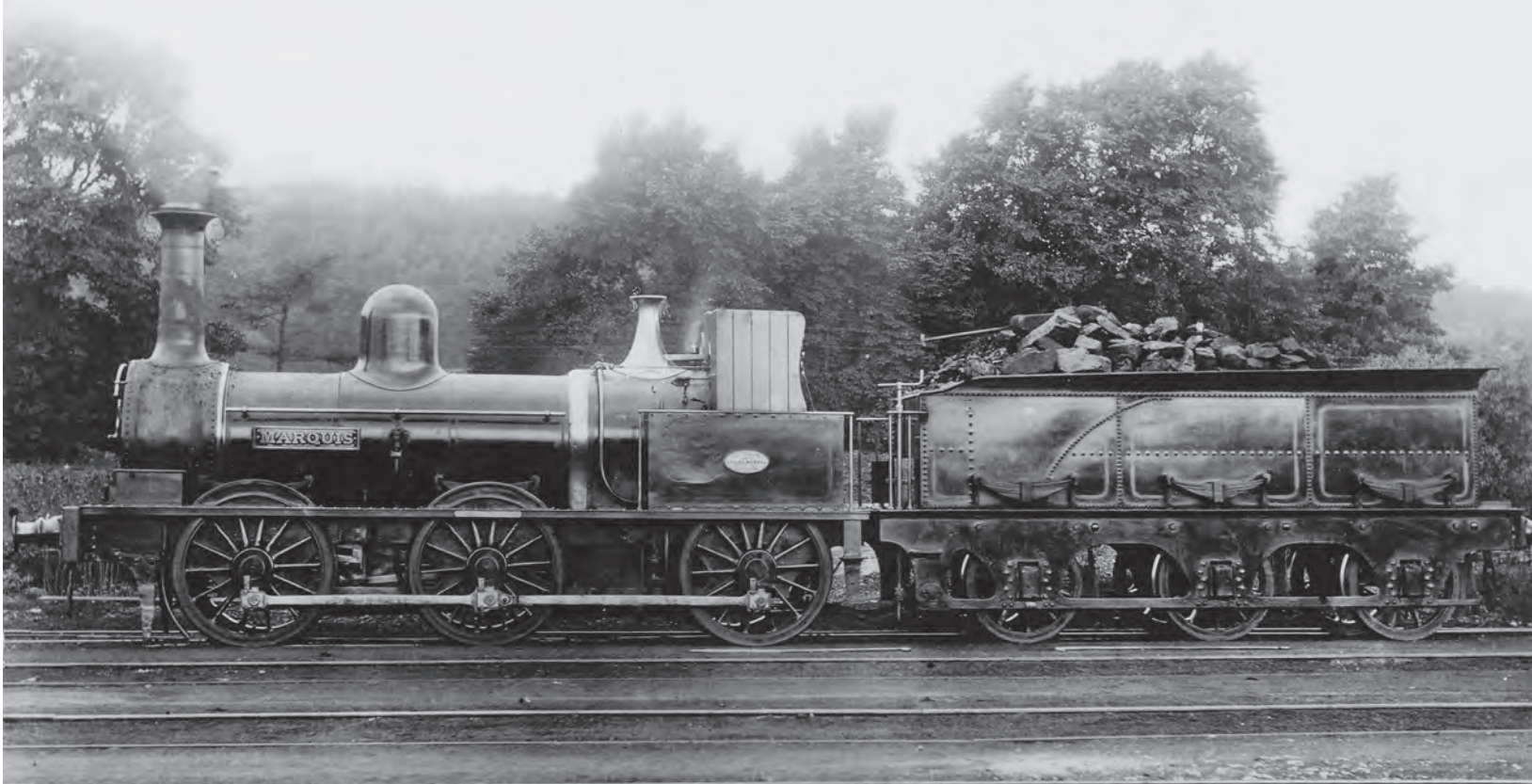
'Small Goods' Sharp, Stewart 0-6-0 No.6 Marquis at Oswestry, March 1889, before rebuilding (in 1895) and losing its name. No.6 was built in July 1873.
