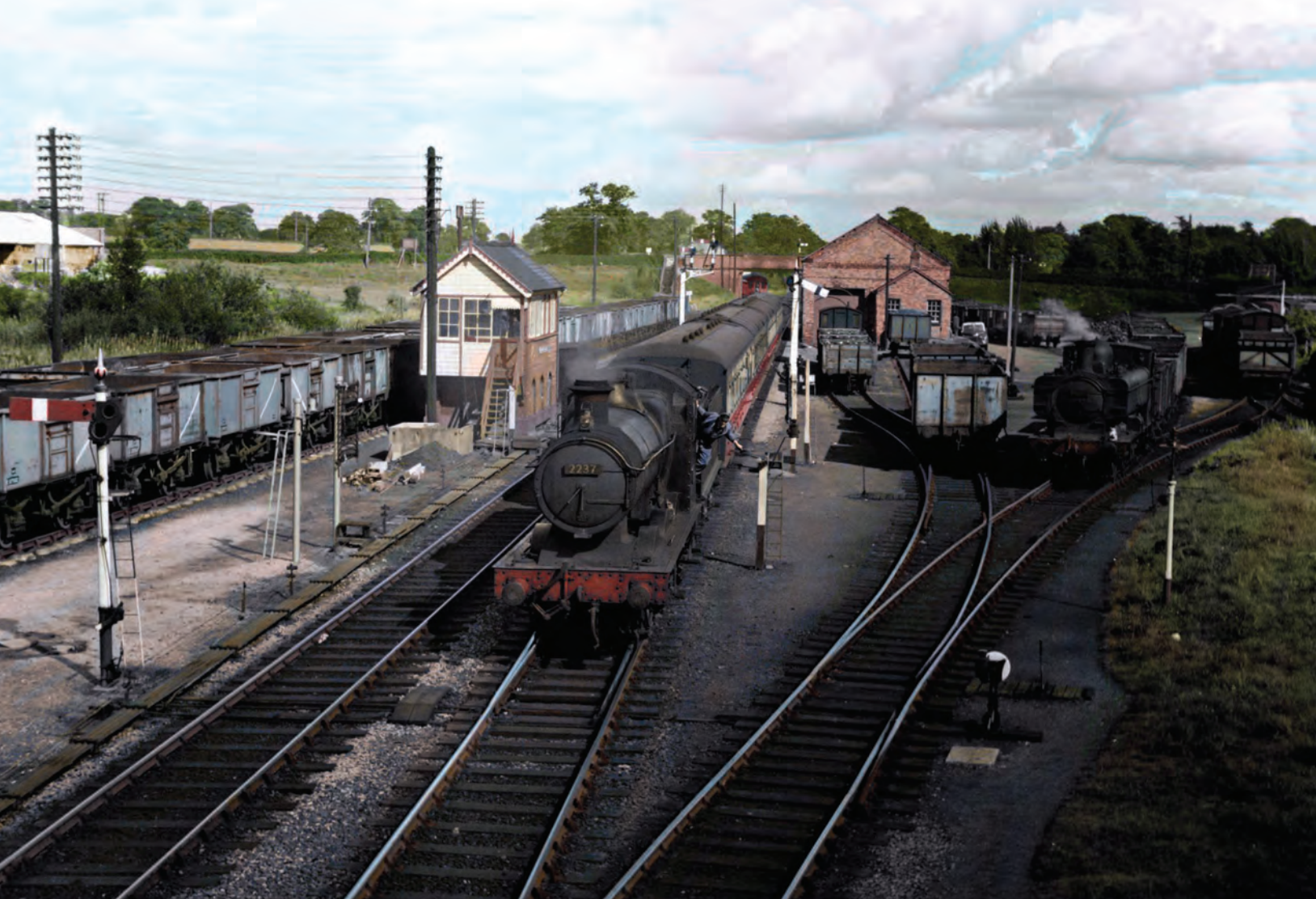
Collett 0-6-0 No.2237 arrives at Ellesmere with an early afternoon Whitchurch- Oswestry train, the fireman collecting the token for the next section, while a GW 57XX pannier tank shunts the goods yard before continuing with its pick-up goods train. (Andrew Dyke colourisation/ Rail on Line)
