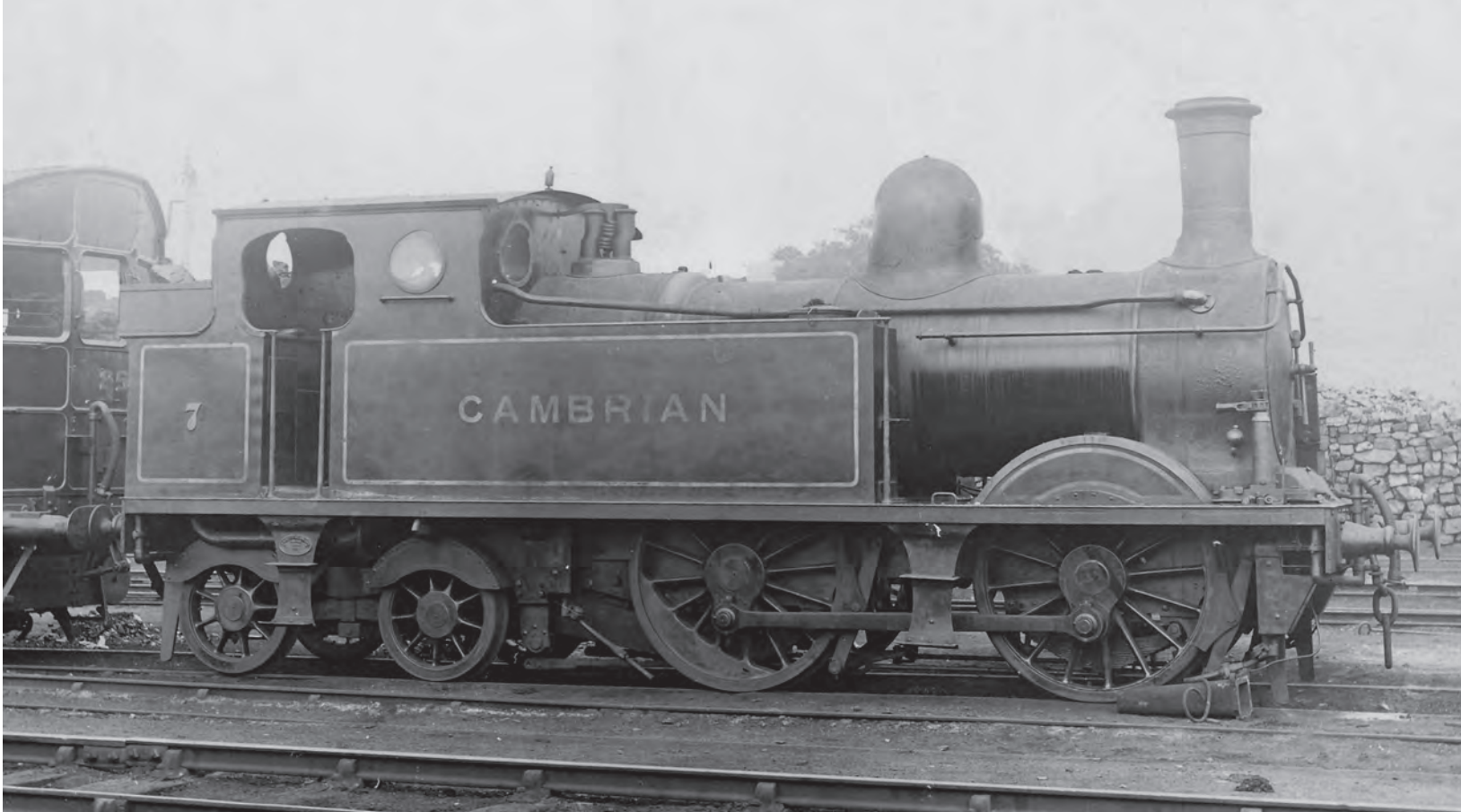
Cambrian 0-4-4T No.7, built in 1895 for the Wrexham-Ellesmere branch. It also worked the Llanfyllin branch and at one stage operated over the Llanidloes Mid-Wales line during alterations to the turntable there. It was sent to Swindon for repair in September 1922 but was found to be in poor condition and was condemned. It is seen here, with rail motor trailer No.25, at Oswestry, c1910.
