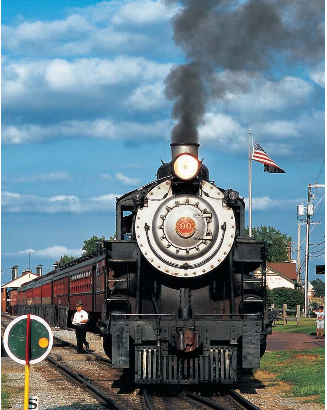
No. 90 has just arrived at the East Strasburg, Pennsylvania, station. This handsome Decapod type was built by Baldwin in 1924 for the Great Western Railway in Loveland, Colorado. In its day as a freight hauler, it moved train loads of sugar beets. It has operated on the Strasburg since 1967. Brian Solomon
