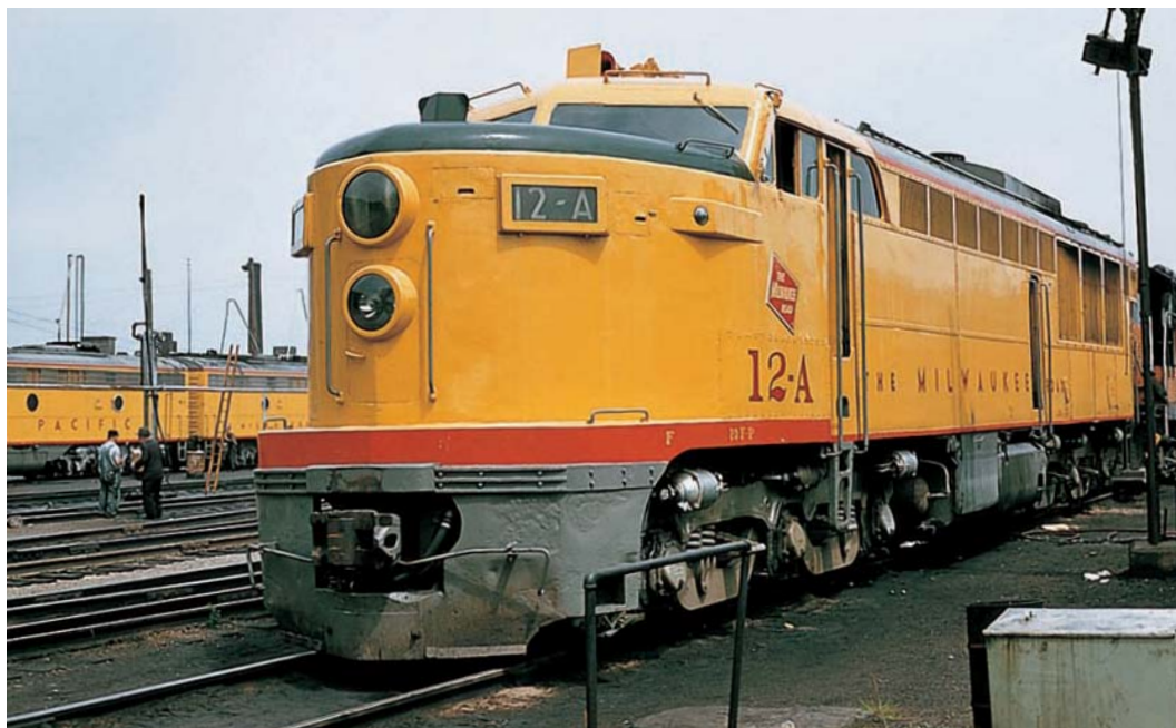
Milwaukee Road ordered 15 powerful Fairbanks-Morse “Erie-built” for service on its Olympian Hiawatha . They were assembled at GE’s Erie, Pennsylvania, plant between December 1945 and March 1947, and they originally were adorned with an attractive stainless-steel styling on the nose. All the Erie-built locomotives rode on A1A trucks and were powered by Fairbanks-Morse’s 2,000-horsepower 10-cylinder opposed-piston diesel. No. 12A is shown at Chicago’s Western Avenue Yard on July 17, 1958. Richard Jay Solomon
