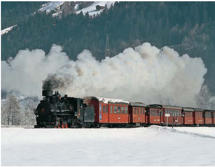
Left: No. 4 works in an Alpine setting on its run up to Mayrhofen, Austria. Built by Krauss at Linz, Austria, in 1909, this locomotive worked for years on the Yugoslavian Railways (JZ) as No. JZ-83-076. It is considered a Class 83 and weighs 36 metric tons. Brian Solomon
