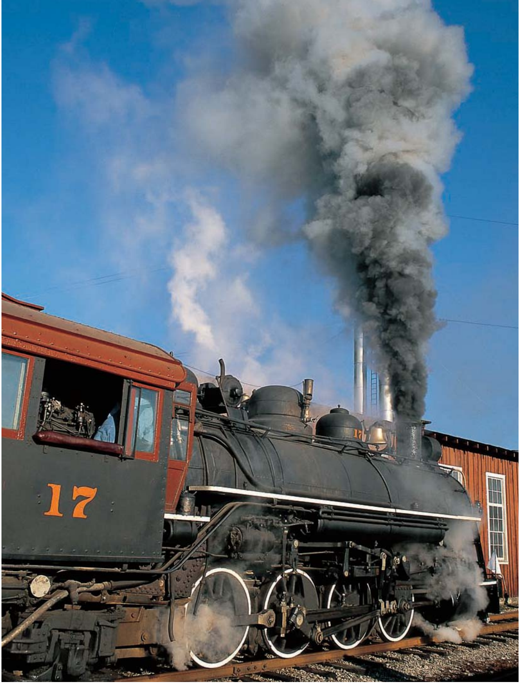
East Broad Top No. 17 is one of the only surviving locomotives in the United States equipped with the unusual Southern valve-gear arrangement. Brian Solomon
