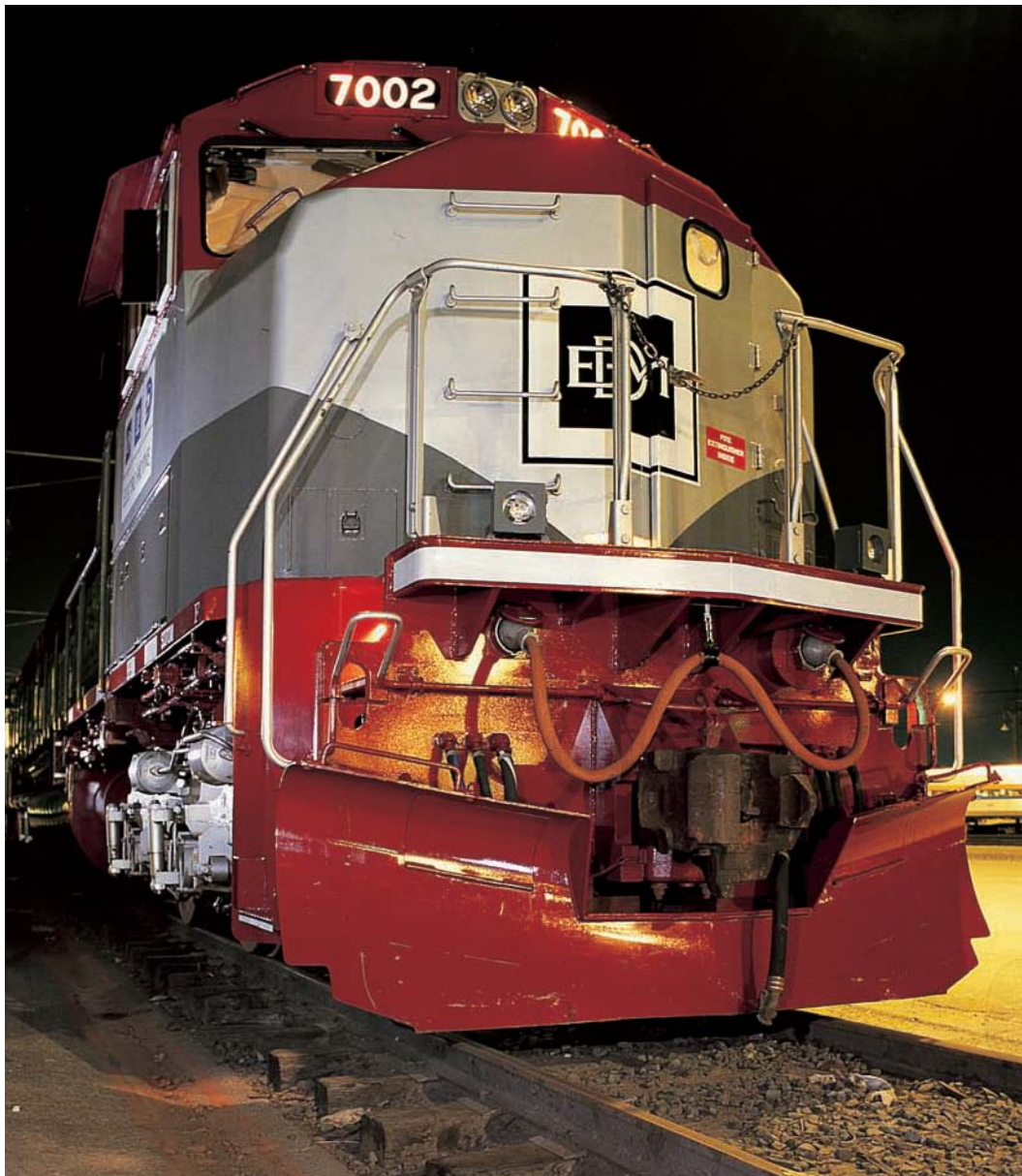
SD70M demonstrators made their rounds on Southern Pacific in June 1993, painted in EMD's latest demonstrator scheme. The primary difference between the SD70M and the SD70 was the cab style. Brian Solomon
