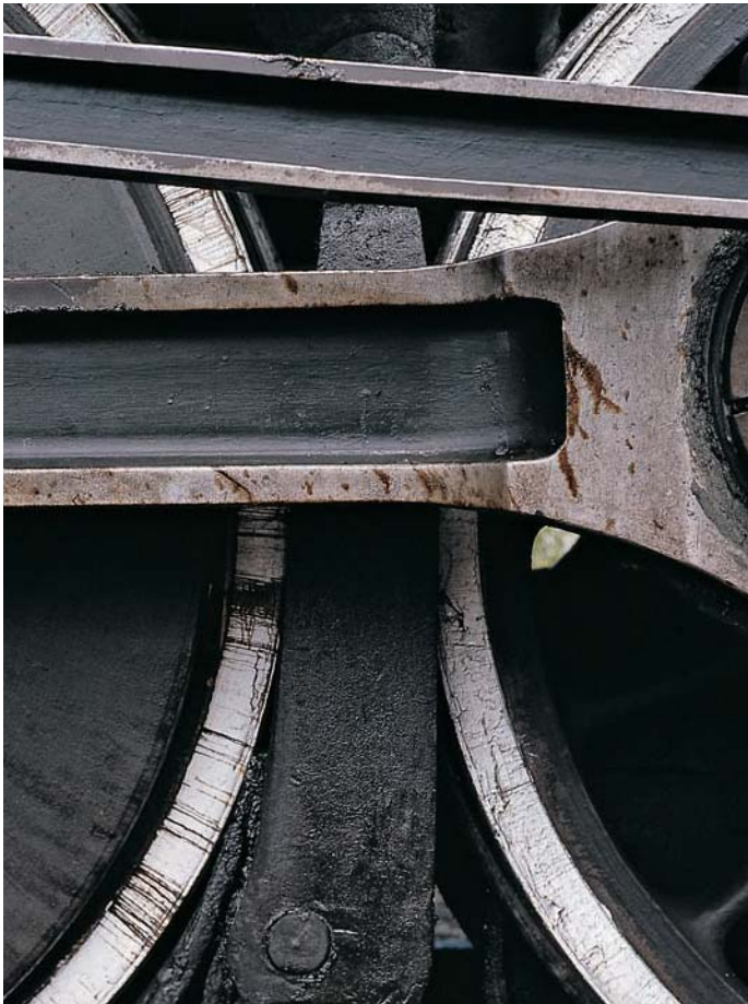
The first Berkshires that served the Boston & Albany were mountain climbers equipped with driving wheels measuring 63 inches in diameter. By contrast, the Nickel Plate's Berkshires were built for speed and featured 69-inch driving wheels. Brian Solomon
