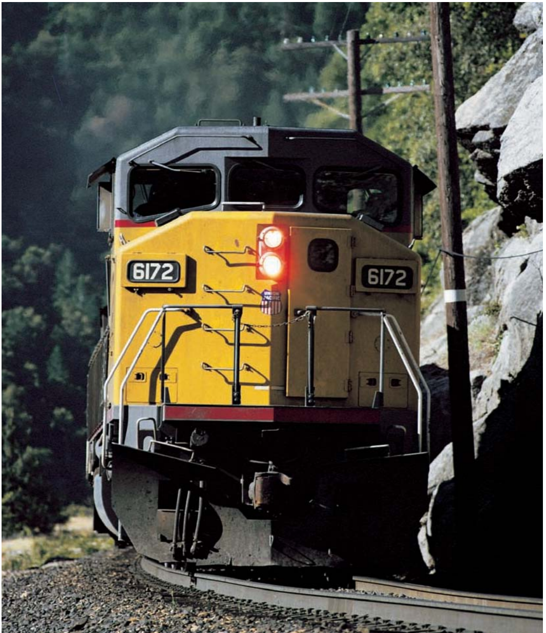
On May 22, 1993, UP SD60M No. 6172 works eastward through the Feather River Canyon on the former Western Pacific main line. Known in some circles as "Cyclops" for their distinctive appearance, SD60Ms were commonly assigned to lead UP freights on this route in the early 1990s. Brian Solomon
