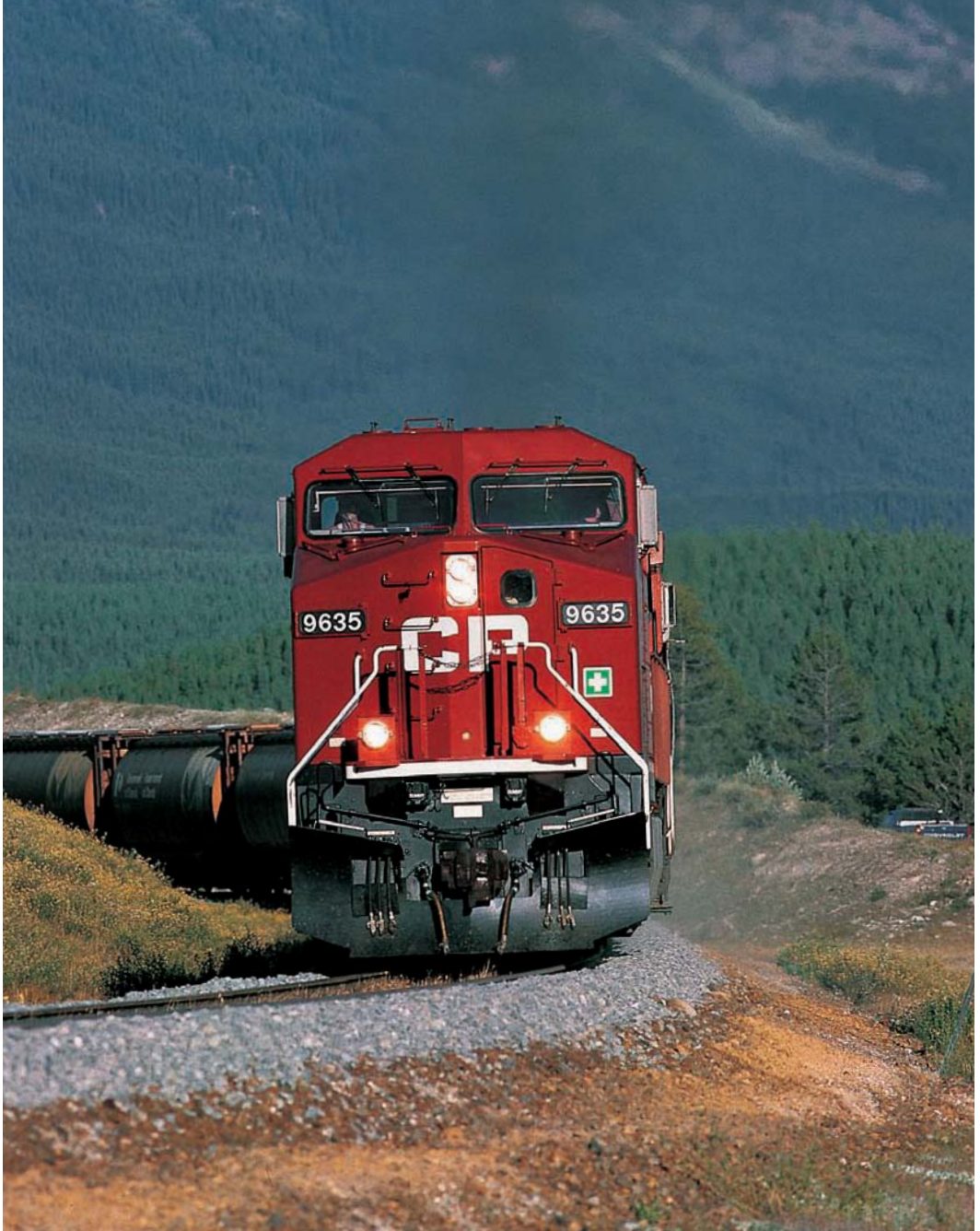
CP Rail AC4400CW No. 9635 works west with a loaded grain train near Lake Louise, Alberta, in August 1998. This is the typical power setup for CP Rail bulk trains operating in western Canada: two AC-traction locomotives on the head end and a third positioned approximately two-thirds back in the train. Chris Guss
