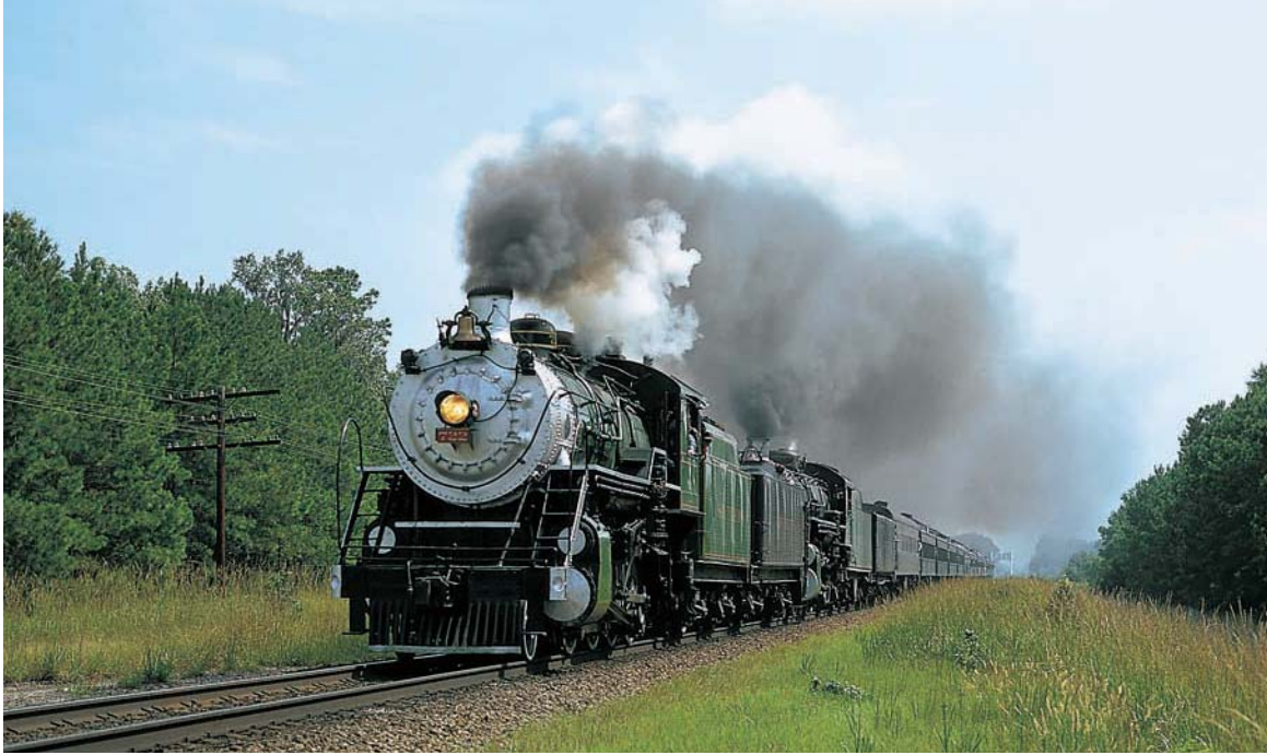
Above: Baldwin built Southern No. 4501 in 1911. The Southern's Ms-class ("s" for "superheating") Mikados were handsome, nicely proportioned, and powerful locomotives but otherwise unremarkable in their day. The Southern revived No. 4501 and made it a star of its steam program, where it entertained tens of thousands of people in two decades of main-line excursions. Working the Seaboard Coast Line rails in 1970, No. 4501 heads southward at Yemassee, South Carolina. George W. Kowanski
