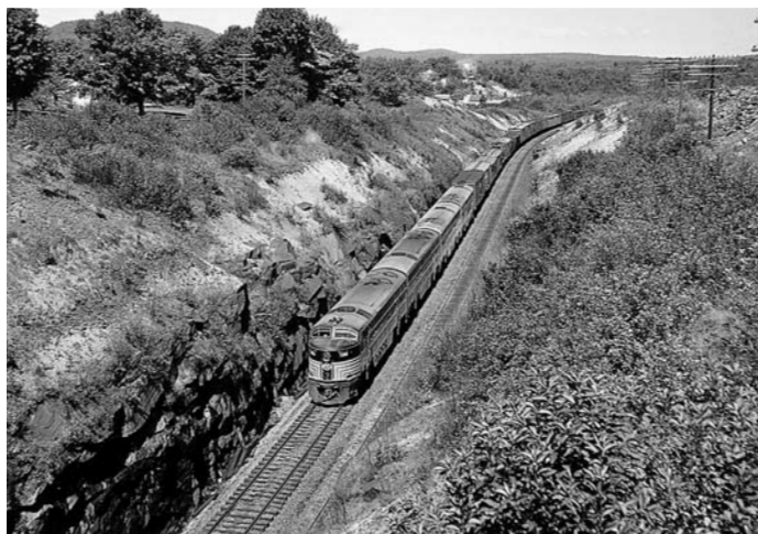
An A-B-B-A set of New York Central's Fairbanks-Morse CFA-20-4 C-Liners roar eastbound through the deep cut east of Washington Station, Massachusetts, on the old Boston & Albany route on August 22, 1954. Leading is No. 5004. The Central bought several C-Liner models in the early 1950s, but the locomotives remained relatively obscure among the hoards of Electro-Motives and Alcos. Robert A. Buck
