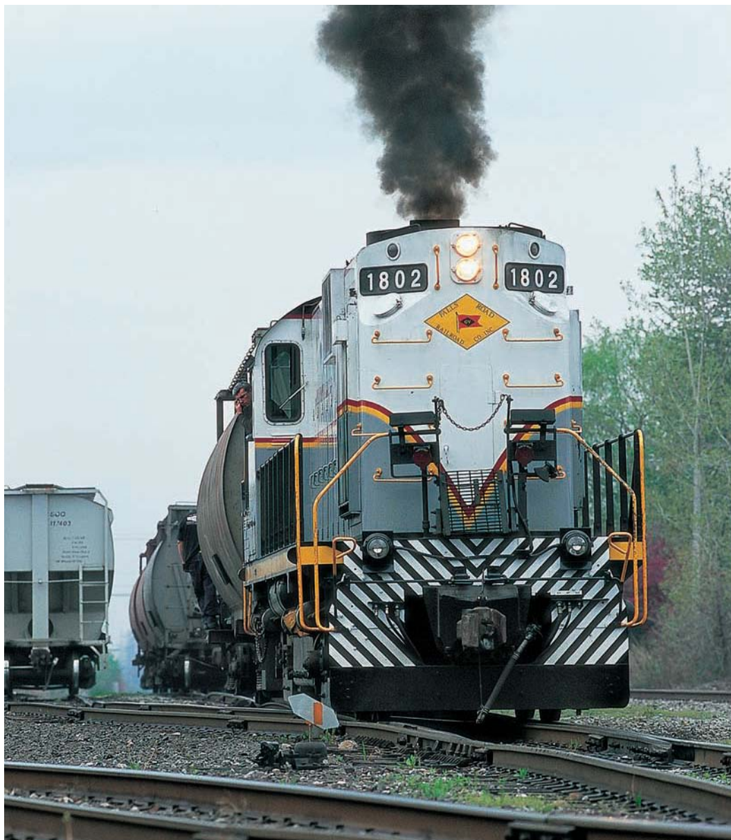
Falls Road Railroad Alco RS-11 No. 1802 is a former Nickel Plate Road locomotive and one of several RS-11s operated by parent company Genesee Valley Transportation. The RS-11 is powered by a 1,800-horsepower 251 diesel engine. Brian Solomon
