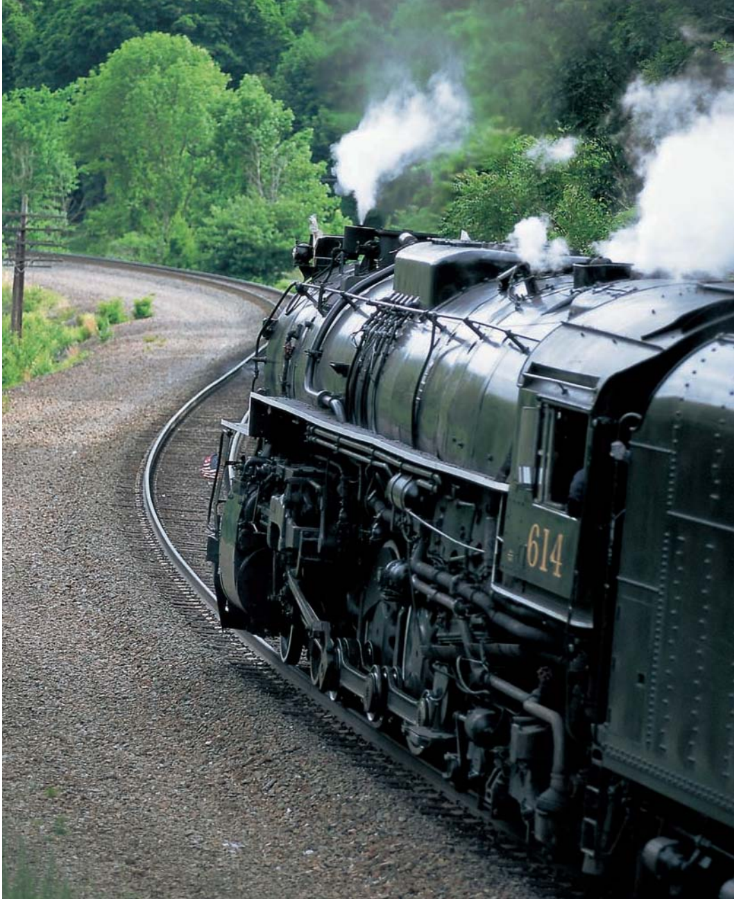
Chesapeake & Ohio No. 614 works east on the former Erie main line at S curves near Tuxedo, New York. This magnificent machine was one of five that Lima built for the coal-hauling C&O in 1948. On the C&O, 4-8-4s were known as Greenbriers, named for the Greenbrier River. Where some railroads ordered 4-8-4s for freight, the C&O's were designed for heavy passenger service. Brian Solomon
