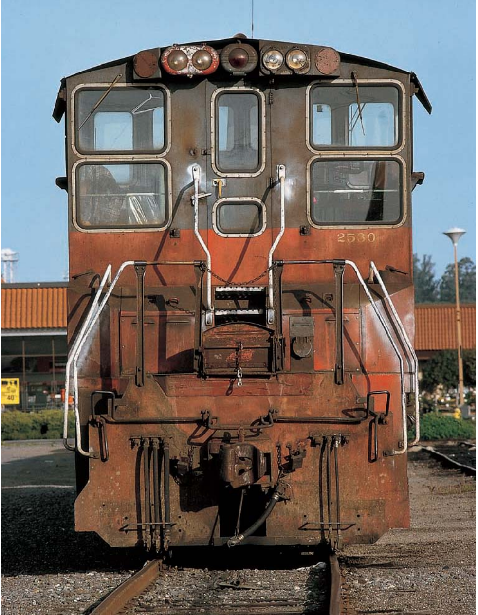
Southern Pacific was famous for its "full-house" lighting on diesel-electric locomotives. SP SW1500 No. 2530 features laterally mounted headlights (right), red oscillating lights on either side of the cab door, and a red warning oscillating light above the door. The red oscillating light would only be actuated in the event of a sudden loss of air-pipe pressure caused by an emergency airbrake application and was intended to warn other train crews that the train was in trouble and potentially derailed. Brian Solomon
