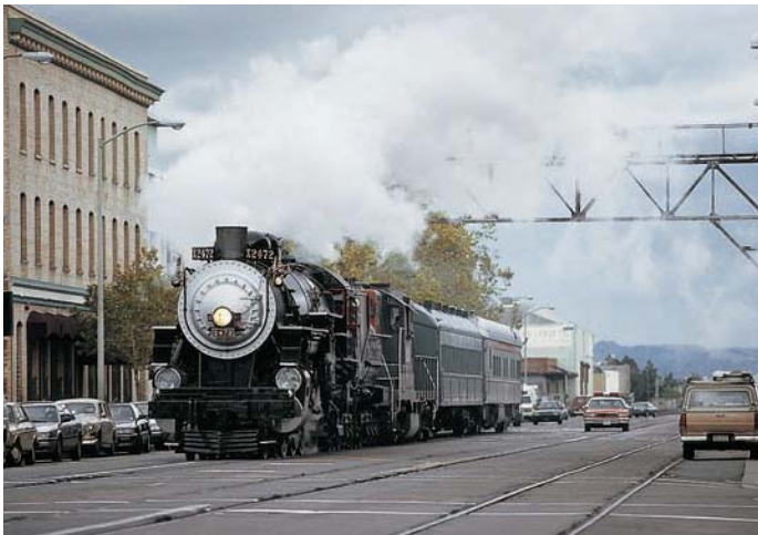
Above: In August 1992, restored No. 2472 leads an eastward excursion on the Coast Line near Harlem, California. This handsome locomotive has thrilled thousands in excursion service since 1991 and is one of a few active Pacific types in the United States. Brian Solomon
