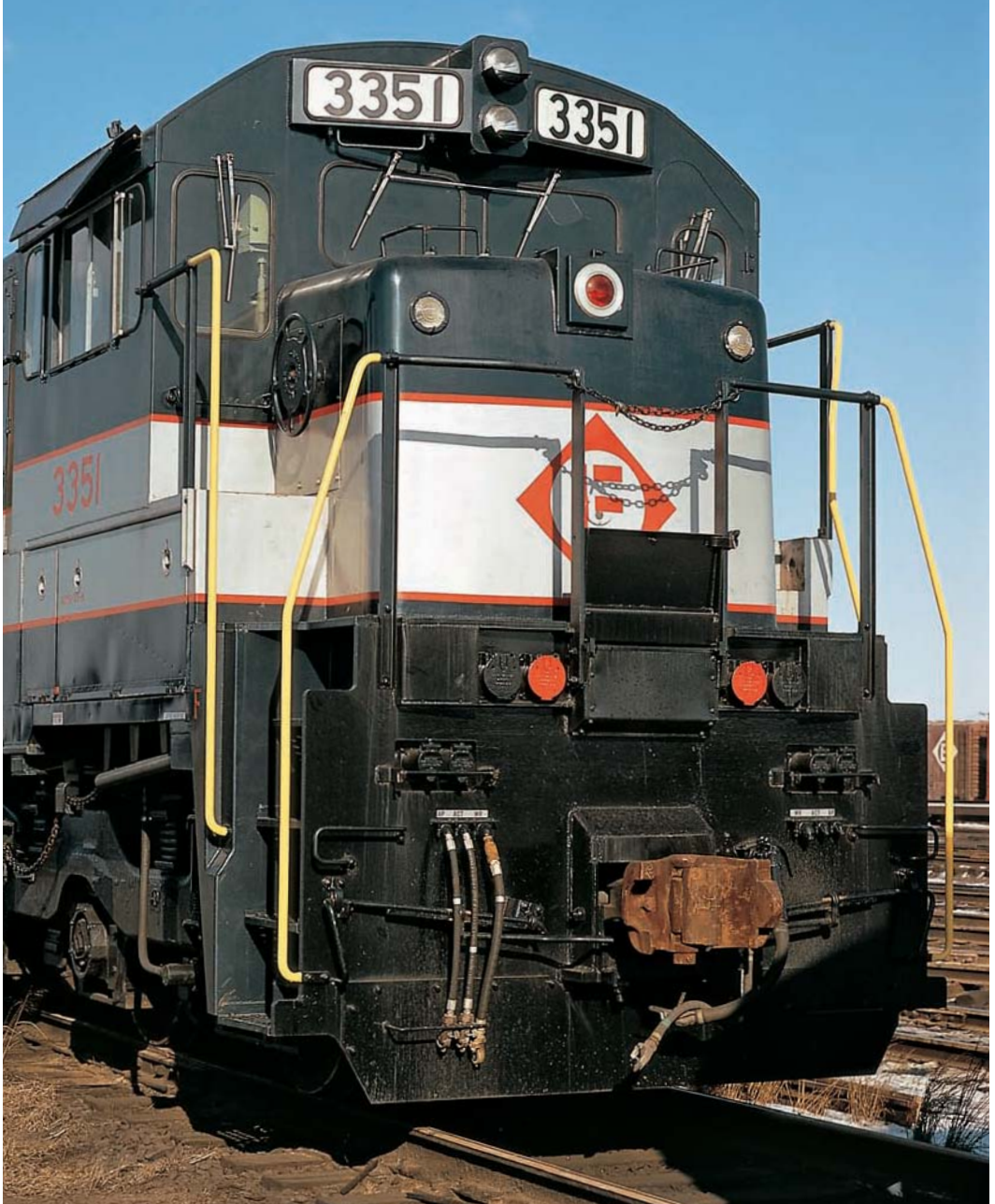
Erie Lackawanna's 32 U34CH diesels were paid for by the New Jersey Department of Transportation and thus wore an unusual variation of the EL livery. These locomotives ultimately served NJ Transit, which assumed operations of commuter rail lines in the state in the early 1980s. The U34CH was a variation of the U36C with head-end power provisions for passenger-car heating and lighting. George W. Kowanski
