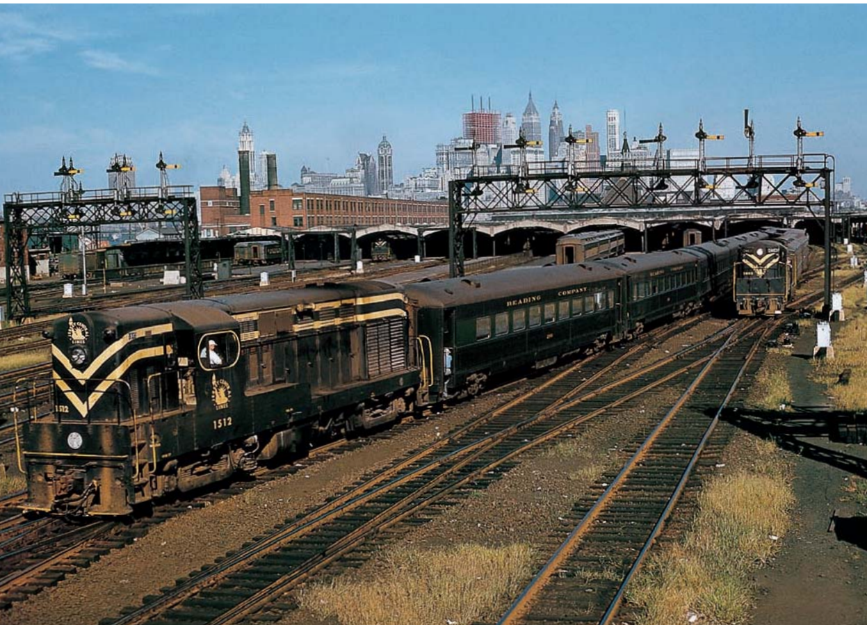
Fairbanks-Morse locomotives abound in this classic photo at Jersey City on the afternoon of August 25, 1959. On the left, Central Railroad of New Jersey H-15-44 No. 1512 switches a Reading Company train, while an H-24-66 Train-Master roars out of CNJ's terminal station with a commuter train. Another F-M can be seen lurking under the train shed. Richard Jay Solomon
