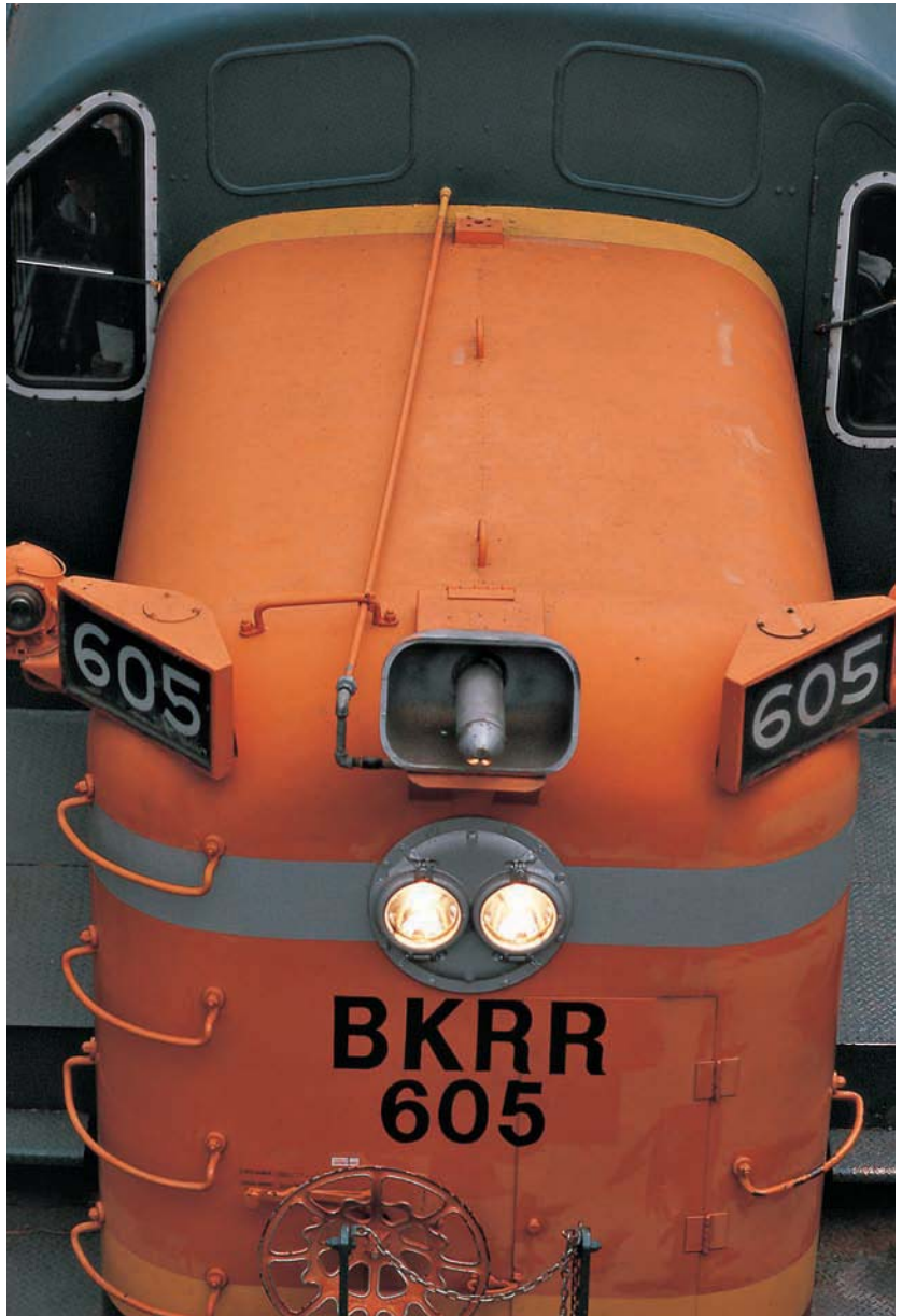
A detail of the short hood on No. 605 shows the classic Hancock air whistle and twin sealed-beam headlight. In 2010, this was among the last as-built RS-3s in revenue freight service in North America. More than 1,750 RS-2s and RS-3s were built, but today only a handful survives outside of museums. Brian Solomon
