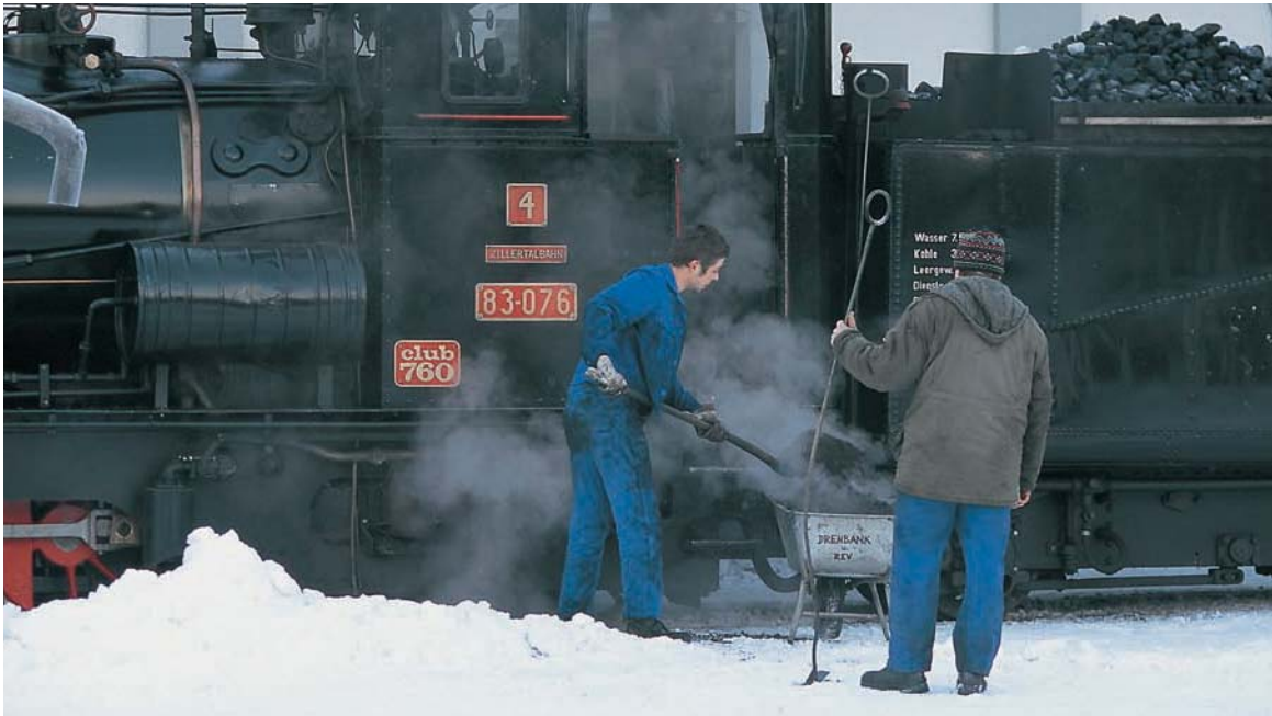
Above: The Zillertalbahn crew prepares No. 4 at Jenbach on an abnormally cold January 2006 morning. This 0-8-2 type was typical of narrow gauge locomotives built for railways of the old Austrian-Hungarian Empire in the early years of the twentieth century. War and politics found the locomotive operating in the newly created Yugoslavia after 1918. Brian Solomon
