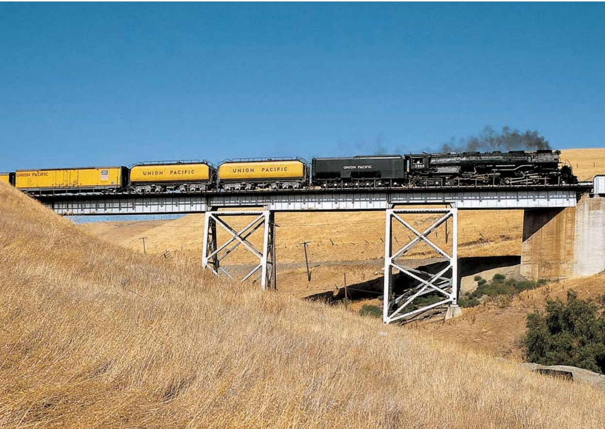
Union Pacific No. 3985 leads an excursion to San Jose over Altamont Pass in 1992. The UP's 4-6-6-4 Challengers were among the most successful high-speed articulated types, combining the benefits of a four-wheel leading truck and tall driving wheels with contemporary innovations for better stability at higher speeds. Brian Solomon
