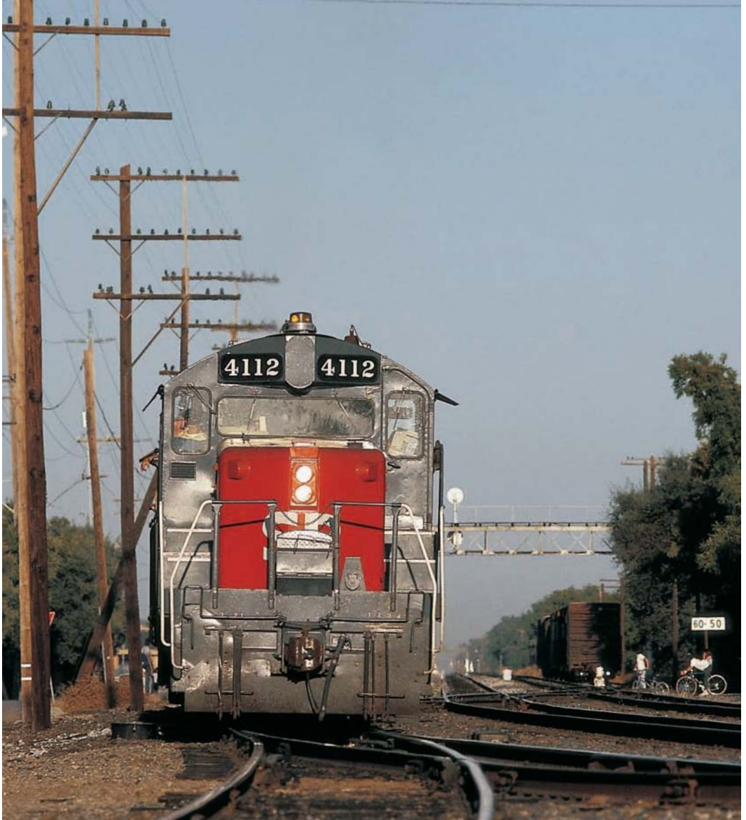
Southern Pacific GP20E No. 4112 leads the Woodland turn at Davis, California, in October 1989. The GP20 was Electro-Motive's early effort at producing a high-output four-motor road switcher, but it was known for turbocharger difficulties. Southern Pacific extended the life of its GP20 fleet by replacing the turbocharger with a more reliable method of engine aspiration. Brian Solomon
