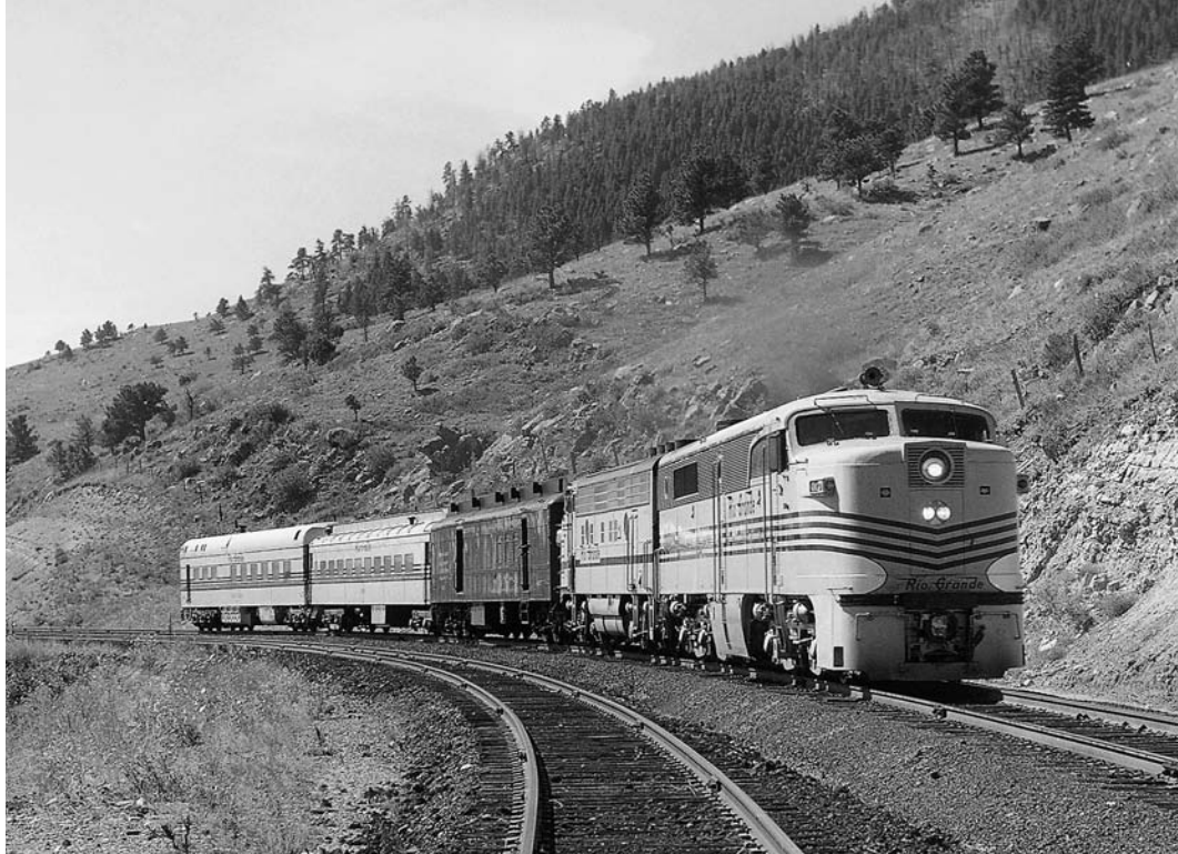
An Alco PA and EMD F7A work upgrade in the Colorado Front Range with Rio Grande's Yampa Valley Mail in 1963. Although PAs and Fs would have rarely worked together on most railroads, such combinations were not uncommon on the Rio Grande. Jim Shaughnessy
