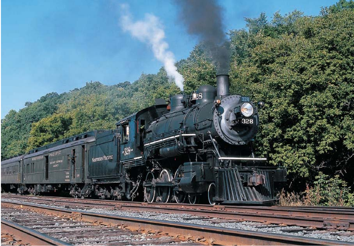
Above: The Ten-Wheeler type was first built in the 1840s but gained in popularity after the 1860s. Long after the perfection of larger types, this wheel arrangement continued to be built as a dual-service locomotive. Northern Pacific No. 328, built in 1905, is a classic example of a versatile early twentieth-century locomotive. Brian Solomon
