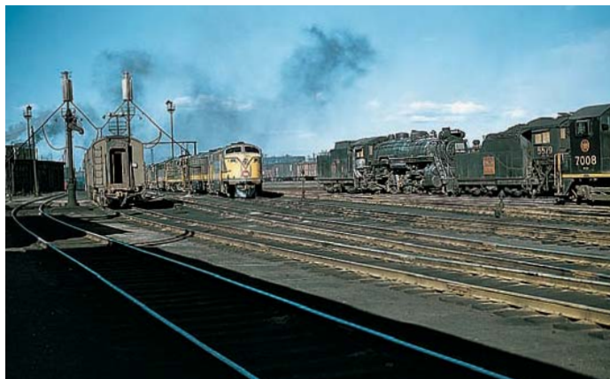
Milwaukee Road ordered 15 powerful Fairbanks-Morse “Erie-built” for service on its Olympian Hiawatha . They were assembled at GE’s Erie, Pennsylvania, plant between December 1945 and March 1947, and they originally were adorned with an attractive stainless-steel styling on the nose. All the Erie-built locomotives rode on A1A trucks and were powered by Fairbanks-Morse’s 2,000-horsepower 10-cylinder opposed-piston diesel. No. 12A is shown at Chicago’s Western Avenue Yard on July 17, 1958. Richard Jay Solomon
