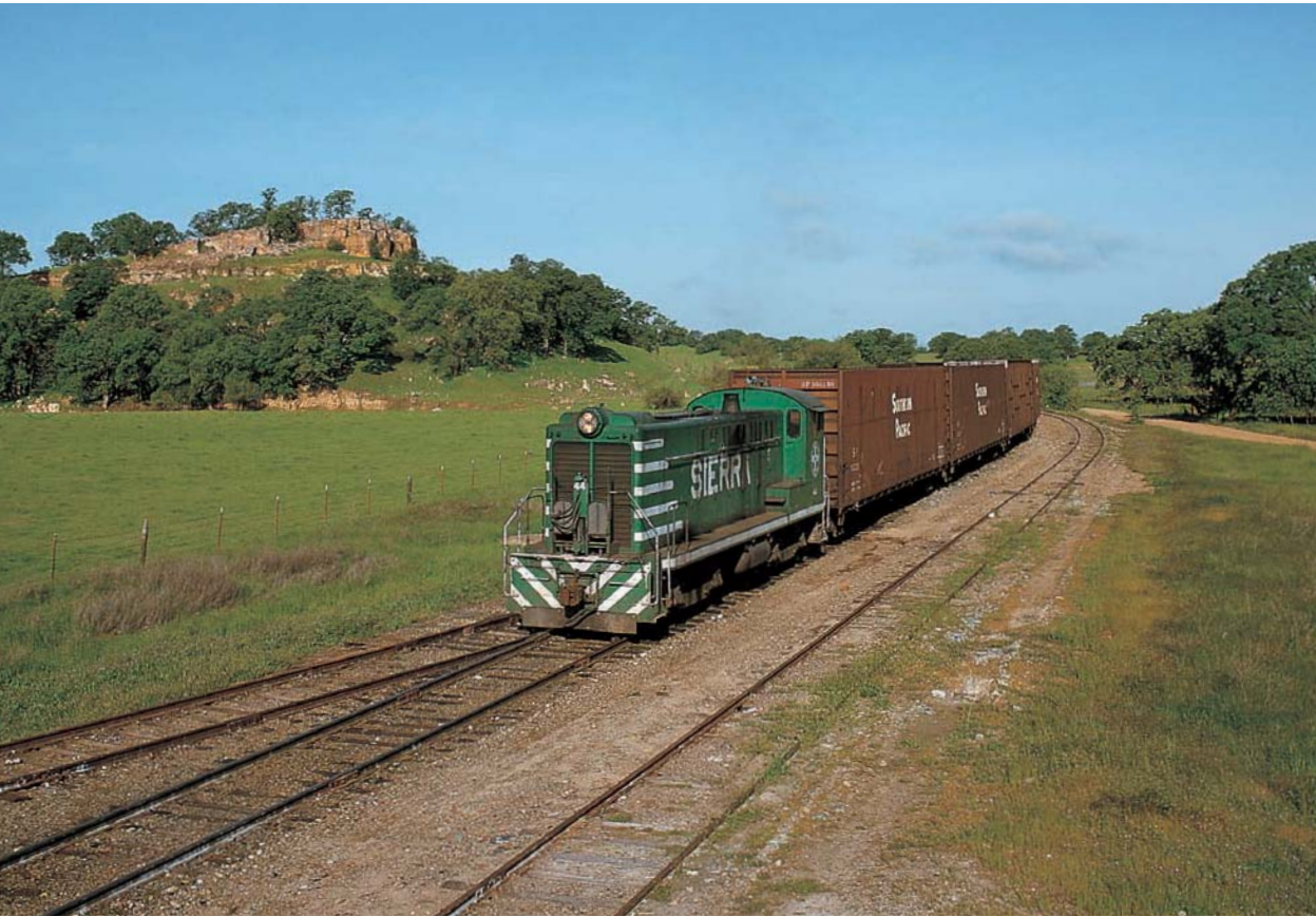
Sierra Railroad S-12 No. 44 works east of Oakdale, California, at Cooperstown on April 3, 1993. Although Sierra bought some of its Baldwin diesels new, this locomotive came secondhand from Sharon Steel. Sierra is one of a few railroads that continue to operate Baldwins in freight service decades after Baldwin exited the business. Brian Solomon
