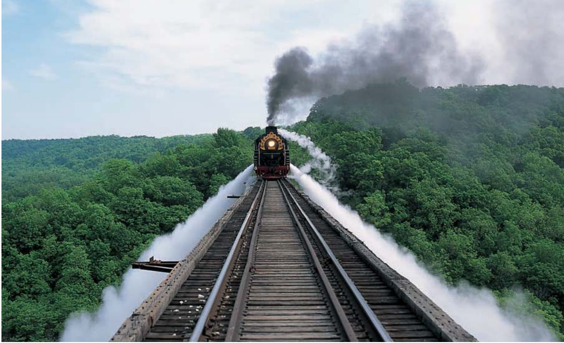
Above: Boone & Scenic Valley No. JS8419 undergoes its routine morning blow-down procedure on the high trestle west of Boone, Iowa. Blow down is necessary to remove mineral accumulation in the boiler. In the summer, the Boone & Scenic Valley runs weekend trips with the locomotive on its former interurban trackage along the Des Moines River in central Iowa. Brian Solomon
