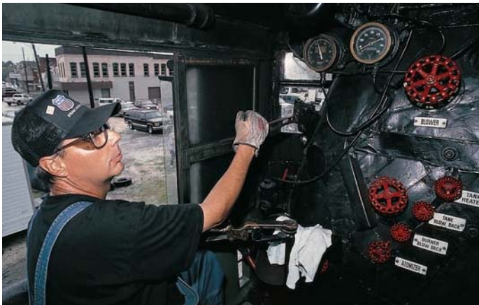
Left: Fireman Rick Braunschweig has his hand on the injector lever and his eye on the sight glass as water fills No. 3985's enormous boiler at Trinity, Texas, in June 2004. Tom Kline
