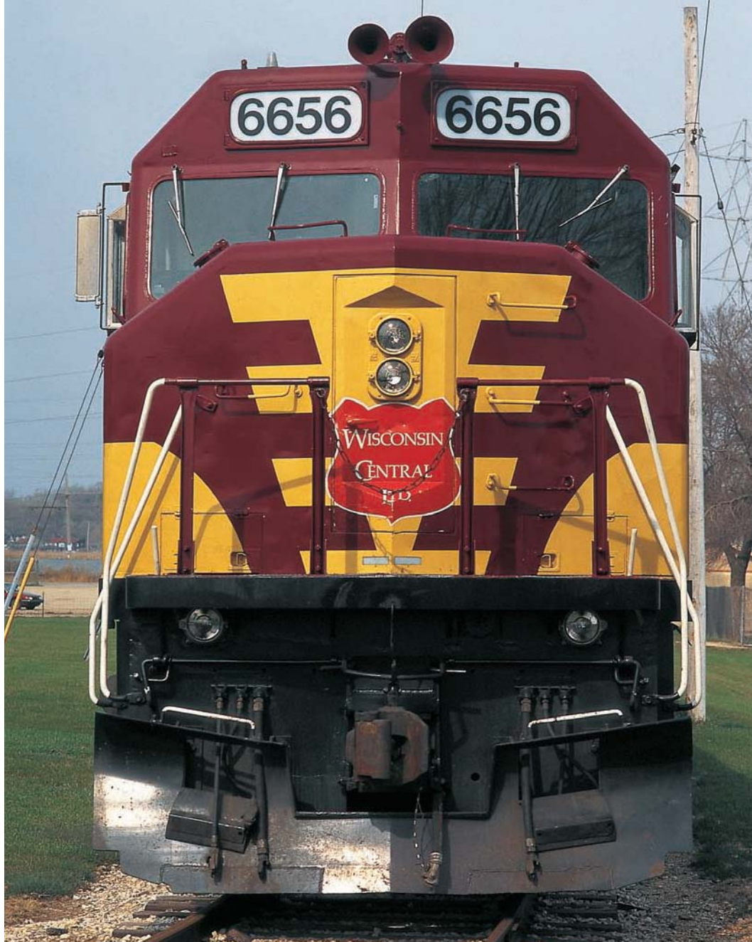
On May 4, 1996, Wisconsin Central F45 No. 6656 was displayed for public viewing on the East Troy Electric at Mukwonago, Wisconsin. Wisconsin Central—along with Montana Rail Link; New York, Susquehanna & Western; and Wisconsin & Southern—operated F45s acquired secondhand after Electro-Motive's 20-cylinder 645E3 prime mover had largely fallen out of favor on the larger railroads. Brian Solomon
