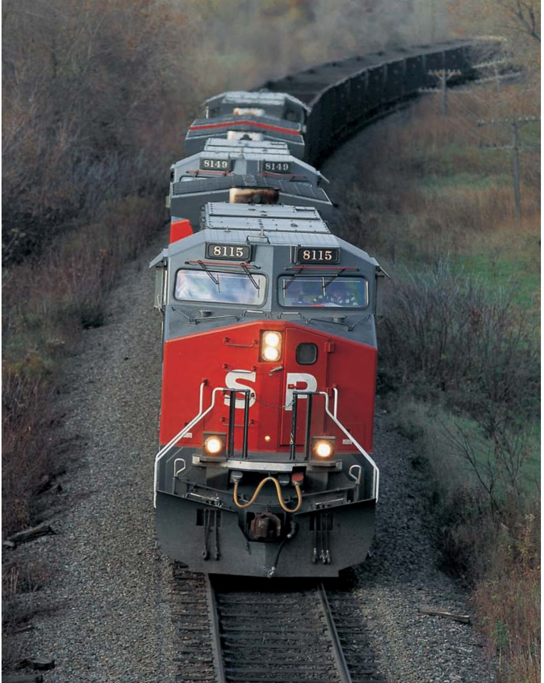
In 1994, Southern Pacific ordered Dash 9-44CWs that were assigned to a variety of heavy services, including iron ore trains operating from Minnesota's Iron Range to Geneva, Utah. In December 1994, a trio of new SP Dash 9s leads a taconite train on Wisconsin Central near Byron, Wisconsin. Brian Solomon
