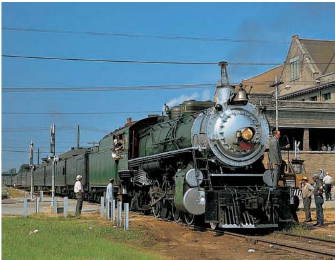
Above: Baldwin built Southern No. 4501 in 1911. The Southern's Ms-class ("s" for "superheating") Mikados were handsome, nicely proportioned, and powerful locomotives but otherwise unremarkable in their day. The Southern revived No. 4501 and made it a star of its steam program, where it entertained tens of thousands of people in two decades of main-line excursions. Working the Seaboard Coast Line rails in 1970, No. 4501 heads southward at Yemassee, South Carolina. George W. Kowanski
