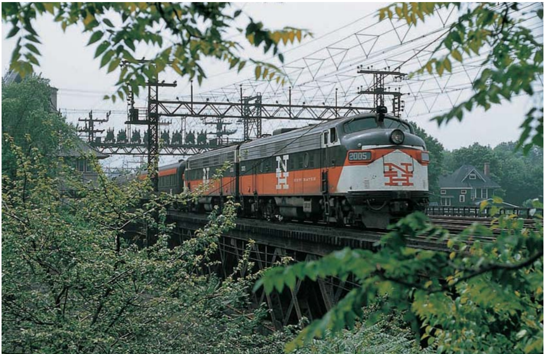
New Haven FL9s at Cos Cob on June 27, 1959. Electro-Motive's FL9 was a unique design, with specifications carefully tailored for New Haven's unusual service requirements. Among its unusual features was its dual-mode propulsion that allowed it to work as a diesel-electric or to draw power from the lineside third rail. Richard Jay Solomon
