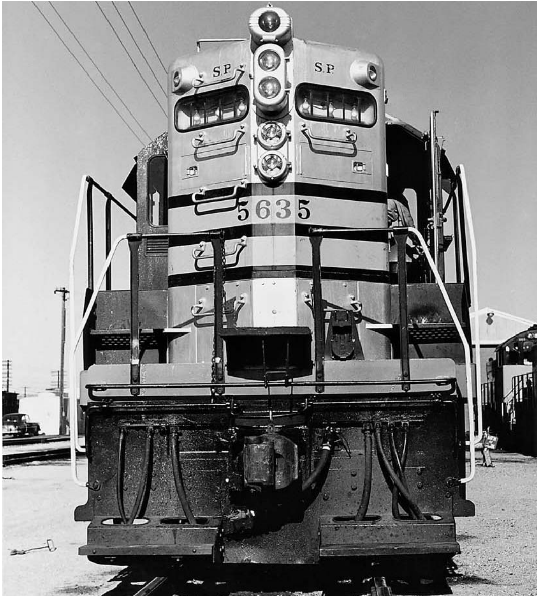
Southern Pacific's early GP9s were painted in its very classy "Black Widow" freight livery. Notice the panel below the numberboards for easy access. SP used numberboards to display train numbers rather than locomotive numbers, as was typical on most other railroads. The train number denotes a specific service, while a locomotive number identifies the specific engine. Bob Morris
