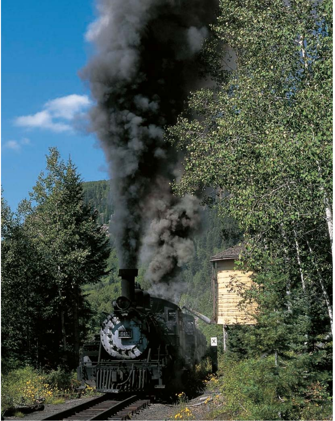
The Cumbres & Toltec Scenic Railroad's heavy excursion trains require a helper from Chama, New Mexico, up the 4 percent grade to Cumbres Pass. No. 463 is a head-end helper that has paused at Cresco tank for water. Before World War I, the Denver & Rio Grande upgraded the west slope of Cumbres Pass with heavier track to permit operation of K-27s as helpers. Brian Solomon
