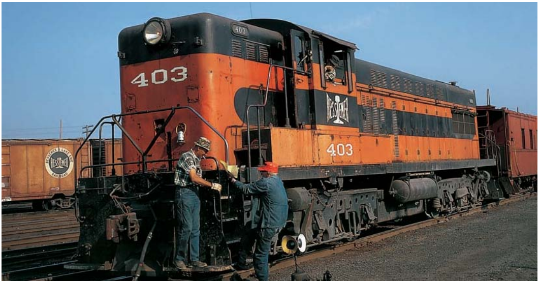
Ore-hauling Bessemer & Lake Erie operated an eclectic fleet of six-motor diesels a generation before six-motor types were standard power on other freight-hauling lines. B&LE's DRS-6-6-1500 No. 403 works at Albion, Pennsylvania, on June 7, 1970. It emerged from Baldwin's Eddystone plant 20 years earlier and enjoyed a relatively long career hauling heavy tonnage. Doug Eisele
