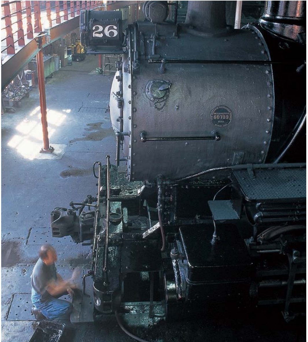
No. 26 receives nominal maintenance at Steamtown's former Lackawanna Scranton roundhouse. This classic 0-6-0 switcher was built by locomotive manufacturer Baldwin for its own use as a shop switcher. It is one of several locomotives that Steamtown has restored to working order. Brian Solomon
