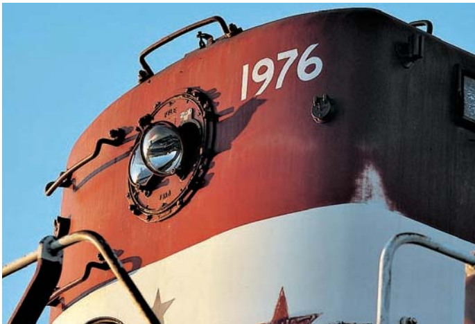
This detail shows the short hood and headlight on G&W RS-1 No. 1976. Built by Alco in May 1955 as G&W No. 30, the locomotive was renamed E. P. McCloskey , renumbered, and painted red, white, and blue for the American bicentennial. Brian Solomon
