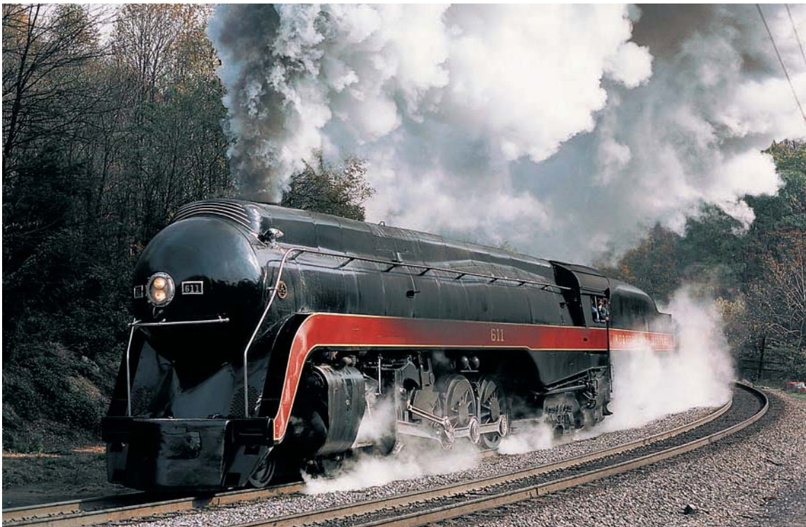
Above: Bathed in its own smoke and steam, N&W No. 611 charges west at Hardy, West Virginia, on October 23, 1982. In their day, the N&W's J-class locomotives were noted as exceptionally smooth-running machines. Precision counterbalancing helped minimize destructive dynamic forces. George W. Kowanski
