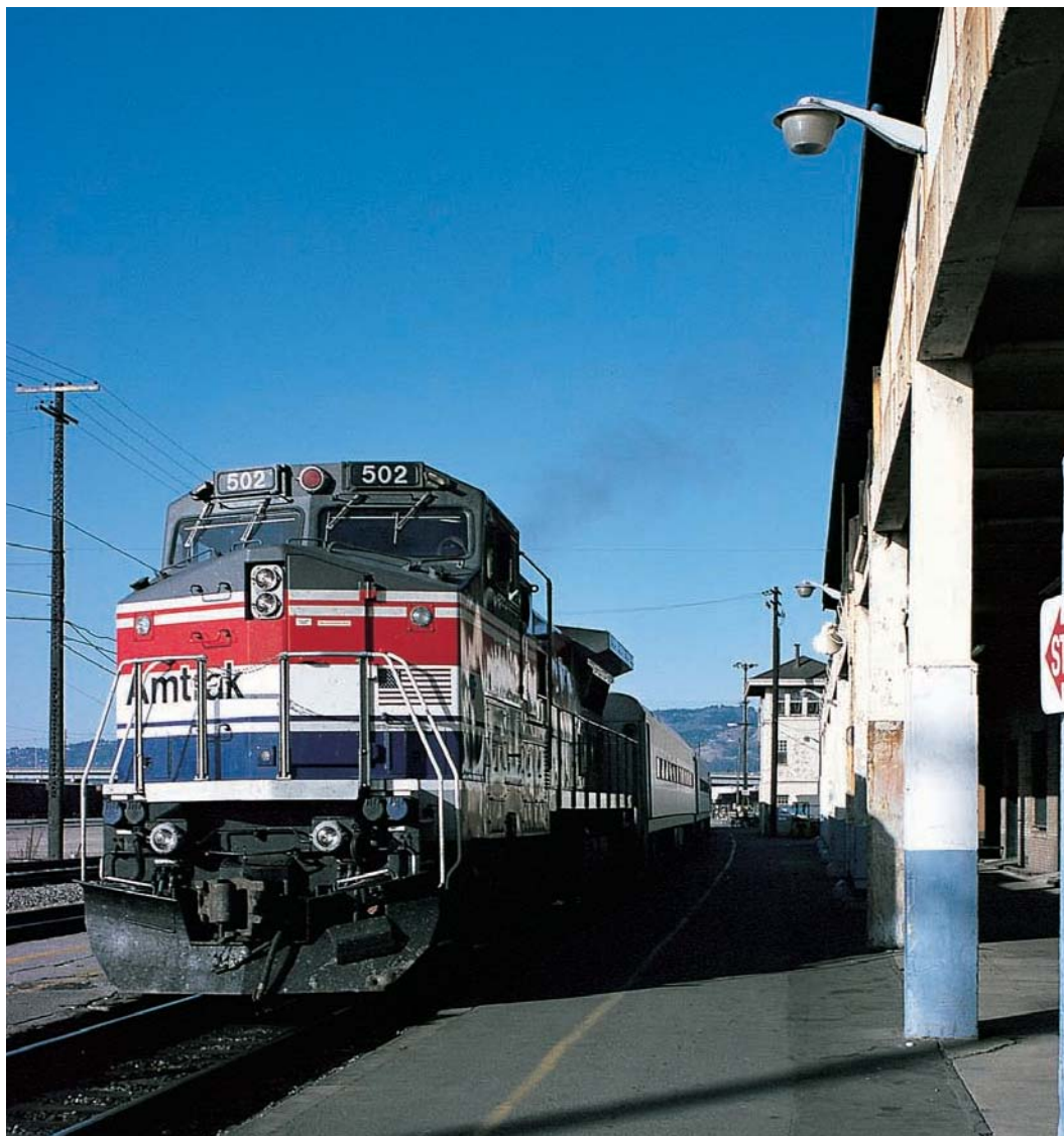
Amtrak General Electric Dash 8-32BWH No. 502 with a Capitol s train is seen at 16th Street Station in Oakland, California, in 1992. Amtrak's 20 Dash 8-32BWHs built in 1991 were similar to Santa Fe Railway's Dash 8-40BWs freight locomotives and share most external dimensions. However, Amtrak's Dash 8-32BWH is powered by a 12-cylinder FDL engine rated at 3,200 horsepower for traction. An extra alternator is used to produce head-end power for passenger cars—thus the H in the locomotive designation. Brian Solomon
