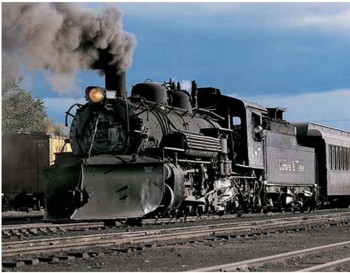
Cumbres & Toltec's former Rio Grande No. 487 carries a removable plow. Beneath the plow is a more typical pilot such as that seen on sister K-36 No. 481 (see pages 140–141). Brian Solomon
