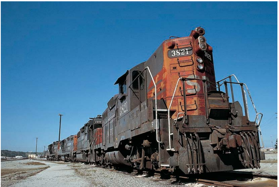
Southern Pacific No. 3821 is among GP9Es laying over at Watsonville Junction on SP's Coast Line. In addition to oscillating lights and fixed headlights, SP diesels typically featured classification lamps, although by the 1990s these had been blanked out. Class lamps had been necessary for the method of train movement authorization under the old timetable and train order rules. Brian Solomon
