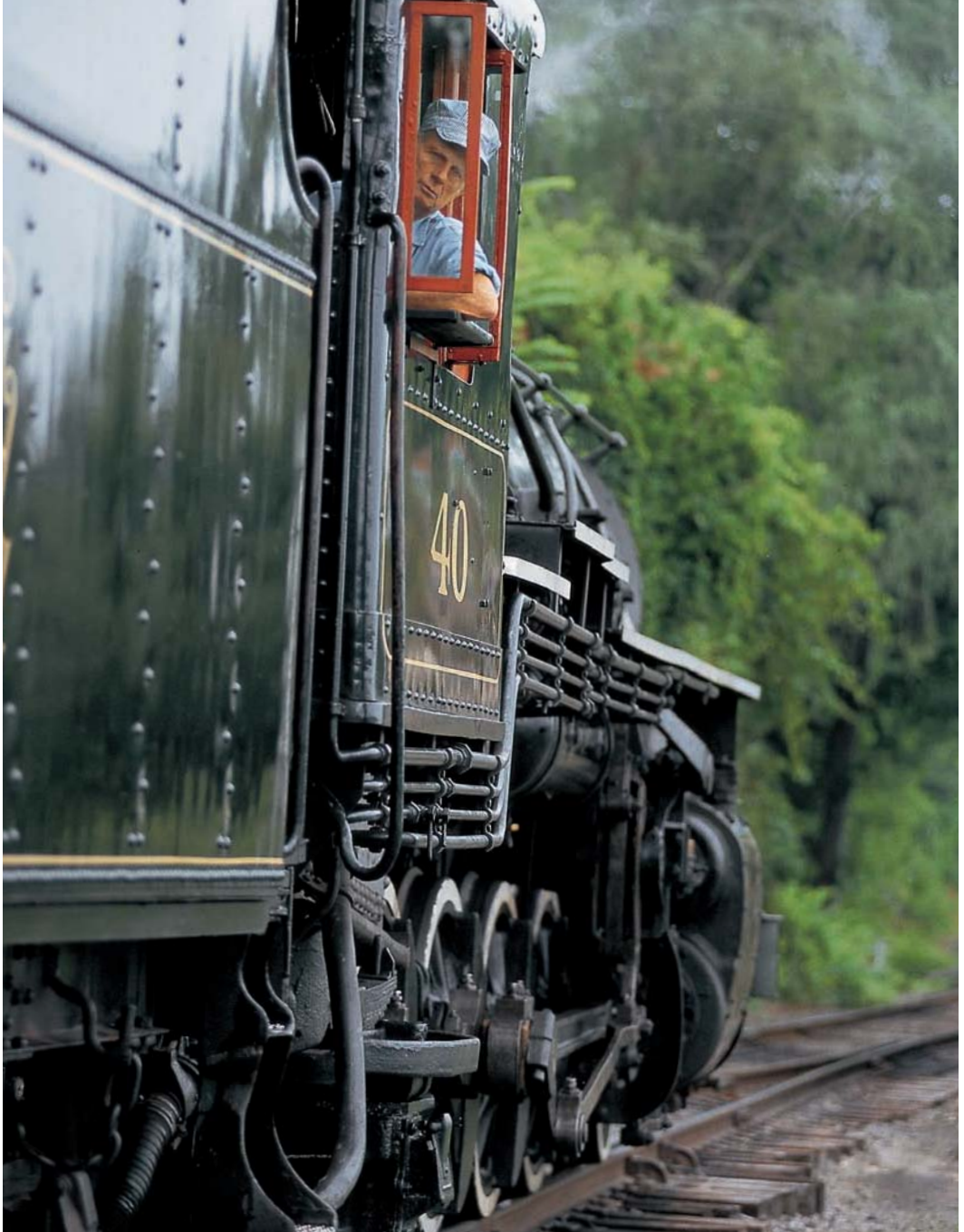
A view down the length of the locomotive from the tender. No. 40's relatively small-diameter drive wheels were typical of branch-line freight locomotives, where traction is more important than speed. Brian Solomon
