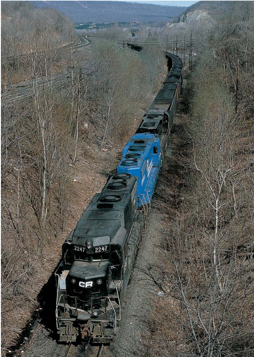
On March 12, 1980, Conrail GP30 No. 2247—still wearing Penn Central black—leads a freight at Overview, Pennsylvania, heading into the former Pennsylvania Railroad Enola Yard. The GP30 was powered by a 16-cylinder turbocharged 567 diesel. Turbocharging helped extract 2,250 horsepower from the 16-567, originally designed for 1,350-horsepower. Doug Eisele
