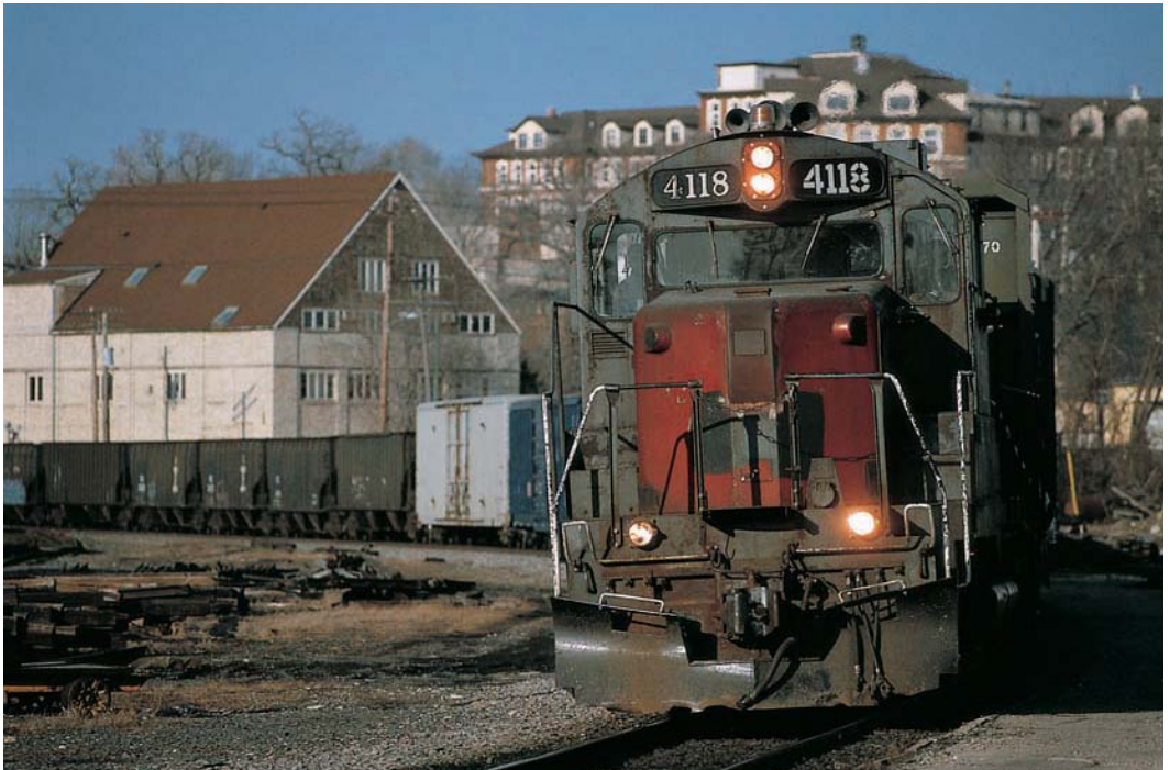
Wisconsin & Southern acquired a variety of EMD road switchers from Southern Pacific, including this old GP20E, originally SP No. 7224. Known by reporting marks WSOR, the railroad operated a network of lines in southern Wisconsin. On March 22, 1996, WSOR No. 4118 leads a freight over Wisconsin Central trackage in Waukesha. Brian Solomon
