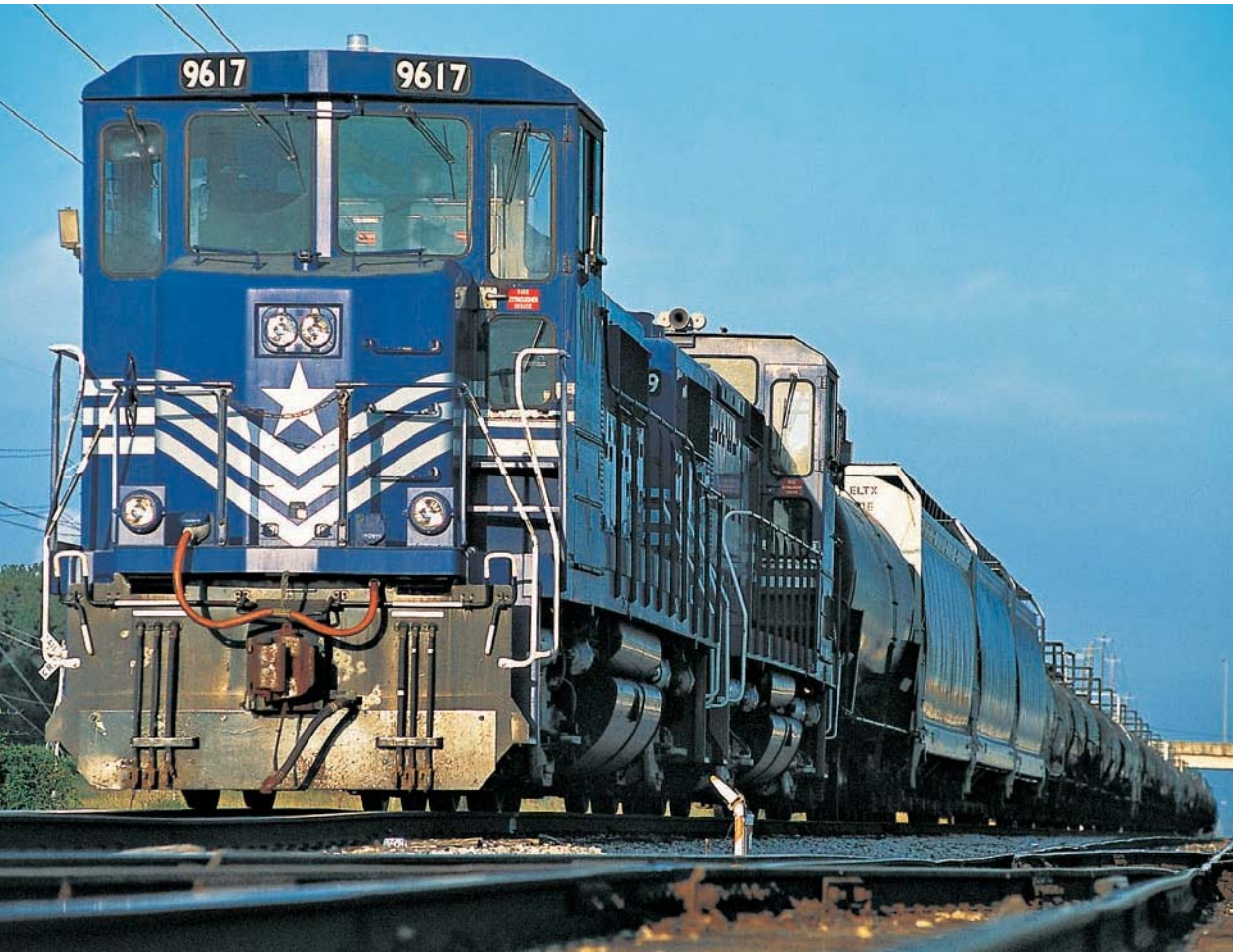
Two Port Terminal Railway Association MK1500Ds work a chemical train at Penn City Yard in Channelview, east of Houston, Texas, on June 12, 2004. MK Rail built 24 MK1500Ds in 1996 for the PTRR. These are the road's sole motive power for switching service in the Houston area. No. 9617 began its career as New York Central GP7 No. 5610 in the early 1950s. Tom Kline
