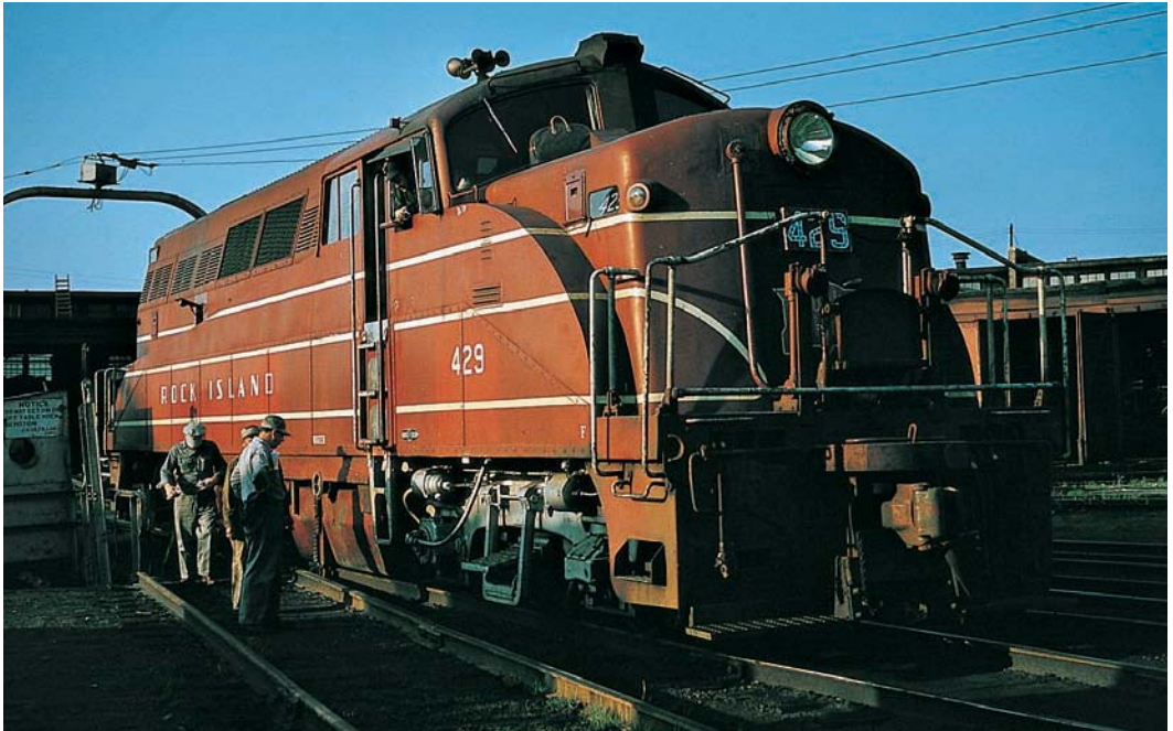
Few were the number of Electro-Motive BL2s—only 52 were built between 1947 and 1948—yet this unusual model found a great variety of work, from hauling potatoes in northern Maine to working branch lines in the Midwest and serving Rock Island in commuter service. At the end of a Chicago suburban run, Rock Island BL2 No. 429 rests at the Blue Island on July 18, 1958. Richard Jay Solomon
