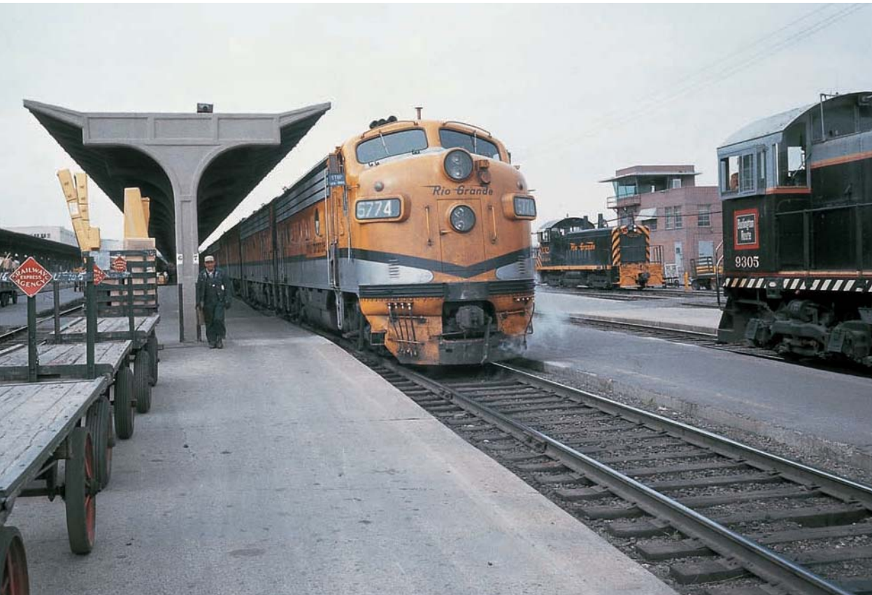
The westbound California Zephyr makes its scheduled station stop at Denver Union Station in 1966 to pick up passengers and exchange the Burlington E-units that brought the train from Chicago with Rio Grande F7s for the trip over the Rockies. To the right of the Zephyr are a Rio Grande EMD SW1200 and a World War II-vintage Burlington Alco S-2 switcher. Richard Jay Solomon
