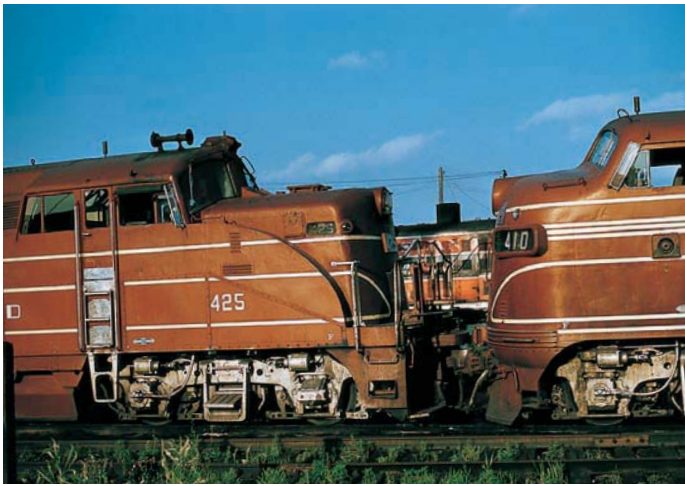
The beautiful and the ugly posed nose to nose: Rock Island F-unit No. 310 and BL2 No. 425 face each other at Blue Island on July 18, 1958. In the late 1940s, Electro-Motive followed the lead established by Alco and introduced this 1,500-horsepower road-switcher model. The odd-looking BL1/BL2 was essentially an F3A in a modified carbody better suited for switching. Richard Jay Solomon
