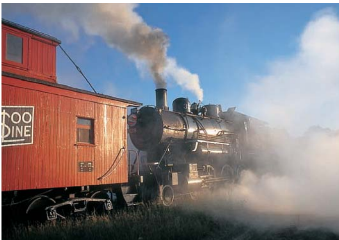
Above: The Ten-Wheeler type was first built in the 1840s but gained in popularity after the 1860s. Long after the perfection of larger types, this wheel arrangement continued to be built as a dual-service locomotive. Northern Pacific No. 328, built in 1905, is a classic example of a versatile early twentieth-century locomotive. Brian Solomon
