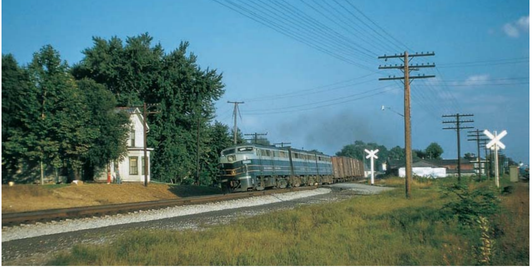
An A-B-A set of Baltimore & Ohio Alco FAs wearing the as-delivered two-tone blue leads a westward freight at Creston in east-central Ohio in the mid-1950s. B&O operated a moderate-sized fleet of Alco FA/FB-2s built between 1950 and 1953. Rated at 1,600 horsepower, these were nominally more powerful than Electro-Motive's F7, which was a more common type on B&O lines in the 1950s. J. William Vigrass
