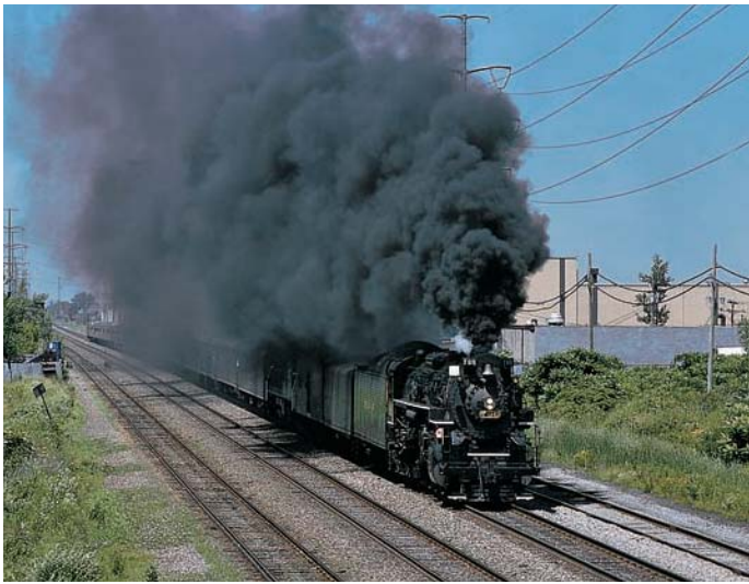
No. 765 works Conrail's multiple-track Niagara Branch near Black Rock, New York. The Berkshire type was the first superpower locomotive, a distinct improvement over earlier designs. The type was built to efficiently haul more freight faster than any previous type. The success of the Berkshire, with its enlarged firebox and boiler, led to a host of new superpower designs. Brian Solomon
