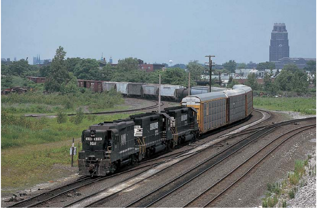
On July 3, 1989, a venerable Norfolk & Western high-hood GP30 leads a westward Norfolk Southern freight at Buffalo, New York. In the distance is the famous Buffalo Terminal. N&W and Southern were the only two railroads to order GP30s with the high short-hood option. Brian Solomon
