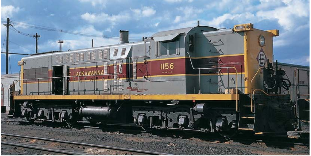
Baldwin's heavy road switcher was powered with the 608SC engine and was initially rated at 1,500 horsepower. It was offered to railroads as a four-motor with either B-B or A1A trucks, or as a six-motor with C-C trucks. These types were respectively designated as models DRS-4-4-1500, DRS-6-4-1500, and DRS-6-6-1500. Erie-Lackawanna DRS-6-6-1500 No. 1156 was photographed at Buffalo, New York, on October 4, 1970. Doug Eisele
