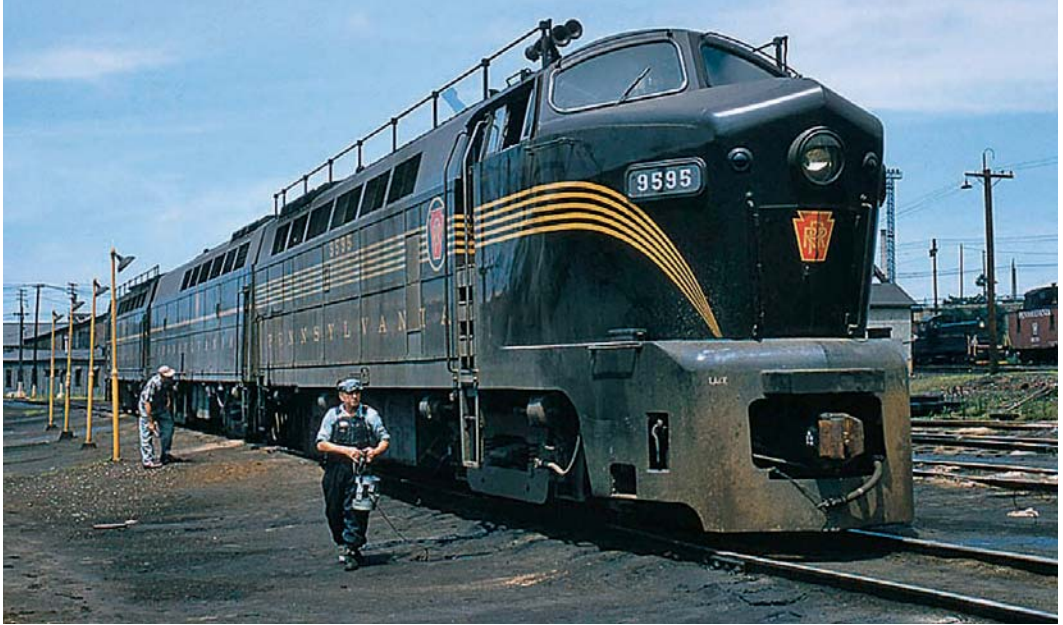
Pennsylvania Railroad RF-16 No. 9595 rests at Cleveland's Kinsman Yard on July 11, 1958. The Pennsy, like many owners of Baldwin road diesels, tended to assign them to very heavy freights; Pennsy, New York Central, and Baltimore & Ohio all operated shark-nose models in mineral service. Today it seems strange that streamlined diesels would have spent so much time working away from the public eye in obscure freight service. Richard Jay Solomon
