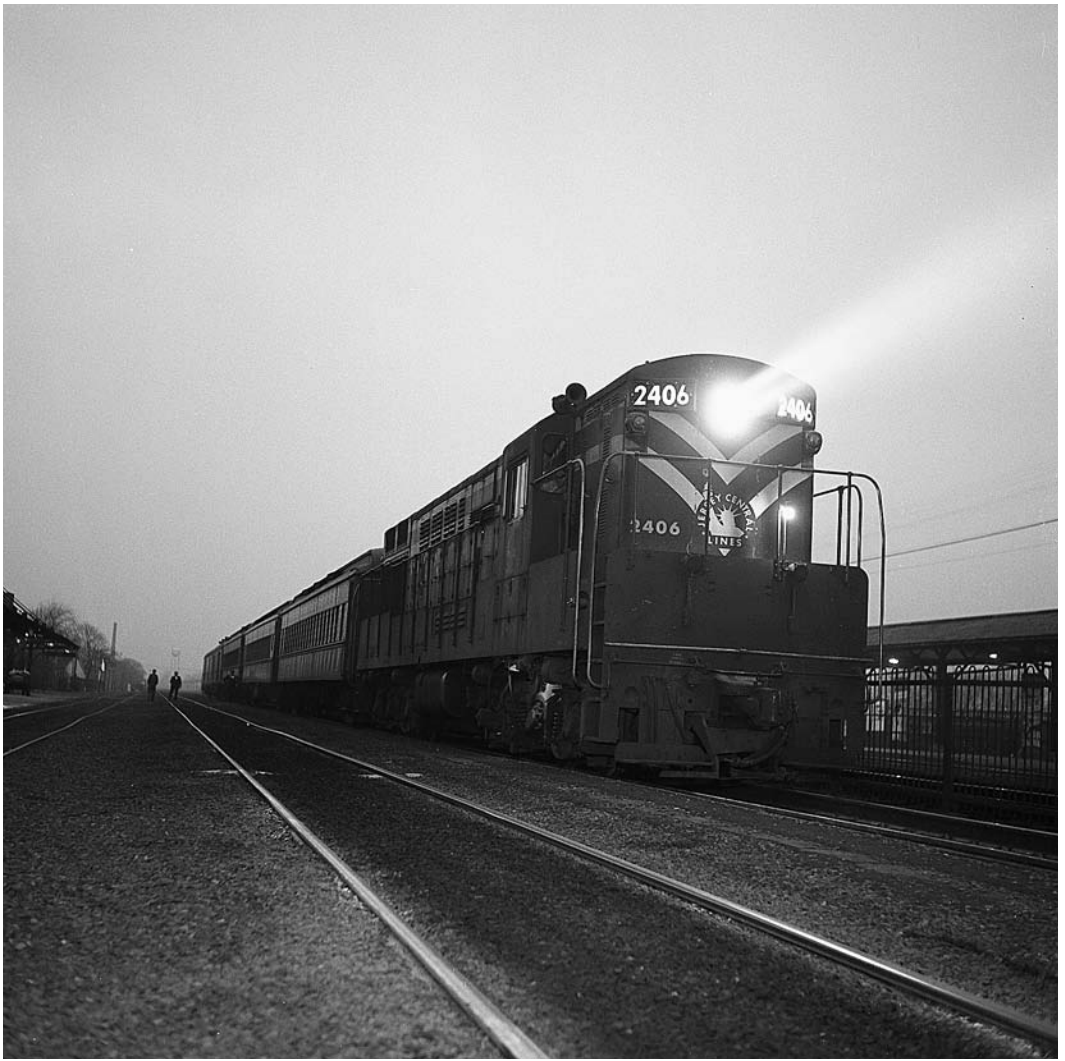
Central Railroad of New Jersey, along with Southern Pacific, assigned 2,400-horsepower F-M Train-Masters to suburban passenger services where frequent stops meant that locomotives needed to get up to speed quickly to maintain schedules. Richard Jay Solomon
