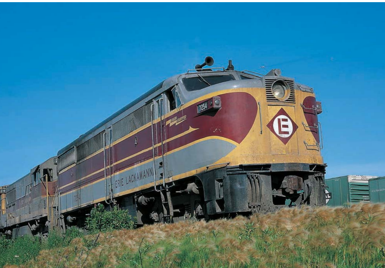
Erie Lackawanna FA-1 No. 7254 catches the sun east of Buffalo at Bison Yard in Sloan, New York, in July 1968. EL inherited its FA/FBs from the Erie Railroad. Powered by Alco's 244 engine, the FA-1 was rated at 1,500 horsepower. While many railroads used FA models into the 1960s, these Alco road units were not as well regarded as the EMD F-units and had become rare by 1970. Doug Eisele collection
