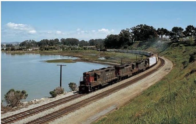
Southern Pacific GP9E No. 3842 and a pair of SD9Es lead a westward freight along the shore of California's San Pablo Bay at Pinole on April 18, 1993. In the 1970s, SP rebuilt many of its 567-powered GP and SD units, which allowed them to continue in revenue freight service into the 1990s. Brian Solomon
