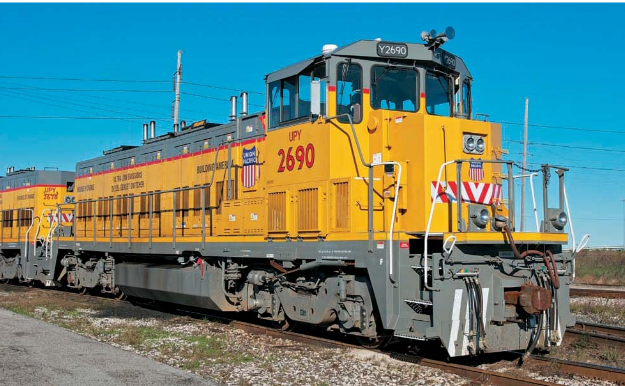
Union Pacific No. 2690 is a Railpower three-Genset, four-motor RP20BD (also variously referred to as a RP20B and RP30GE) assigned to switching work in Texas. Pat Yough
