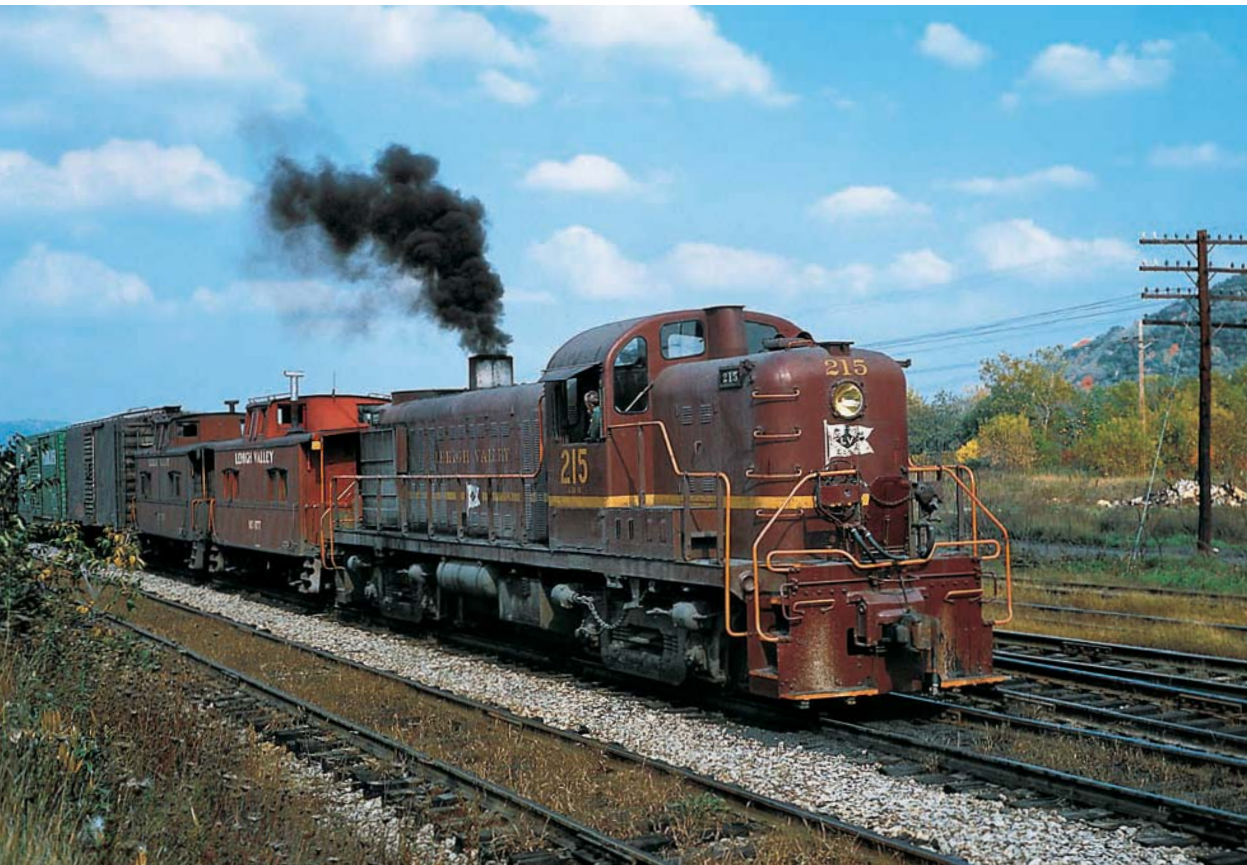
Lehigh Valley Alco RS-3 No. 215 drills the yard at Manchester, New York, on October 17, 1971. Alcos were famous for their smoke shows when notched out rapidly; the 244 engine in particular was especially smoky. R. R. Richardson photo, Doug Eisele collection
