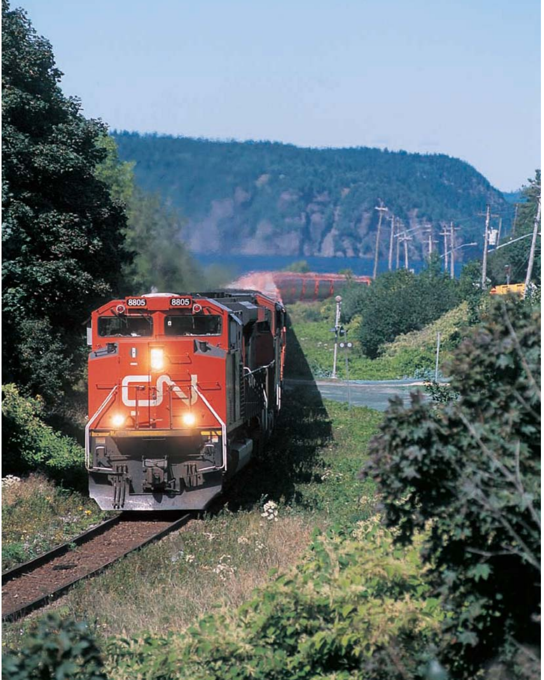
Canadian National has not embraced the AC-traction trend. Instead it has purchased DC-traction models exclusively from both General Electric and EMD in recent years. On September 9, 2009, SD70M-2 No. 8805 leads train 406 at Rothesay, New Brunswick. George S. Pitarys
