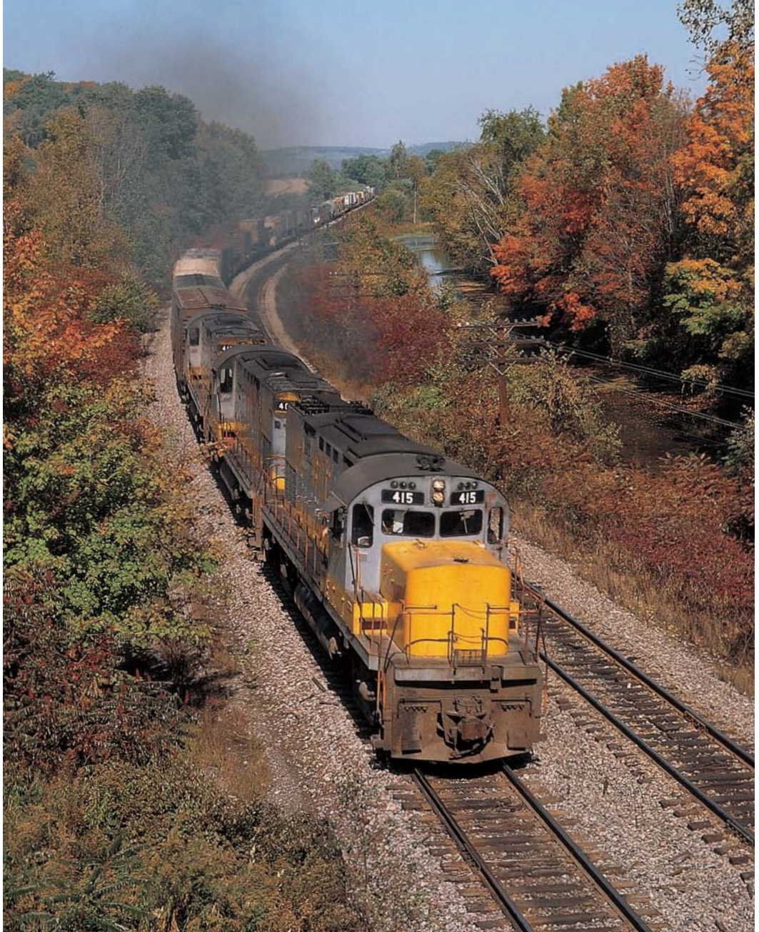
On October 5, 1974, Lehigh Valley No. 415 and two other LV C-420s lead an eastward freight. All are in Lehigh's as-delivered gray and yellow livery. With the introduction of the Century series in 1963, the C-420 was the 2,000-horsepower model that succeeded the short-lived RS-32. Where only 35 RS-32s were built, the C-420 accounted for 131 units, including a pair sold to Mexico. R. R. Richardson photo, Doug Eisele collection
