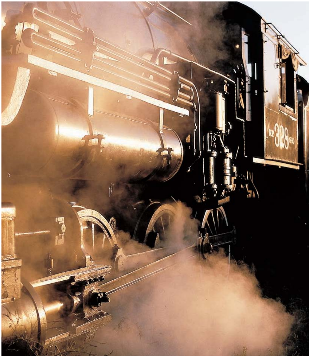
The first rays of daylight catch Northern Pacific No. 328 under steam at Dresser, Wisconsin, in August 1996. The large horizontal tank above the cylinders and running gear is the air reservoir used for the Westinghouse automatic airbrake. Brian Solomon
