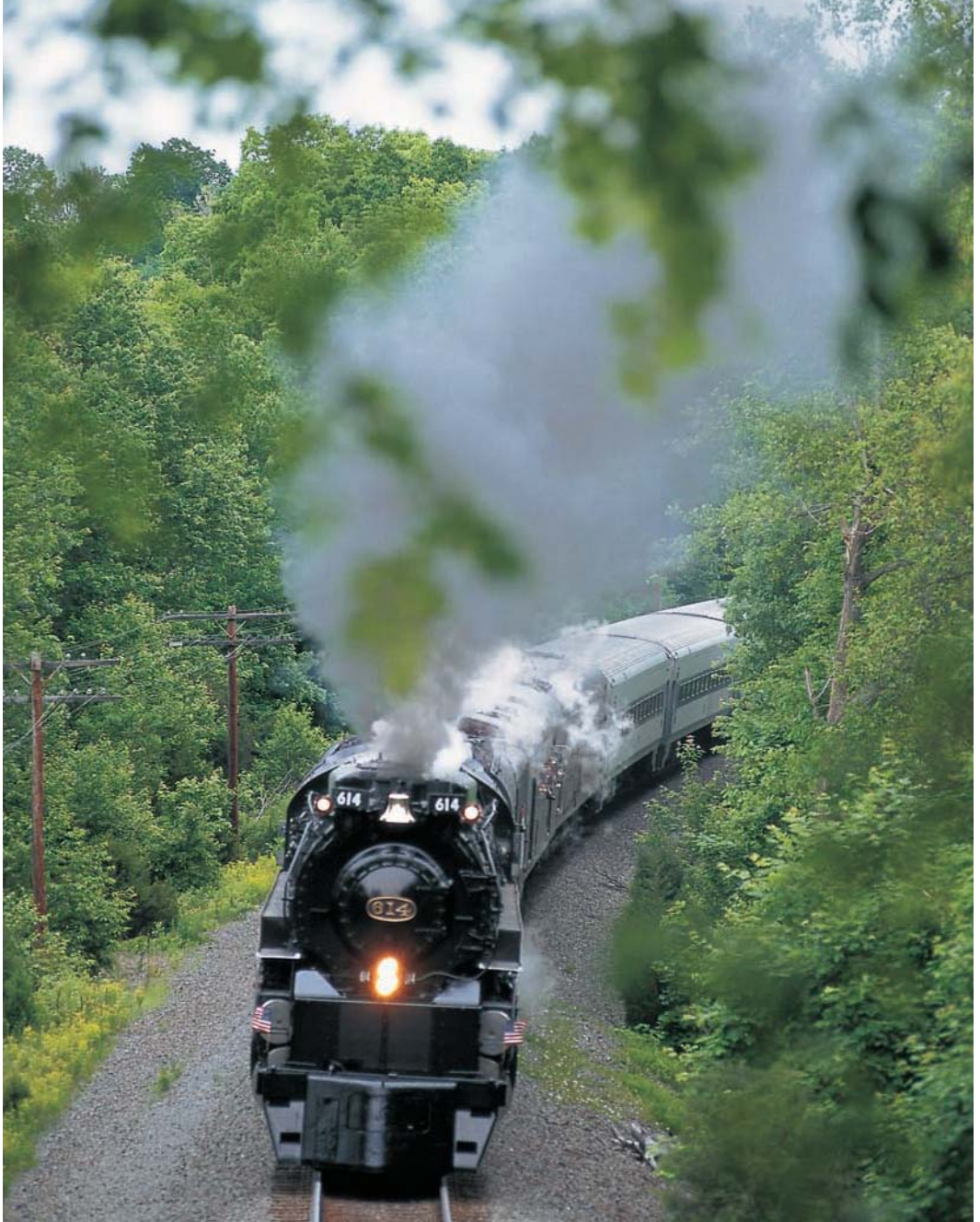
A low headlight and a high bell were typical of most C&O late-era steam power. Mechanically, the C&O's J-3a 4-8-4s were near cousins to the Nickel Plate Road's S-class Berkshires. Working an excursion train on the former Erie Graham Line, No. 614 pounds the rails near Salisbury Mills, New York. Brian Solomon
