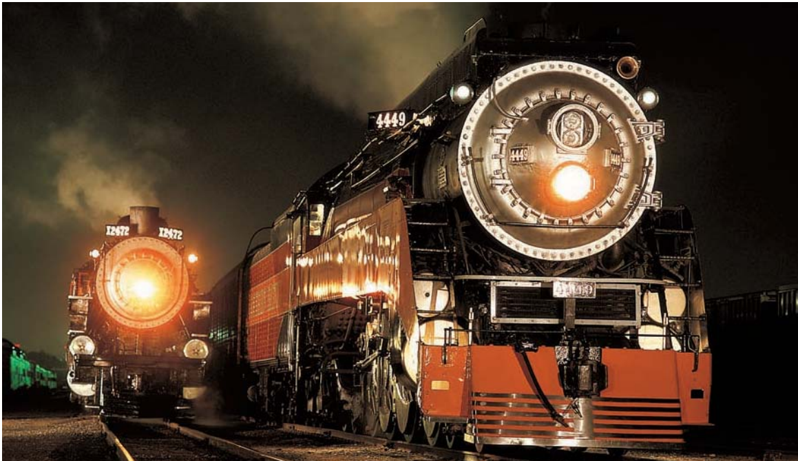
Above: Two generations of Southern Pacific passenger steam: On the left is Baldwin-built P-8 Pacific-type No. 2472, one of 15 locomotives delivered in 1921; on the right is No. 4449, built in 1941. When new, both types represented the best of the railroad's passenger power. Today, these classics inspire nostalgia for passenger trains that once connected California cities with those across the southwestern United States. Brian Solomon
