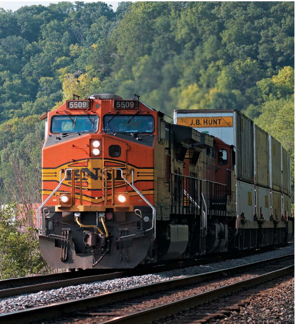
BNSF Dash 9-44CW leads an eastward double-stack along the Mississippi at Savanna, Illinois, on June 24, 2010. The Dash 9 employed variations of the 16-7FDL diesel and GE 752 traction motor, and it represents 30 years of engineering refinement. Brian Solomon
