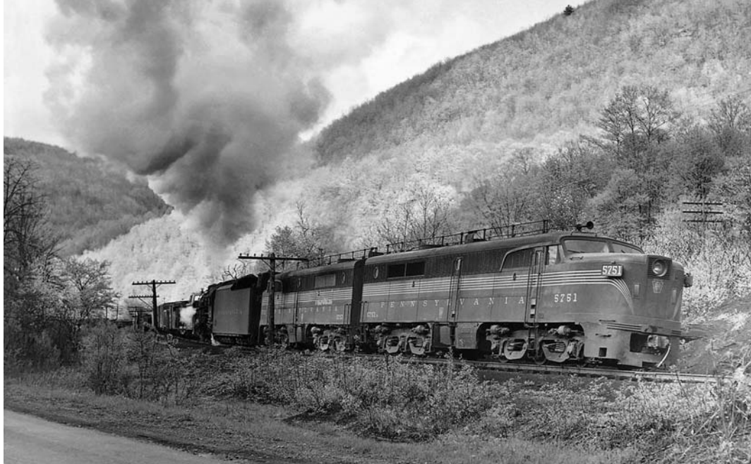
In 1947, Pennsylvania Railroad bought 10 PAs and 5 cab-less PB "boosters" from Alco. These had been intended for passenger service, but within a decade the Pennsy reassigned them to less glamorous jobs. On May 4, 1957, Nos. 5751A and 5757A work as helpers along with a venerable 11s Decapod on freight climbing northward on the Elmira Branch. Jim Shaughnessy
