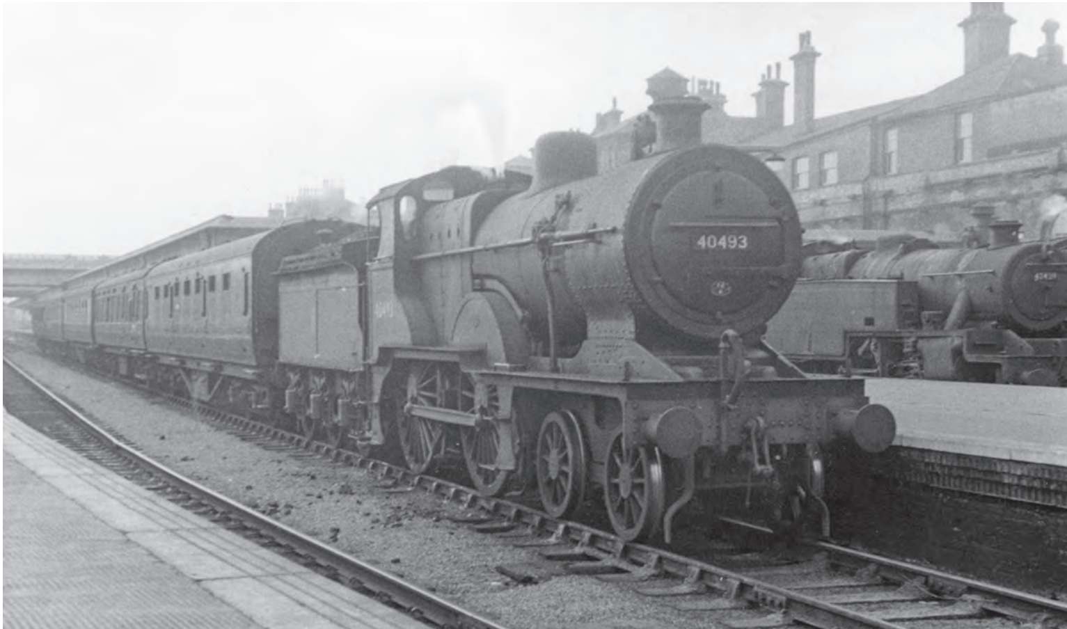
Another Johnson Midland design and Fowler rebuild, 4-4-0 Class '2P' No. 40493 has arrived with the 9.20am Lincoln-Derby semi-fast on 14 September 1957. Built in 1897 at the nearby Works, this was condemned from Nottingham shed in July 1959 and cut up by T.W.Ward, Killamarsh. ( M.E. Kirk/Martyn Reeve Collection )
