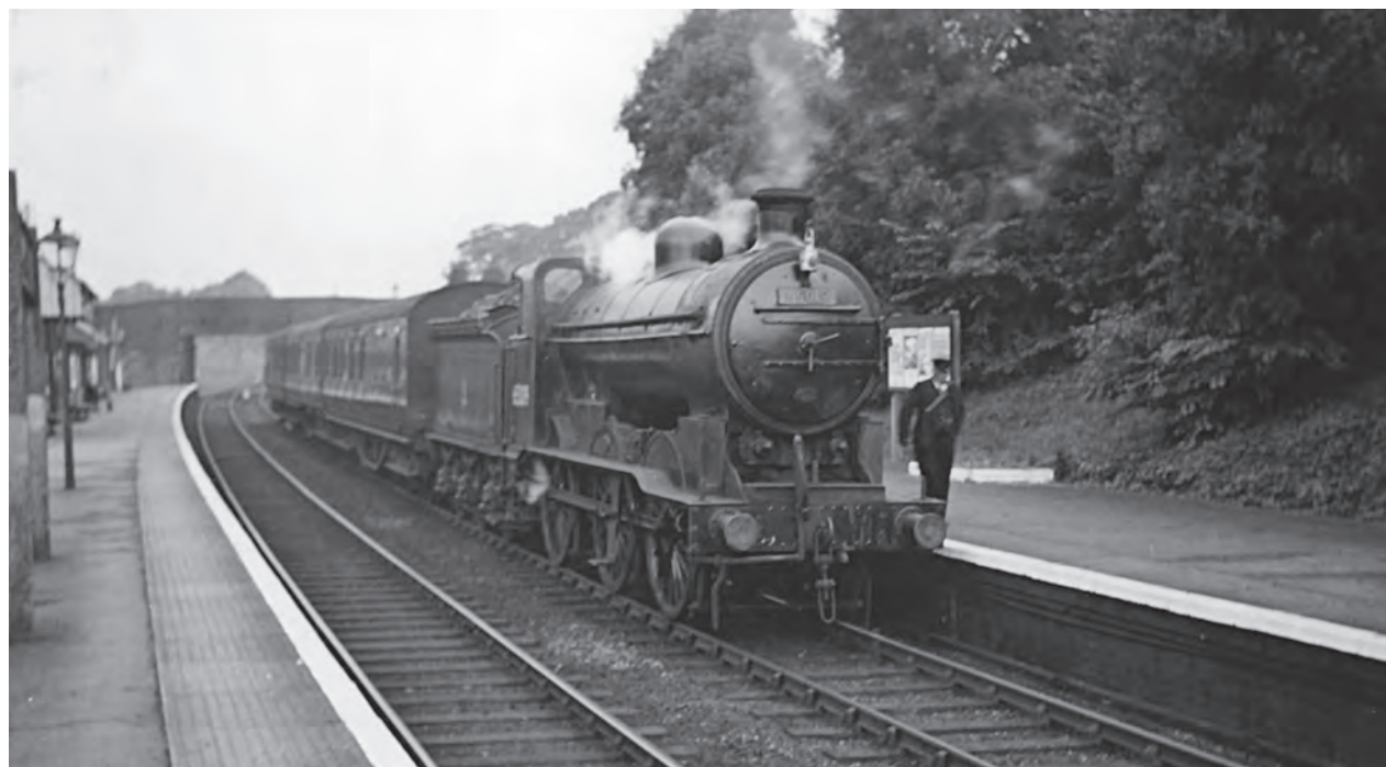
In Darkest Notts, a description by M.E. Kirk, the 5.35pm Nottingham (Victoria)-Newark (North Gate) local service is arriving at Radcliffe-on-Trent on 18 July 1952 with Ivatt 0-6-0 Class 'J2' No. 65019 in charge. This locomotive was built in 1912 at Doncaster Works and scrapped there when withdrawn from Colwick shed in March 1953. (M.E. Kirk/Martyn Reeve Collection)
