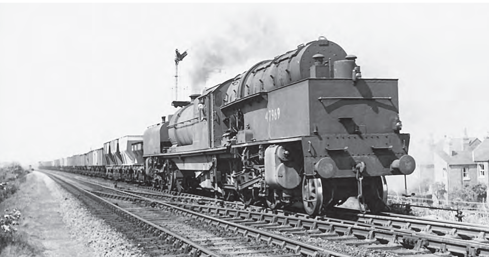
Beyer-Garratt Class 2-6-6-2T No. 47969, with its distinctive revolving bunker, runs bunker-first with a Clay Cross to Wellingborough train of empty iron-ore tippler and hopper wagons for the Northamptonshire ore fields as it passes Meadow Lane Junction on the High Level goods line in May 1957. Toton driver William (Bill) Webb revered these locomotives and liked nothing better than running bunker first, where he could sit with his feet up without smoke and steam enveloping the cab and obscuring the sighting of signals. No. 47969 was withdrawn from Hasland shed in August 1957 and disposed of at Crewe Works. ( Joe Wade )
