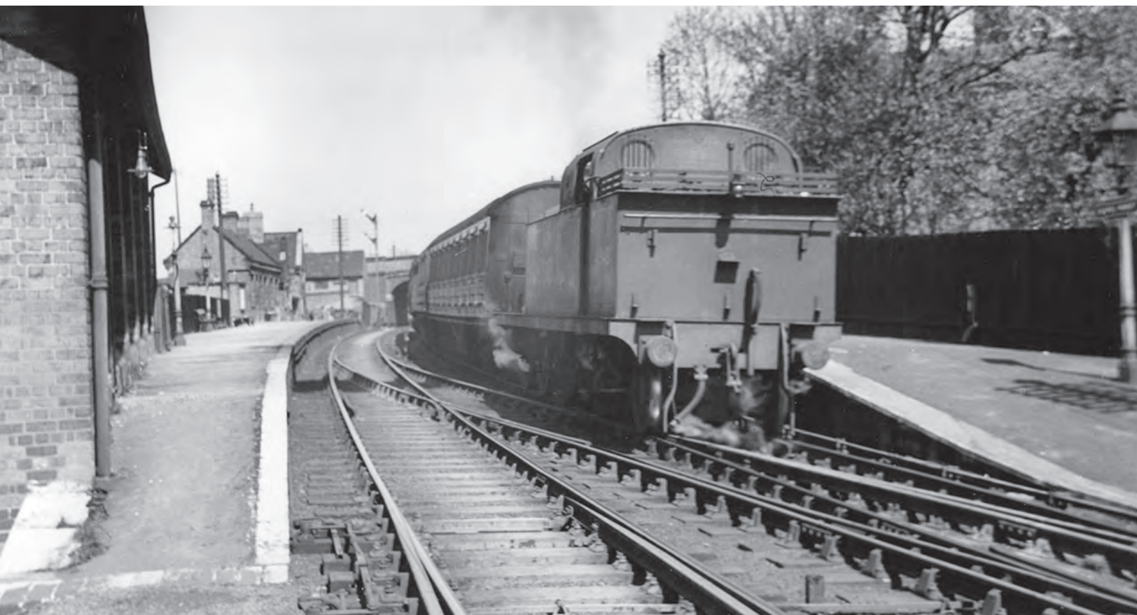
On 2 May 1953 the 11.25am Worksop-Nottingham (Midland) is about to leave Bulwell Market station hauled by Whitelegg 4-4-2T Class '3P' No. 41943. Built in 1927 at Derby Works, it was disposed of there when withdrawn from Mansfield shed in February 1956. The station opened on 2 October 1848 as Bulwell; it was renamed Bulwell Market in August 1952 to distinguish it from other Bulwell stations. It was closed along with other stations along the line in 1964 and reopened in 1994 as part of the new Robin Hood line. (M.E. Kirk/Martyn Reeve Collection)
