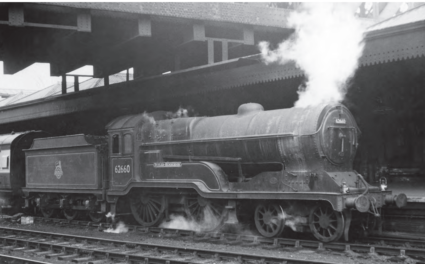
A closer look at the deplorable external condition of Robinson Class 4-4-0 'D11' No. 62660 Butler-Henderson with a Lincoln-Derby express standing underneath the Great Central line overbridge. Following its withdrawal in November 1960 from Sheffield (Darnall) shed, No. 62660 would be preserved by the British Transport Commission and restored to full Great Central livery. ( M.E. Kirk/Martyn Reeve Collection )
