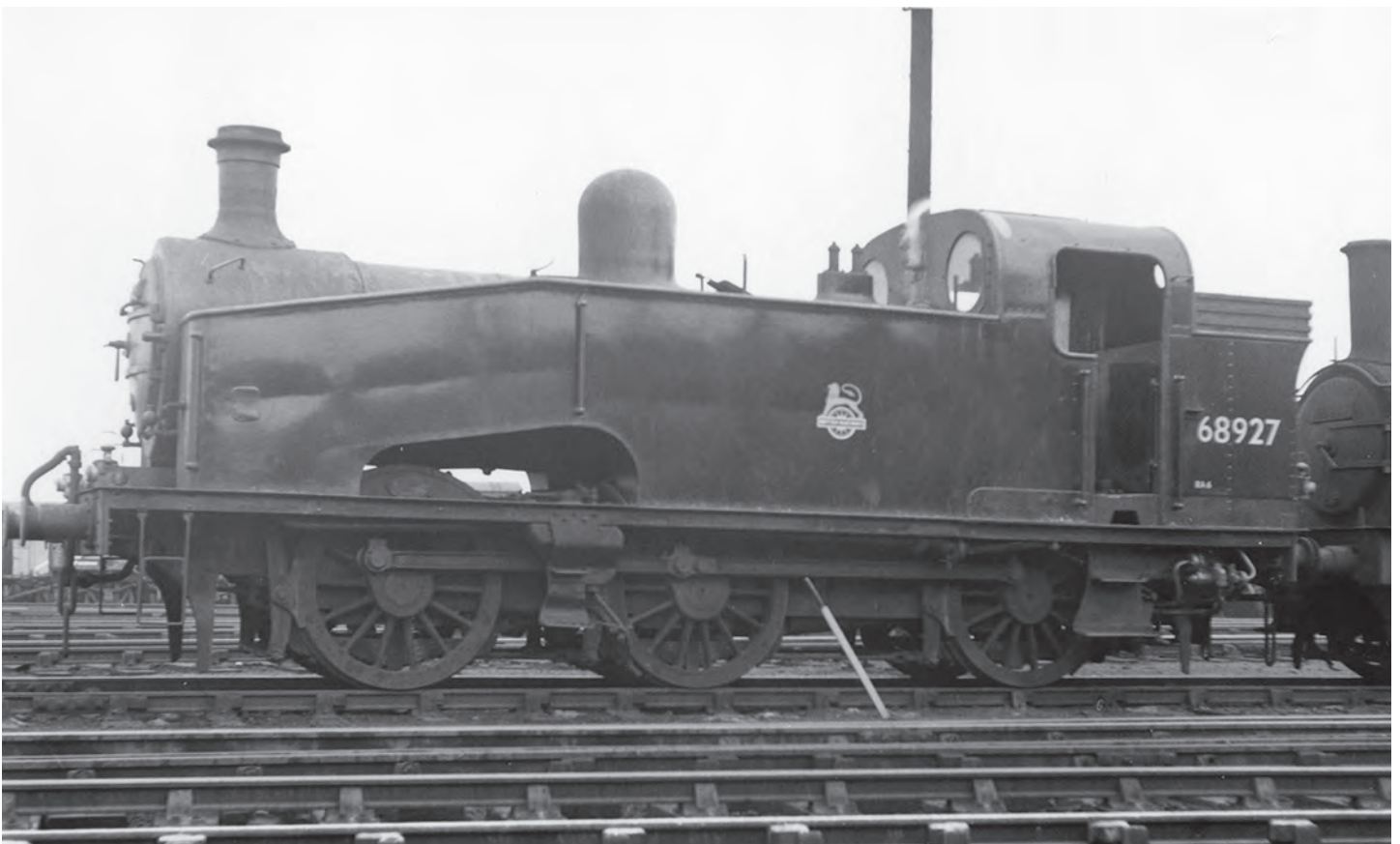
Recently outshopped, Gresley 0-6-0T Class 'J50' No. 68927 is seen here at Colwick shed on 10 June 1956. Built in 1922 at Doncaster Works, it was scrapped there when withdrawn from Colwick shed in April 1961. ( M.E. Kirk/Martyn Reeve Collection )
