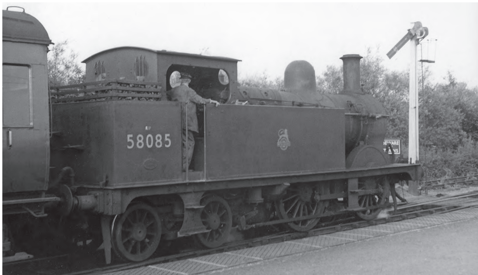
The 4.10pm from Southwell is ready to leave Rolleston Junction on 31 August 1955 with Johnson 0-4-4T Class '1P' No. 58085. Built in 1900 by Dubs & Co. Glasgow and condemned from Lincoln shed in April 1959, it was later cut up at Derby Works. The 2½ mile single track branch line from Rolleston (on the Midland Railway's Nottingham-Lincoln line) to Southwell was opened in 1847. The push-and-pull unit for passenger trains was finally withdrawn in June 1959, with goods traffic continuing for a further six years. (M.E. Kirk/Martyn Reeve Collection)
