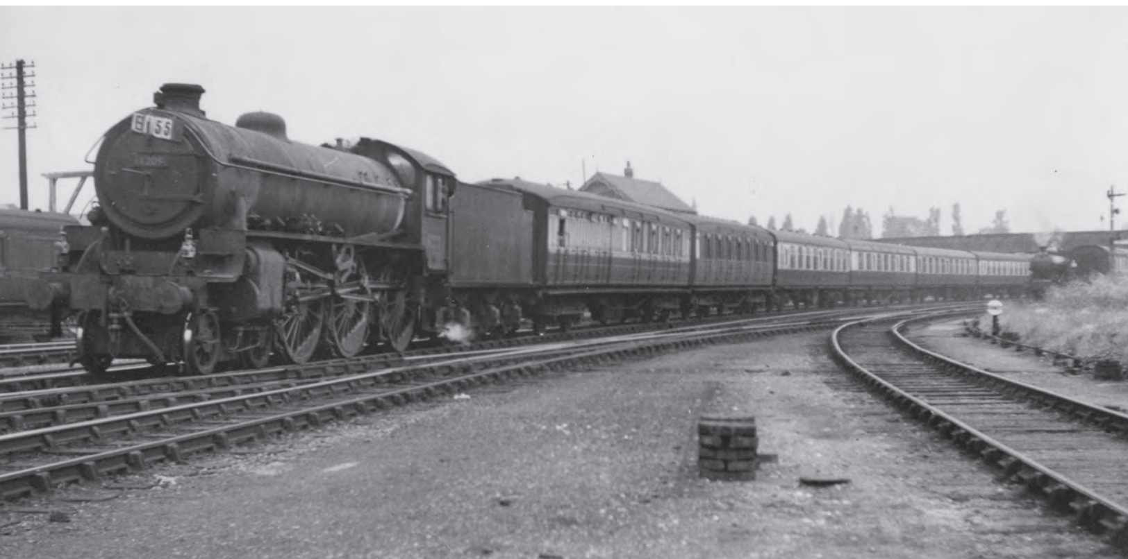
The 12.55pm (SO) Llandudno to Nottingham (Victoria) express is entering Friargate station on 10 July 1954 hauled by Thompson 4-6-0 Class 'B1' No. 61209. Manufactured by the North British Locomotive Company Glasgow in 1947 and withdrawn after a relatively short life from Colwick shed in September 1962, it was disposed of by Albert Loom, Spondon. A 0-6-2T Class 'N1' is on the right. (M.E. Kirk/Martyn Reeve Collection)
