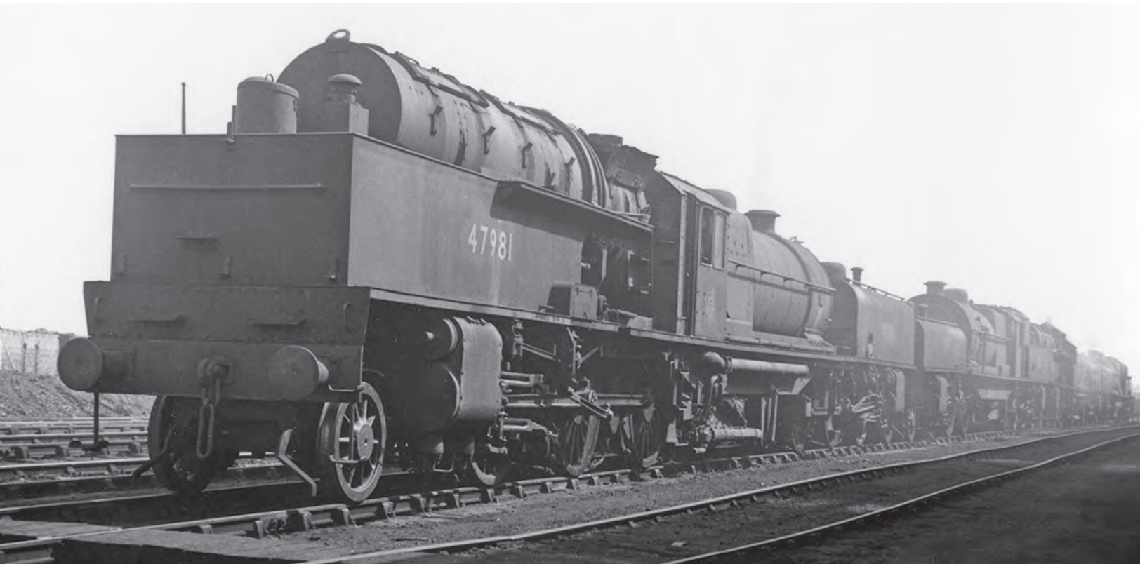
Photographed on the Garratt Road at Toton shed on 13 May 1956. Before the introduction of those giant 2-6-6-2T locomotives, the Toton-Brent coal trains were double-headed by Class '3F' and '4F' 0-6-0 tender engines. Here at rest are 47981, 47998, 47996, which were condemned from Toton during 1956 and 47994 withdrawn from Hasland shed in March 1958; all were cut up at Crewe Works. (M.E. Kirk/Martyn Reeve Collection)
