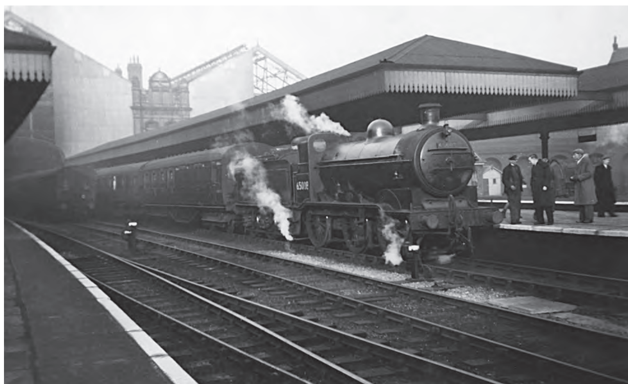
The 1.12pm (SO) stopping train from Pinxton has arrived in Nottingham Victoria station on 19 January 1952 behind Ivatt 0-6-0 Class 'J1' No. 65008. Built in 1908 at Doncaster Works, it was scrapped there when withdrawn from Colwick shed two months after this picture was taken. (M.E. Kirk/Martyn Reeve Collection)
