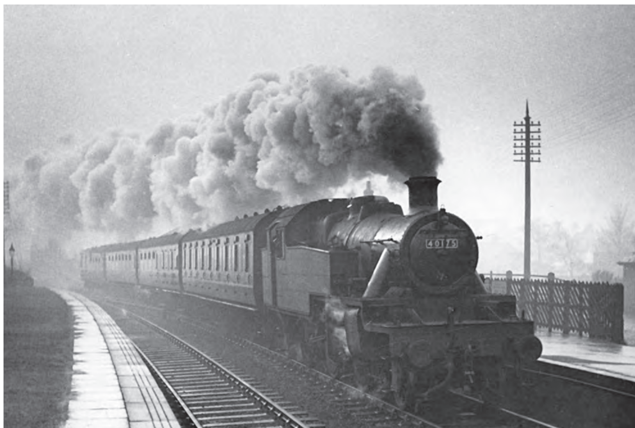
On 2 May 1953 the 11.25am Worksop-Nottingham (Midland) is about to leave Bulwell Market station hauled by Whitelegg 4-4-2T Class '3P' No. 41943. Built in 1927 at Derby Works, it was disposed of there when withdrawn from Mansfield shed in February 1956. The station opened on 2 October 1848 as Bulwell; it was renamed Bulwell Market in August 1952 to distinguish it from other Bulwell stations. It was closed along with other stations along the line in 1964 and reopened in 1994 as part of the new Robin Hood line. (M.E. Kirk/Martyn Reeve Collection)
