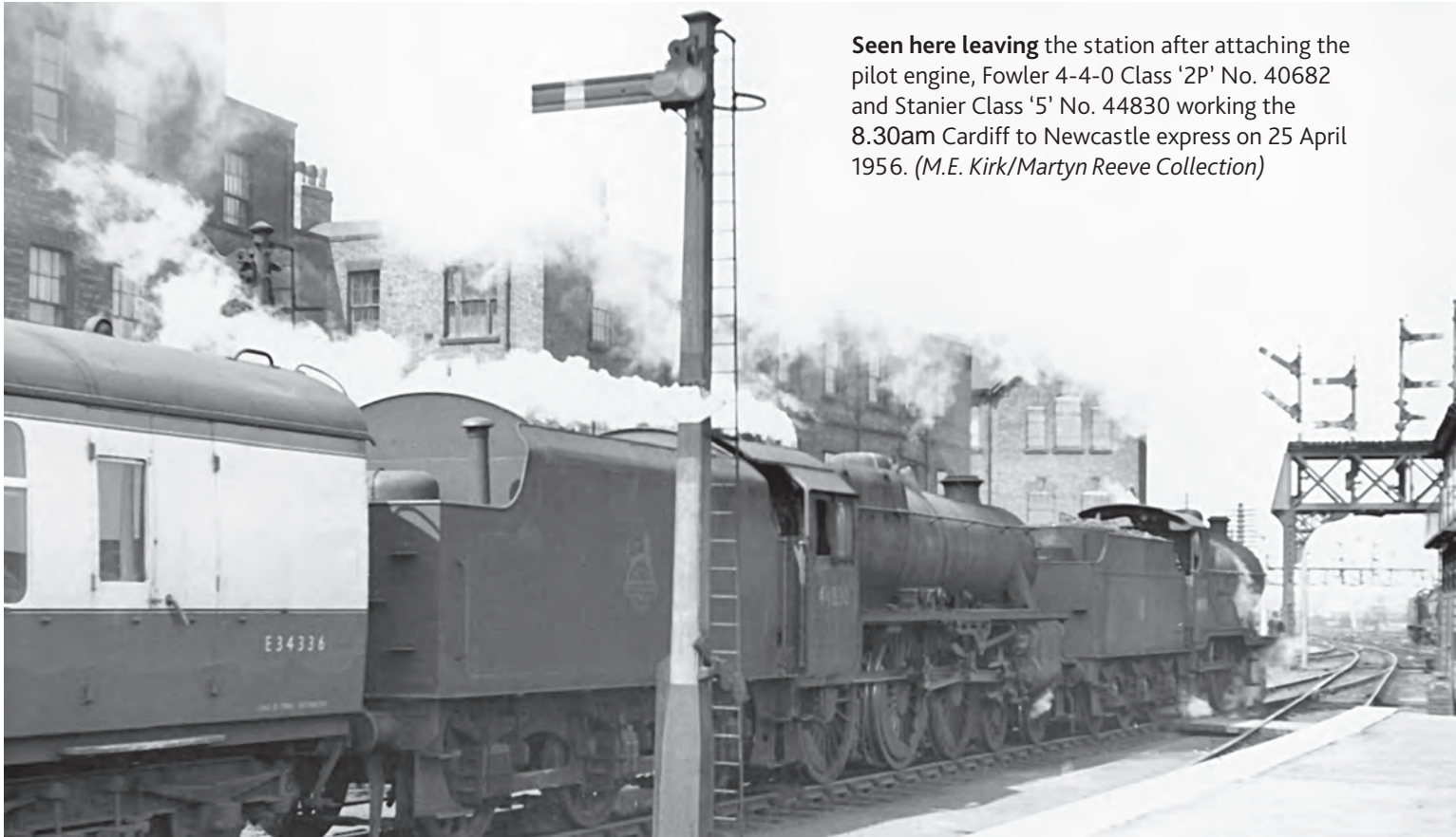
Derby station on 25 April 1956 , ex-LMS Stanier 4-6-0 No. 44830 piloted by Fowler Class '2P' No. 40682 are in charge of the 8.30am Cardiff-Newcastle express. The 'Black Five' was built in 1944 at Crewe Works and withdrawn from Heaton Mersey shed in August 1967 and disposed of at T.W.Ward, Beighton. 40682 was built in 1932 at Derby Works and condemned from Nottingham shed in February 1961 and disposed of by Albert Loom, Spondon. On platform 2 is the 1.05pm (SO) to Manchester (Central) with Fowler 'Compound' No. 40927, which emerged in 1927 from the Vulcan Foundry, was withdrawn from Derby shed in July 1957 and broken up at the nearby Works. ( M.E. Kirk/Martyn Reeve Collection )
