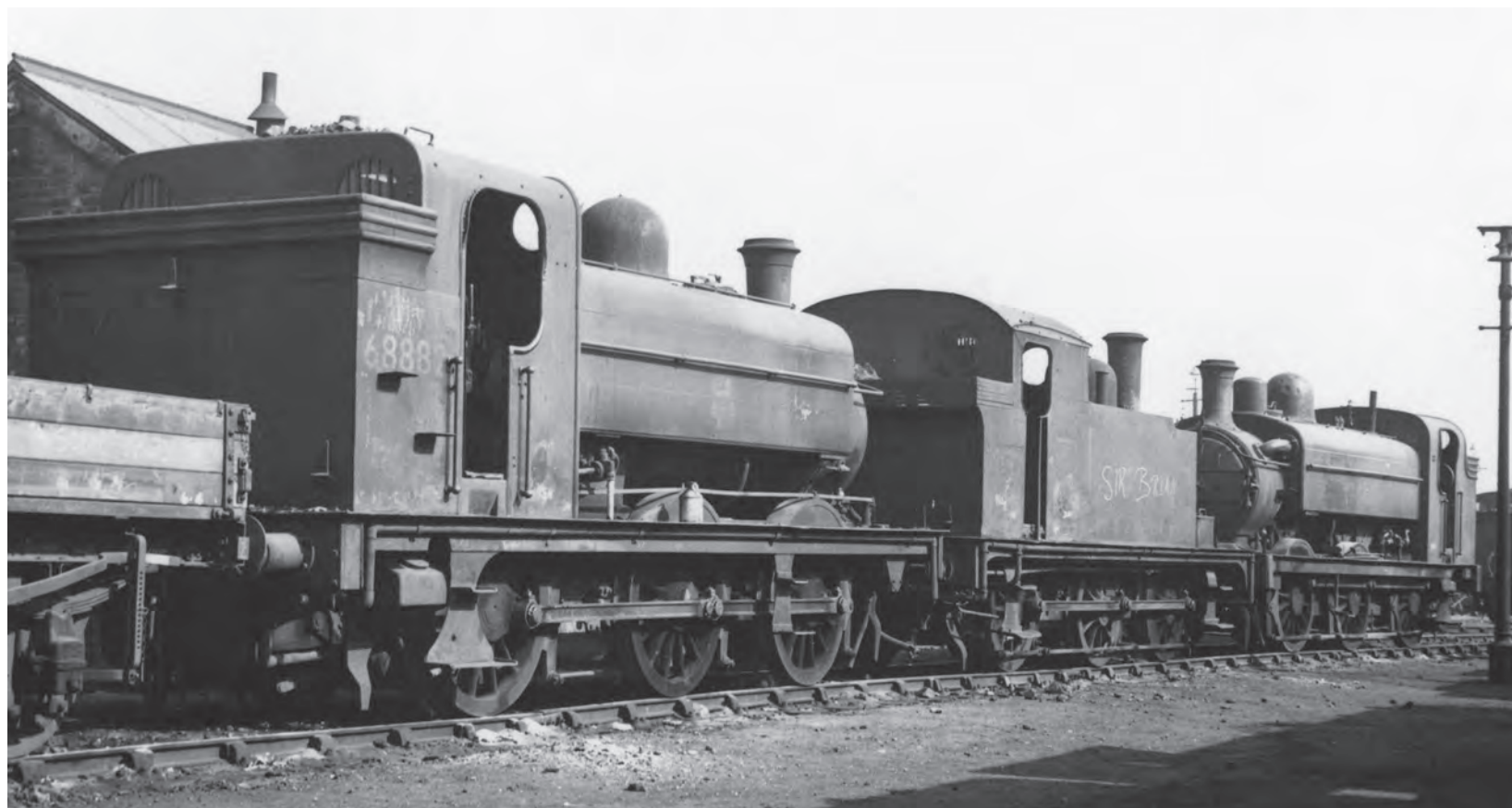
Colwick Shed on 13 May 1956. Stirling 0-6-0ST Class 'J52' No. 68882, built in 1908 at Doncaster Works and disposed of there when withdrawn from Colwick shed in January 1958. Holden 0-6-0T Class 'J69' No. 68629, built in 1904 at Stratford Works and broken up at Gorton Works when condemned from Colwick shed in November 1959. Stirling 0-6-0ST Class 'J52/1' No. 68759, built in 1900 at Doncaster Works and cut up there when withdrawn in July 1956 from Colwick shed. (M.E. Kirk/Martyn Reeve Collection)
