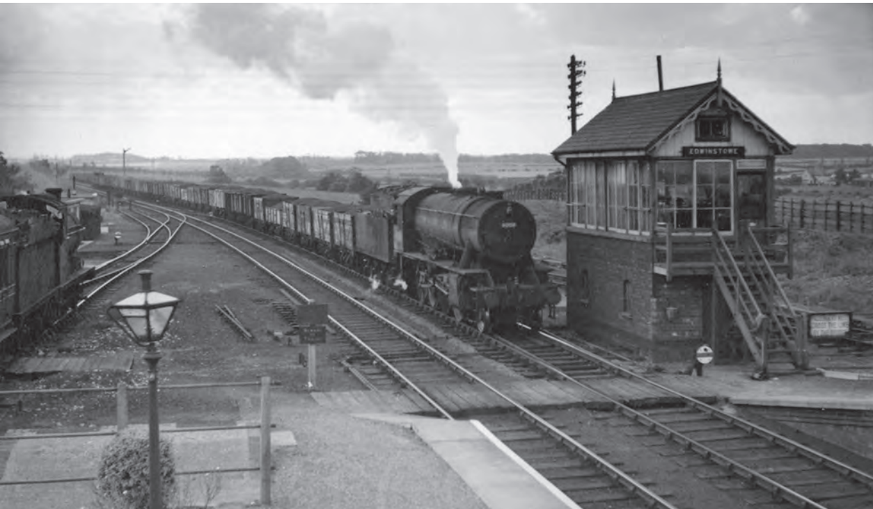
A coal train from Shirebrook is passing the signal box at Edwinstowe on 26 June 1954 hauled by ex-WD 'Austerity' 2-8-0 No. 90018, manufactured in 1943 by the NBL Co. Glasgow, withdrawn from Doncaster shed in April 1966 and broken up at Drapers, Hull. (M.E. Kirk/Martyn Reeve Collection)
