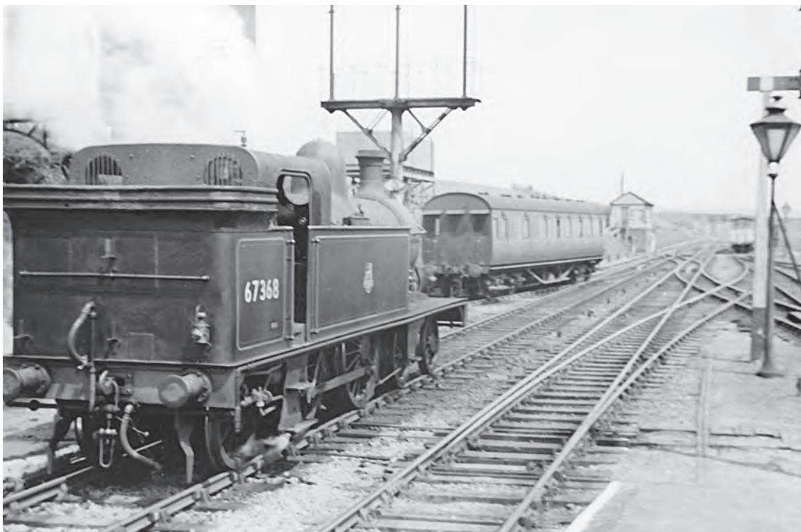
In Three Counties (the title given to this image by M.E. Kirk) on 13 May 1953. On the LNWR Seaton-Uppingham branch from where passenger services were withdrawn in June 1960 and the line closed to all traffic in 1964. Here, the 11.10am Seaton to Uppingham train composed of Ivatt 4-4-2T Class 'C12' No. 67368 and push-pull trailer still in LMS livery waits to depart. Built in 1900 at Doncaster Works, this locomotive was scrapped there when withdrawn in October 1955 from Peterborough (Spital Bridge) shed. (M.E. Kirk/Martyn Reeve Collection)
