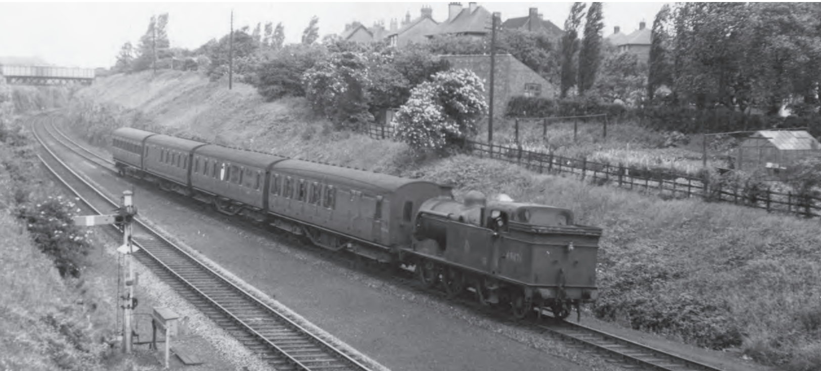
The 10.40am (SO) Edwinstowe-Nottingham (Victoria) local train entering Hucknall Central station on the Great Central line with Ivatt 0-6-2T Class 'N1' No. 69476 in charge on 26 June 1954. Built in 1912 at Doncaster Works, it was scrapped there when condemned from Colwick shed in March 1955. The station was closed on 4 March 1963 along with most other local stations on the line. ( M.E. Kirk/Martyn Reeve Collection )
