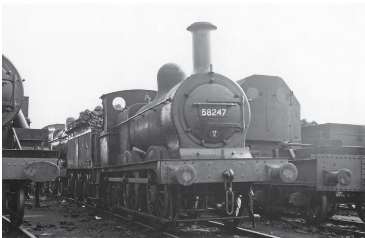
Johnson 0-6-0 Class '2F' No. 58247 is ready to go back into traffic in May 1956 after a visit to the adjacent Works. Built in 1887 at Derby Works, it was scrapped there when withdrawn from Rowsley shed in January 1958. ( M.E. Kirk/Martyn Reeve Collection )
