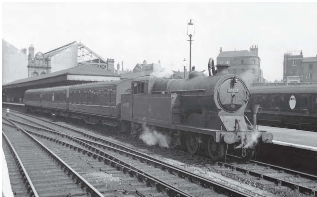
Robinson 4-6-2T Class 'A5' No. 69807 has just arrived at Nottingham Victoria station on 16 August 1952, working the 10.40am (SO) service from Edwinstowe via Mansfield (Central). Built in 1911 at Gorton Works and condemned in July 1958 from Colwick shed, it was broken up at Darlington Works. (M.E. Kirk/Martyn Reeve Collection)
