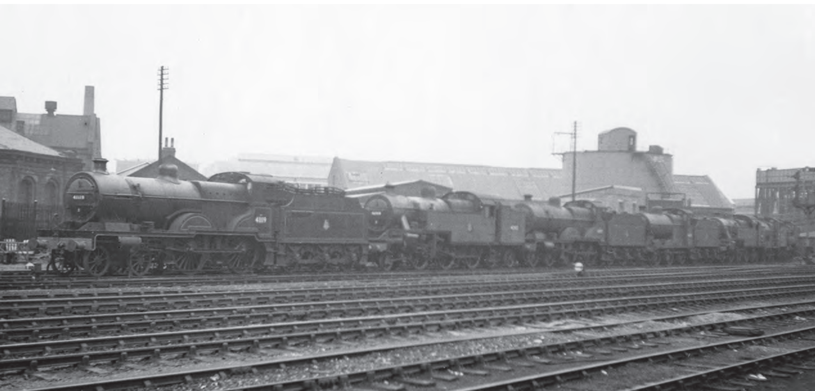
Viewed from platform 6 at Derby station at 8.30pm on 12 June 1955 is a line-up of Fowler locomotives. 4-4-0 'Compound' No. 41119, built in 1925 at Horwich Works and withdrawn from Leeds (Holbeck) shed in December 1958 was broken up at T.W.Ward, Killamarsh. 2-6-4T Class '4P' No. 42410, built in 1933 at Derby Works and withdrawn in September 1966 from Huddersfield shed, was cut up at Cashmore's, Great Bridge. 'Compound' No. 40917, built in 1927 at the Vulcan Foundry and condemned from Bournville shed in December 1956, was scrapped at Derby Works. 0-6-0 Class '4F' No. 44096 built in 1925 by Kerr Stuart, it was condemned in September 1964 from Gorton shed and disposed of at Cohens, Ickles. In the rear is Fowler 2-6-4T No. 42347 & Fowler No. 44560, ex-Somerset & Dorset Joint Railway. (M.E. Kirk/Martyn Reeve Collection)
