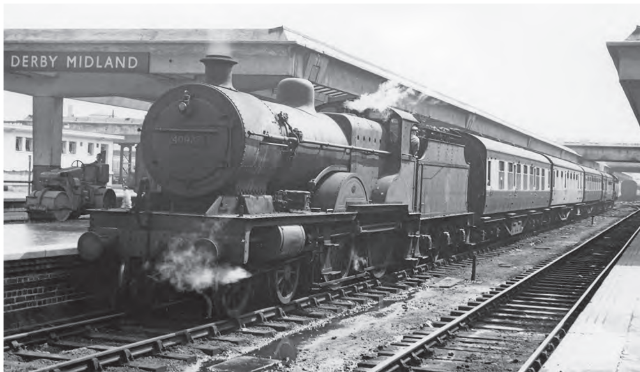
The 5.15pm Derby to Worcester (Shrub Hill) stopping train with Midland 4-4-0 Class '2P' No. 40511 in charge simmers gently on platform 4 on 12 May 1956. Built in 1899 by Sharp, Stewart and Company and withdrawn in January 1961 from Toton shed, it was scrapped at Albert Loom, Spondon. (M.E. Kirk/Martyn Reeve Collection)
