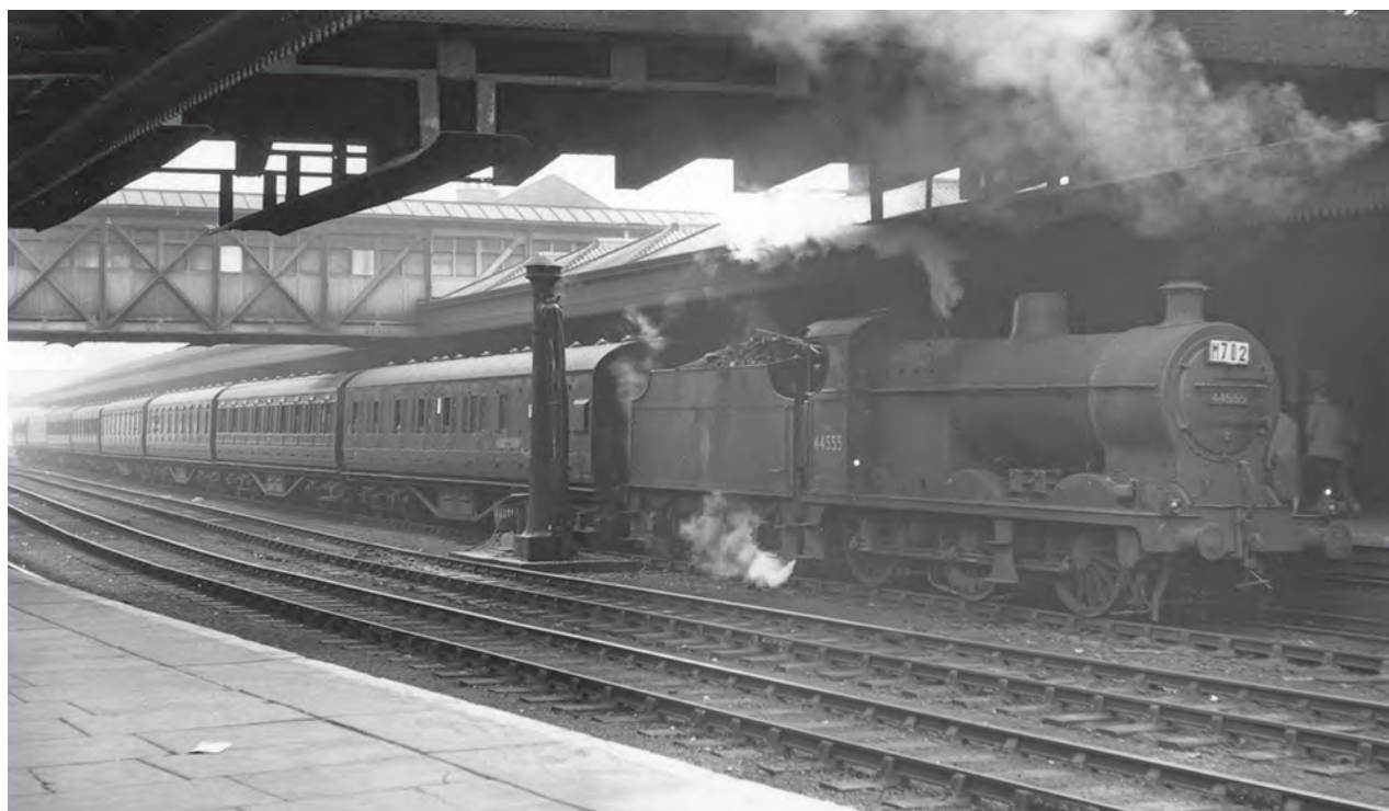
Arriving at Nottingham station on 10 March 1956 with the 2.35pm stopping train from Leicester is Fowler 2-6-4T Class '4P' No. 42342, built in 1929 at Derby Works and disposed of there when withdrawn from Kentish Town shed in June 1962. (M.E. Kirk/Martyn Reeve Collection)
