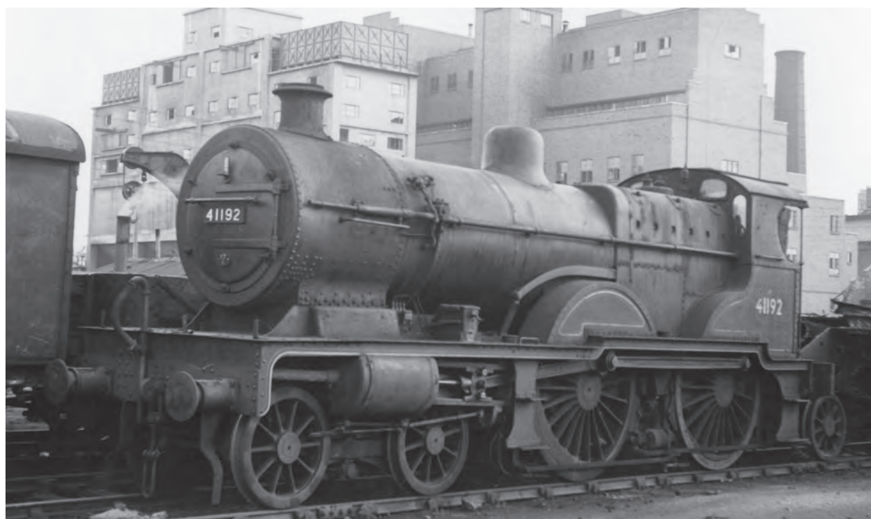
Minus its tender, Compound 4-4-0 No. 41192 is receiving attention on 12 May 1956. Built in 1927 at the Vulcan Foundry, it has only another year in service before withdrawal from Derby Shed and cutting-up at the nearby Works. (M.E. Kirk/Martyn Reeve Collection)
