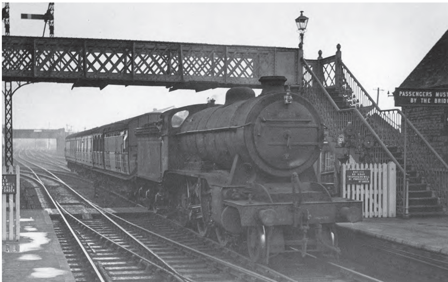
An unkempt Gresley 2-6-0 Class 'K2' No. 61768 is working the 12.42pm Nottingham (Victoria)-Gedling and Carlton local train entering Basford North station on 24 December 1953. Manufactured in 1918 by the NBL Co. Glasgow, it was withdrawn from Colwick shed in January 1959 before being cut up at Darlington Works. The station closed on 7 September 1964. (M.E. Kirk/Martyn Reeve Collection)
