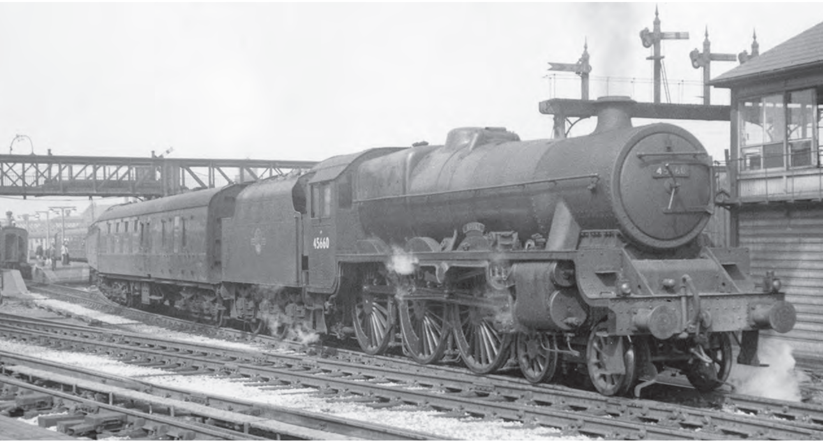
The 12.48pm York-Bristol express leaves the station behind 'Jubilee' 4-6-0 Class '6P' No. 45660 Rooke on 16 May 1959. Built in 1934 at Derby Works and withdrawn from Leeds (Holbeck) shed in July 1966, it was disposed of at Drapers, Hull. (M.E. Kirk/Martyn Reeve Collection)
