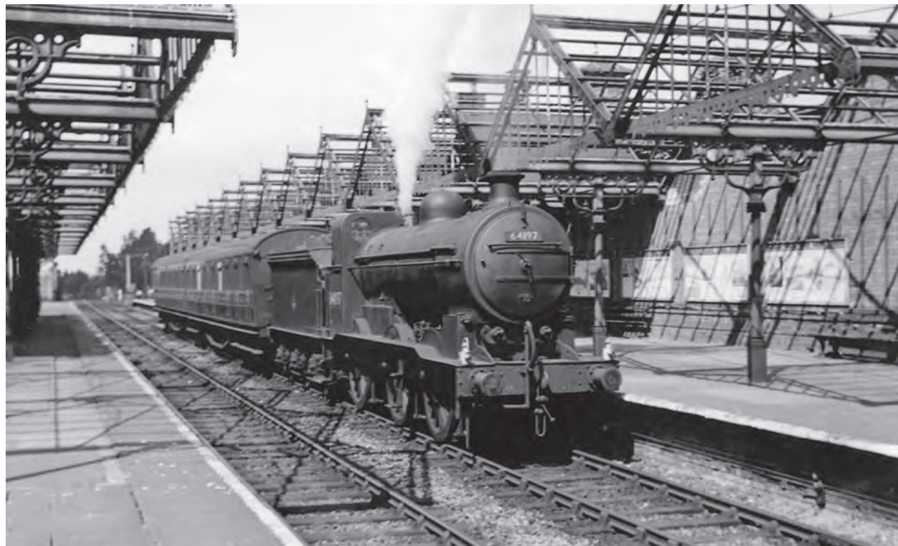
Fowler 0-6-0 Class '4F' No. 44403 is waiting to leave Melton Mowbray (Town) on 19 July 1952 with the 9.05am (SO) Kings Norton-Yarmouth (Beach) and Lowestoft (Central) train. Manufactured in 1927 by North British Locomotive Co. Glasgow, this locomotive was withdrawn from Coalville shed in June 1964 and broken up at Cashmore's, Great Bridge. (M.E. Kirk/Martyn Reeve Collection)
