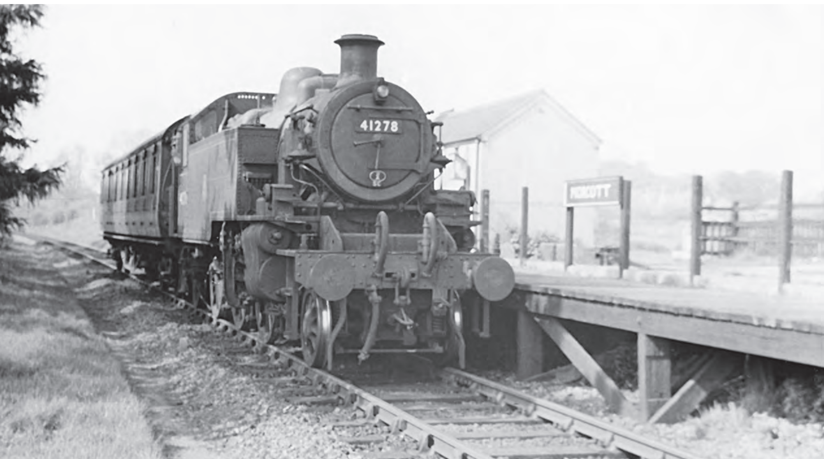
The 9.47am Seaton-Stamford local train is seen here on 13 May 1953 arriving at Morcott station with Ivatt 2-6-2T Class '2MT' No. 41278 providing the motive power. Built in 1950 at Crewe Works, it was broken up there when withdrawn from Llandudno Junction shed after just twelve years in service. Freight services finished on 4 May 1964 and passenger on 6 June 1966. (M.E. Kirk/Martyn Reeve Collection)
