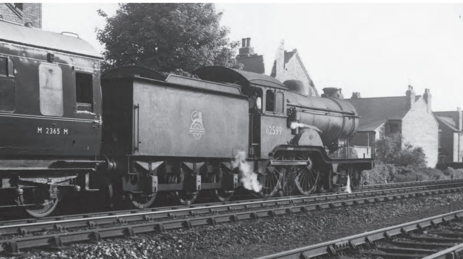
Certainly looking in better condition than some of the Holden 4-4-0 'D16s', No. 62599 is at Carlton & Netherfield on 2 June 1957 heading the 5.30pm Lincoln (St Marks)-Nottingham stopping train. Built in 1910 at Stratford Works, it was disposed of there after being withdrawn from Lincoln shed in September 1958. ( M.E. Kirk/Martyn Reeve Collection )
