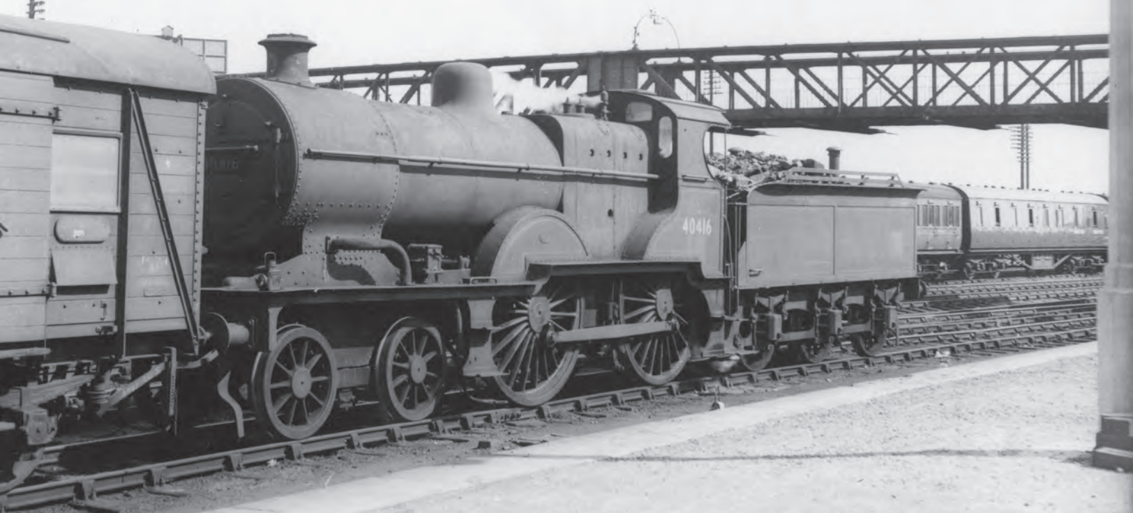
A grimy Johnson 4-4-0 Class '2P' No. 40416 is shown here on station pilot duty at Derby on 2 July 1955. Built in 1892 by Sharp, Stewart and Company, it was withdrawn in May 1959 from Derby shed and disposed of at Crewe Works. (M.E. Kirk/Martyn Reeve Collection)
