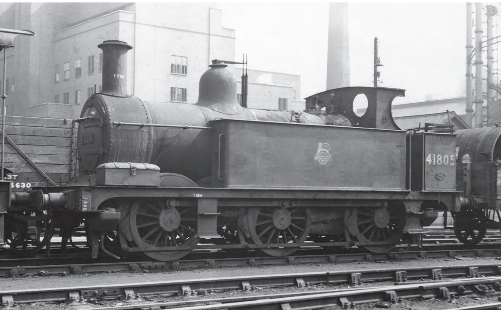
Johnson 0-6-0T Class '1F' No. 41805 , built in 1891 at Derby Works and disposed of there was condemned from Canklow shed in April 1956, a month before this picture was taken. (M.E. Kirk/Martyn Reeve Collection)
