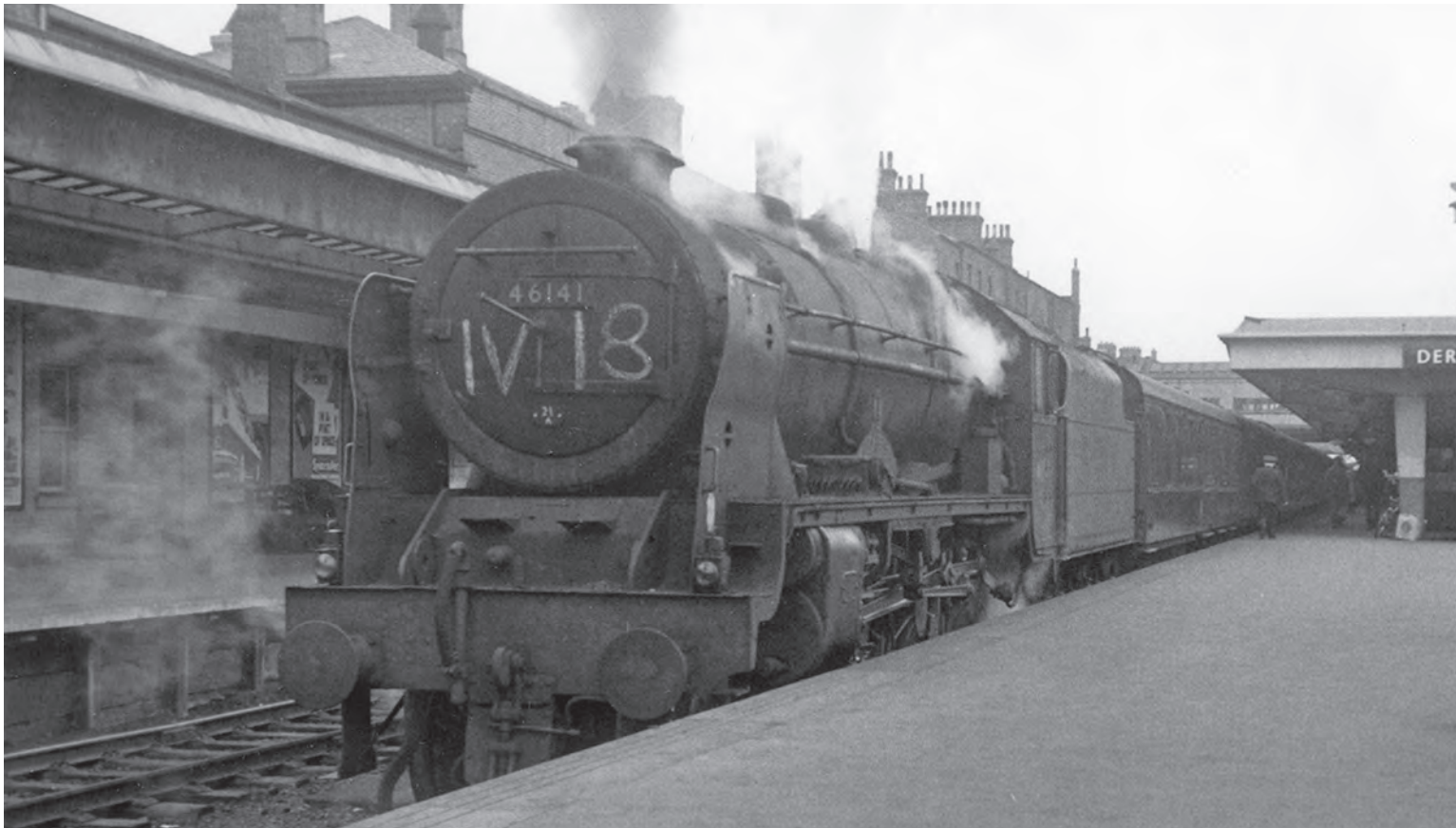
Easing the 7.35am Nottingham-Bristol out of platform 2 is 'Royal Scot' 4-6-0 Class '7P' No. 46141 The North Staffordshire Regiment in May 1962, manufactured in 1927 by the North British Locomotive Co. Glasgow and withdrawn from Carlisle (Upperby) shed in April 1964 and cut up at Crewe Works. (M.E. Kirk/Martyn Reeve Collection)
