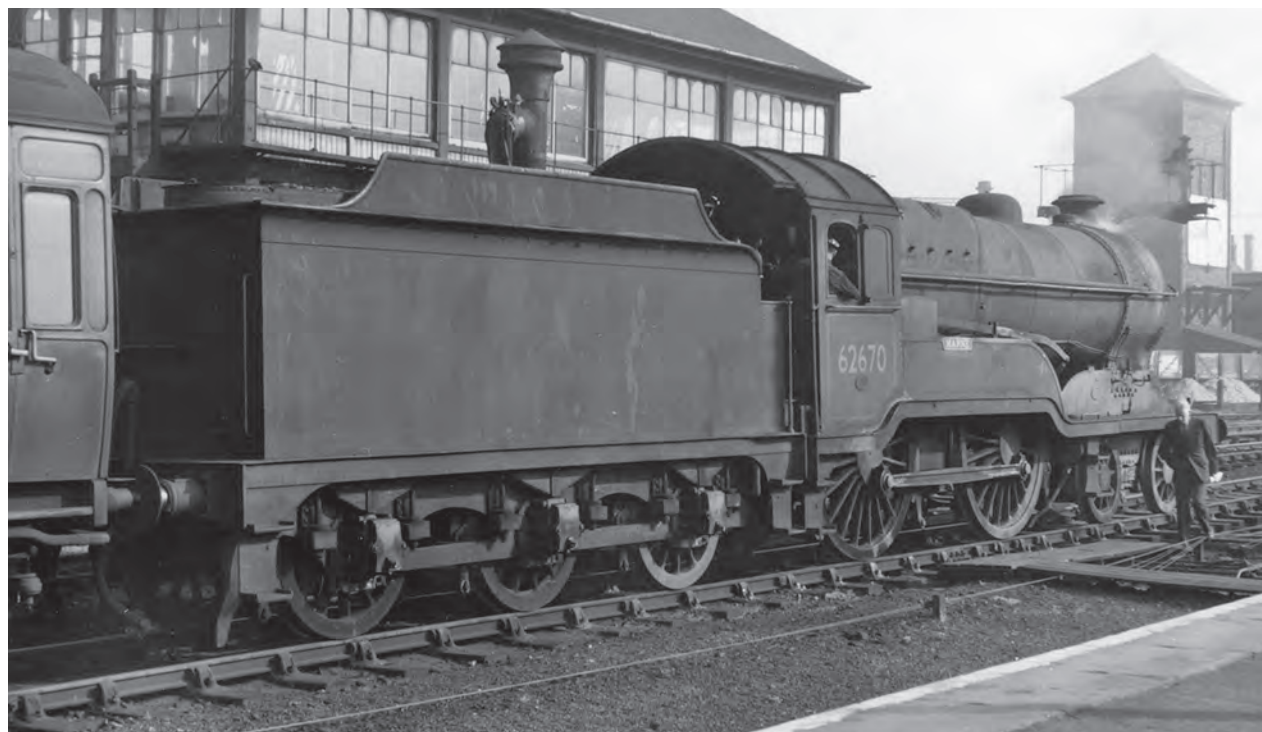
Lincoln (40A) Motive Power Depot must have been short of engine cleaners judging by the condition of Robinson 4-4-0 Class 'D11/1' No. 62670 Marne , bound for Lincoln (St Marks) on 29 September 1956 with a local stopping train. Built in 1922 at Gorton Works and withdrawn in November 1960 from Sheffield (Darnall) shed, it was broken up at Doncaster Works. (M.E. Kirk/Martyn Reeve Collection)
