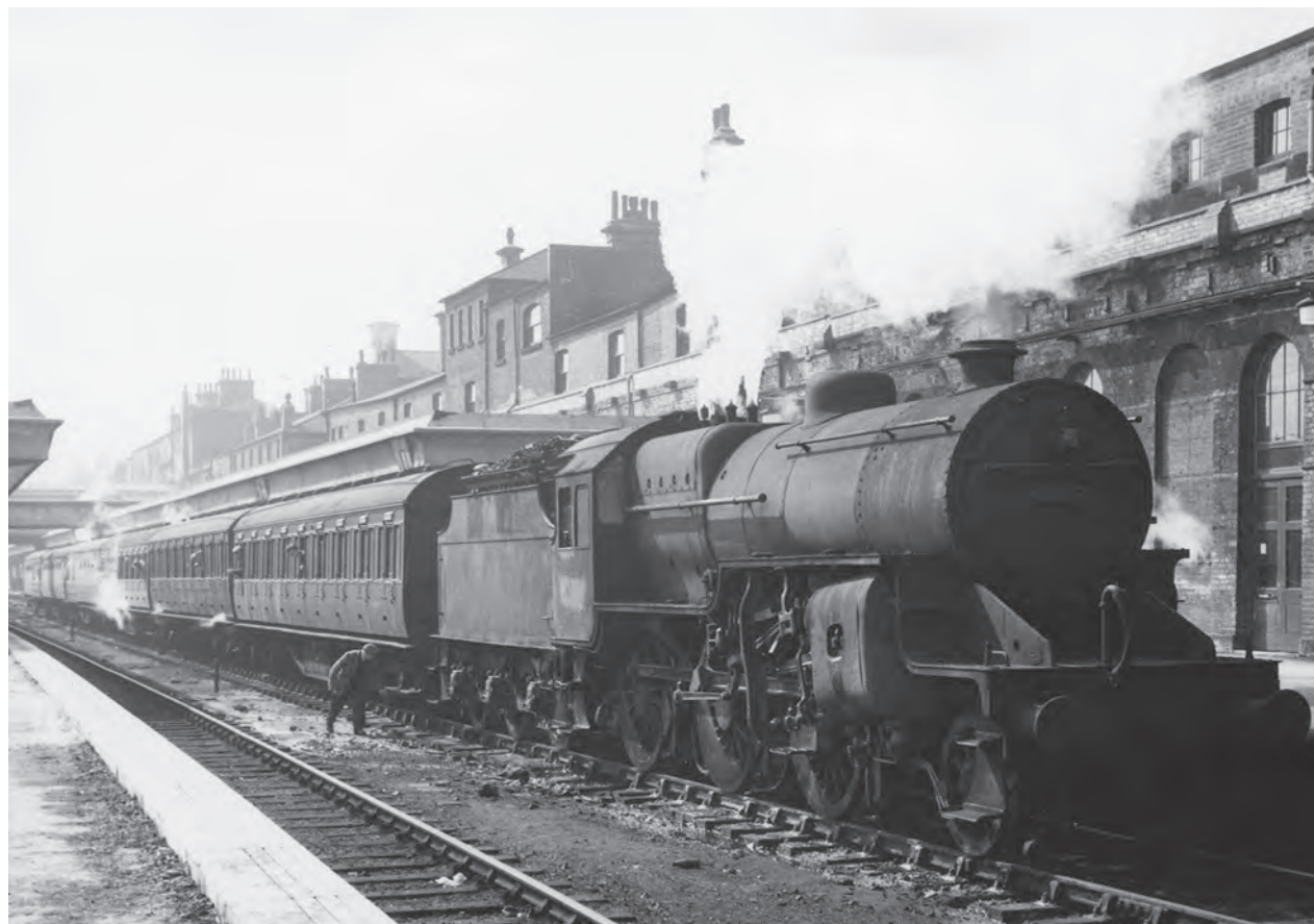
The 10.50am (Sun) Derby to Crewe stopping train waits on platform 2 on 15 April 1956 and is being worked by Fowler 2-6-4T Class '4P' No. 42316. It was built in 1928 at Derby Works and scrapped there when withdrawn from Stockport (Edgeley) shed in February 1963. (M.E. Kirk/Martyn Reeve Collection)
