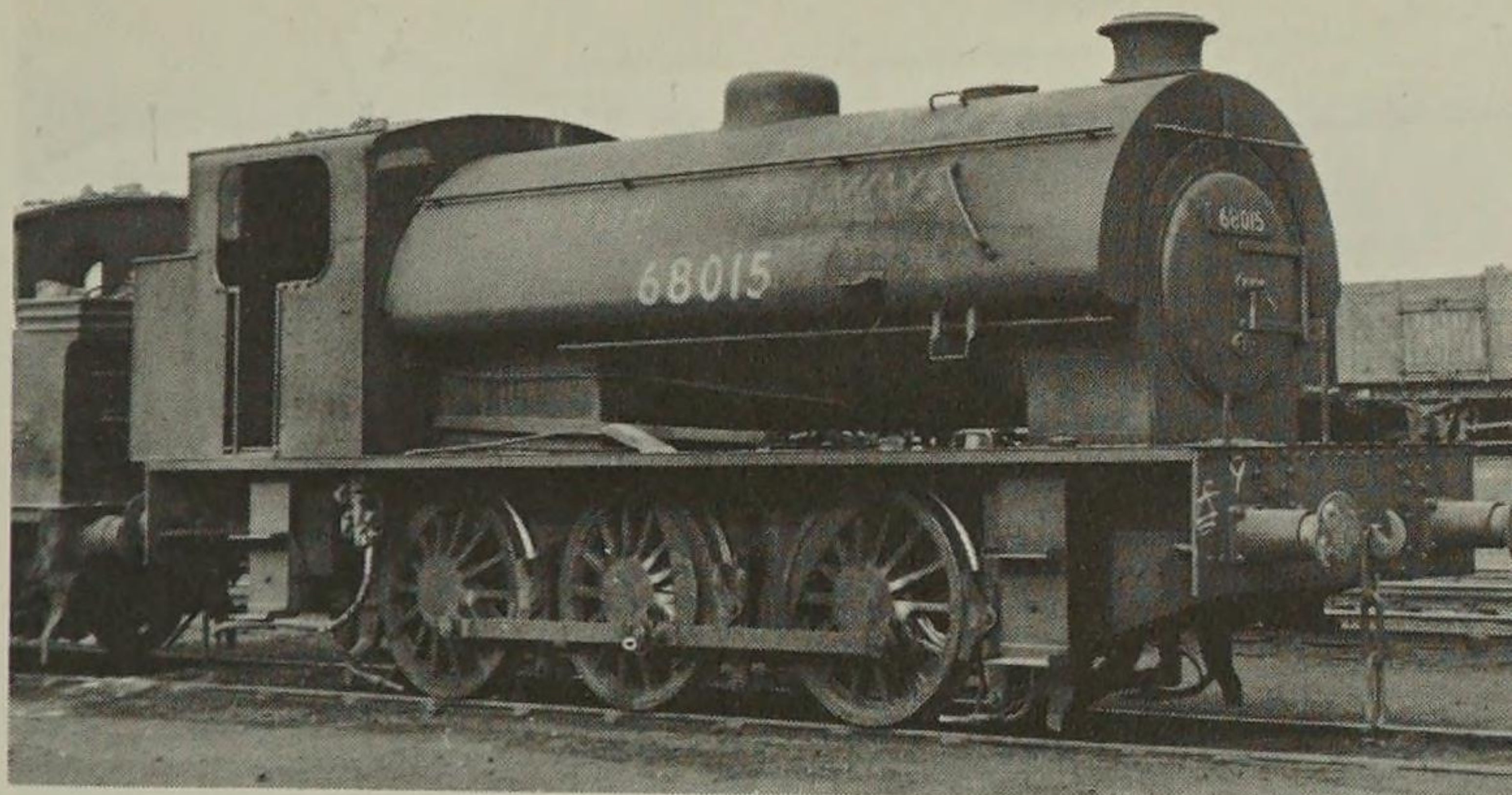
WD design of saddle tank for wartime use. One of the engines subsequently obtained by the LNER
