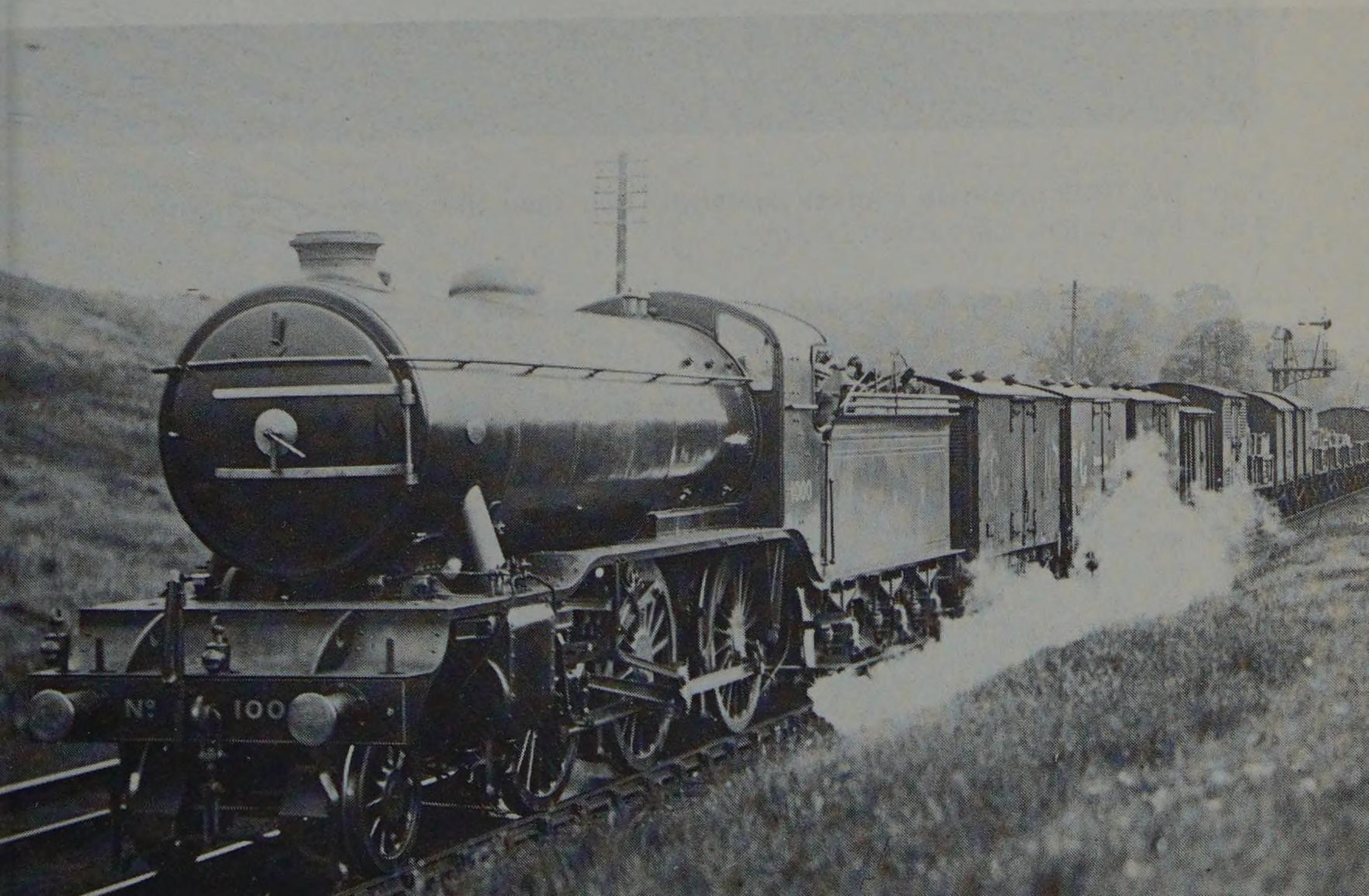
Below: GNR No 1000 at the head of a 75 wagon down goods train in 1920. Indicating equipment is in place on cylinders but the engine is not actually being tested. Locomotive Publishing Co
