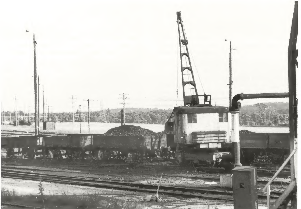
The Hodgkinson three-ton electric coaling crane, a resident at Taree for many years. Similar cranes were used at Gosford, Temora and Eveleigh Depots.
