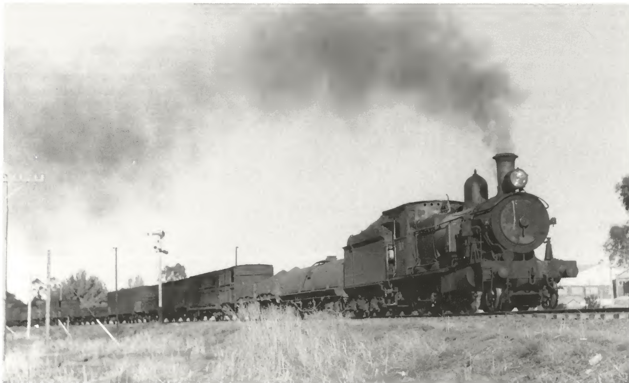
Superheated 30T class locomotive 3131 departs Griffith on No.39 goods (with passenger accommodation) for Hillston and Roto. The bogie water gin behind the tender should ensure that 3131 does not run out of water on the long trip across remote, often windswept, plains with limited watering facilities en route. Thursday, 18 May 1961.
