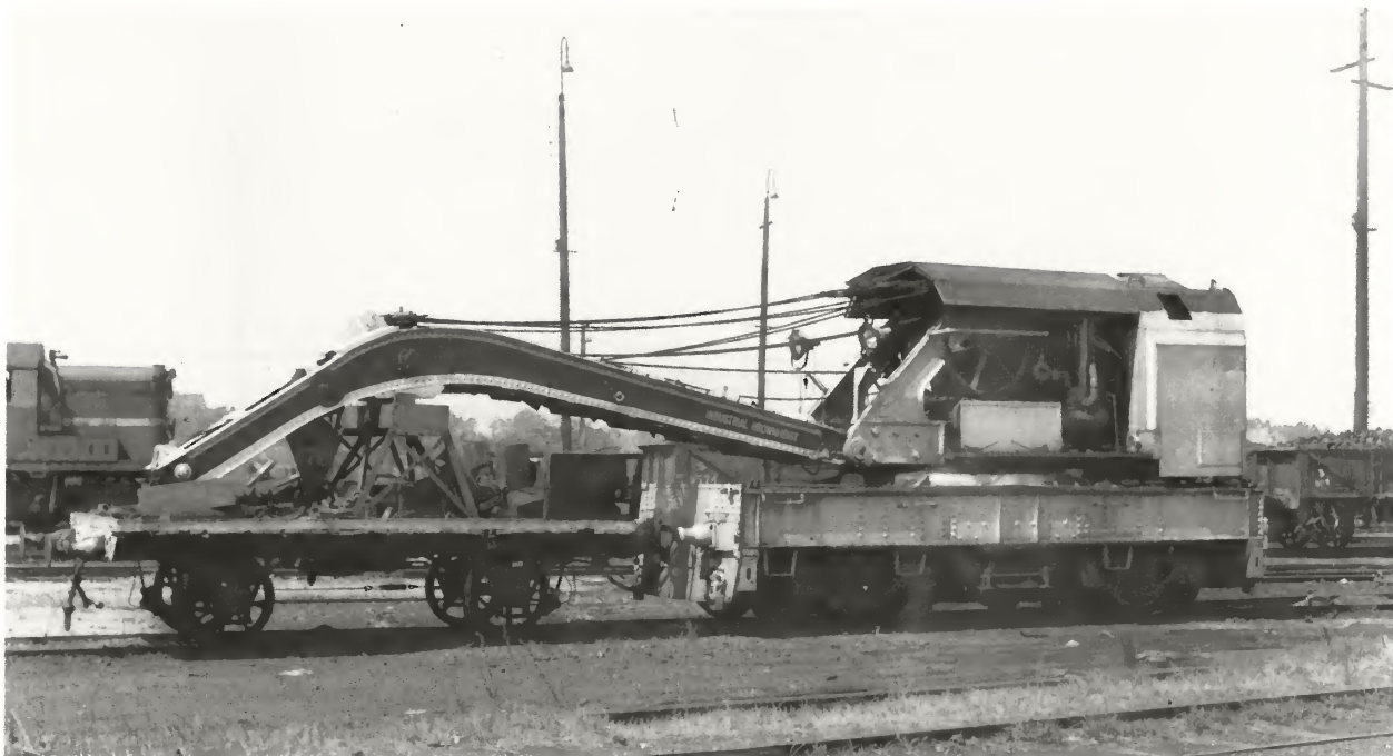
Taree Depot played host to a 50 ton (50.8 tonne) accident crane during the late 1950s and 1960s. Crane 1081, a product of 'Industrial Brownhoist', with its jib support vehicle, is shown at Taree in early 1964. I.Wallace
