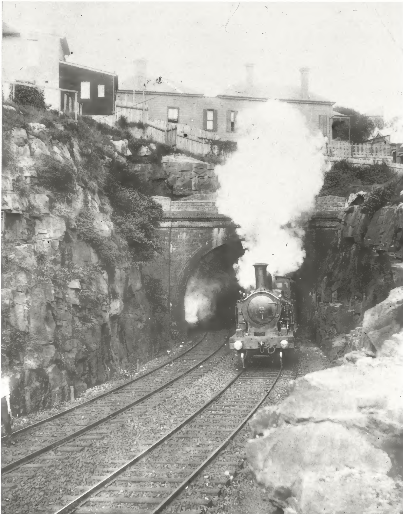
Polished buffers and handrails, and reversed marker lamps distinguish an S class 4-6-4 tank engine as it blasts uphill out of Blues Point tunnel with a down North Shore passenger in 1924. This portion of the original line is now reduced to single track and sees infrequent use as access to the Lavender Bay car sidings. SRA
