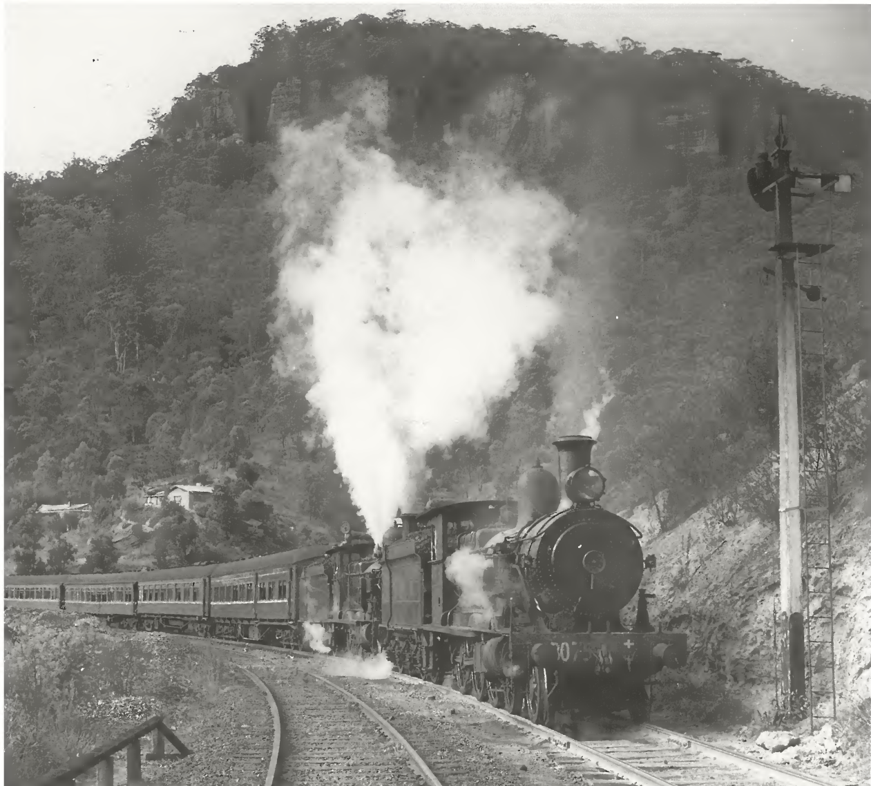
Both water columns are in use to replenish the tenders of a pair of 30T class engines on a northbound tour train. The signal is Brogans Creek's down starter, while the troughing on the left carries wire associated with track circuits.
