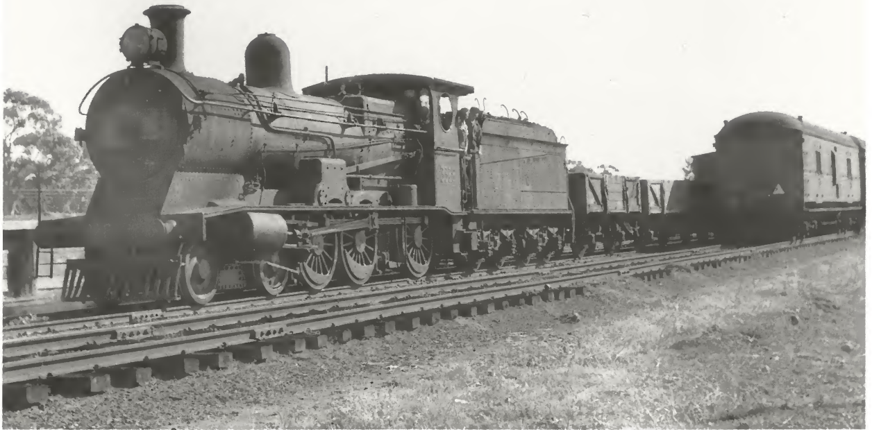
At the head of an up goods, Narrandera based 3328, one of very few P class at the time fitted with a cowcatcher, stands in the loop at Wumbulgal to allow the down Griffith passenger service, hauled by 3082, to cross. The Narrandera P class engines worked over many unfenced lines, thus warranting a cowcatcher. Thursday, 18 May 1961.
