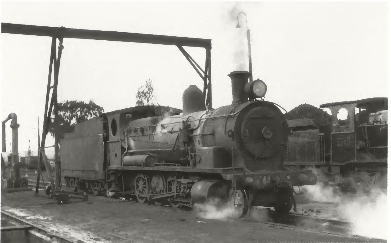
Goulburn-based 5444, fitted with specially balanced driving wheels, denoted by the 'X' on the front buffer beam, stands outside the shed at Cootamundra loco on Wednesday, 17 May 1961. 3345 lurks behind 5444 and the jib of Cootamundra's steam coal grab 1058 is in the background, on left of photo.
