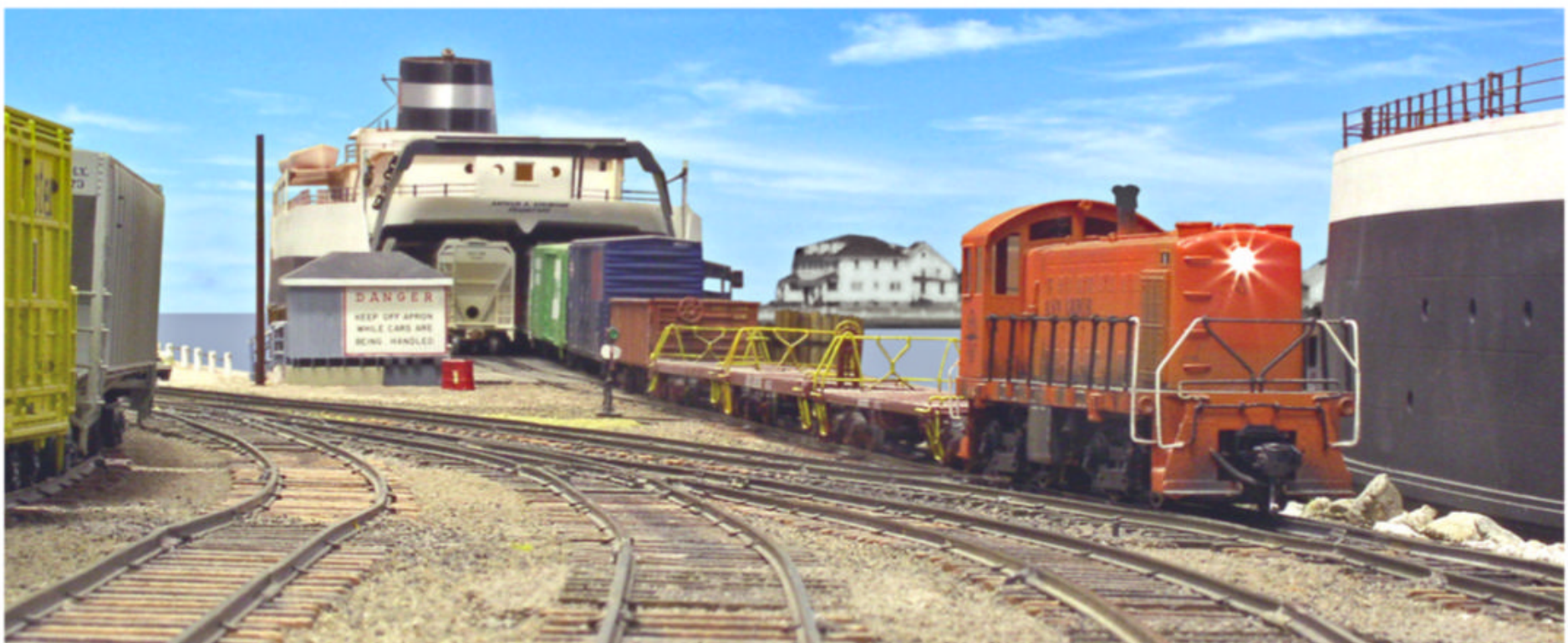
Ann Arbor Alco S-3 no. 6 employs idler flats to switch cars on and off the car ferry Arthur K. Atkinson at the East Slip in Betsie Lake at Frankfort/Elberta, Mich. The Alco has to struggle to pull an entire 12-to-15-car cut at one time. [Arnt Gerritsen's Ann Arbor RR]
