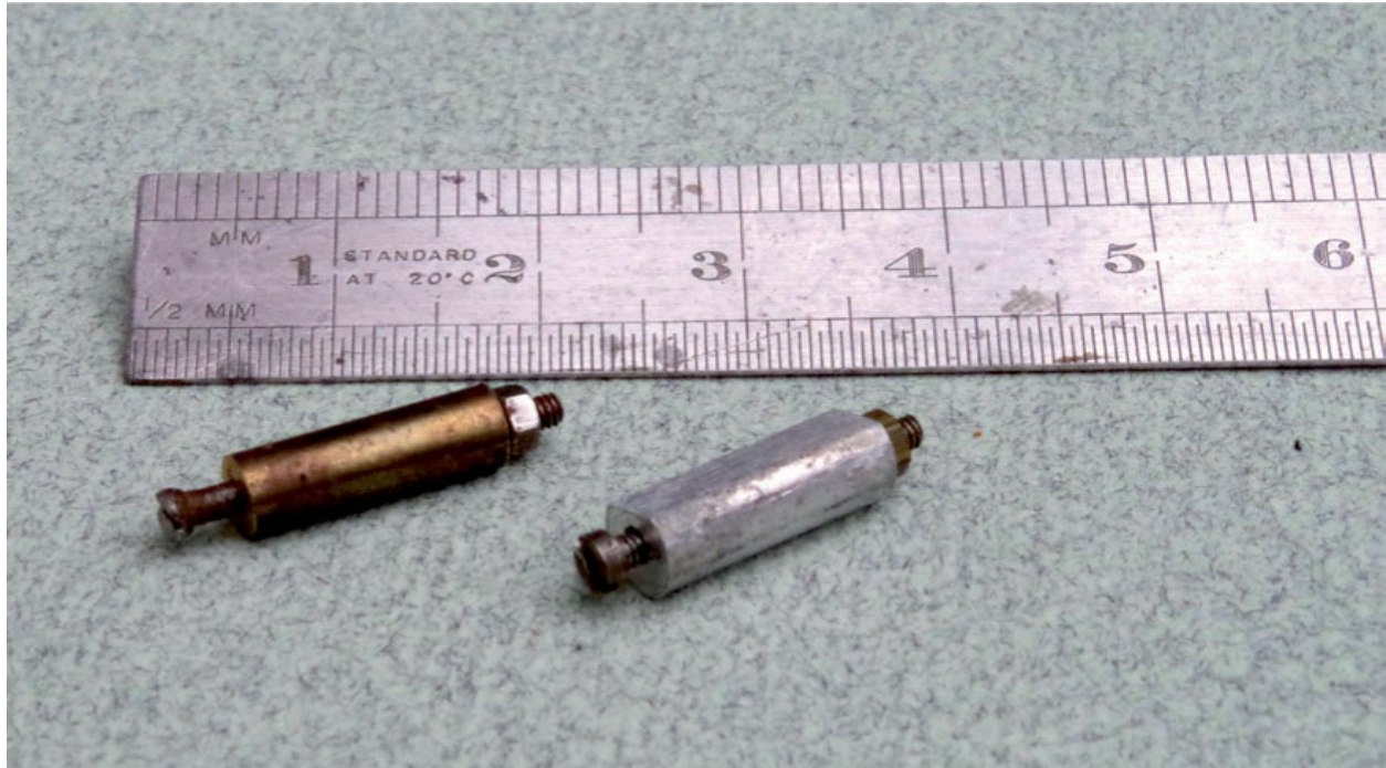
Frame spacers used for chassis construction.
