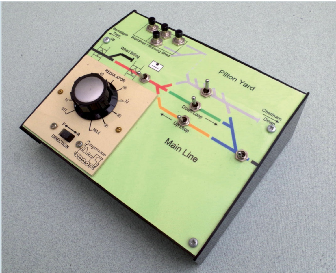
Cab control panel for a 009 layout. The grey yard area is being controlled locally (switch 'up'), the green Down loop is isolated (switch 'centre') and the blue, yellow and red sections (switches 'down') are allowing another operator to drive a train straight through the Up loop.
