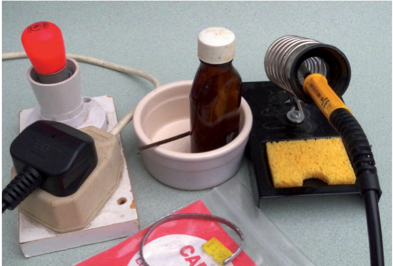
The various items needed for low melting-point soldering. The glowing bulb shows that the iron will reach a suitable temperature for whitemetal.
