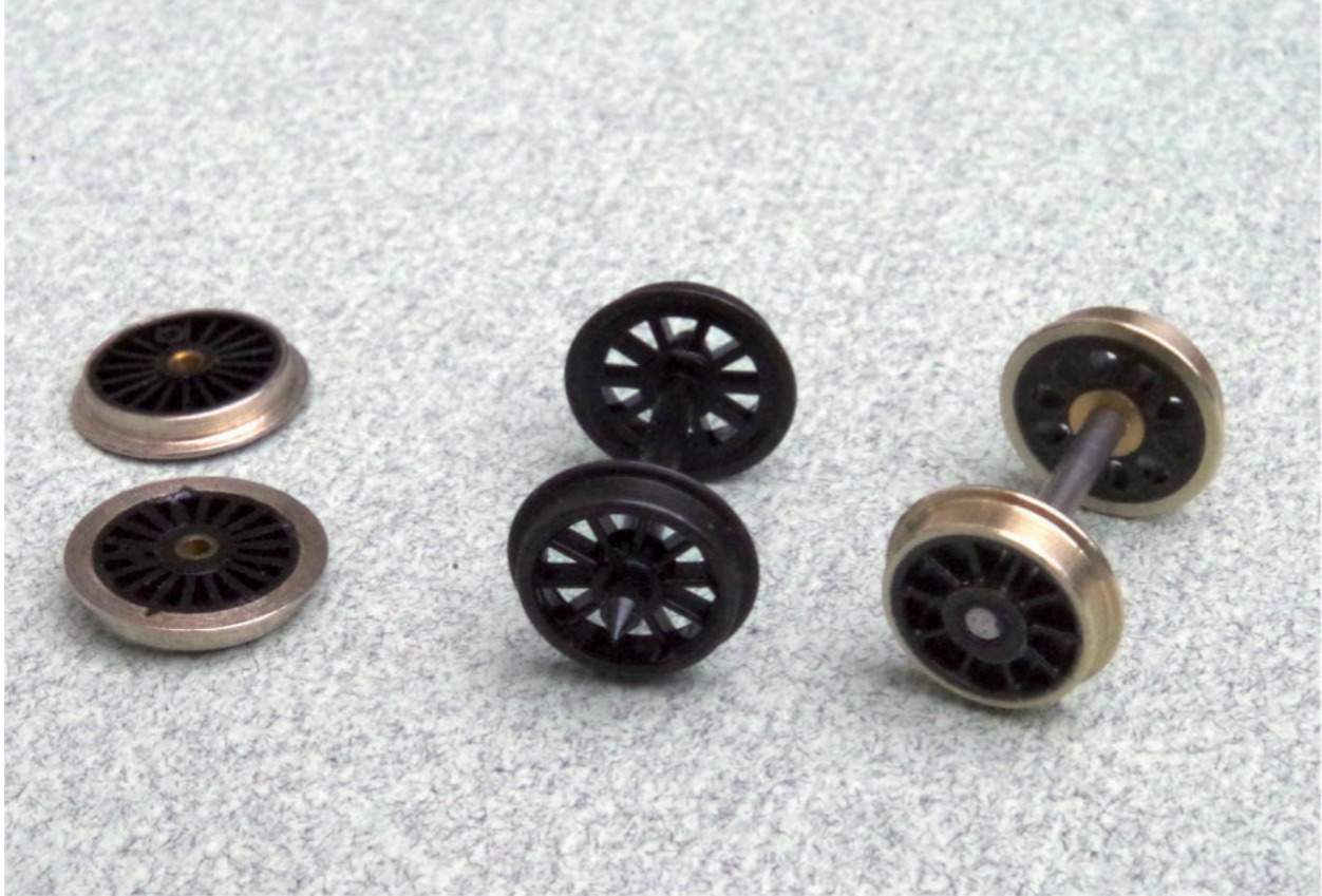
Driving wheels suitable for 009 locomotives. Those on the left are intended for N gauge locomotives, the remainder are 4mm/1ft scale bogie/wagon wheels.
