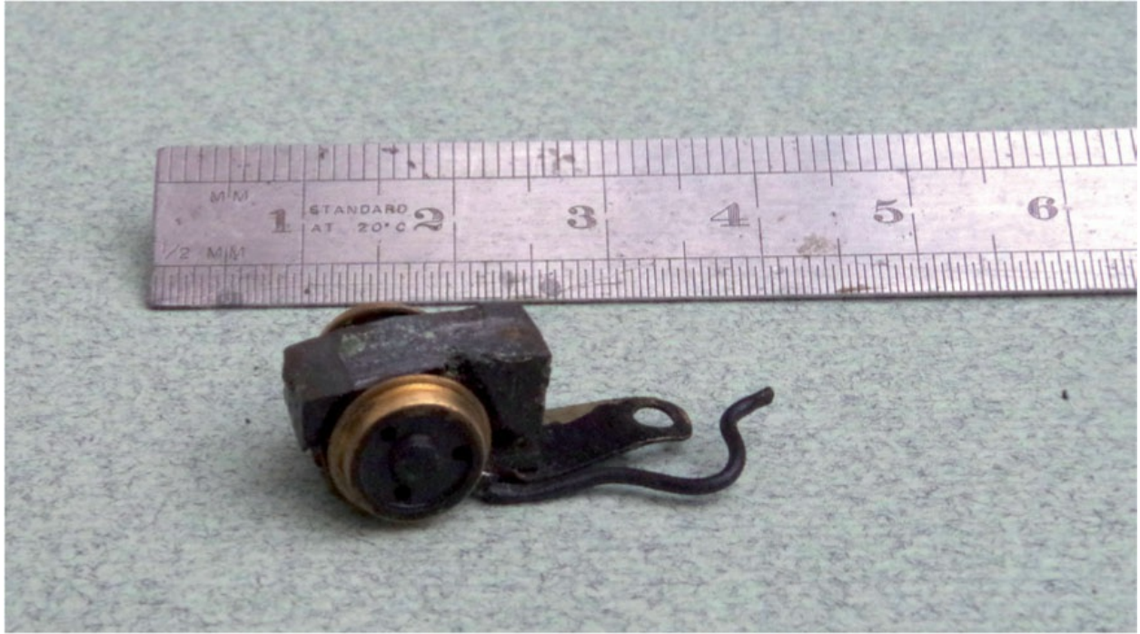
View of an inside-framed split-axle truck made by the method described.
