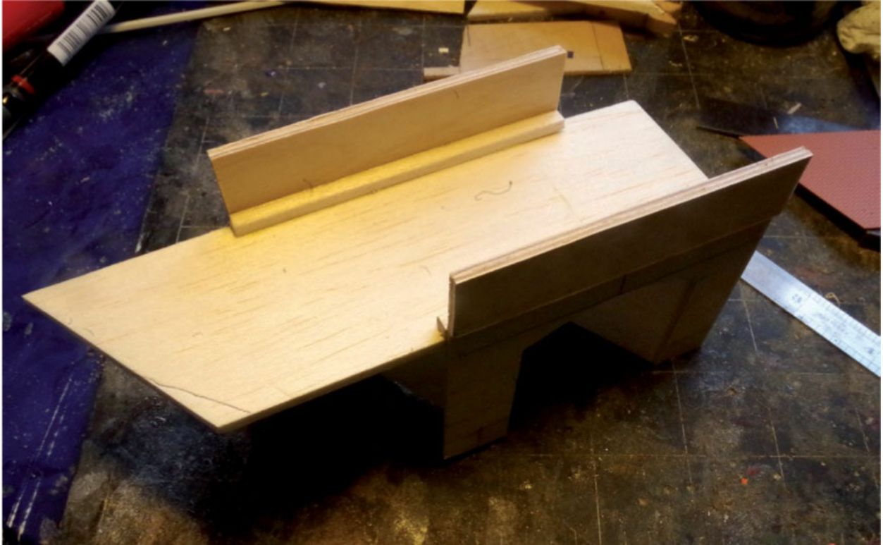
The skeleton of the bridge from above. Separate strips of brick-embossed styrene form the courses of bricks that stand proud of the surface.
