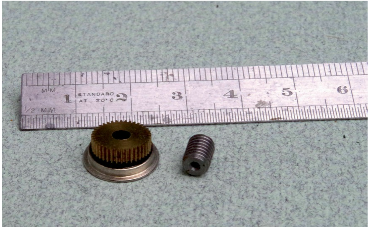
An 11mm driving wheel with a 38:1 worm gear set, illustrating the practical limit on worm gear ratio for 009. This might just work, but with any smaller wheels it would not.
