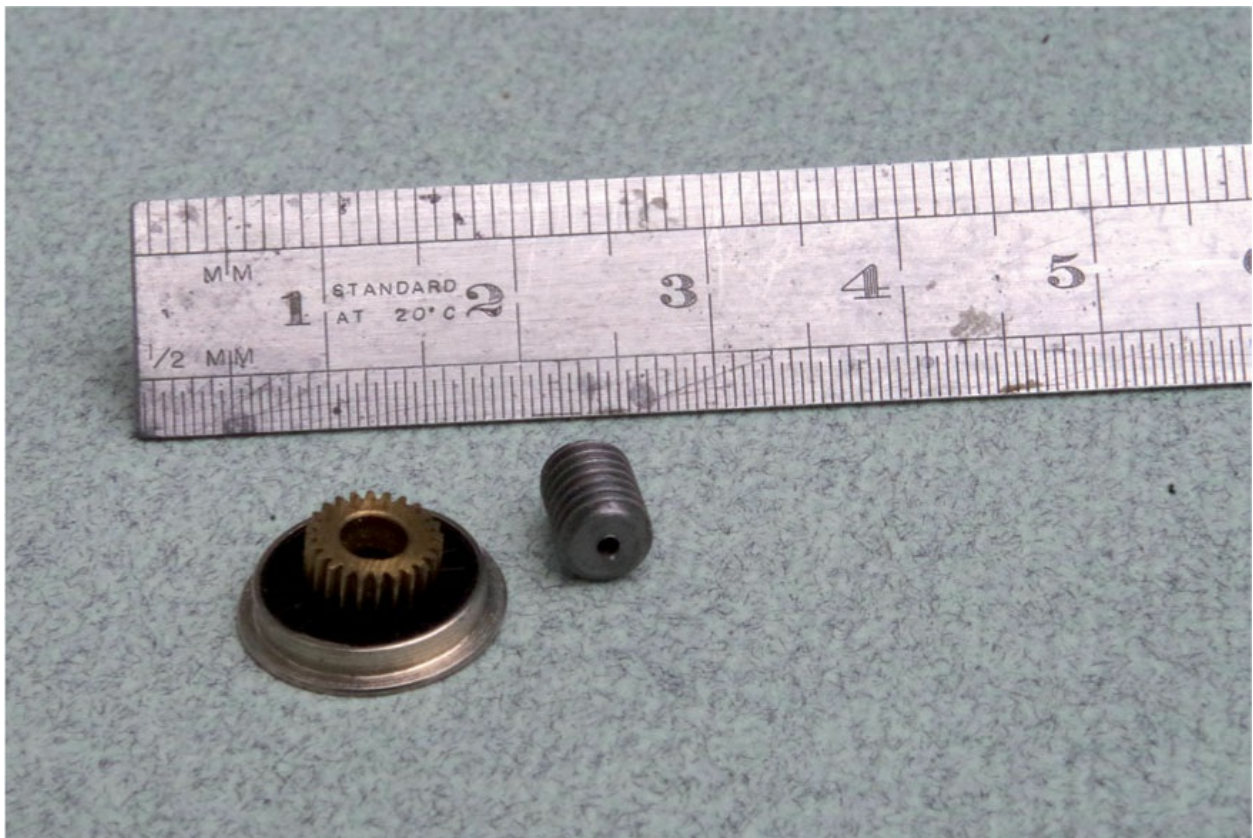
An 11mm-diameter driving wheel shown with a 24:1 worm gear set. This is clearly feasible.
