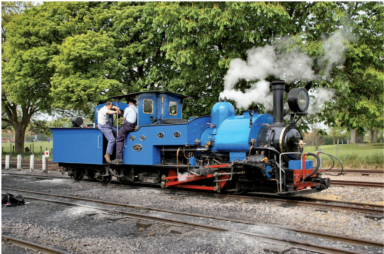
Another powerful 2ft gauge locomotive, this outside-framed 0-4-0ST from the Darjeeling Himalaya Railway has its Walschaert's valve gear readily accessible.
