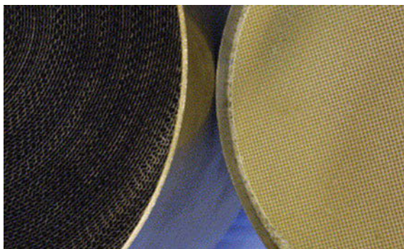
Fig. 3 Diesel oxidation catalysts (Adapted from Ref. [37])
