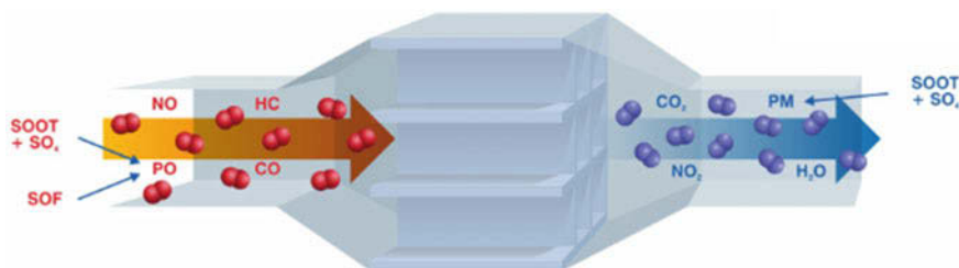
Fig. 3 Schematic of a diesel oxidation catalysts
