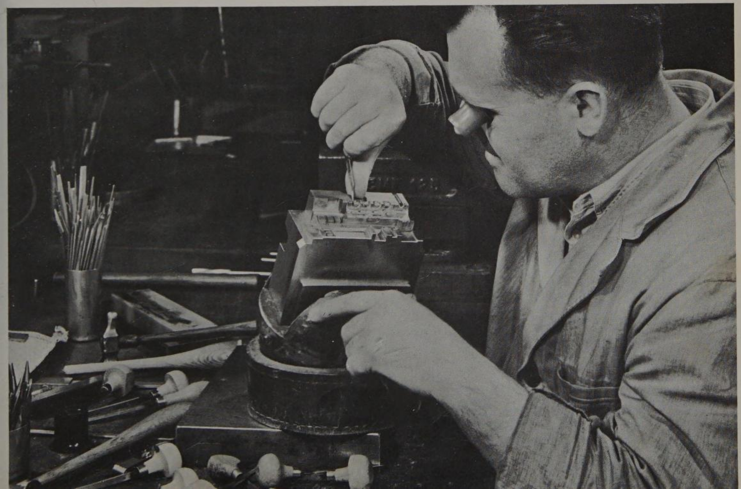
101 An engineer in the Märklin factory making a die.
