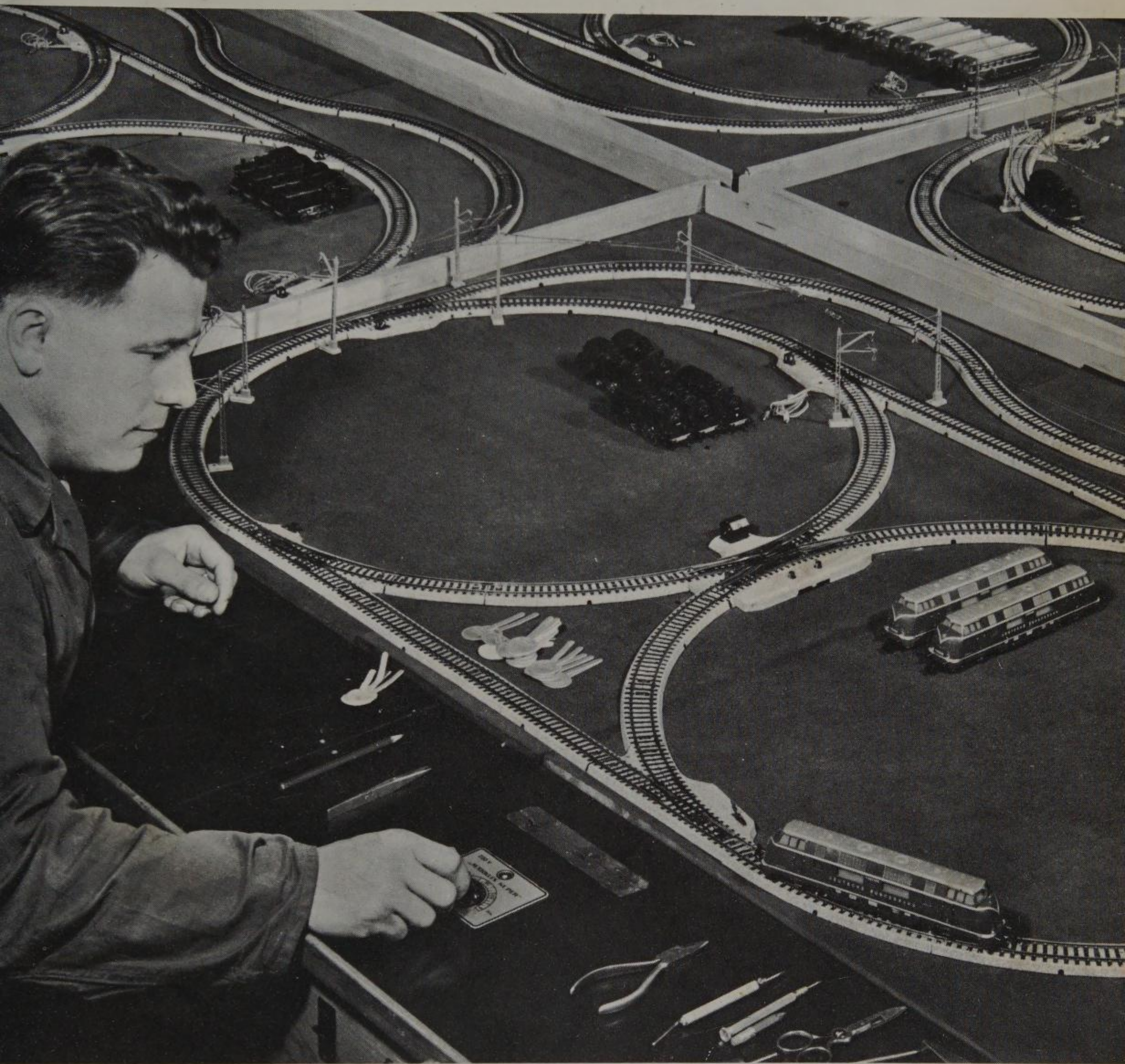
56 A technician in the Märklin factory testing model locomotives that have come off the production line.
