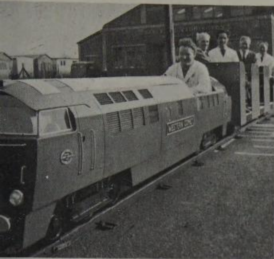
202 Typical of many modern miniature railways, this is a 10\frac{1}{4} in. gauge 'Western' class diesel locomotive pulling articulated trucks (cars). It is powered by a Ford 1,600 c.c. cross-flow engine.
