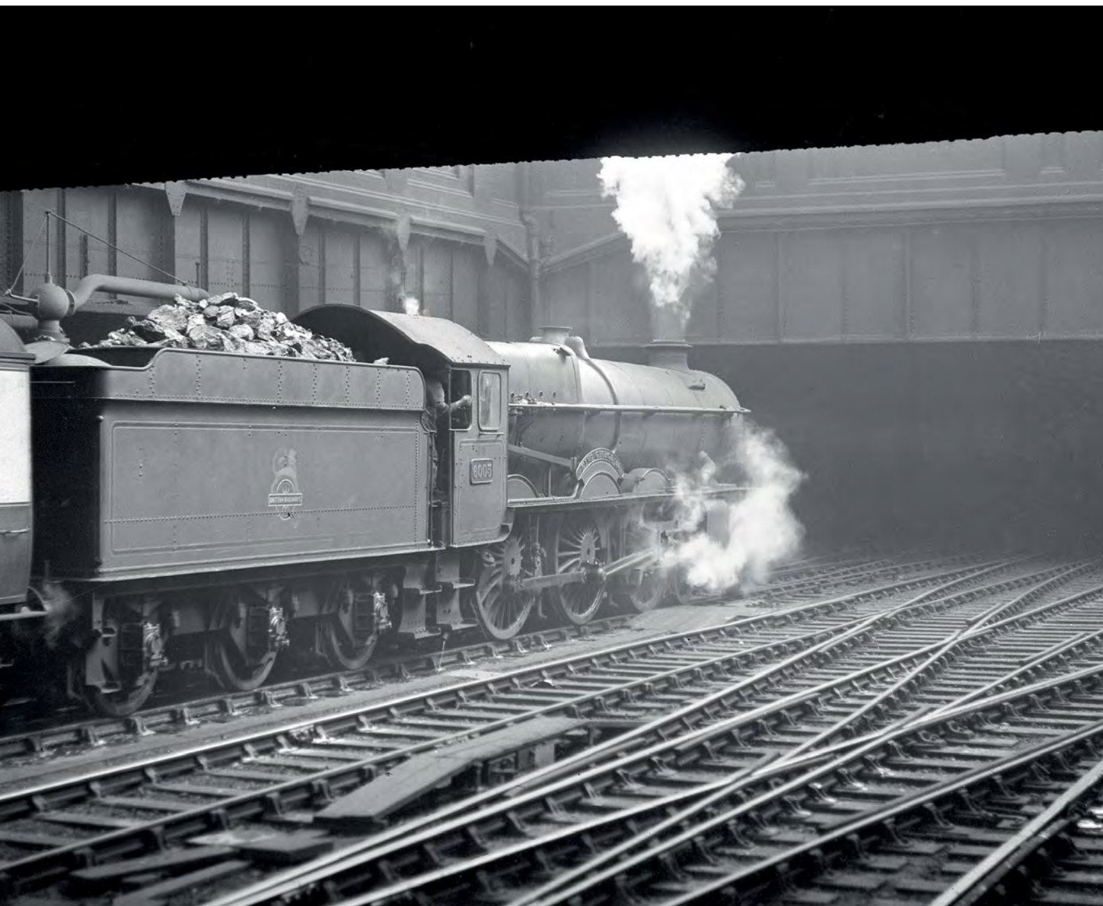
By standing at the end of Platform 6 at Birmingham's Snow Hill station spotters had an excellent view of trains approaching from the north and Stourbridge as they passed the timber-built elevated North signal box, seen in this view as Banbury-allocated ex-GWR 'Grange' class 4-6-0 No 6879 Overton Grange approaches with a southbound freight train. Beyond the brakevan on the right we see the large water tank. Kidderminster Railway Museum I23036
