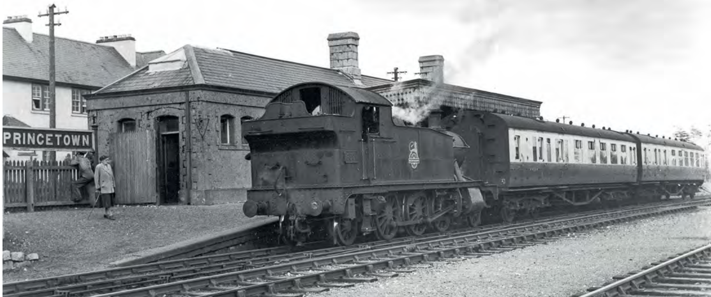
Passenger trains over the Princetown branch over Dartmoor to and from Plymouth continued to run until March 1956, and on 29 October 1955 2-6-2T No 4591 is pictured at the Princetown terminus with its two coach train. Until 1955 the '4400' class 2-6-2Ts worked the trains over the line, but these were replaced by the '4500/4575' class 2-6-2Ts as the '4400s' were restricted to 120tons (four coaches) between Yelverton and Princetown. Rex Kennedy Collection
