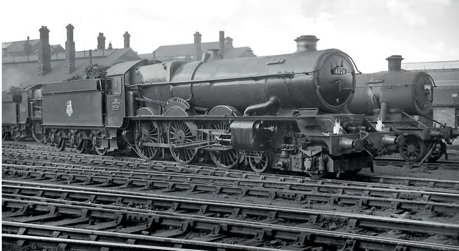
The last 'King' to be rebuilt with a double chimney and blastpipe was No 6026 King John , seen here on Swindon shed on 16 June 1953 after receiving a Heavy General repair. Behind No 6026 is the penultimate '2884' class 2-8-0 to be put into traffic, No 3845, and 'Star' class 4-6-0 No 4062 Malmesbury Abbey . When withdrawn from Old Oak Common in July 1962, King John had run an estimated 1.6million miles in 32 years. R.C. Riley/Transport Treasury
