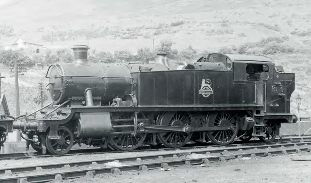
The '5700' class 0-6-0PT No 9671 (built 1948, weight 50tons) is seen here pulling out of Taunton station with an empty coaching stock train on 16 June 1959. With the completion of No 6779 in December 1950, originally introduced in 1929 the '5700' class of 0-6-0PTs finally totalled 863 locomotives, of which 613 had been built at Swindon Works and 250 by no fewer than six private builders. It therefore narrowly exceeded the 857 L&NWR 'DX' class 0-6-0s built between 1858 and 1874 by Crewe Works, which also built 86 engines of the same design for the Lancashire & Yorkshire Railway. K.L. Cook/Rail Archive Stephenson
