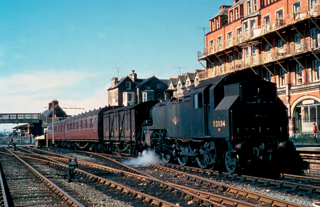
BR Standard '3MT' 2-6-2T No 82034 waits in the excursion platform at Barmouth with a local working to Dolgelley in the summer of 1964. Released to traffic in January 1954 it has carried lined-green livery since September 1958. Allocated to Machynlleth between April 1961 and April 1964 it was to be found on local passenger work as well as on goods trains, and at busy times could also be seen on pilot duties over Talerddig bank. Arguably from one of the most attractive of the Standard classes, No 82024 was withdrawn in December 1966 from Patricroft shed. Colour-Rail.com
