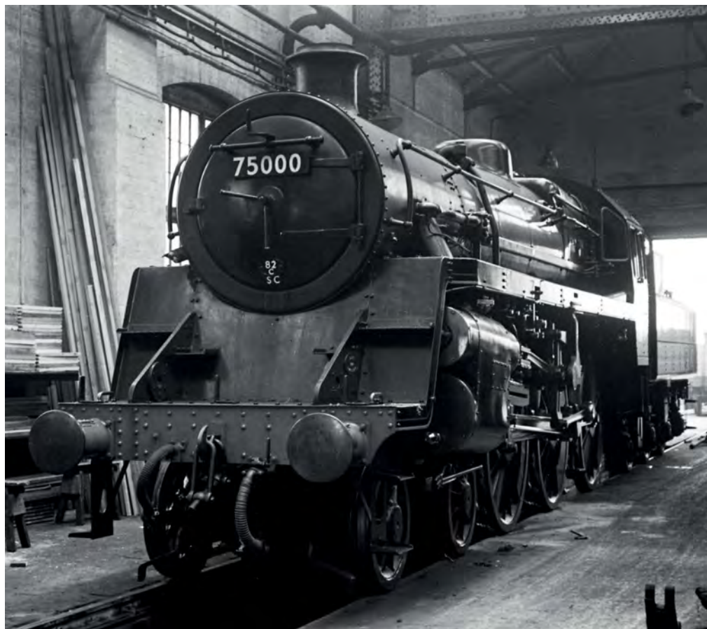
The first BR Standard locomotive to be completed at Swindon Works, in May 1951, '4MT' 4-6-0 No 75000, is pictured at Swindon on 29 May of that year. The '4MT' 4-6-0s had more than their fair share of teething troubles before settling down to become one of the success stories of the Standard locomotives. No 75000 itself suffered a seized tender wheel-set on a test run and had to be returned to the Works for remedial action. The locomotive was retained at Swindon for testing purposes before being sent to Shrewsbury in September 1951. Withdrawal came in December 1965 from Worcester shed. Colour-Rail.com/10995
