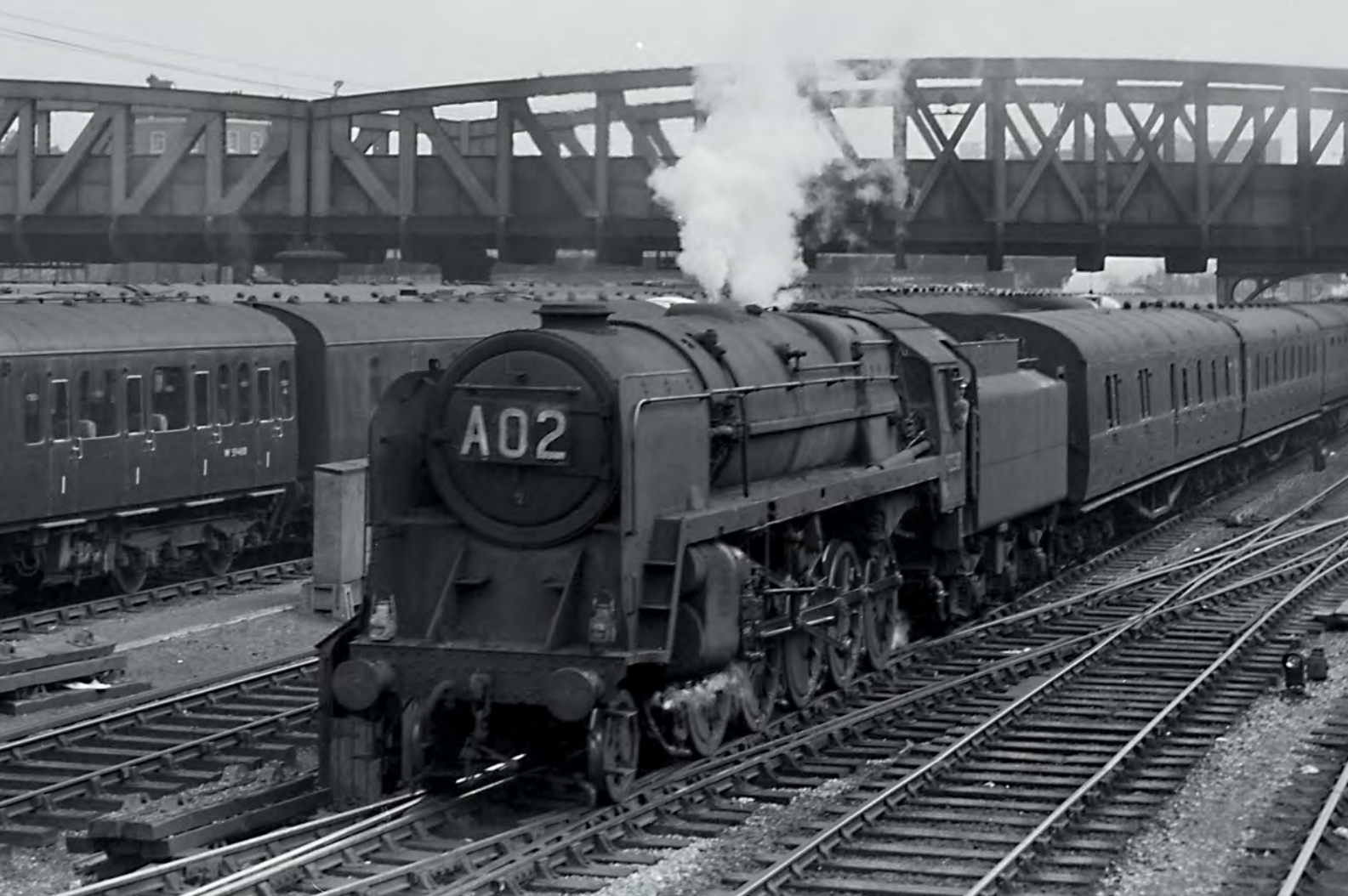
During the summer of 1964, BR Standard '9F' 2-10-0 No 92220 Evening Star , the last steam locomotive to be built at Swindon Works, carrying a Cardiff East Dock shed plate, stands at Oxford at the head of a goods train. It is hard to believe that under the grime and limescale is a lined-out green passenger livery and a copper-capped chimney. Entering traffic in March 1960 at Cardiff (Canton) shed No 92220 ended its working life at Cardiff East Dock after spells at Old Oak Common, Oxford, and Bath (Green Park). Joe Richardson/Colour-Rail.com
