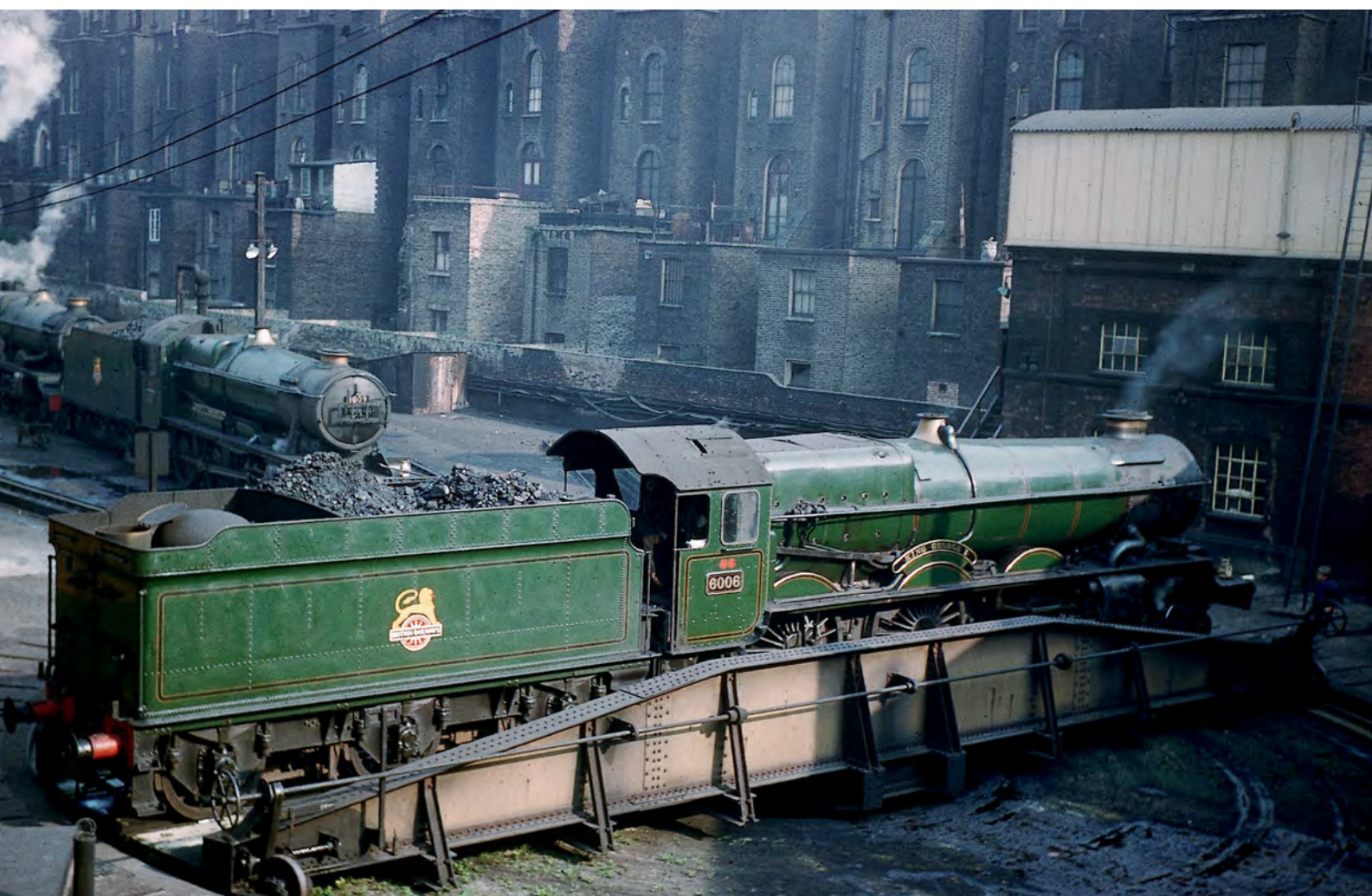
The low angle of the sun on 30 March 1957 highlights 'King' class 4-6-0 No 6006 King George I , now fitted with a double chimney, as it is turned at Ranelagh Bridge depot prior to working back to Wolverhampton later in the day. In the background is 'County' class 4-6-0 No 1009 County of Carmarthen and an unidentified 'King' which have already been turned and serviced and are waiting to back down to Paddington to pick up their respective down workings. R.C. Riley
