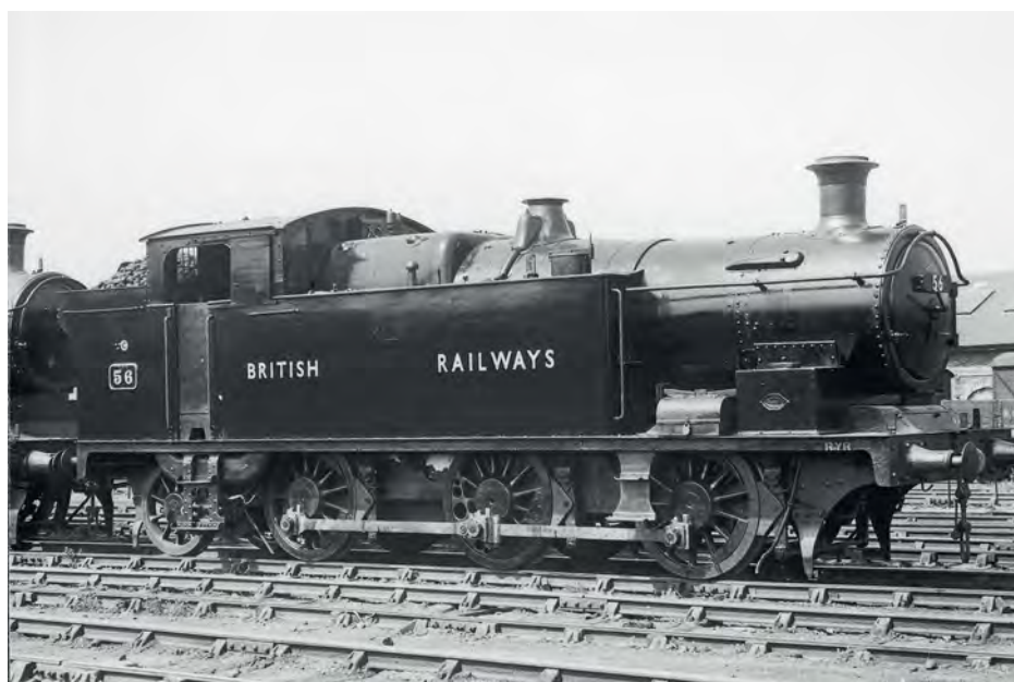
Sporting the BRITISH RAILWAYS legend on its tank sides, former Rhymney Railway 'A' class 0-6-2T No 56 is seen on shed at Cardiff (Cathays) in June 1949. Enthusiasts visiting Cathays shed at that time were often amazed at how clean they kept their locomotives; it was originally a Taff Vale Railway depot. Designed by Hurry Riches, by 1948 all those engines of the class entering BR service were fitted with either 'A1' boilers or GWR boilers.
