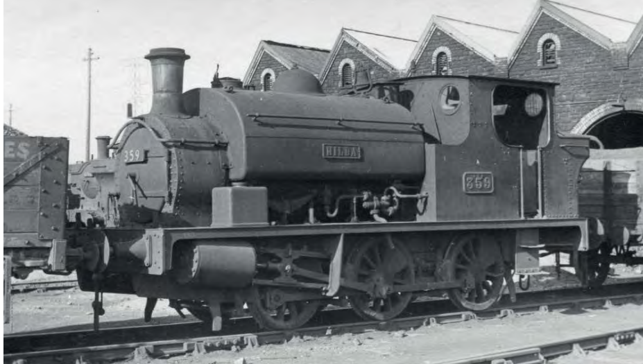
Two locomotives of the former Llanelly & Mynydd Mawr Railway reached BR days in service, one 0-6-0ST and one 0-4-0ST. The 0-6-0ST, No 359, carried the name Hilda on its saddle tanks, as seen here, and was regularly to be found on Danygraig shed, Swansea, where it is pictured on 17 April 1949. Built by Hudswell Clarke in 1917, it lasted in traffic until February 1954, and was reboilered by the GWR and fitted with a warning bell on top of the tank. A former Rhondda & Swansea Bay Railway shed, Danygraig, was a fascinating place to visit with its collection of unique pre-Grouping company small tank engines allocated over the years.
