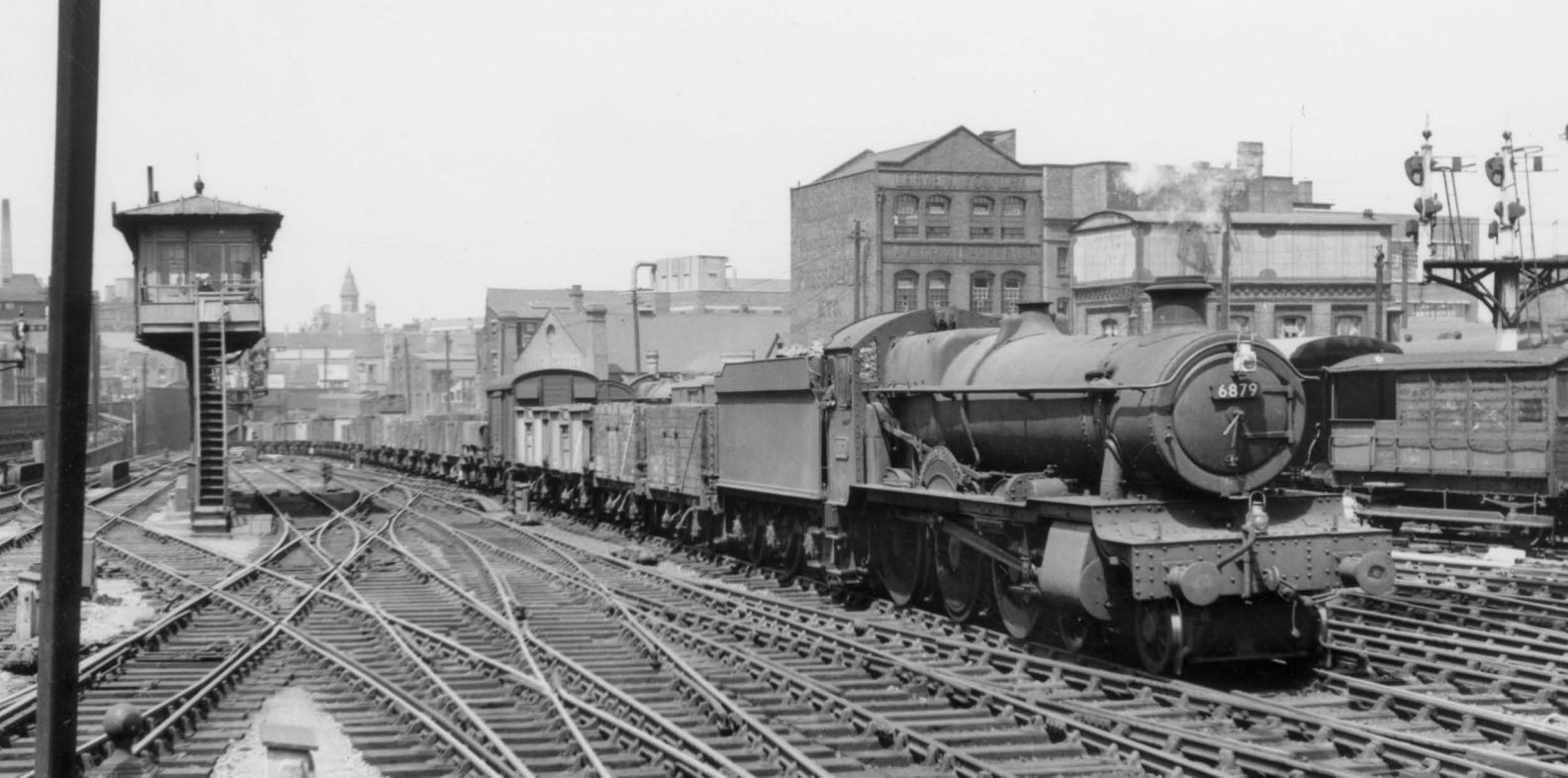
By standing at the end of Platform 6 at Birmingham's Snow Hill station spotters had an excellent view of trains approaching from the north and Stourbridge as they passed the timber-built elevated North signal box, seen in this view as Banbury-allocated ex-GWR 'Grange' class 4-6-0 No 6879 Overton Grange approaches with a southbound freight train. Beyond the brakevan on the right we see the large water tank. Kidderminster Railway Museum I23036
