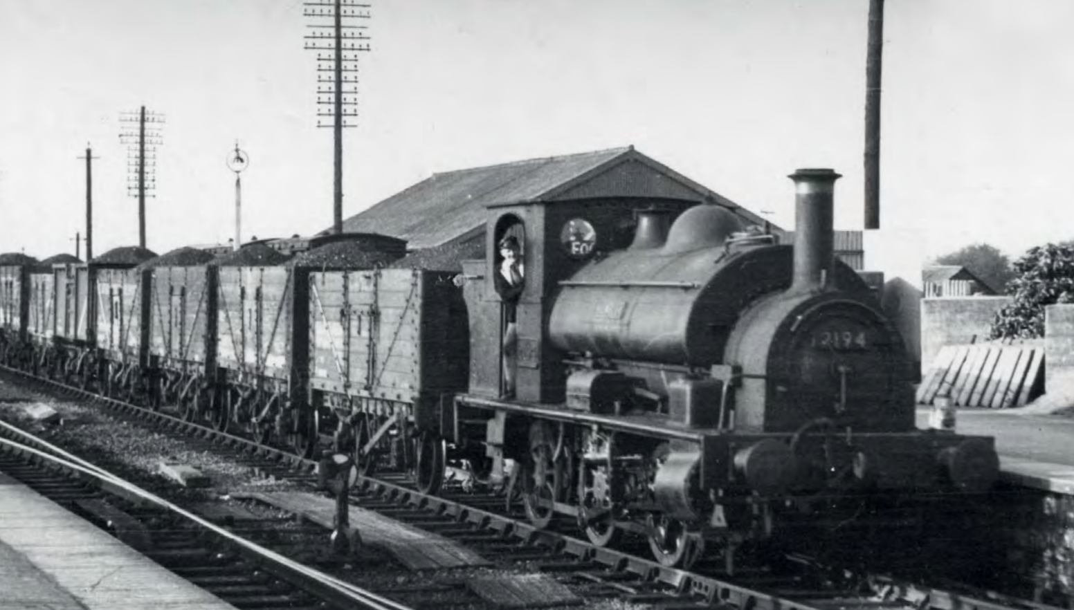
On 20 April 1951 Taunton-allocated Burry Port & Gwendraeth Valley Railway 0-6-0ST No 2194 Kidwelly is pictured at Bridgwater hauling a coal train. This was one of two locomotives of this type built for the BP&GVR by the Avonside Engine Company in 1903. Their weight was 31 ton 7cwt, and they had 3ft 6in driving wheels and outside cylinders. No 2194 was moved from Weymouth to Taunton in the 1940s principally to carry out shunting duties at Dunball Wharf at Bridgwater for the Shell/BP depot, and was withdrawn from Taunton shed in February 1953. Great Western Trust
