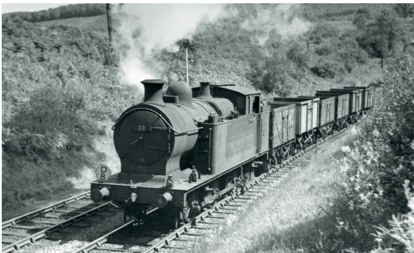
Locomotives from seven different classes of 0-6-2Ts of former Rhymney Railway origin entered BR service in 1948, working the many passenger and freight turns in conjunction with other Welsh valleys' railway companies. In this scene Rhymney 'RI' class 0-6-2T No 38 is seen on a typical duty, hauling an up coal train, and leaving Wenvoe tunnel near Caerphilly on 13 August 1954. The 'RI' class was a development of the 'R' class of 1907, and the engines were built by Beyer, Peacock and Hudswell Clarke, ten of these engines entering BR service. No 38 was withdrawn in October 1957, one of the final two in service.
