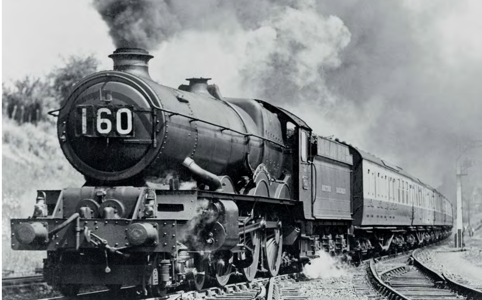
After the war the Great Western Railway took steps to improve the thermal performance of the 'Kings', and the first member of the class to be fitted with a four-row superheater was No 6022 King Edward III , which was released back into traffic from Swindon Works on 5 March 1948. Here No 6022 is seen passing the siding at the foot of Hemerdon bank, which is equipped with a catch point, when in charge of a down express for Plymouth. The tender carries the BRITISH RAILWAYS legend in full in GWR style letters. Kidderminster Railway Museum
