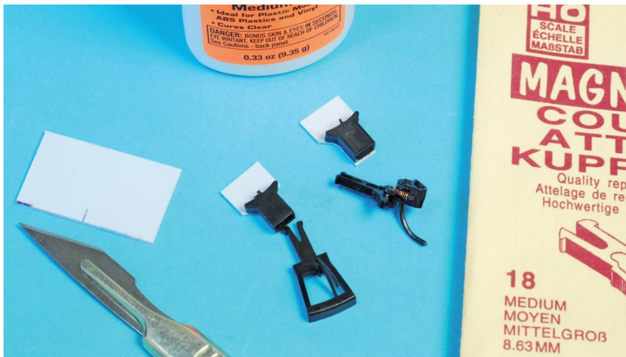
NEM coupling pockets were fixed to 1mm thick plastic sheet, trimmed to form low-profile mounts.
