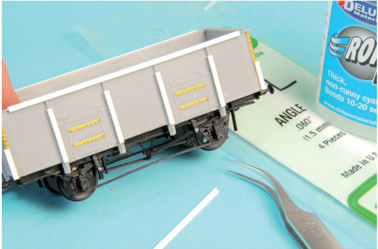
Various sizes of plastic strip and angle section replicate the distinctive plating over the stanchions.
