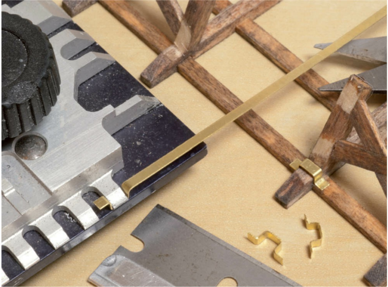
Strengthening plates and brackets are easy to create from 10thou (0.25mm), 2mm wide brass strip, fixed with cyano.
