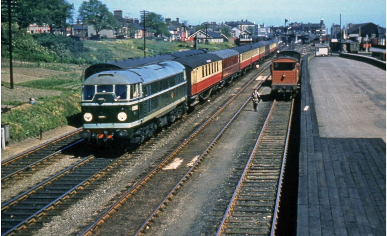
D5505 on passenger duty at Lowestoft. Only the outermost axles on each bogie beneath the D5500s were powered, giving them an 'A1A-A1A' wheel arrangement, the 'A' denoting powered axles, the '1' denoting unpowered ones.
