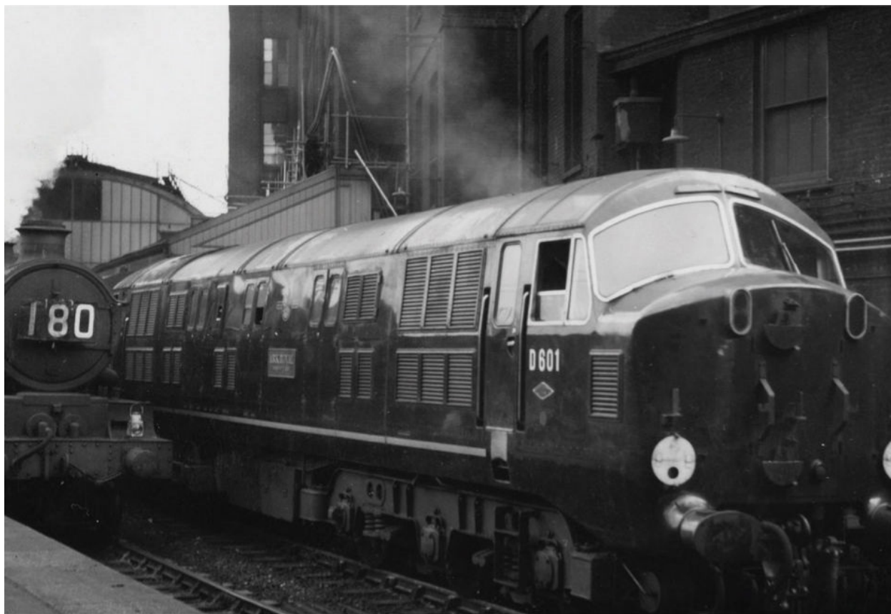
‘Diesel-hydraulics’ – like North British-built D601 Ark Royal , seen at Paddington in August 1958 – use a pump-like torque converter to convey power (via gears) from the engine to the wheels.
