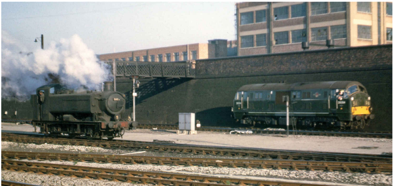
Though largely unsuccessful, the diesel-hydraulic D6300s were used extensively in Cornwall, and around Bristol and London. Here, D6354 waits at Old Oak Common with Pannier tank no. 8481.
