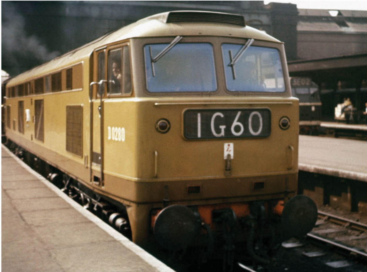
In original livery, D0280 Falcon prepares to leave King's Cross in 1962. BR's Chief Engineer (Traction and Rolling Stock) was reportedly unimpressed with Brush's use of high-speed Maybach engines therein.
