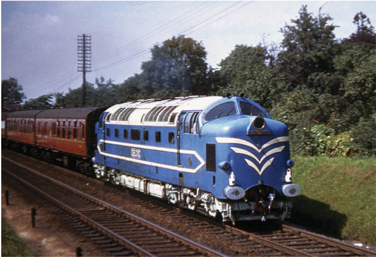
Deltic itself is seen at Ordsall in June 1960. The name derives from the locomotive's triangular cylinder arrangement. It was donated to the Science Museum in 1963.
