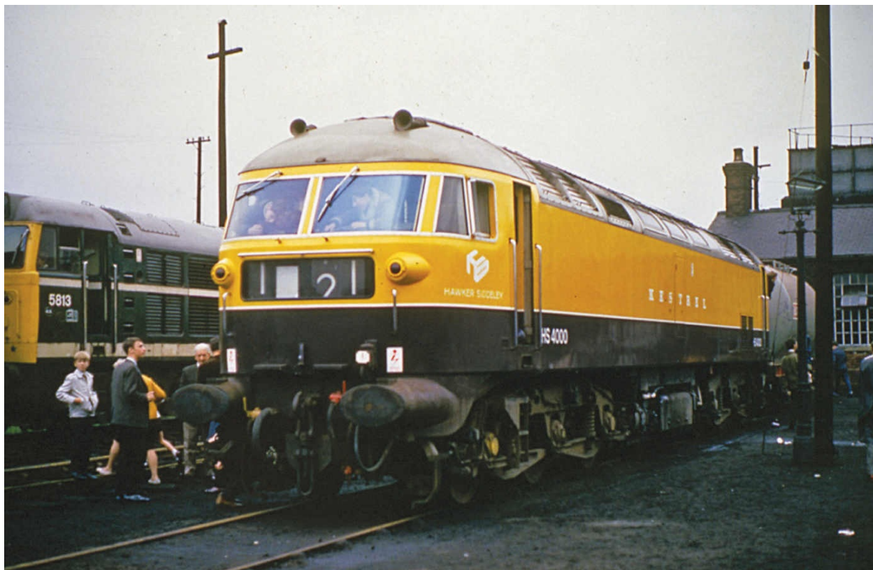
Brush's experimental 4,000hp diesel-electric Kestrel was tested on BR from 1968. Though capable of 125mph running, it was too heavy to be driven faster than 100mph.
