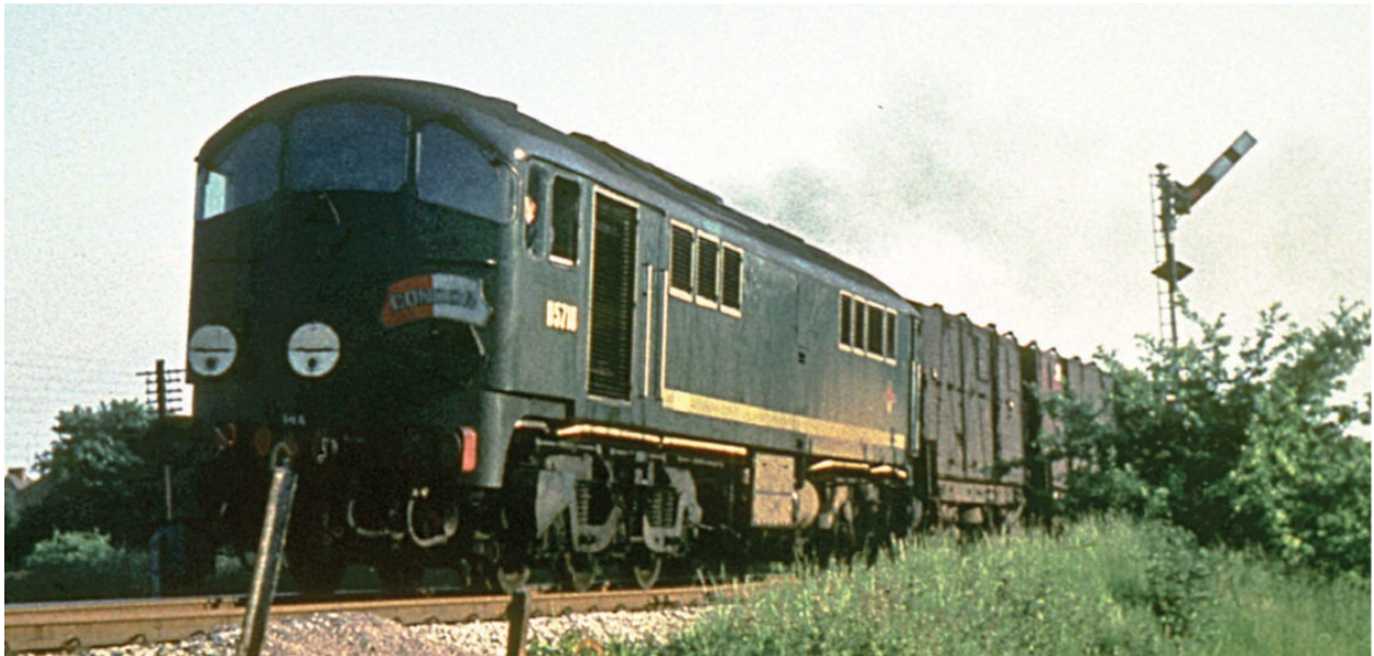
D5718 on the 'Condor' – BR's Anglo-Scottish express freight service – in 1960. The D5700s proved so unreliable on this train that customer demand dropped until alternative traction was provided.
