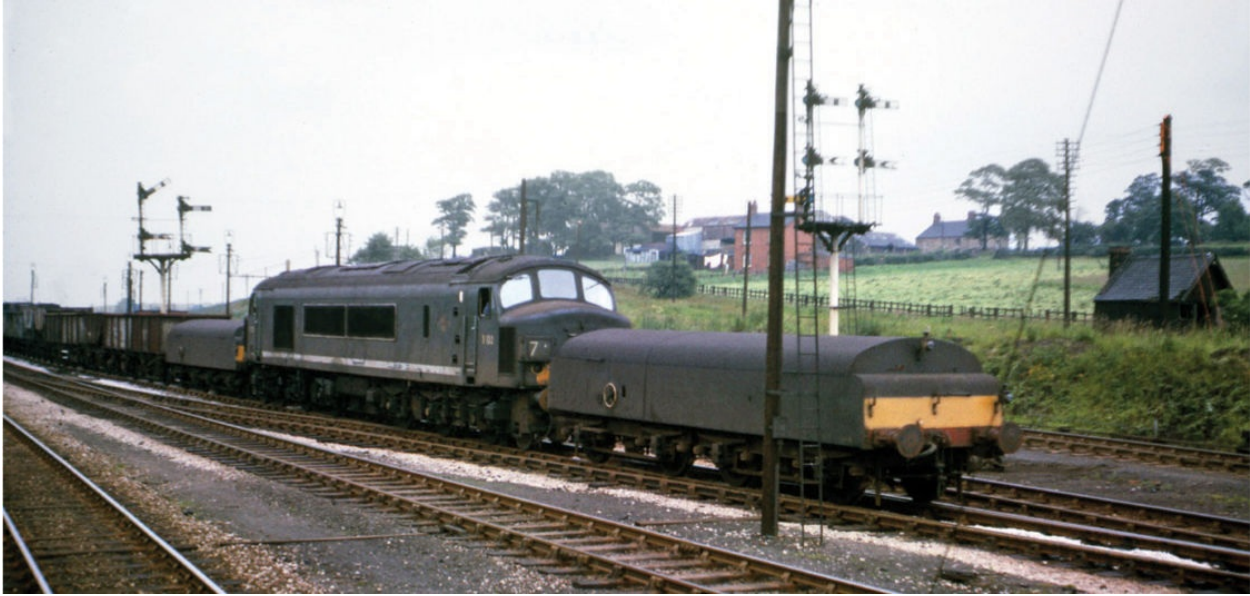
D102 – from BR's second 'Type 4' batch (also known as 'Peaks') – coupled to a pair of 'brake tenders', which provide extra braking power on freights formed entirely (or largely) of 'unfitted' wagons.
