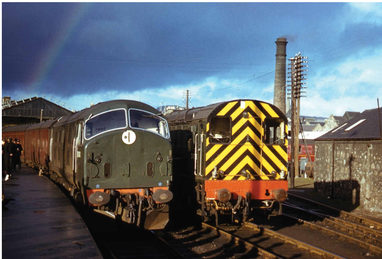
Despite a reputation for unreliability, there would eventually be fifty-eight NBL diesel-electric Type 2s on BR's books. D6141 (left) is seen here at Inverness alongside a locomotive of more successful design.
