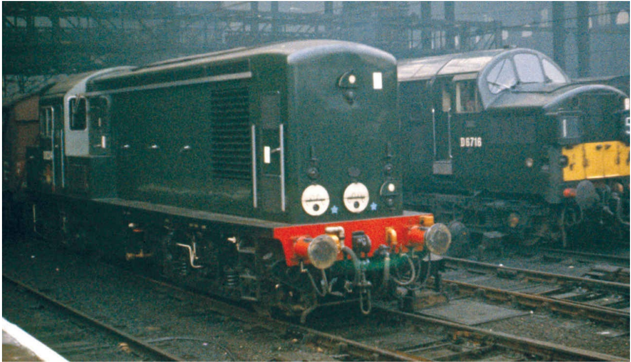
The D8200s were designed by British Thomson-Houston and built between 1957 and 1961. D8243 (left) is seen at Liverpool Street in original livery.
