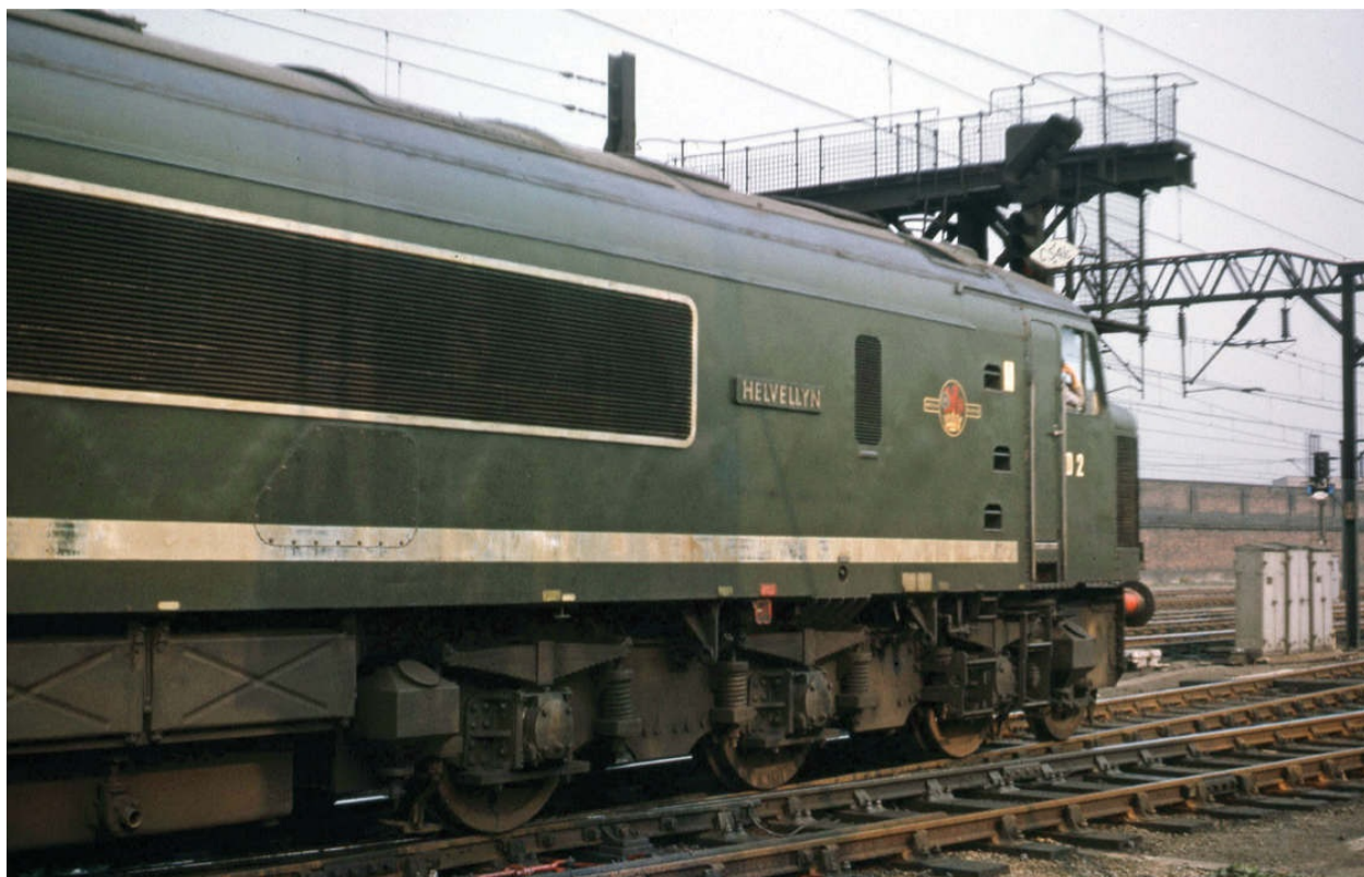
D2 Helvellyn captured at Crewe. The locomotive is one of the ten-strong class of Derby-built Type 4s, which featured BR's favoured Sulzer engine, but whose weight saw relegation to heavy freight traffic. Named after British mountains, they became known to many as 'Peaks'.
