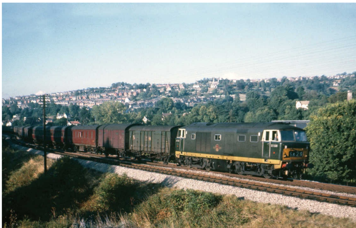
Beyer Peacock built 101 diesel-hydraulic Type 3s for the Western Region. Introduced from 1961, their Mekydro-manufactured transmissions led them to be dubbed ‘Hymeks’. Here, D7039 nears Ham Hill.
