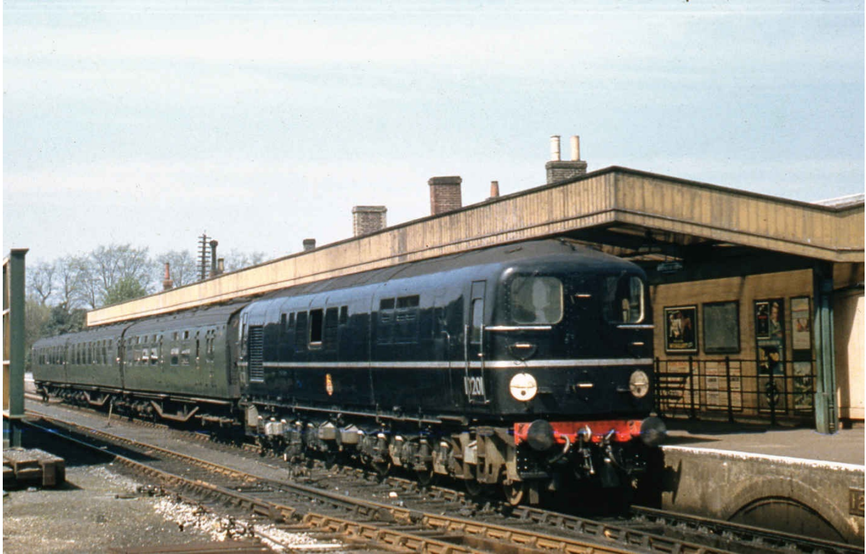
The Bulleid-designed no. 10201 appeared in 1950. Like no. 10202, it was capable of 1,750hp. A 2,000hp variant came in 1954, but all three were withdrawn at the end of 1963.
