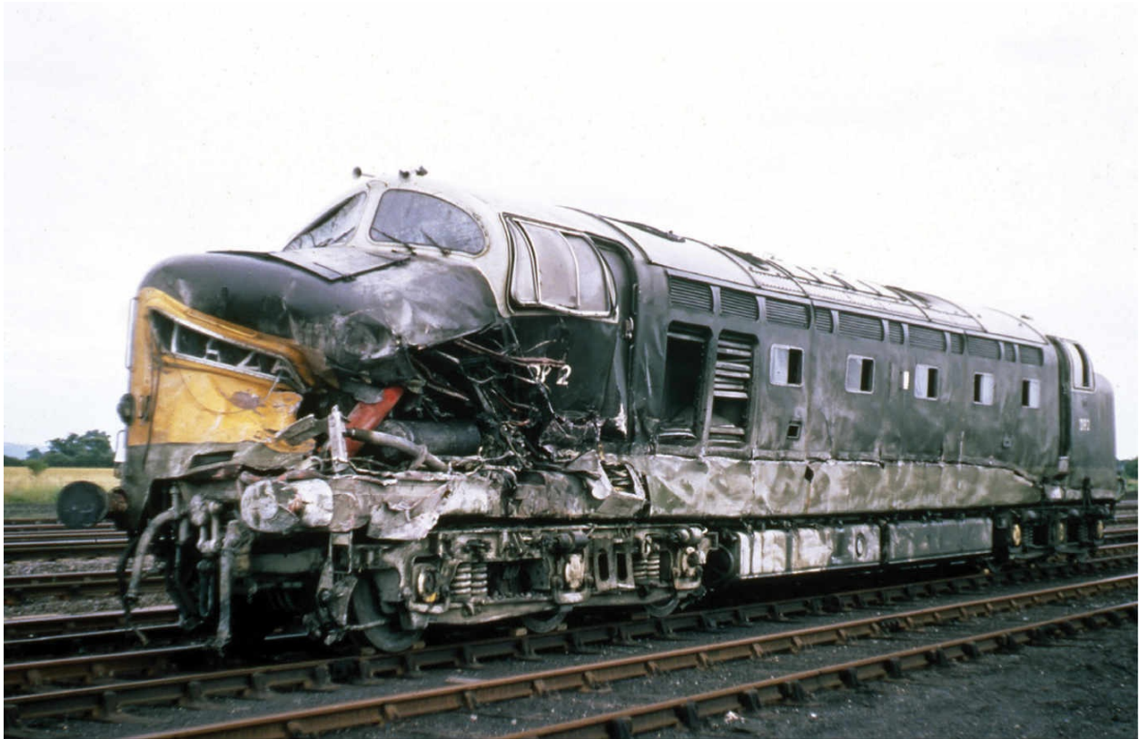
The damage caused to DP2 in the fatal collision at Thirsk on 31 July 1967 was so great the locomotive was withdrawn and dismantled for spares.
