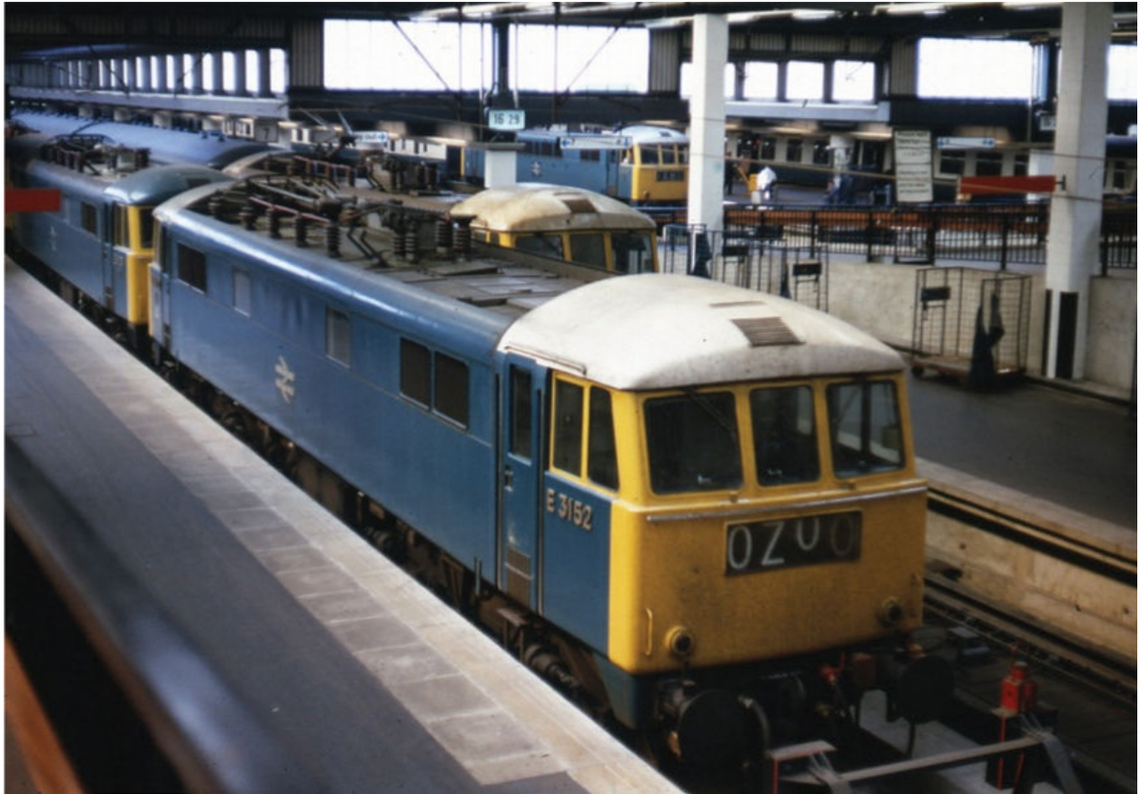
AL6 E3152 at Euston. Note the overhead wires, from which 25kV AC power is collected by the pantograph on top of the locomotive.
