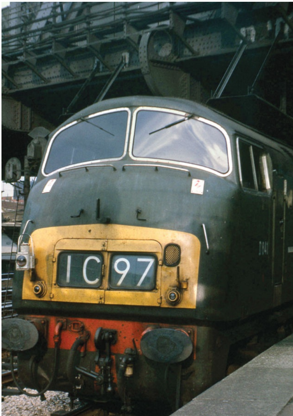
D841 Roebuck – one of the North British ‘D800s’ – at Paddington. Swindon locomotives used Maybach engines connected to Mekydro transmissions, but the NBL examples married MAN engines to Voith transmissions.
