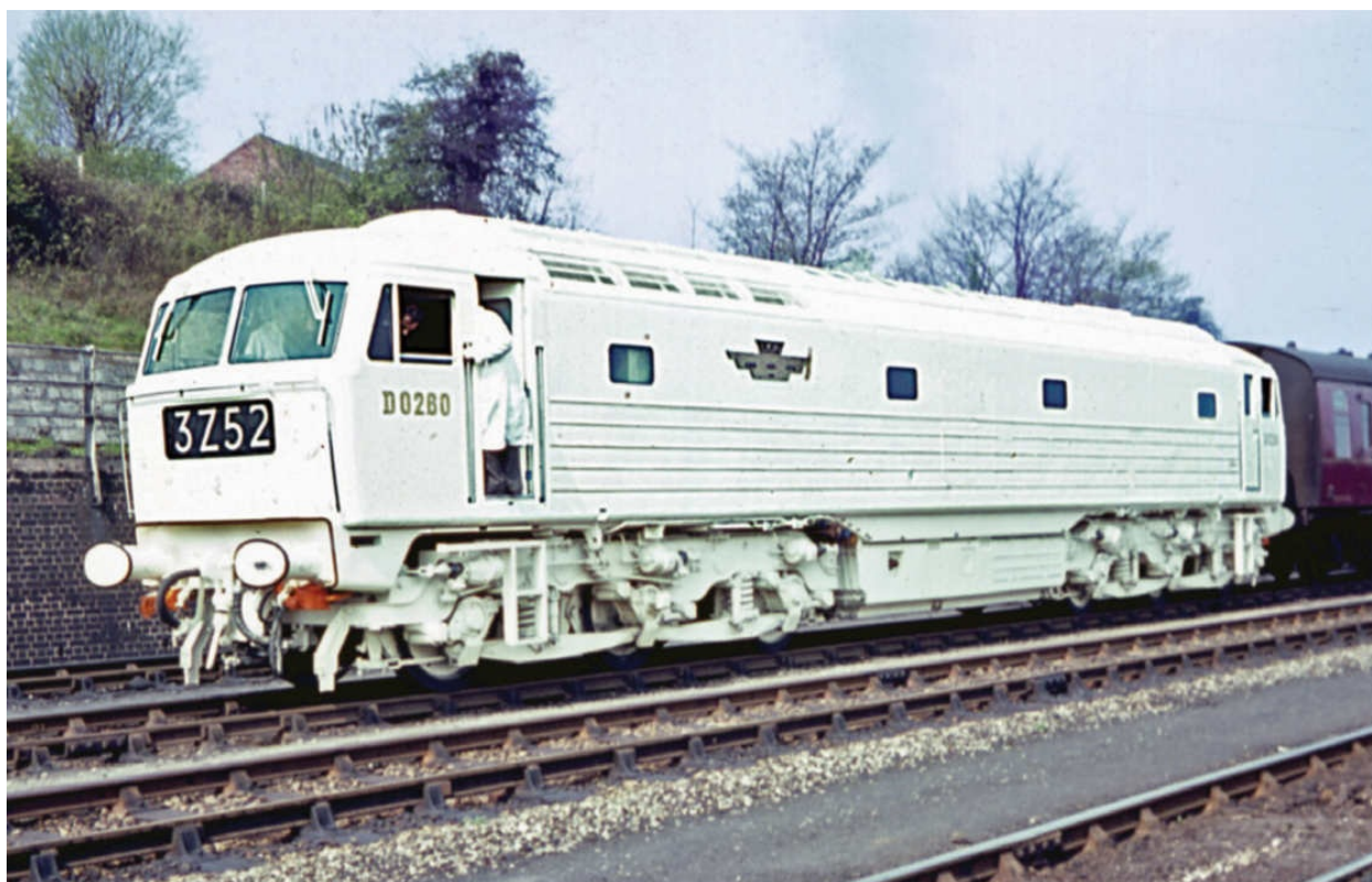
English Electric's DP2 about to enter Northchurch Tunnel on a passenger working. The locomotive showed it was possible to build a 2,700hp 'diesel-electric' that weighed less than a comparable 'diesel-hydraulic'.
