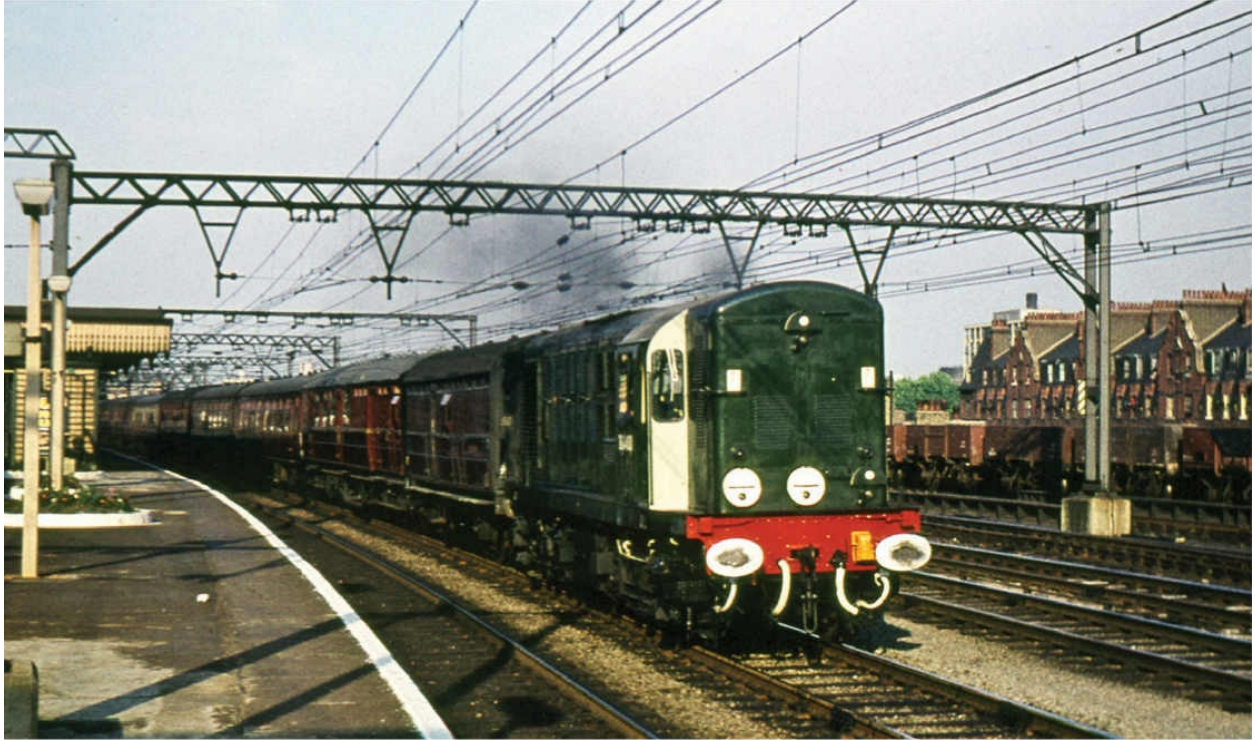
D8400 – the doyen of its class – is seen at Bethnal Green in 1961. Like the D8200s, the D8400s suffered piston and cylinder head problems.
