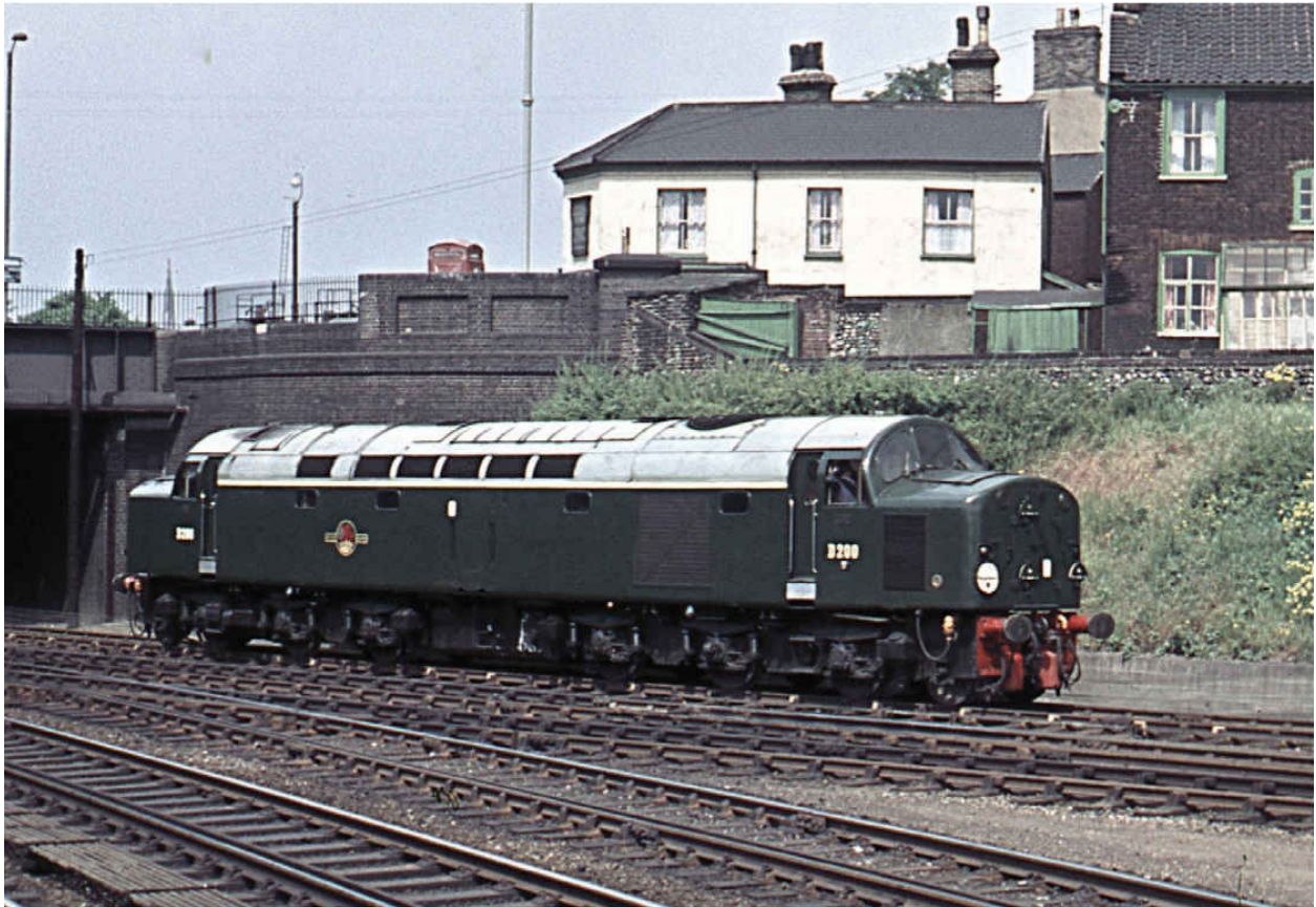
The first English Electric Type 4, D200, runs light at Wensum Curve. Like all Pilot Scheme Type 4s, its unpowered outer axles helped distribute the weight more evenly.
