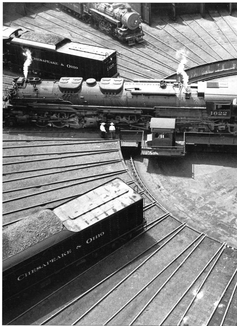
LEFT: The most powerful steam locomotive ever built in series production was the 'Allegheny' type. Designed and constructed by the Lima Locomotive Works, Lima, Ohio, for the Chesapeake & Ohio Ry., some were also used on the Virginian Ry. On test, they registered nearly 7500hp at the drawbar, 1000 more than the legendary 'Big Boys' of the Union Pacific. Here, 'Allegheny' No.1622 rolls off the turntable at the C&O roundhouse in Huntington, West Virginia, while sister No.1627 stands by; a third 1600 is in the foreground with only its fully-coated tender in view. Two supervisors – their hats informally distinguishing their rank – watch the running gear of No.1622 as it moves regally by.
