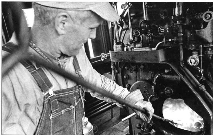
LEFT: Fireman Arkinstall, a veteran of steam passenger-train service on the Pennsylvania RR, uses a firehook to help prepare the coal firebed on former Great Western Ry. engine No.60 for later departure. Above the open firedoor is a rack for oil cans.
