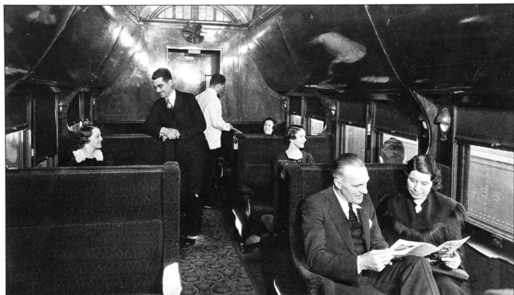
LEFT: Interior of a Pullman sleeping car on the Northern Pacific Railway in the early 1920s. The car is 'made up' here for day use. At night, Pullman attendants 'made down' the car by unfolding the upper berths, converting the seats into lower berths, and hanging privacy curtains.
