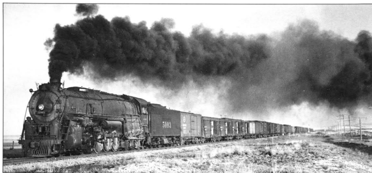
LEFT: The grandest 'Texas'-type of all was the 5001-class of the Santa Fe. Each of these 35 nearly-6000hp locomotives could roll freight at 70mph. Here is No.5003 with 70 cars near Vaughn, New Mexico, in 1940.
