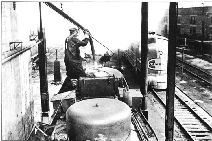
LEFT: At Los Angeles about 1940, hostler Beal, responsible for engine servicing, fills the sand dome of Santa Fe locomotive No. 3437, a passenger steamer. A harbinger of change, a General Motors-built E2 diesel from the Super Chief grows past. Santa Fe was one of the first major carriers fully to endorse diesels; steam last ran on AT&SF in the summer of 1957.
