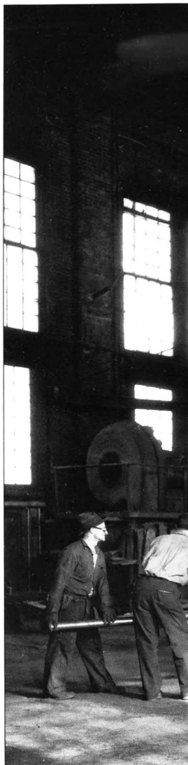
RIGHT: A locomotive shop foundry crew beats white-hot steel into shape under the steam hammer for a new side rod, in this scene from the 1930s.
