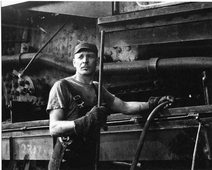
LEFT: At the Steamtown National Historic Site in Scranton, Pa., roundhouse foreman Roger Samuels uses a hose to clean out the ashpan of Canadian Pacific No. 2317, a heavy passenger locomotive.
