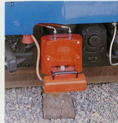
Below right The under-arm power collection shoe can be fitted with a protective cover when not in use.
