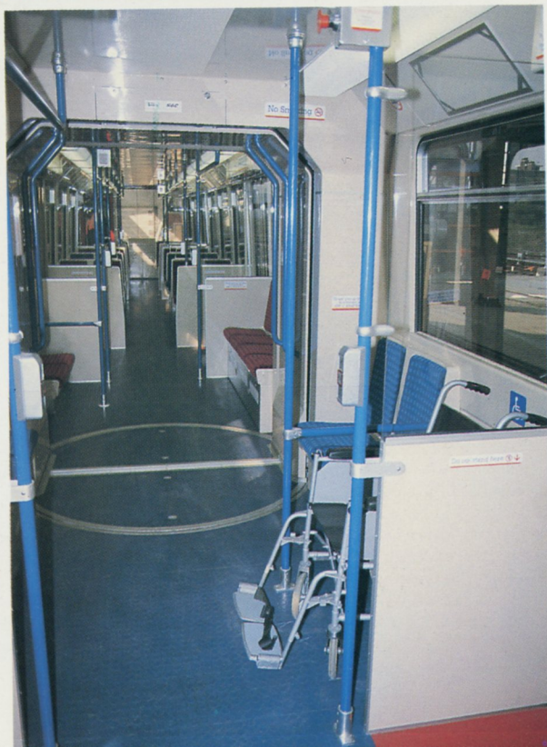
Interior view of car 03 showing a wheelchair in place near the centre of the car, seating finished in two colours of moquette and the red floor marking to show the area into which the doors fold back when opening.
