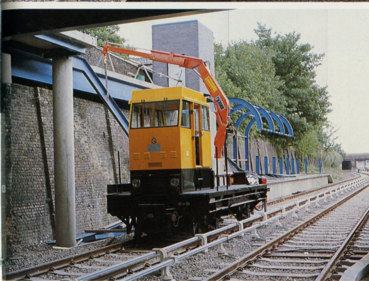
As well as the 11 passenger cars, a single Wickham CT30 service vehicle is included in the contract for the initial railway. It is pictured helping to assemble steelwork at All Saints station.
