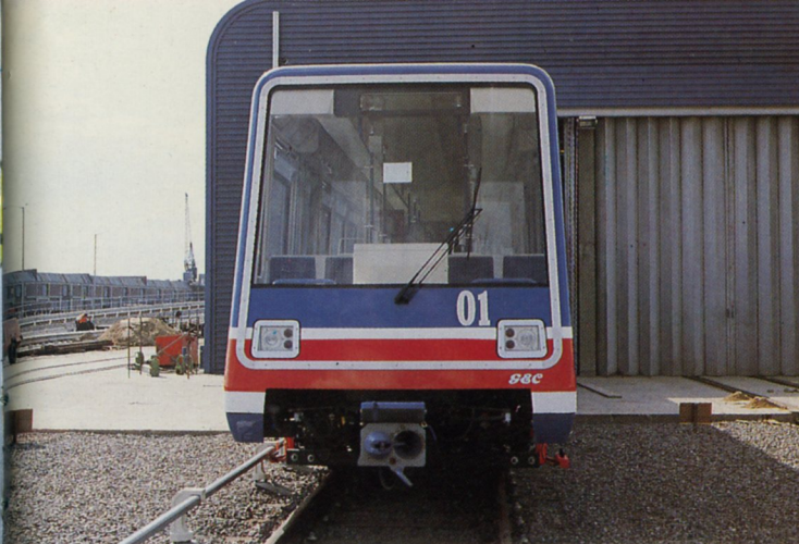
Cars 01 and 04 are fitted with on-board rail lubrication equipment. The neck of the filler pipe is just visible below the headlight on the left of this view.
