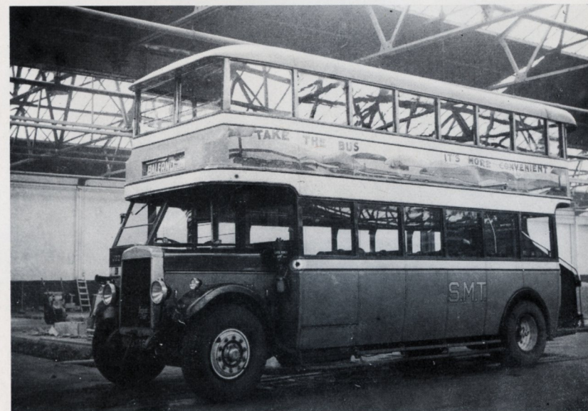
23. Double-deckers reappeared in 1929 in the form of the Leyland Titan. A second lot has enclosed stairs. One of the first lot is shown: it was later J22.
