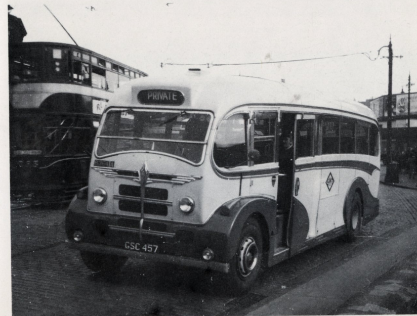
58. The forerunner of the Burlingham "Seagull" pattern coach body arrived in 1949, on A.E.C. B364, here shown with improved front styling.
