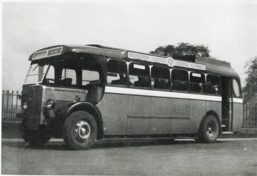
32. A.E.C. "Regal" coaches with 28-seat Burlingham bodies incorporating a toilet compartment were introduced in 1933, and similar 32-seaters without toilets in 1934. One of the former type is shown, B70.
