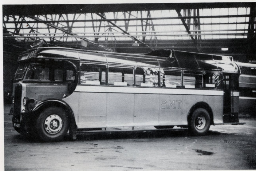
38. The Leyland "Tiger" buses of 1935 with 34-seat Cowieson bodies retained the rear entrance and introduced the flared skirt. H108 is shown.
