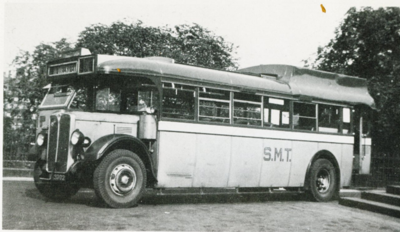
31. New buses in 1932 were A.E.C. "Regals" with 34-seat bodies by W. Alexander. Their petrol engines were later replaced by oil engines and after the war they received new 35-seat bodies of the then current pattern. This is B65.
