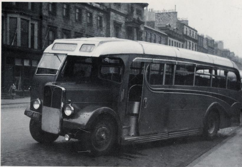
59. Burlingham also provided more orthodox 35-seat coach bodies for more new A.E.C.'s in 1949. The one shown is B370.
