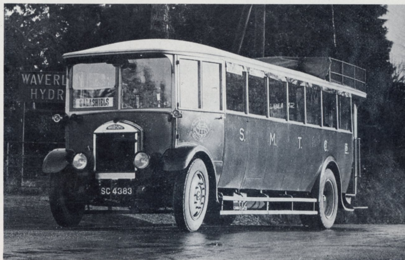
19. There were still many more Maudslays such as this one of 1929 with S.M.T. 32-seat body, later K59.
