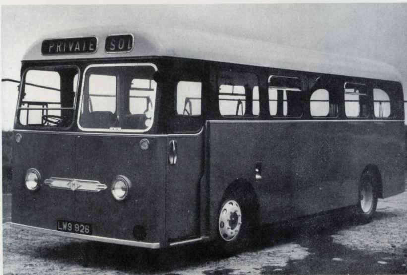
68. S1 was an experimental lightweight 32-seater built by the company themselves in 1955.
