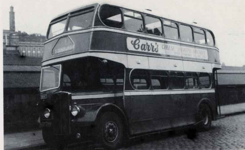
61. A.E.C. 53-seat double-deckers were also bought in 1948, 1949 and 1950, with bodies by W. Alexander, Duple and Burlingham respectively. BB87 is one of the Burlingham lot.
