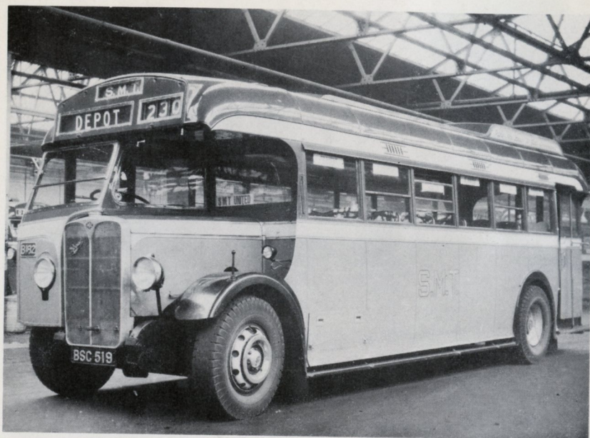
47. There were more A.E.C. "Regal" buses in 1938 with 34-seat rear entrance W. Alexander bodies of which B182 is the example shown.
