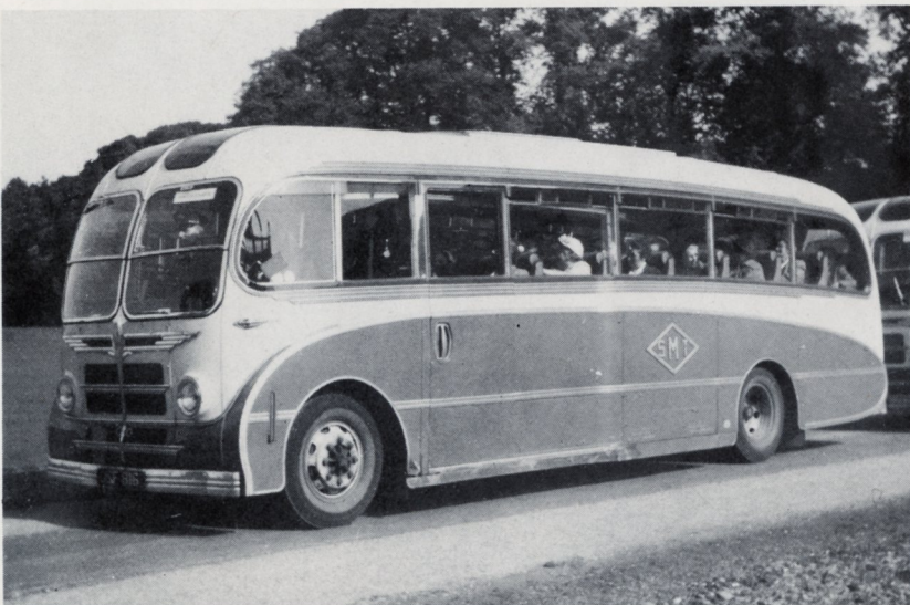
64. The Burlingham Seagull pattern coach body with 30 seats was provided for more new Bedfords in 1952, while some earlier post-war Bedfords received 24-seat versions of this body. Many earlier A.E.C. "Regals" were also rebodied with 35- or 37-seat Burlingham Seagull coach bodies. This is a Bedford 30-seater, C191.
