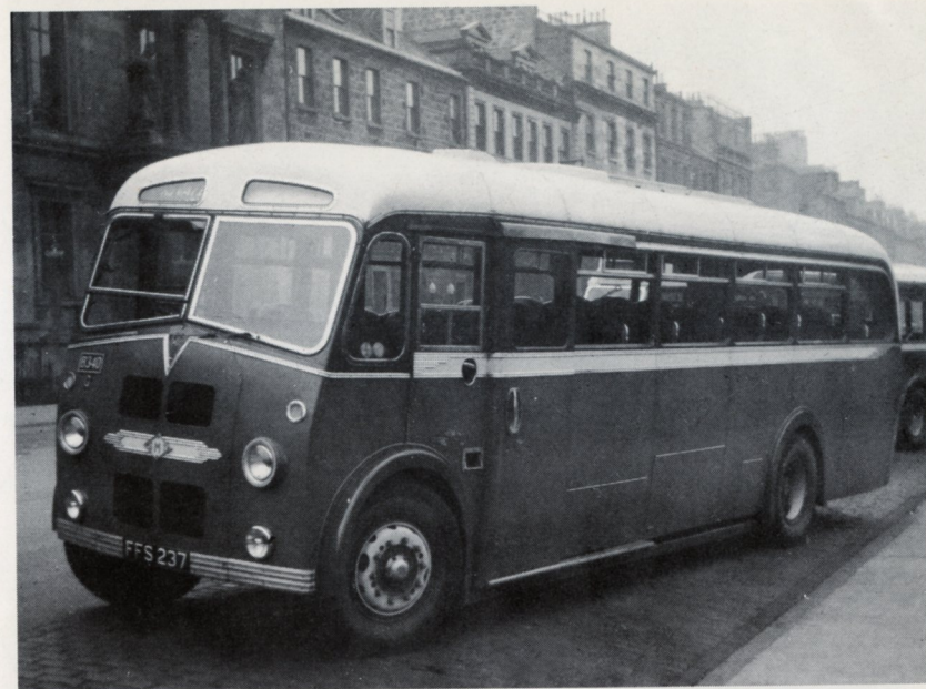
65. Fifteen A.E.C. "Regals" of 1948 were also rebuilt with full-front bodies. B340 is one of these.
