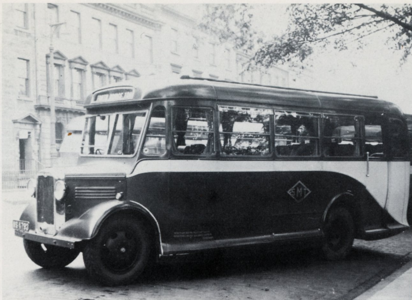
39. A few Duple-bodied Bedfords added in 1935 also had rear entrances and were painted a very dark blue. This is C44.
