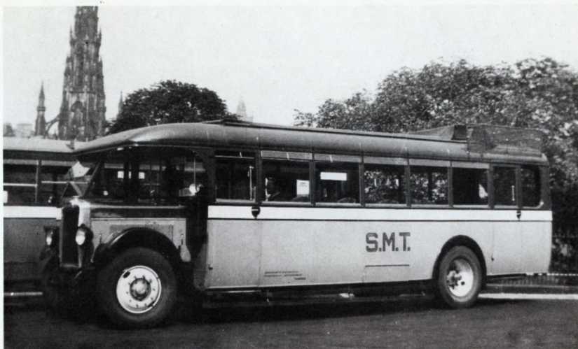
25. There were also Leyland "Tiger" coaches in 1929 with 29-seat bodies by Cowieson. This one was later H17.
