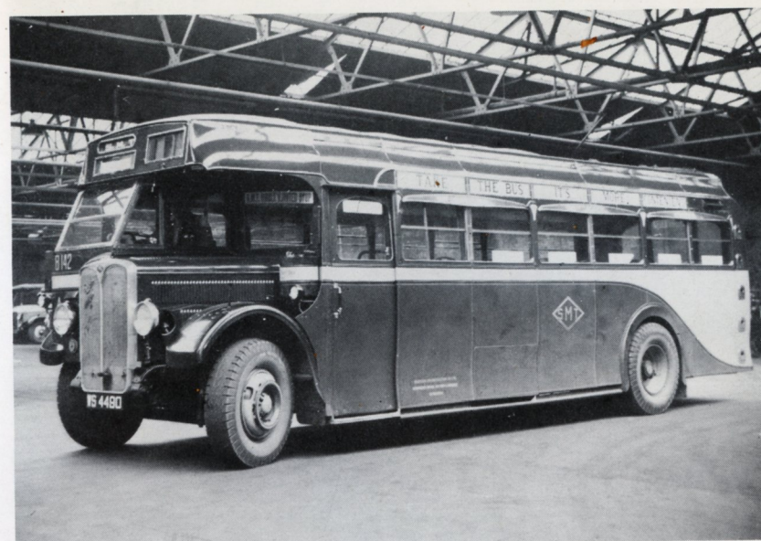
37. A front entrance was adopted for the 1935 A.E.C. "Regal buses" with 32-seat bodies by W. Alexander. This one is B142.
