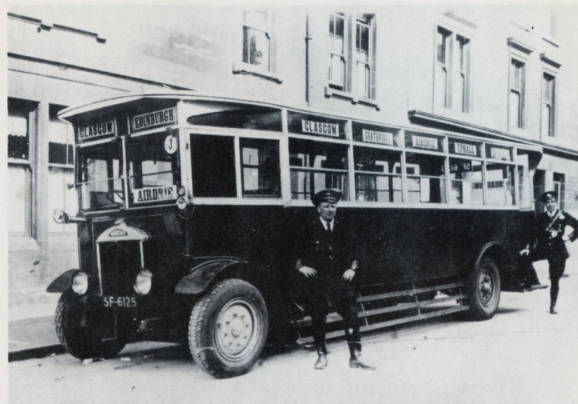
14. The first of the S.M.T.'s new 32-seat saloons in 1926 were Maudslays, ten with S.M.T. bodies, 25 with Short Bros. bodies and 25 with bodies by Vickers, of which this is one, later numbered K132. (Travel Press & Publicity Co. Ltd.)
