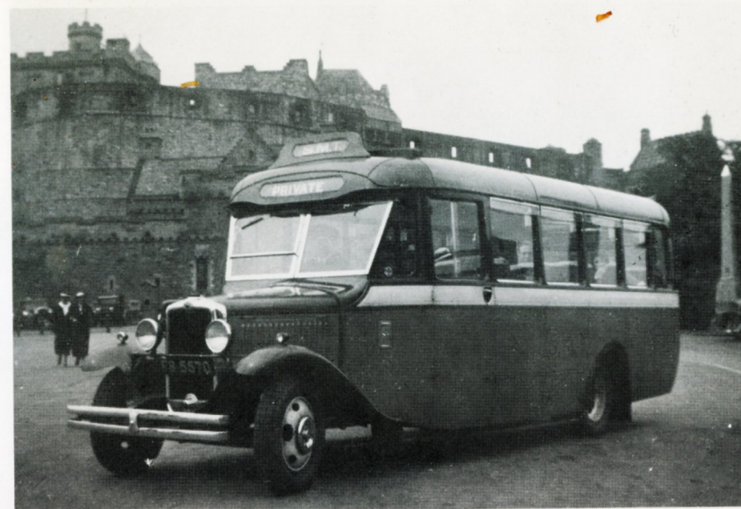
33. The first Bedfords, in 1933, had 20-seat Burlingham bodies as C14 shown here, though they had been preceded in 1930 by a few Chevrolets with 14-seat coach bodies by Alexander Motors, Edinburgh.
