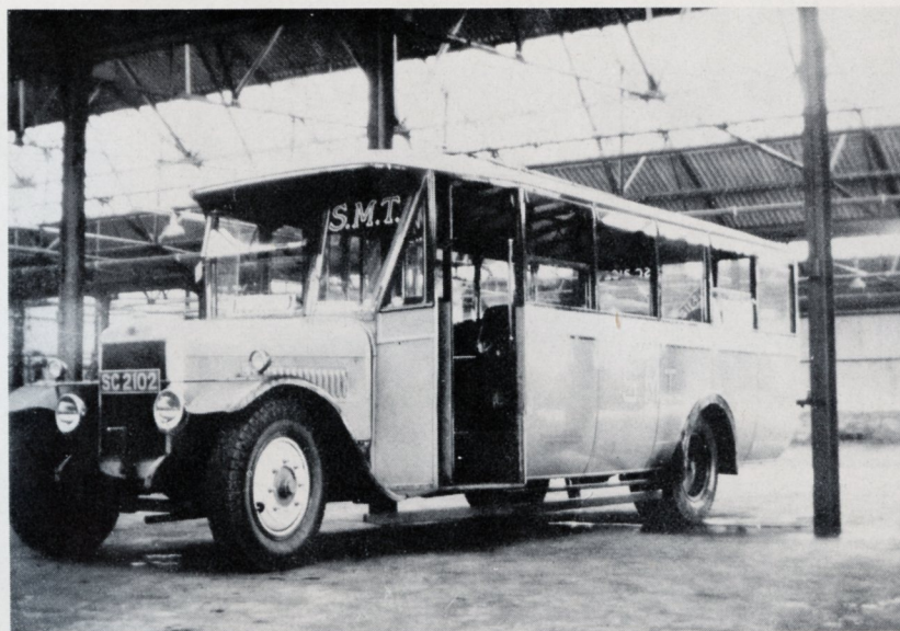
21. The small buses were also replaced with 20-seat Star saloons. The bodies by Hall-Lewis and by Hoyal were similar. This one was later N37.
