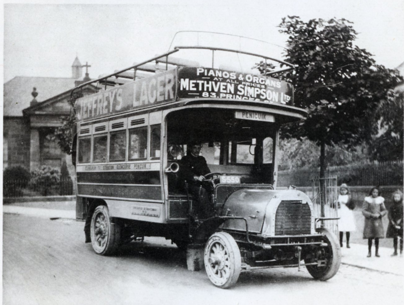
3. One of the second lot of Maudslays with wider body and transverse seats.
