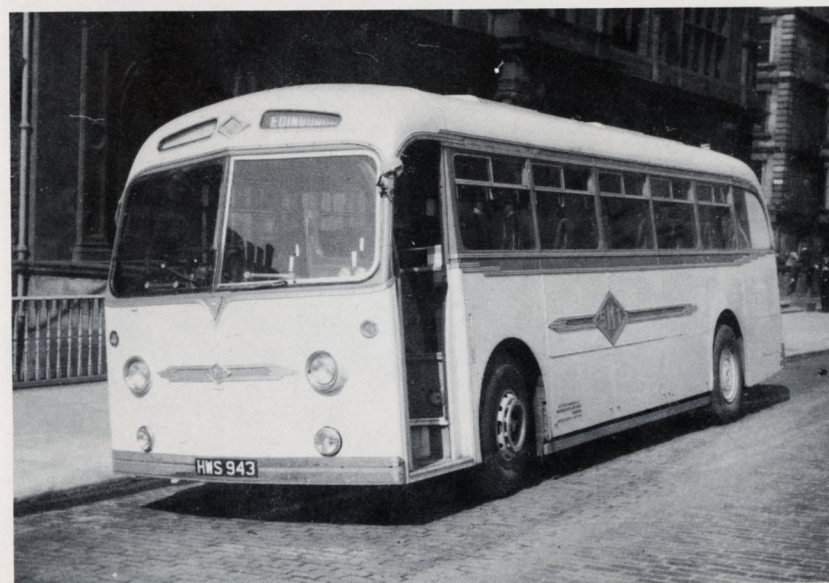
62. The A.E.C. Mk IV underfloor engine coach appeared in 1951 with 30-seat body by W. Alexander incorporating toilet compartment. The 1952 lot lacked this and seated 40 instead. B441 is one of the 1951 lot.
