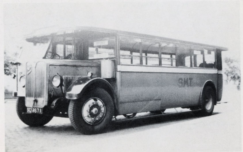
30. The first oil engine bus was also an A.E.C. with 30-seat Strachan body, numbered B2.
