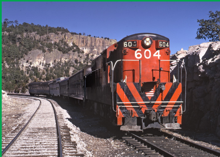
The last locomotive constructed by Fairbanks-Morse, 1963-built ChP No. 604, looks sharp at the head of a passenger extra in early 1974. Four photos, Brian Schmidt collection
