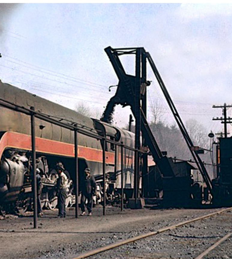
Left: J-class 4-8-4 604, having come in with the Pelican , is coaled and inspected on March 2, 1957. After turning and further servicing, the 4-8-4 will depart with mail train 10.
