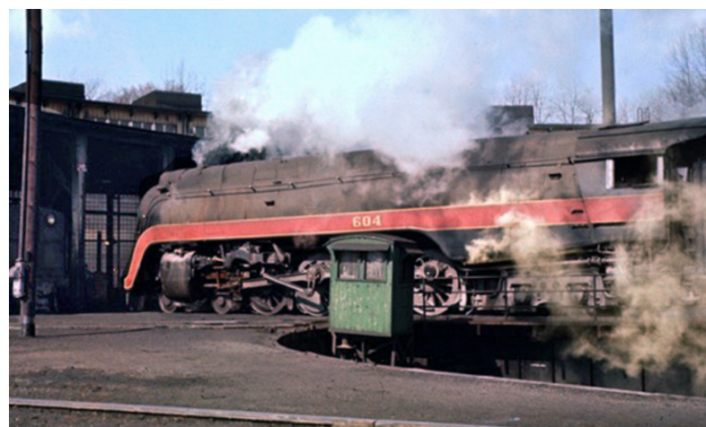
Left: J-class 4-8-4 604, having come in with the Pelican , is coaled and inspected on March 2, 1957. After turning and further servicing, the 4-8-4 will depart with mail train 10.
