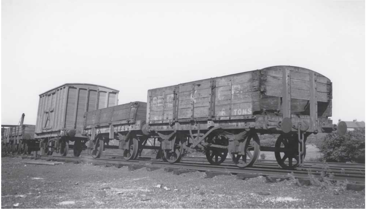
A selection of second- and third-hand goods wagons used for internal traffic on the East Kent Railway, here seen dumped in the yard at Shepherdswell, c1935. These include an ex-SE&CR 6-ton open, a three-plank open and an ex-South Eastern Railway van. ( Rev A.W.V. Mace, Milepost 92 )
