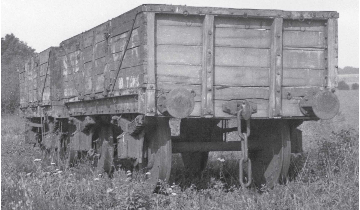
On 2 September 1938, a pair of former SER open wagons stand derelict on a siding at Shepherdswell, the former SE&CR lettering working its way through the thin coat of East Kent Railway light grey paint. These wagons have cut down rounded ends. ( R.S. Carpenter Collection )
