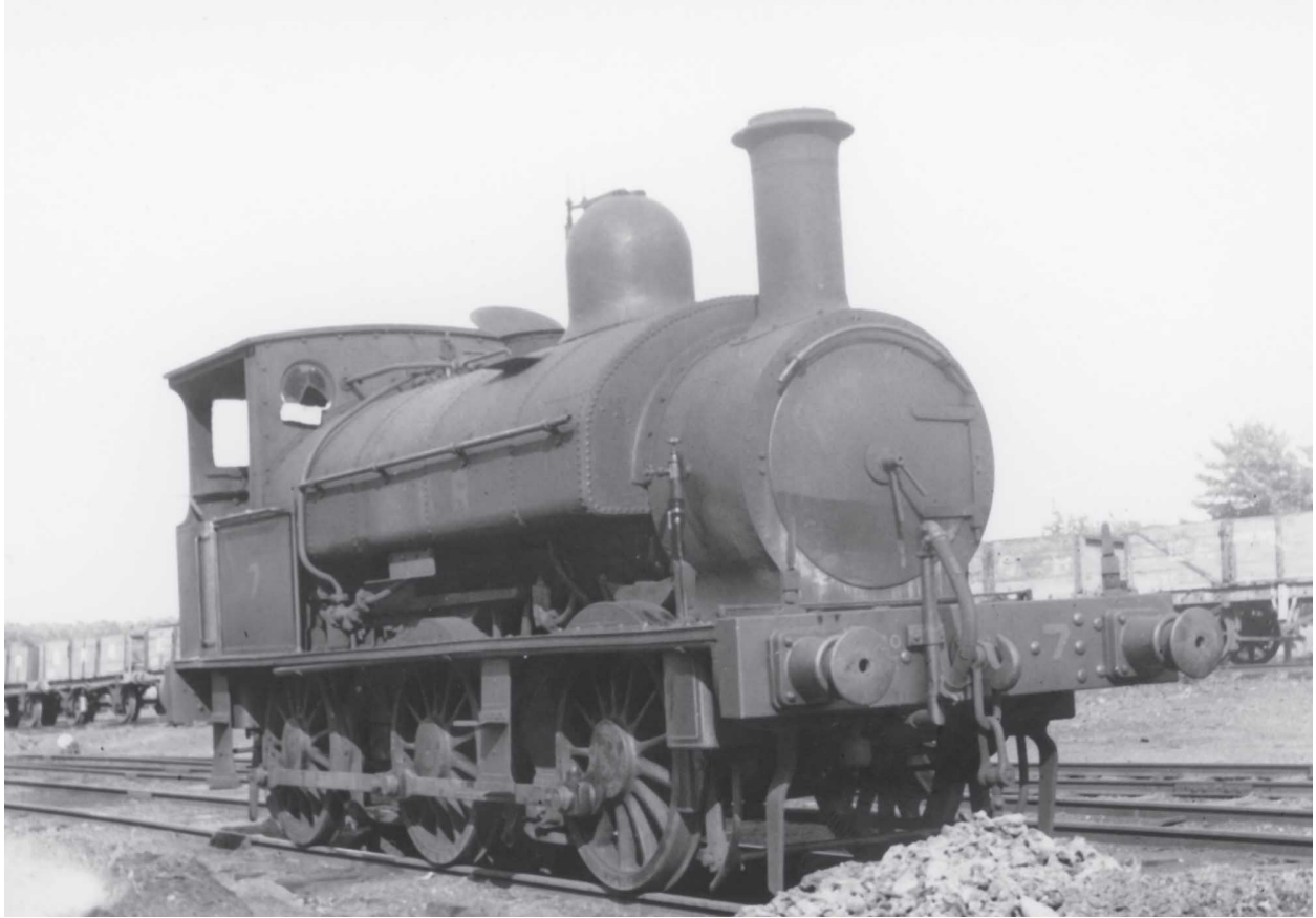
No. 7 in its later plain unlined black condition, c1938, showing its new smokebox of a different pattern to the Beyer Peacock sloped original and the Great Western patterned chimney, salvaged from the scrapped No. 1. ( Cuthbert Hamilton Ellis )
