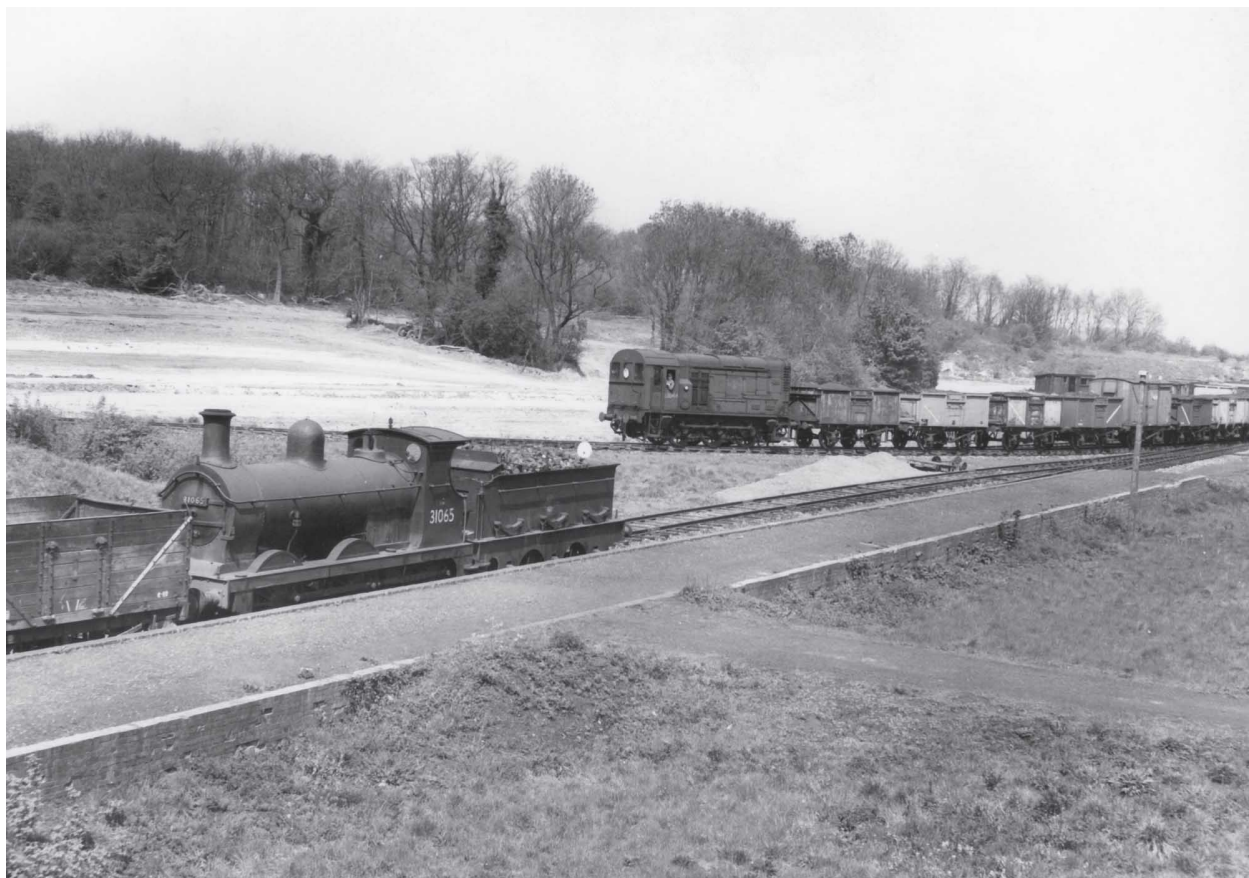
Contrast in motive power, a 350 H P 0-6-0 diesel mechanical shunter No. D3044 eases its train of coal wagons past the junction at Shepherdswell former East Kent Railway Station, while 01 class 0-6-0 tender goods 31065, waits in the platform with a train of open wagons for its journey to Tilmanstone Colliery in April 1960. ( Derek Cross )
