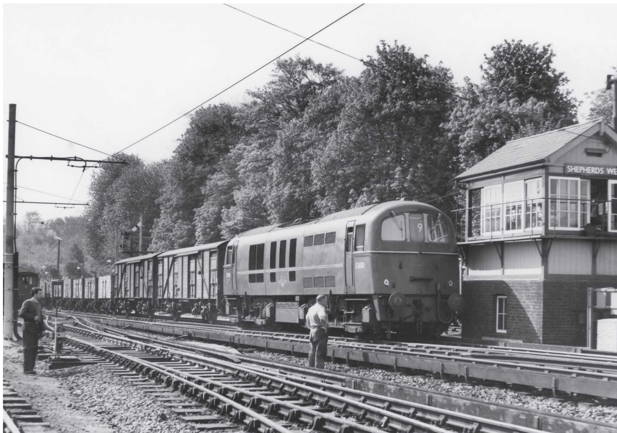
Class 71 No. E5000 arrives at Shepherds Well exchange sidings, with a mixed freight train from Dover of ferry vans and 16-ton mineral wagons, in April 1960. The overhead catenary was installed for these electric locomotives to be able to shunt in sidings and yards, not on the third rail, these locomotives being dual overhead and third rail pick up on the 750 DC system. ( Derek Cross )
