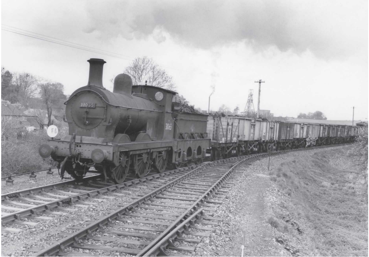
In March 1960, 01 0-6-0 tender goods 31065 heads a train of coal wagons at the same location, heading for the exchange sidings at Shepherdswell. This locomotive is now preserved on the Bluebell Railway in East Sussex, where it is one of five Ex-SE&CR locomotives resident on that line. ( Derek Cross )
