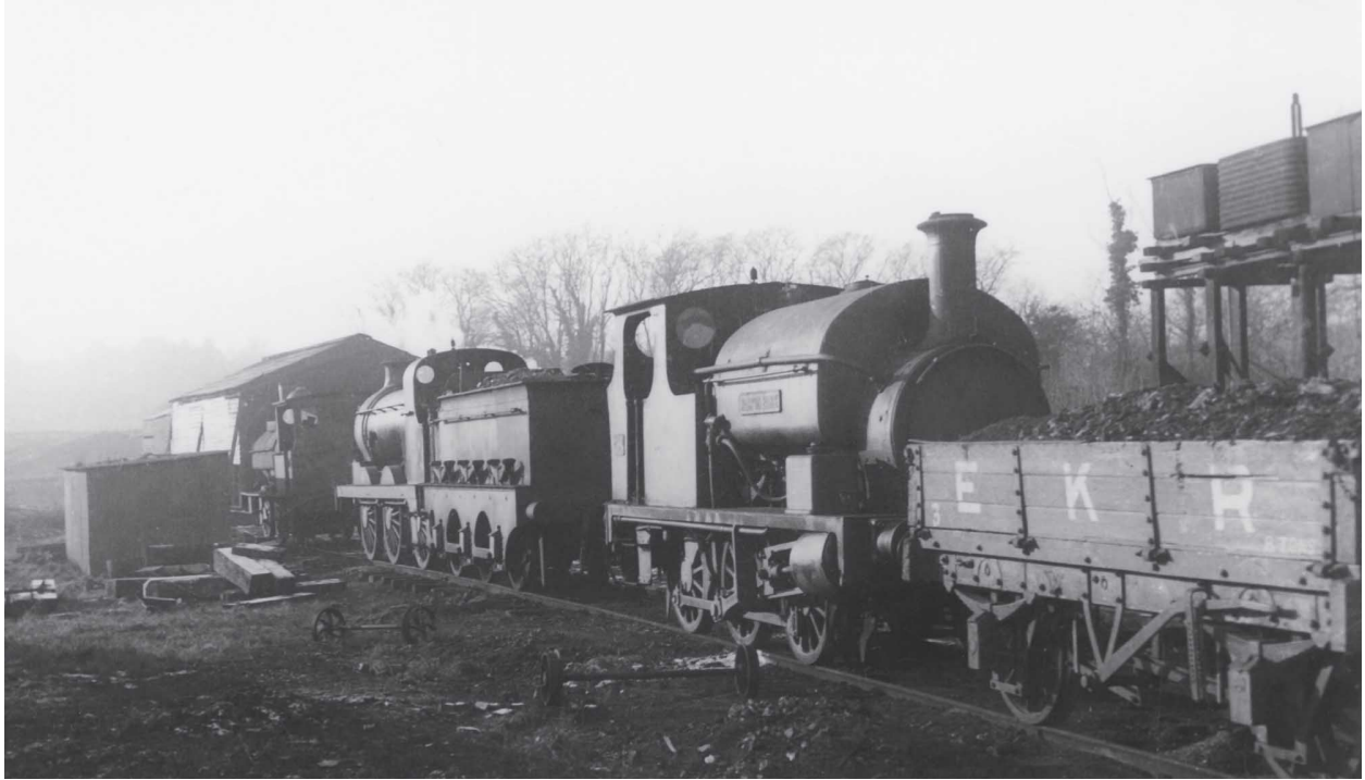
A line of East Kent Railway locomotives in the evening sun at Shepherdswell locomotive shed, showing 0-6-0 saddle tank No. 2, Walton Park , at the head of the line, followed by one of the ex-SE&CR 0 class locomotives, No. 6 or No. 8 and finally ex-L&SWR 0330 class 0-6-0 saddle tank No. 7 at the rear, c1930. ( Lens of Sutton Association )
