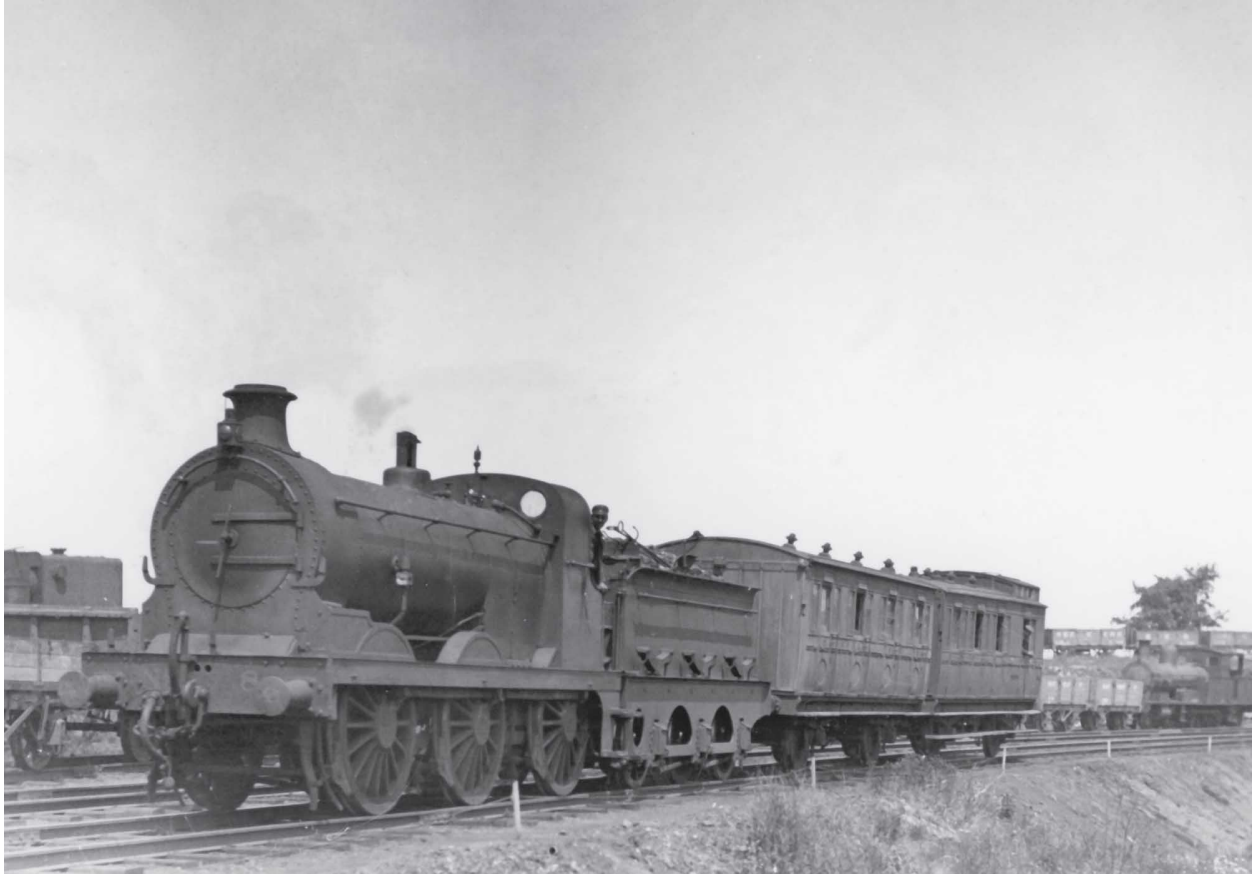
No. 8 arrives at the approach to Shepherdswell East Kent Station, with a train of two elderly four-wheeled carriages, Nos. 8 and 9, both former London Chatham & Dover Railway vehicles, c1930. Note the line of wagons in the background with No. 5, the ex-L&SWR Adams Radial 4-4-2 tank in store. (Author's Collection)
