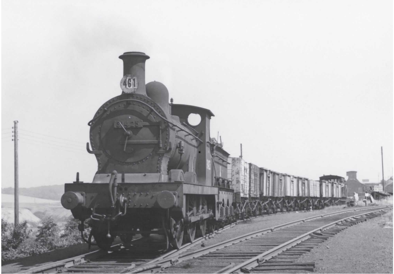
At Tilmanstone Colliery, 01 0-6-0 tender goods 31425, prepares to leave with a loaded coal train for the exchange sidings at Shepherdswell on 8 July 1959. ( J.H. Aston )
