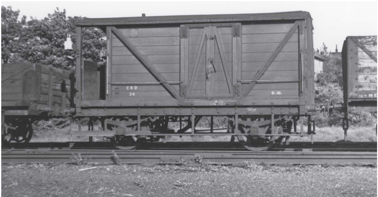
On 2 September 1938, a pair of former SER open wagons stand derelict on a siding at Shepherdswell, the former SE&CR lettering working its way through the thin coat of East Kent Railway light grey paint. These wagons have cut down rounded ends. ( R.S. Carpenter Collection )
