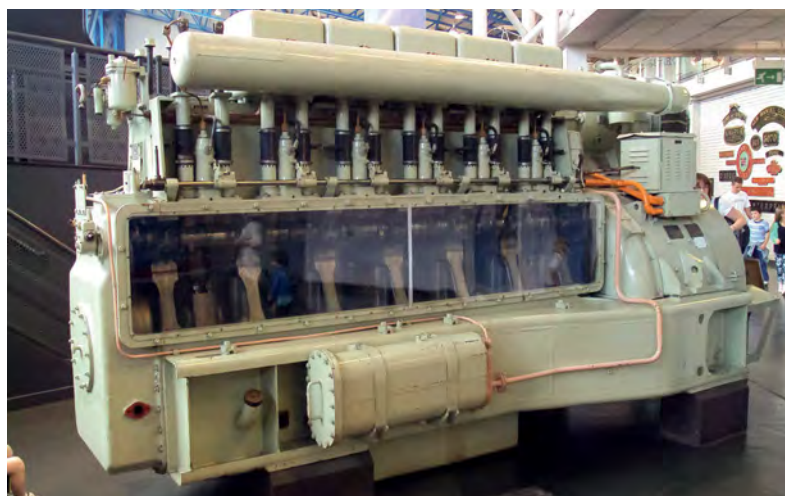
A partly sectioned Sulzer 6LDA28 straight six diesel engine on display at the National Railway Museum, York. (Wikipedia Commons/ReptOn1x)
