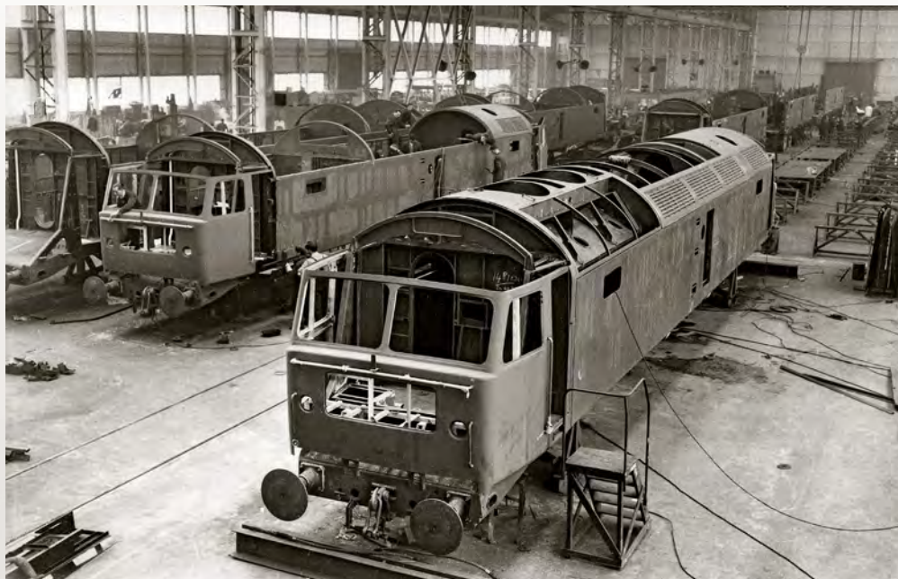
Several Type 4 bodyshells under construction at the Brush Falcon Works in Loughborough in the early 1960s. (Colin Marsden Collection)
