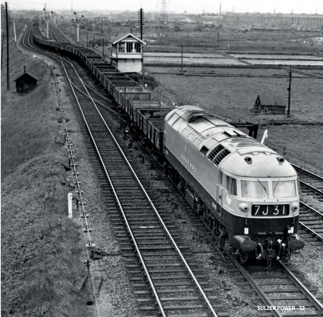
BELOW: In May 1968 HS4000 powered a 670-ton test train between Crewe and Carlisle during a series of high output tests. The highlight was the demonstration of its ability to top Shap at an impressive 46mph with 20 coaches in tow. (Colin J Marsden collection)
