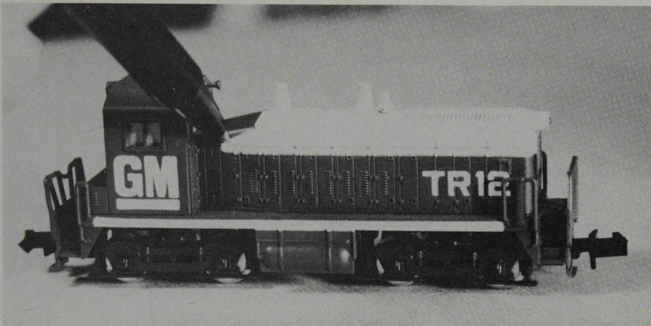
Fig. 8-21A Another loco that lends itself to easy conversion to HO narrow gauge is the Atlas/Rivarossi SW-1 switcher. I bought this one at a swap meet for $7 in perfect shape, while a new one would be about $35. Measure the HO cab and cut out the stock cab accordingly. Cut less from the area than you need to, and file to fit later. It's always easier to take away material than to add it if you made an error.
