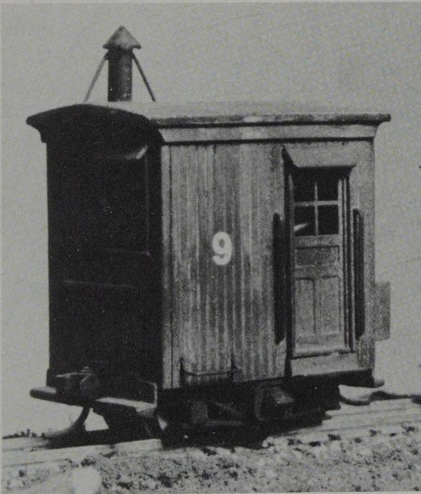
Fig. 7-11 The planking on the sides of this caboose was done by scribing styrene with an X-Acto knife.
