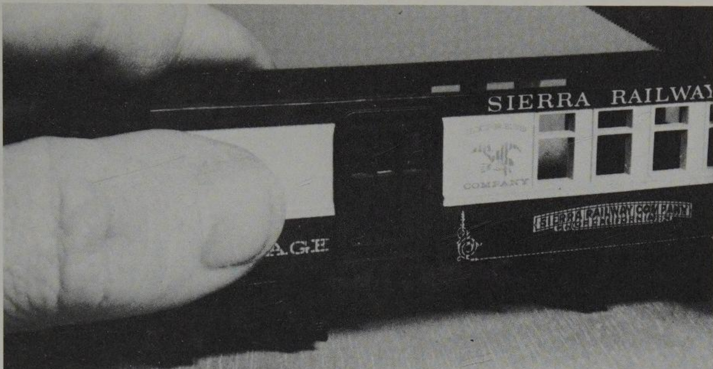
Fig. 8-26A The MDC Sierra combine has been the basis for many of my favorite conversions. I like the short look as popularized on the Gorre & Daphetid and the real Sierra Railway. This necessitates cutting the body between the first two windows and an equal amount at the rear section for balance.
