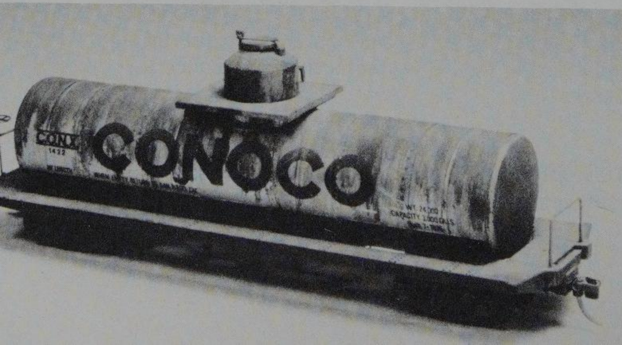
Fig. 7-7 A flat car can be the basis for an interesting tank car. Here a standard AHM tank with a platform has been added.
