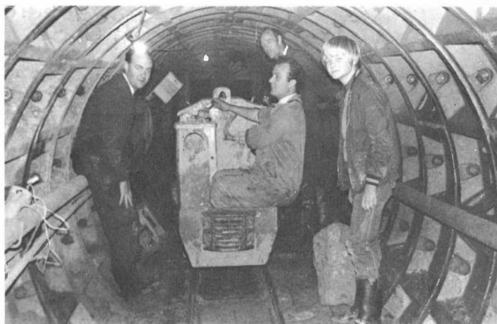
N.G.R.S. N. Staffs area visit 30.9.72. The party underground & inspecting Clayton 5792 (1970), a 1ft 6ins gauge four wheel battery electric.
