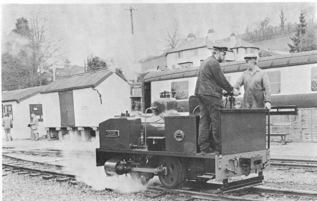
After being named DOUGAL the previous day, 0-4-0T AB 2207/46 is seen in use at Llanfair Caerinon on Easter Sunday last .. Note that she has been rebuilt with much larger sidetanks than when at Provan gasworks. (Michael Bentley).
