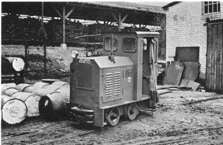
Gebr. Brill, Torfwerke Georsdorf (16), 600mm gauge. 4w-DM Diema 1991/56 stands outside the workshops on 13th April, 1975. Note the more modern all steel wagons in use here. (Brian Rumary).
