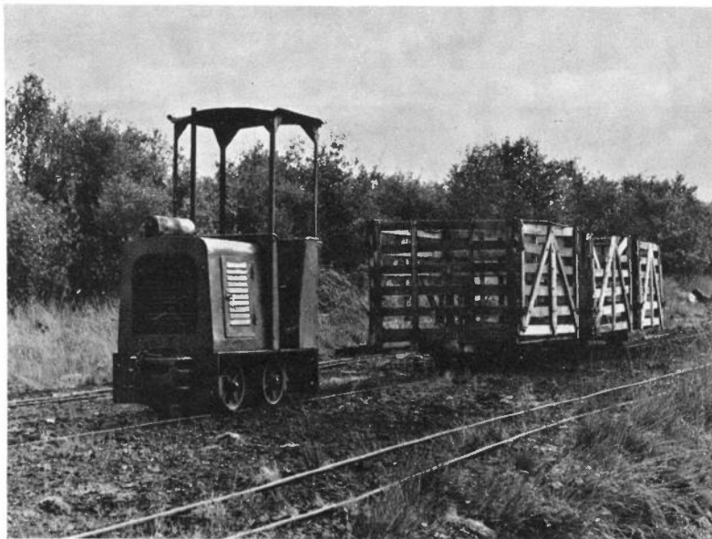
Unknown owner, Torfwerke Georgsdorf (17). 600mm gauge 4wDM Schöma 2618/62 stands on a loop line with some small wooden slatted peat wagons typical of those used at many small U.K. and German peat bog railways.
