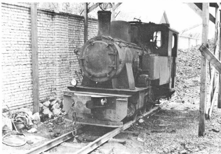
Martin Murray's article on Narrow Gauge Railways of the Polish Sugar Beet Industry did not include a photograph of a Las 0-6-0 tank. These are the largest class on Polish industrial railways, 800 being built between 1946 and 1959. Chrzanow 2762/1951 awaits the next season at Lubna on 26th May. 1976 (Bo Gyllenberg)
