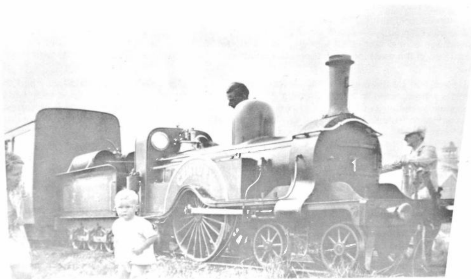
A late (c1939) photo at Jaywick showing the Polytechnic loco with the name CENTURY, which was only carried for a short period. Note brake pipe on leading buffer beam, air reservoirs on tender and brake pump on cab side. (Collection A. C. Baker)
