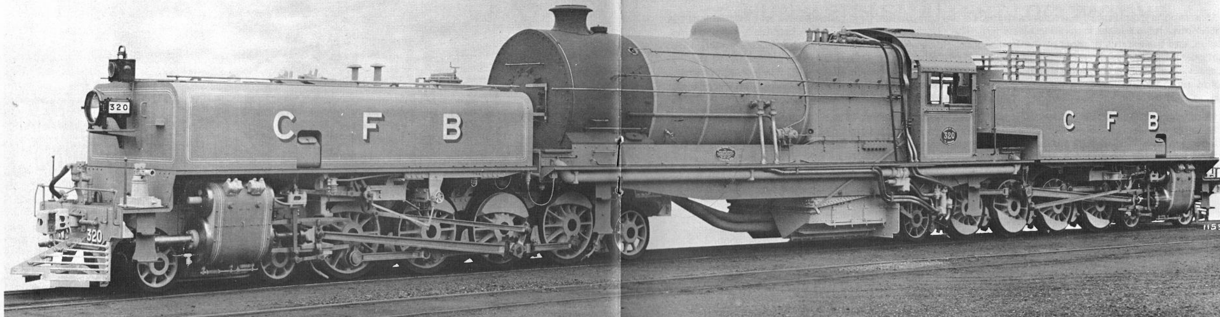
C.F.B. 320 is one of the second batch of wood-burning Beyer-Garratts supplied to the railway. These fourteen locomotives, designated class 10B, differed slightly from the first examples in having bar frames, piston valve cylinders and a small increase in heating surface. Their total weight exceeded 171 tons, but the maximum axle load was limited to 13.2 tons allowing operation on 60 lb rail. (collection R. Bridge)
