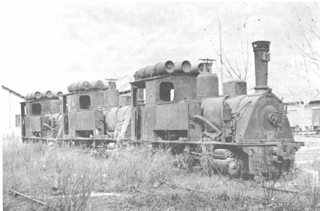
Ferrocarriles Catalanes: Three of the derelict 0-6-0 tanks at Martorell. The leading engine is lettered OG, being originally allocated to the Olván—Guardiola section. All were built by La Maquinista Terrestre y Marítima, Barcelona to a Krauss design between 1904 and 1911.
