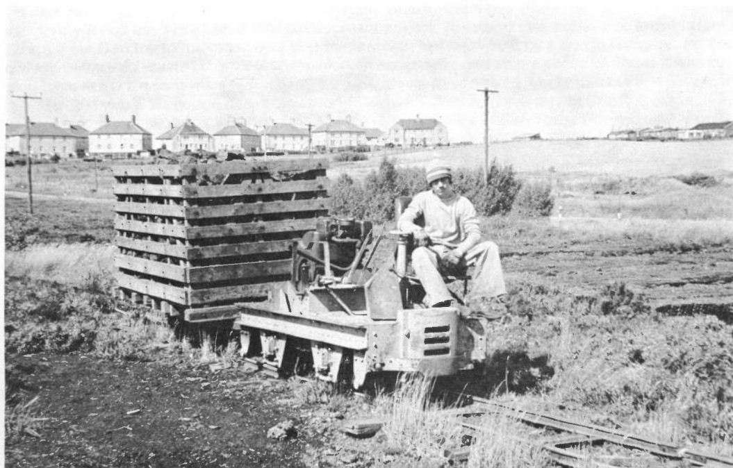
Caledonian Peat Products Ltd: Motor Rail 7512/1938, rebuilt with a Lister LD2 engine, near the mill.
