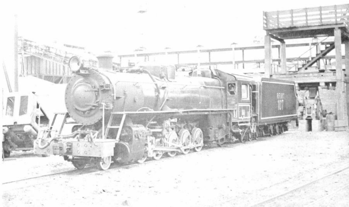
107, one of the first batch of locomotives, in store following an overhaul in the Rio Gallegos workshops. The steel pilot had not been fitted. In the background are the ship loading conveyors. (B. Roberts)
