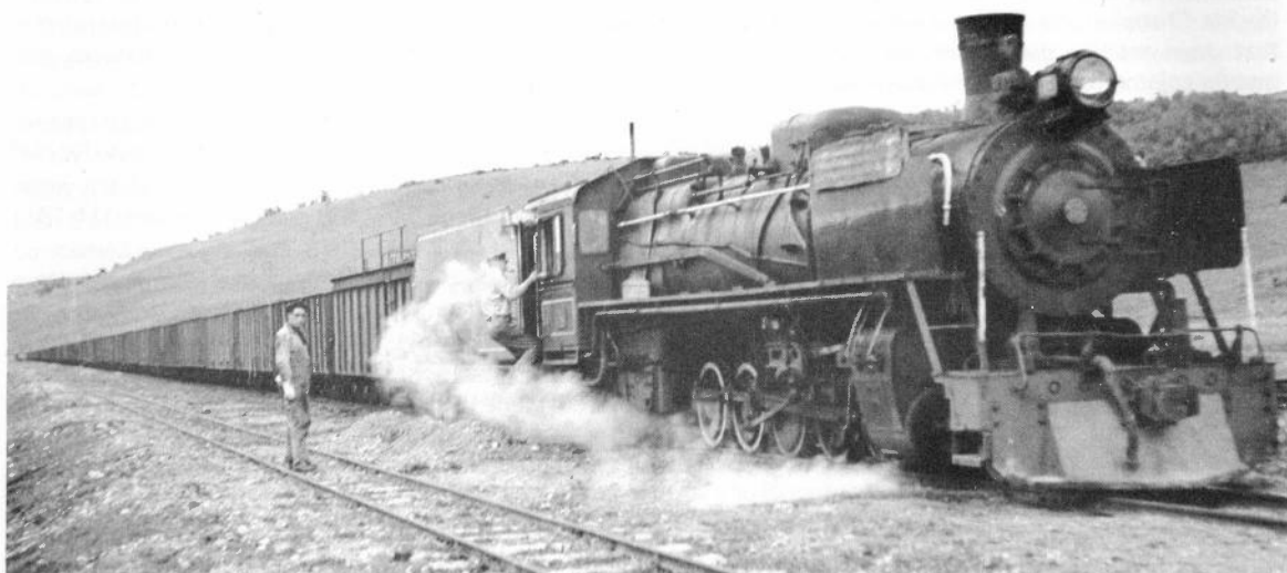
L.D. Porta climbs on board 113 before leaving with the 75 wagon test train in November 1965. The corrugated iron sheet fixed to the smoke deflector protects the smokebox vacuum and steam chest pressure gauges fitted for the tests. (N. Dudley)
