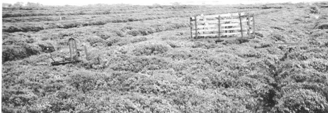
The loco frame and a wagon almost submerged in heather on the derelict 2ft 8in gauge system near New Pitsligo
