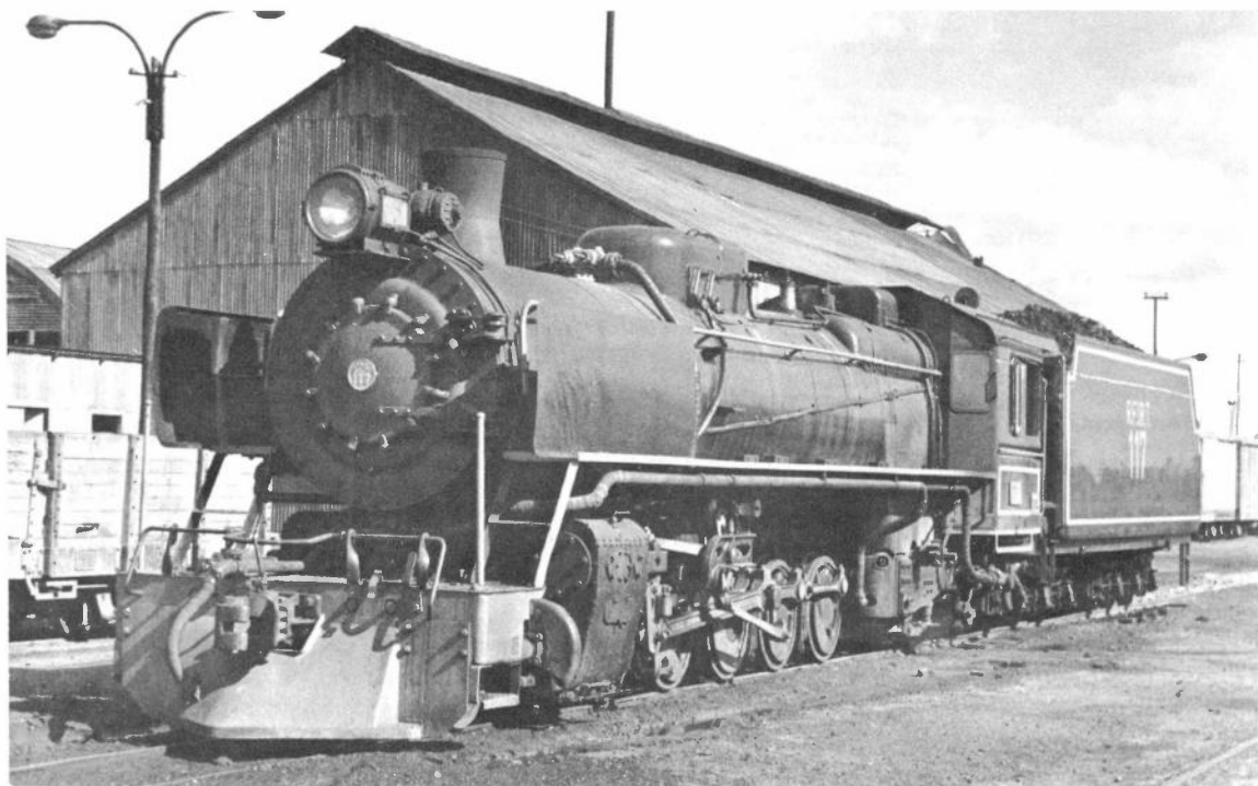
117, one of the second batch of locomotives built in 1963, stands here at Río Gallegos and shows many of the modifications applied by Sr Porta. The chimney shape is much less attractive, and this loco has lost the top section. The piston tail rod cover is visible, and the blank covers on the steam chest and air relief valve flange. The lagged pipe below the running
