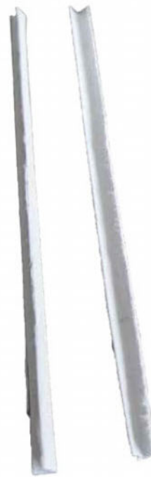
The gutters are cut with a scalpel, then coated with instant adhesive to make them rigid.
