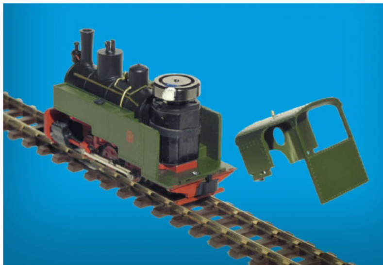
Inside the cabs, the motor with its top-mounted flywheel. The cab of the Decauville is simply clip-fitted to the running board and the water tanks.
