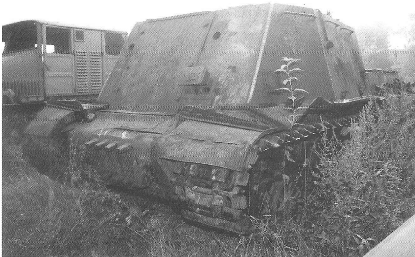
An excellent example of an ISU-T Model 1945, here shown as a Polish conversion. This particular vehicle uses a thinner gun aperture plate than on other models. The shape and thickness of these armoured covers varies from tank to tank, a result of the many field modifications. The view from the rear shows the missing opening for the tow rope, indicating that no internal winch is mounted.
