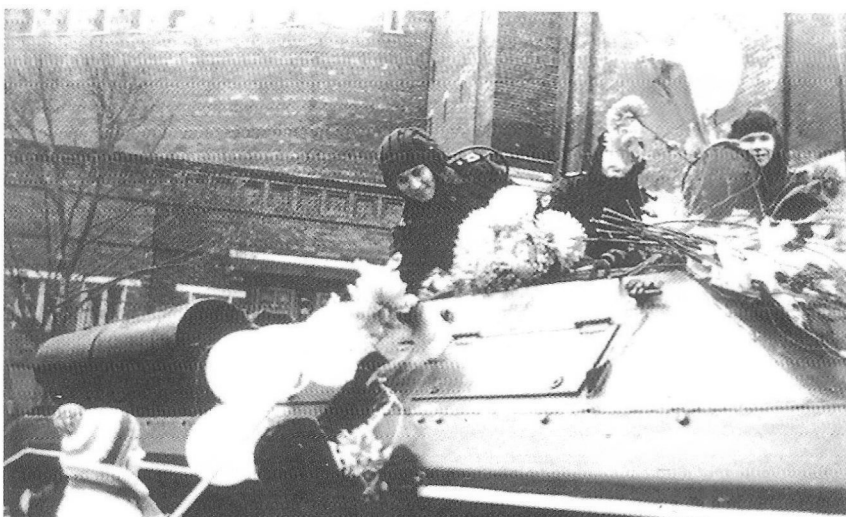
Two IS-2MT armoured tow tractors on parade in the Soviet Union. The distinctive stowage boxes and side skirts along the hull are clearly recognisable. Note the parade "markings" - wheel hubs, return rollers and the lower part of the side skirts are painted white.
