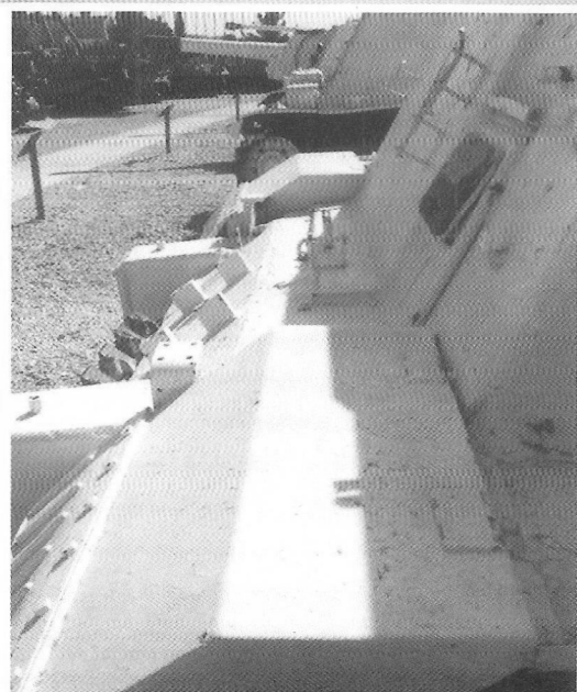
Center, right: The mount for the saw and below it for for the spade.
