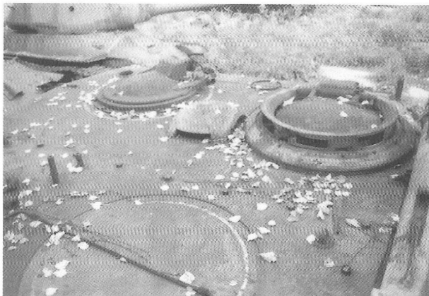
Left : The top of the superstructure of the BTT-1T with the new-type commander's and loader's hatch. The round welding seem behind them indicates an earlier attempt to mount deep fording equipment.
