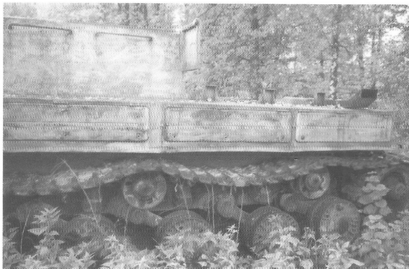
Right side of the same BTT-1T with the stowage box arrangement. Note the elongated exhaust at the rear of the engine compartment.
