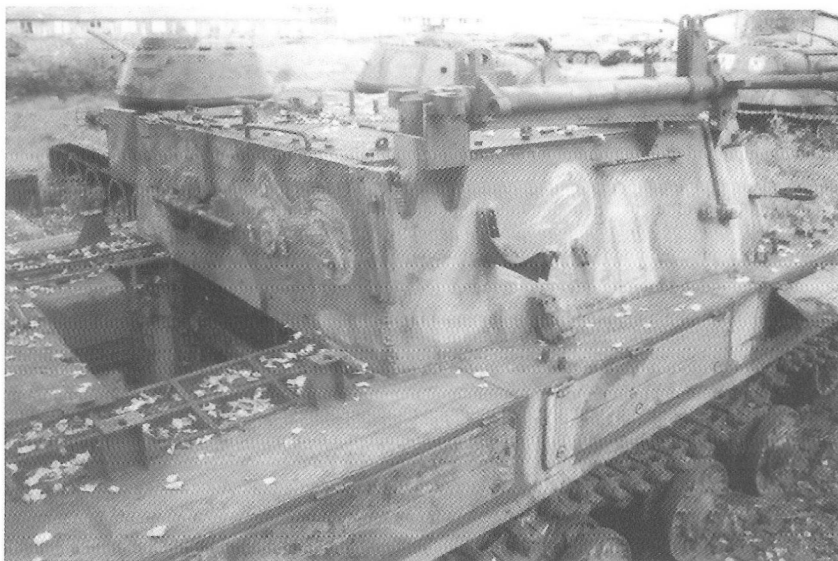
The right side of the upper superstructure with the distinctive stowage box arrangement alongside the hull plus the small jib crane. The rear stowage platform is gone, but the mounts are still recognisable. Note the absence of the winch aperture on this variant.
