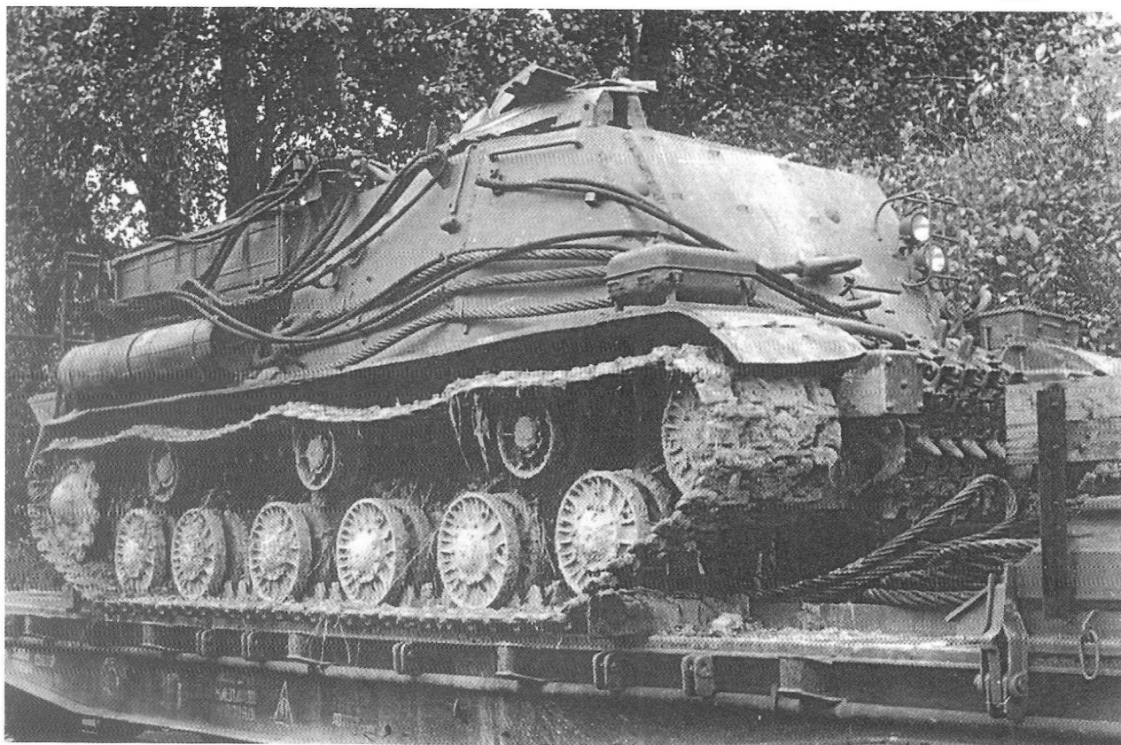
These excellent photographs of a BTT-1 on a flatbed trailer during railroad transport make identification of this ARV easy. All specialised equipment, such as the rear stowage platform, jib crane mount, rear spade, and frontal pushbars are fitted. Note the small oil canister and tool stowage box fitted to the right and left front fender, a usual application for the later versions of this vehicle. A number of tow ropes is fitted to the side and front of the superstructure, ready for quick use. (Alain Dupouy)
