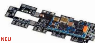
NEU 58941 LokSound 5 micro 47,5mm x 14,0mm x 4,5mm / Kato USA Widebody
