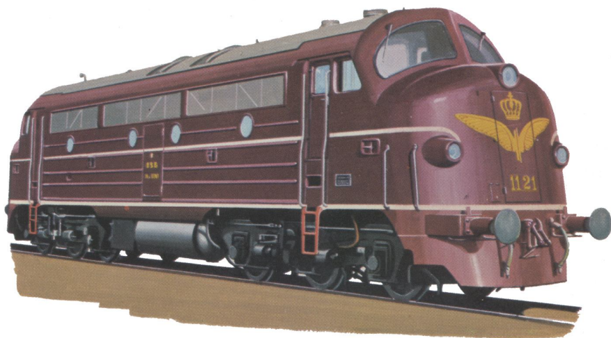
111 Danish State Railways: 1,750-horsepower diesel-electric main-line locomotive.
