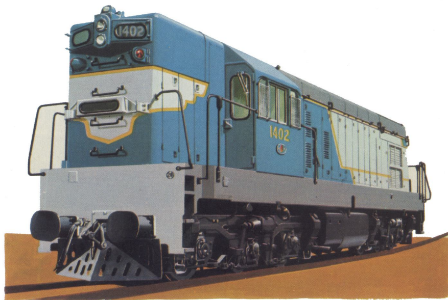
131 Queensland Railways: 90-ton Co-Co diesel-electric main-line locomotive.
