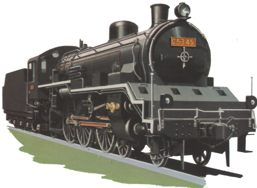
117 Japanese National Railways: the 'C53' class three-cylinder 4-6-2 express locomotive.
