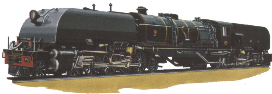
73 Rhodesia Railways: the '20th' class Beyer-Garratt 4-8-2 + 2-8-4 locomotive.
