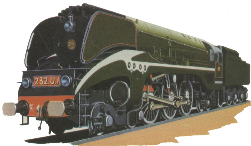
55 French National Railways: the '232.U.I' four-cylinder compound 4-6-4.
