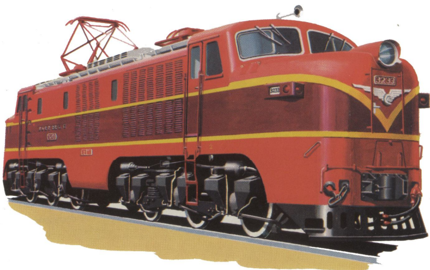
145 Chilean State Railways: Co-Co express passenger electric locomotive.
