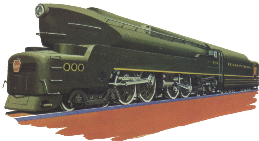
7 Pennsylvania Railroad: 4-4-4-4 express passenger locomotive of 1942.
