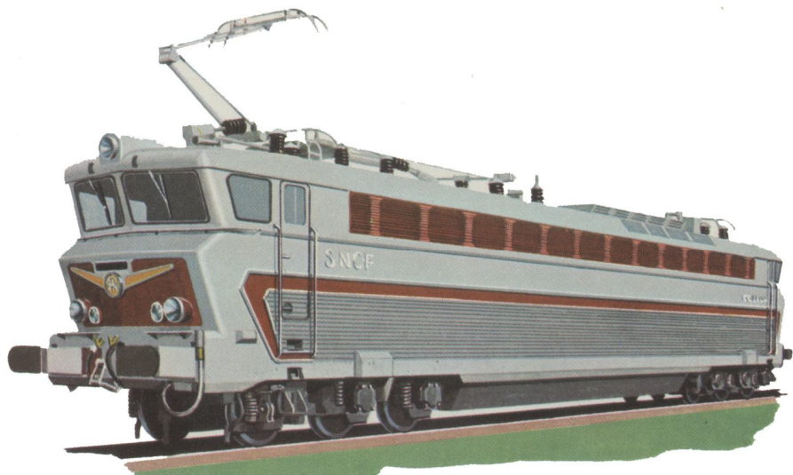
121 French National Railways: quadri-current high-speed electric locomotive.
