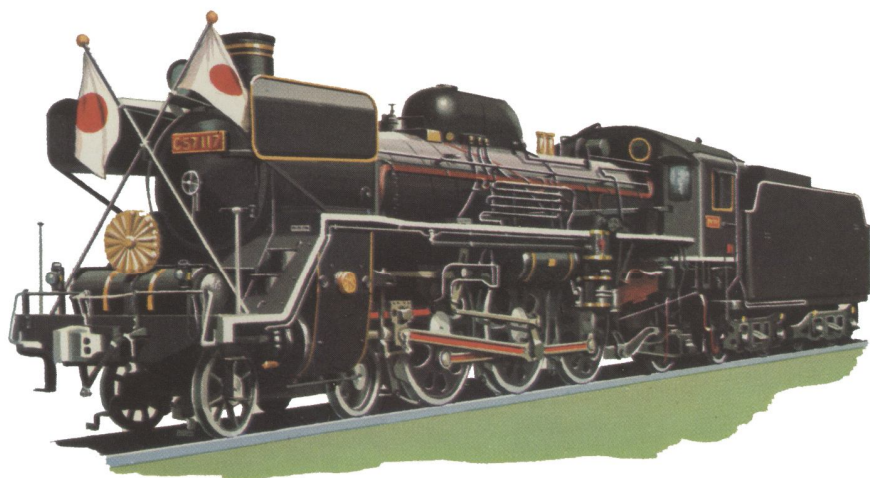
119 Japanese National Railways: the 'C57' 'light' 4-6-2 passenger locomotive.
