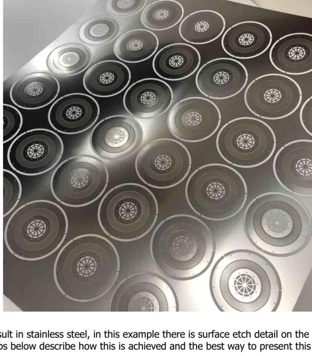
The above images show the final result in stainless steel, in this example there is surface etch detail on the front and on the back of the part, the steps below describe how this is achieved and the best way to present this in a file for etching.
