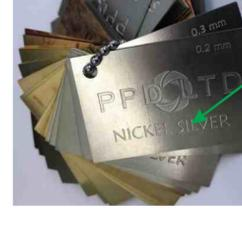
Remember to measure the width of any surface etched text, the width must be a minimum of 0.18mm.
